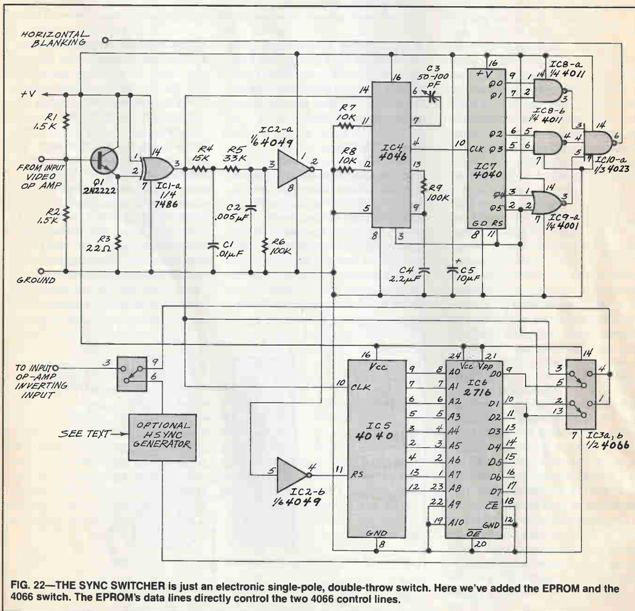
FIG. 22—THE SYNC SWITCHER is just an electronic single-pole, double-throw switch. Here we've added the EPROM and the 4066 switch. The EPROM's data lines directly control the two 4066 control lines.
