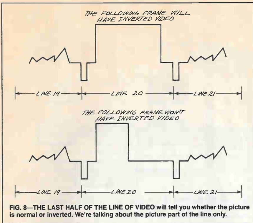
**FIG. 8—THE LAST HALF OF THE LINE OF VIDEO** will tell you whether the picture is normal or inverted. We're talking about the picture part of the line only.
