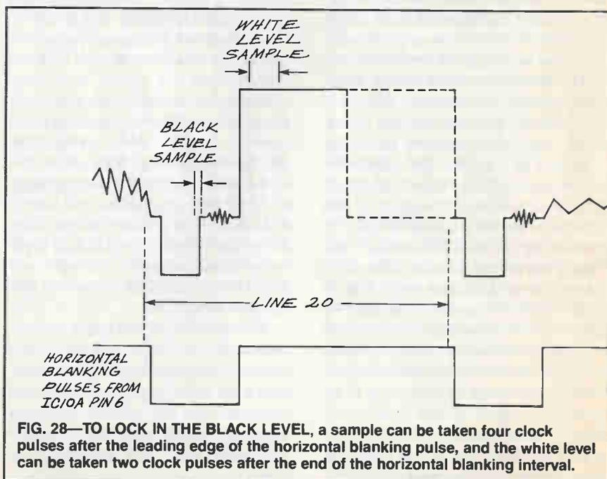
FIG. 28—TO LOCK IN THE BLACK LEVEL, a sample can be taken four clock pulses after the leading edge of the horizontal blanking pulse, and the white level can be taken two clock pulses after the end of the horizontal blanking interval.
