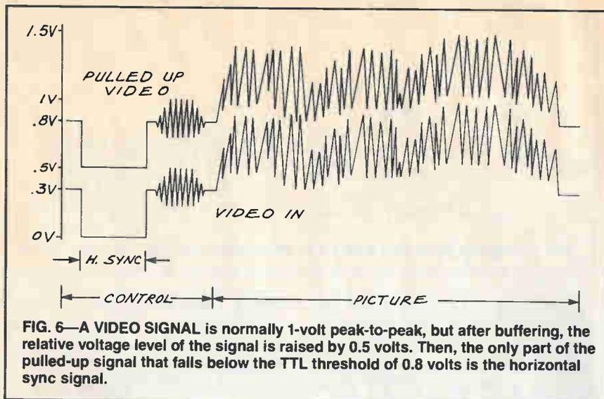
**FIG. 6—A VIDEO SIGNAL** is normally 1-volt peak-to-peak, but after buffering, the relative voltage level of the signal is raised by 0.5 volts. Then, the only part of the pulled-up signal that falls below the TTL threshold of 0.8 volts is the horizontal sync signal.
