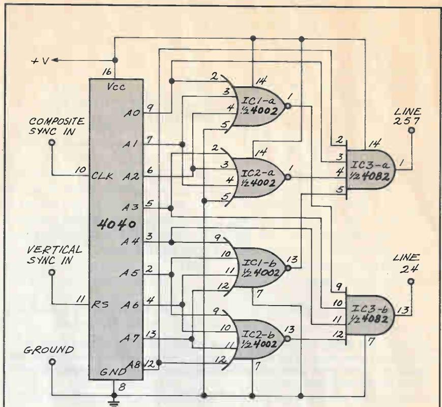
FIG. 30—MANY READERS SENT IN ALTERNATIVES to the EPROM decoding scheme I used to detect lines 24 and 257. This one uses only three chips.
