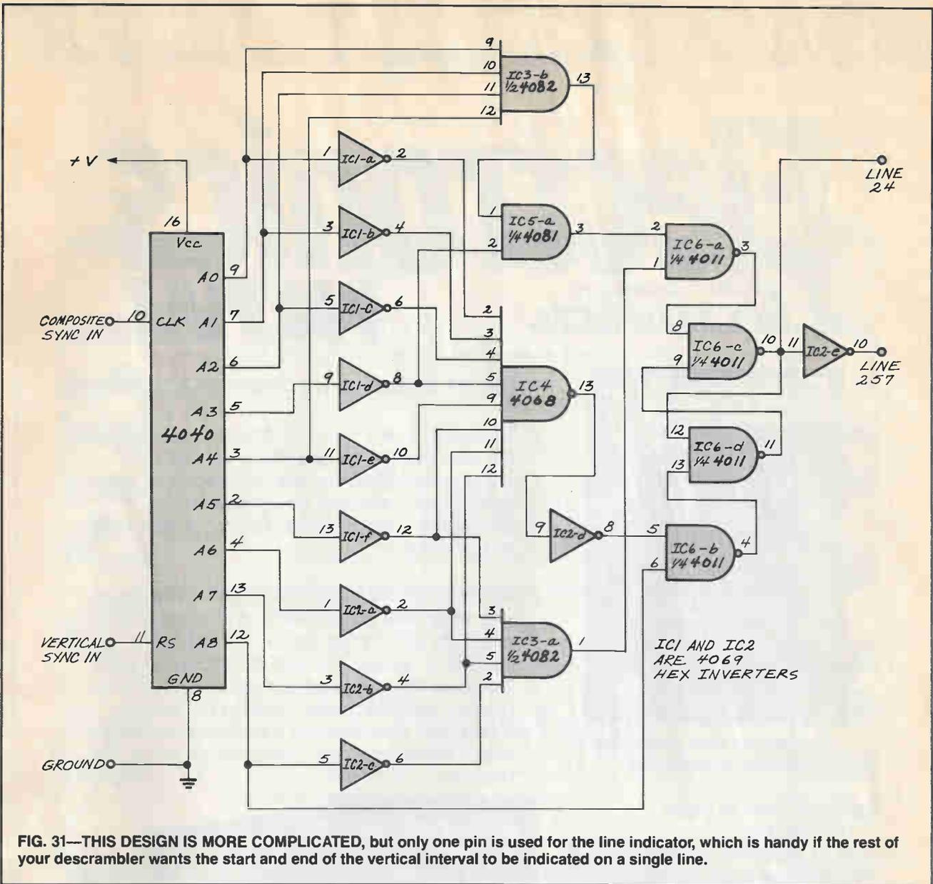
FIG. 31—THIS DESIGN IS MORE COMPLICATED, but only one pin is used for the line indicator, which is handy if the rest of your descrambler wants the start and end of the vertical interval to be indicated on a single line.
