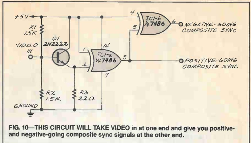
FIG. 10—THIS CIRCUIT WILL TAKE VIDEO in at one end and give you positive- and negative-going composite sync signals at the other end.
