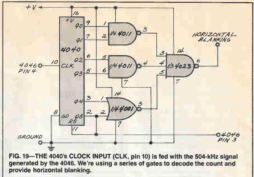
FIG. 19—THE 4040's CLOCK INPUT (CLK, pin 10) is fed with the 504-kHz signal generated by the 4046. We're using a series of gates to decode the count and provide horizontal blanking.
