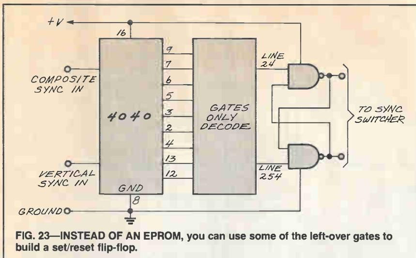
4040 counter signals the arrival of either line 24 or line 257. If you use gates to decode the counter output, you'll have to find a way to do the same thing. One approach would be to use some left-over gates to build a set/reset flip-flop whose control lines are triggered by the arrival of lines 24 and 257. The basic idea to effect this desired action is outlined in Fig. 23.
