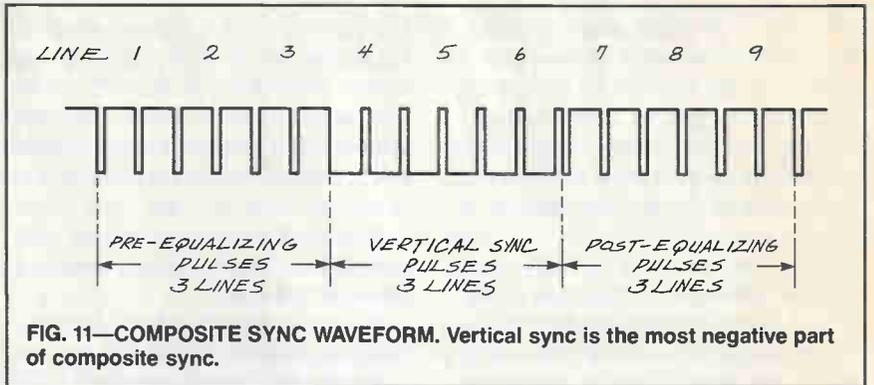
FIG. 11—COMPOSITE SYNC WAVEFORM. Vertical sync is the most negative part of composite sync.
