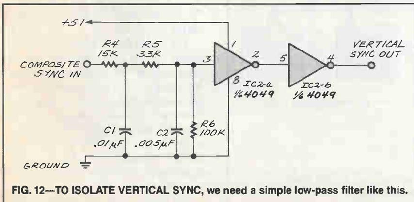
FIG. 12—TO ISOLATE VERTICAL SYNC, we need a simple low-pass filter like this.
