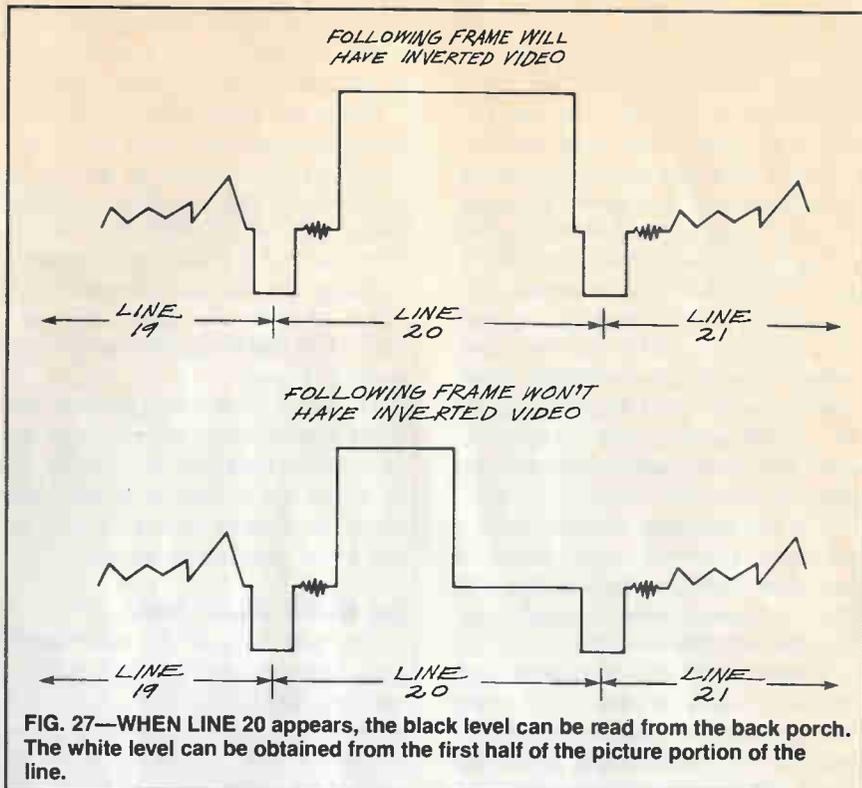
FIG. 27—WHEN LINE 20 appears, the black level can be read from the back porch. The white level can be obtained from the first half of the picture portion of the line.
