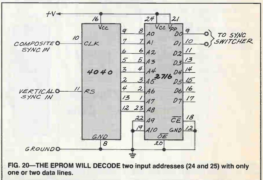
FIG. 20—THE EPROM WILL DECODE two input addresses (24 and 25) with only one or two data lines.
