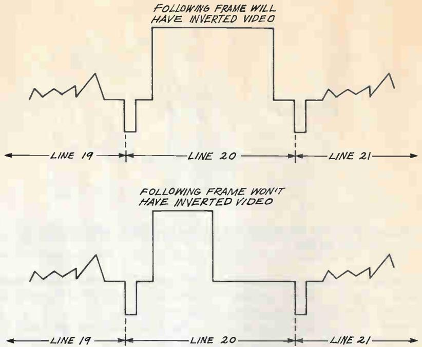
**FIG. 25**—TO CORRECT inverted video, we need the information buried in line 20.
