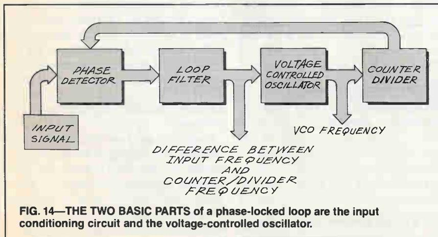
FIG. 14—THE TWO BASIC PARTS of a phase-locked loop are the input conditioning circuit and the voltage-controlled oscillator.
