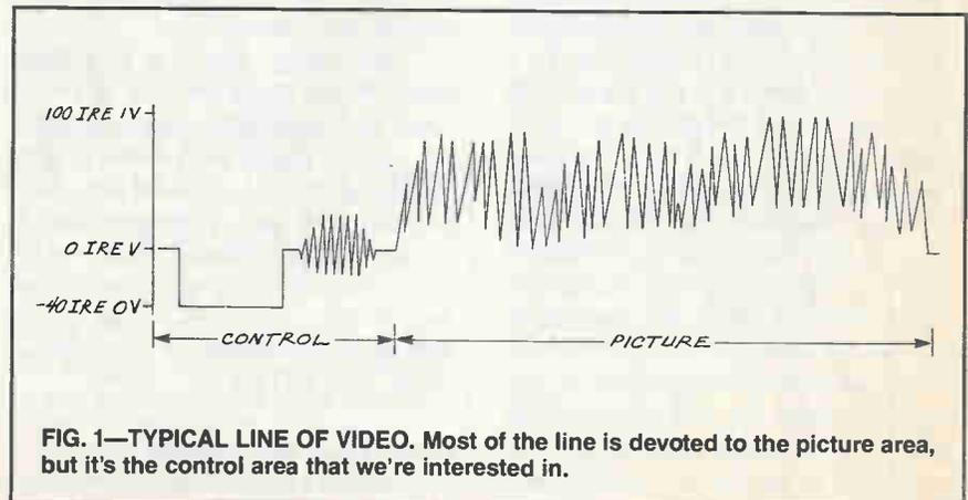
FIG. 1—TYPICAL LINE OF VIDEO. Most of the line is devoted to the picture area, but it's the control area that we're interested in.
