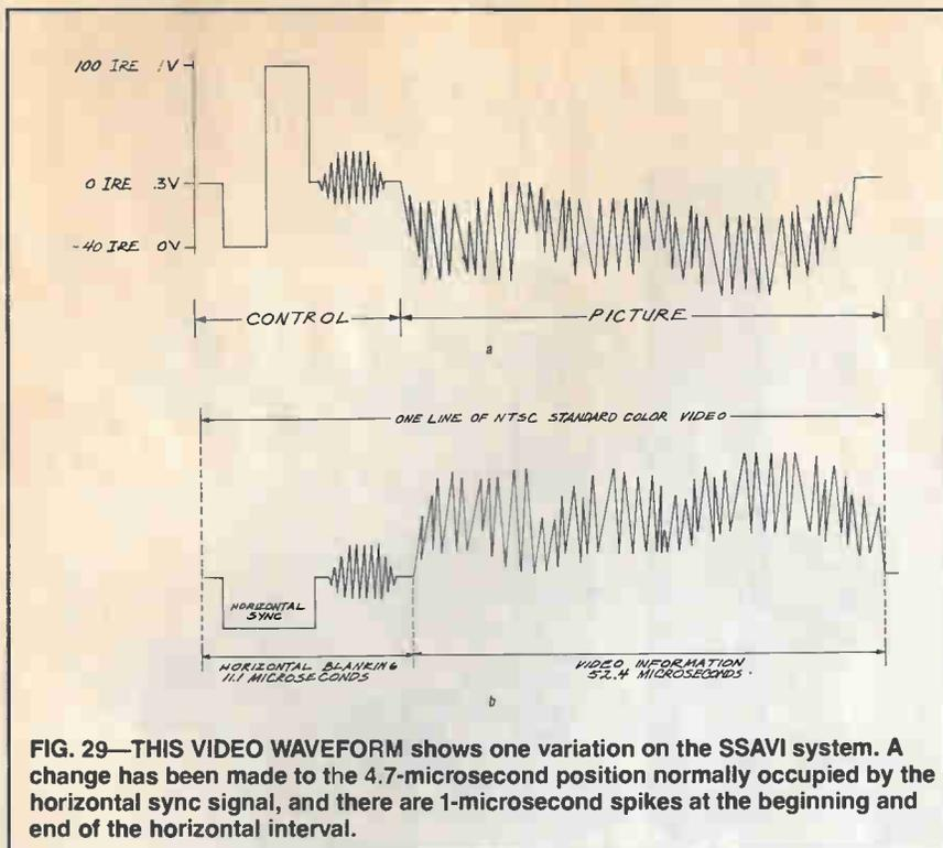
**FIG. 29—THIS VIDEO WAVEFORM** shows one variation on the SSAVI system. A change has been made to the 4.7-microsecond position normally occupied by the horizontal sync signal, and there are 1-microsecond spikes at the beginning and end of the horizontal interval.
