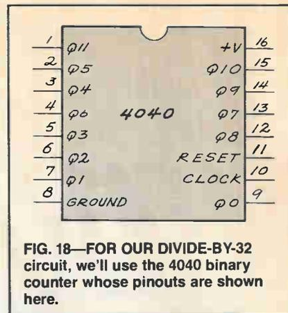
**FIG. 18—FOR OUR DIVIDE-BY-32 circuit, we'll use the 4040 binary counter whose pinouts are shown here.**
