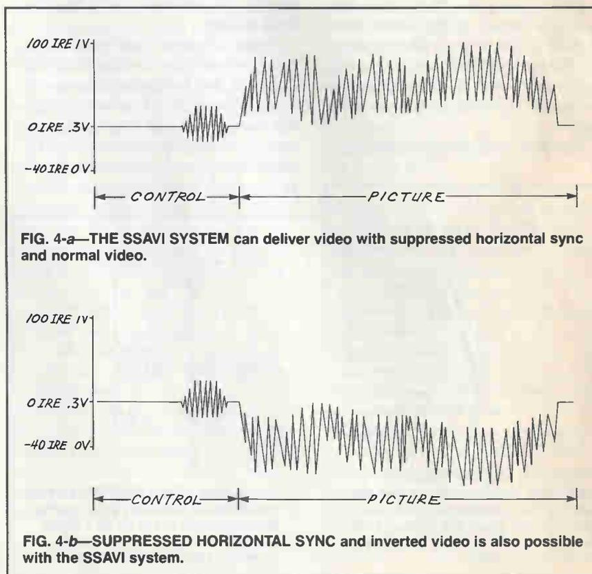
FIG. 4-a—THE SSAVI SYSTEM can deliver video with suppressed horizontal sync and normal video.
