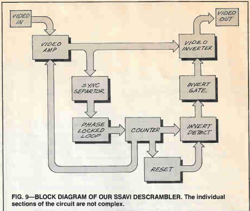
FIG. 9—BLOCK DIAGRAM OF OUR SSAVI DESCRAMBLER. The individual sections of the circuit are not complex.
