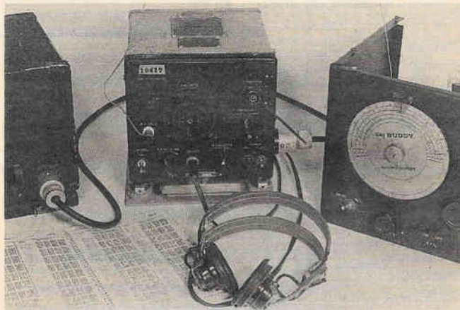
Here's the LM21 at work providing alignment signals for the Sky Buddy repair project. The power supply is at left; the calibration book is partially under the headphones (which are used to zero-beat the frequency-meter output with the signal from the internal reference crystal).
