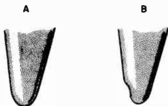
Fig. 522-a,-b. Good needle (a) and worn needle (b).
