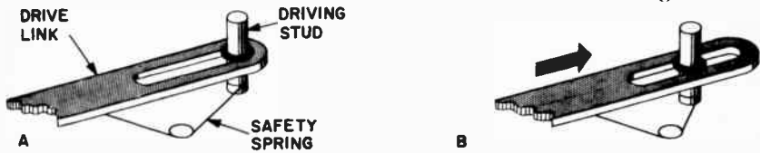
Fig. 908-a, b. Drive-link safety drive. A spring holds the driving stud in position.
