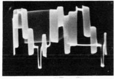
This photo shows the pulse adjusted to the correct width. To meosure pulse widths, remember that there are 63.3 microseconds from the leading edge of one pulse to the leading edge of the next. By counting squares on the screen graticula, pulse widths may be measured with sufficient occuracy for service work.
