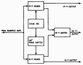
Fig. 409. In the (R-Y) (G-Y) demodulation system, a circular pattern is obtained in the test of Fig. 408 when the two demodulators are fed subcarrier signals which differ in phase by 146°.
