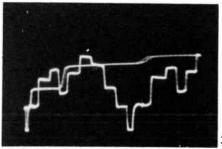
The absolute level still remains to be set. The photos show the effect of varying the blue Y gain control.
