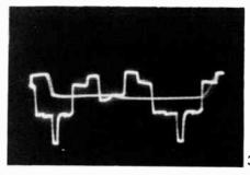
The blue Y gain control (photos 33, 34 and 35) is then varied to make the blue bar occupy 11 squares on the grailcule, and the relative proportions of the Y signal are then correct.
