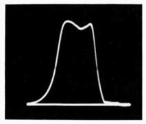
Fig. 322. Influence of the color-intensity control setting on the shape of the bandpass amplifier response. (A) Control at maximum. (B) Control at minimum.
