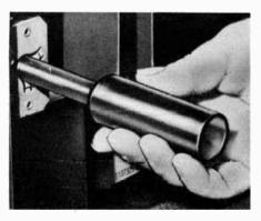
Fig. 105. A tubular high-voltage cheater. (Courtesy of Walsco.)
