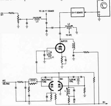
Fig. 207. Typical circuit arrangement for a color subcarrier oscillator, buffer stage and reactance-tube circuit. L1 is the oscillator plate tank coil; L2 is the buffer plate coil and L3 is the quadrature coil. (Courtesy of Motorola, Inc.)
