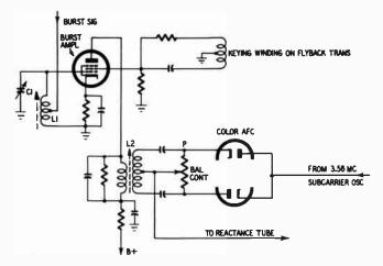
Fig. 208. Burst amplifier and color afc circuits.
