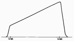
Fig. 608. A rising frequency characteristic in the bandpass amplifier can be used to compensate for a nonuniform if characteristic.
