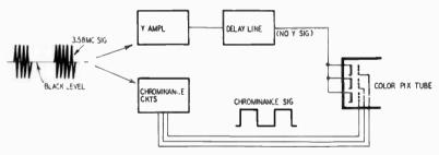
Fig. 339. When the 3.58-mc component of the applied signal has no Y (crankshaft) component, the Y amplifier is not energized. Only the chrominance circuits are energized. The Y component is artificially produced at the picture tube by advancing the brightness control. Under this condition, the color-difference bars always register perfectly with the black bars. A check of the delay line is not obtained.
