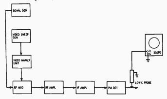
Fig. 612. Test setup to check the overall response with a video-modulated picture carrier.
