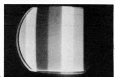
The cantrals can also be set on the basis of a chrominance signal as abserved on the screen of a wide-band scape. However, same service technicians prefer the picture-tube display and believe that it provides a claser check an bar widths than does a scape.
