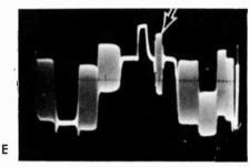
The burst now has a greater amplitude than that of the photo marked D.
