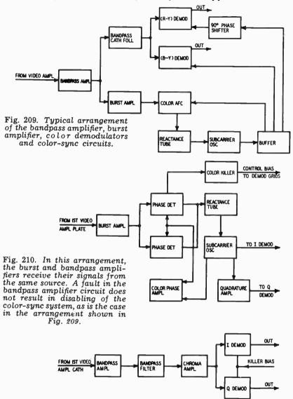
demodulators but the burst amplifier derives its signal prior to the bandpass amplifier. Thus, in Fig. 210, a fault in the bandpass amplifier does not affect operation of the color sync circuits but will affect color reproduction. In Fig. 209, a fault in the bandpass
