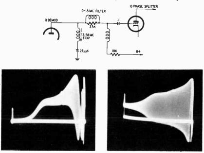
Fig. 308. Typical circuit arrangement of a Q demodulator circuit. The photo at the left shows the response obtained when using a demodulator probe. The photo at the right is the response when using a low-capacitance probe.
