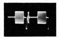
Fig. 213. Scope test shows whether pulse is positive- or negative-going.
