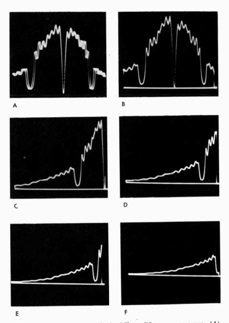
Fig. 323. Progressive steps in check of Y amplifier response curve. (A) Response curve with retrace unblanked, but sweep phasing control properly adjusted. (B) Retrace converted to zero-volt reference line. (C) Zero-frequency point tuned to right-hand end of base line. (D) Generator dial moved through 1.65 mc to locate 1.65-mc point on Y response curve. (E) Generator dial moved through 2.65 mc. (F) Generator dial moved through 3.58 mc to check color-subcarrier trap frequency.
