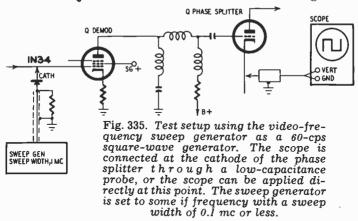
center frequency of the sweep generator can be set to any convenient value, such as 10 mc or 20 mc.
