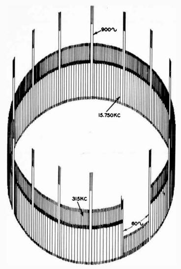
Fig. 909. Composite video crosshatch pattern.
