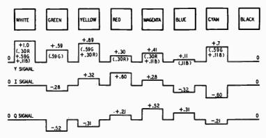
Fig. 506. The Y, I and Q signal voltages developed when scanning a 100%-saturated color bar pattern. The Y signal is the same as in (R-Y) (B-Y) transmission.
