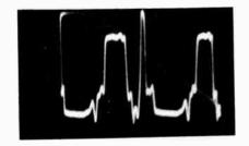
This is the reproduction of an (R-Y) bar through a peaked bandpass amplifier. The (R-Y) demodulator in this case has a gradually rounded characteristic.
