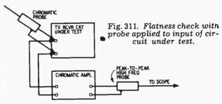
If there is excessive capacitance across the input of the circuit in the receiver under test, high frequencies will be attenuated. Under normal circumstances the circuit capacitance will not be sufficiently large to attenuate the high-frequency response to any appreciable extent. However, if an incorrect test point is selected for application of the sweep voltage, this difficulty may be encountered in a normally operating receiver.
