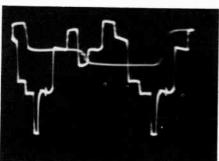
The green Y gain control may be adjusted first, and the effect of varying this control is shown in the accompanying photos (27, 28 and 29).
