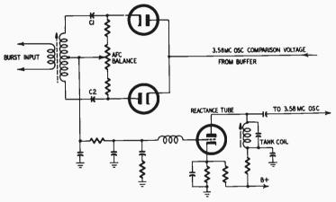
Fig. 217. Defects in the color afc phase detector and in the reactance-tube circuit can cause failure of the 3.58-mc oscillator.
