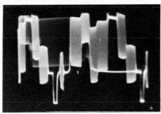
The burst width (photos 3, 4 and 5) is also adjustable in most coses. In this photo the burst width is set to minimum.
