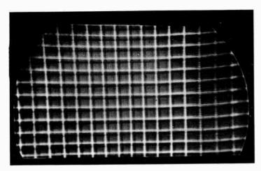
Fig. 111. Crosshatch pattern displayed on misconverged picture tube.
