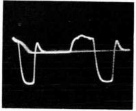
Output from Q detector; considerable contamination of Q bar with voltage from the I bar; I bar extends upward in photo; Q extends downward. Contamination is caused by misadjustment af calor phasing control.
