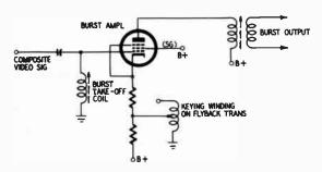
Fig. 203. The burst amplifier is keyed by a gate pulse from the sweep section.
