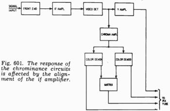
rf and mixer stages without attenuation but the relatively narrow bandpass of the if amplifier in a black-and-white receiver attenuates the 3.58-nic signal somewhat, without greatly affecting the Y signal, most of which is lower in frequency. The color signal is further at-
