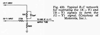
the grid of the matrix tube checked with a scope for their required fractions, two tests are required and the proper proportions must either be remembered or looked up in a text. On the other hand, application of a (G-Y) /90° signal to the receiver requires only one check and the result is shown in the form of a simple null (or the lack of it, in the event of trouble).
