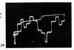
Since the omplitude of the green-bor Y component is 0.59, it is convenient to odjust the verticol goin of the scope so that the green bor occupies 59 squares. See photos 30, 31 and 32.
