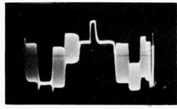
This photo shows no burst signal on the back porch of the blanking signal.
