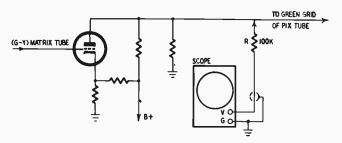
Fig. 509. An isolating resistor is unsuitable for matrix tests; a low-capacitance probe should be used instead.
