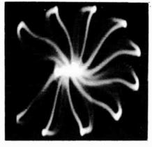
Fig. 414. Vectorimeter pattern. The vectors will rotate when the color phasing control is turned.
