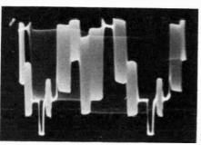
Most color bar generators provide a burst gain control. This affects the burst voltage as shown in the photos.
