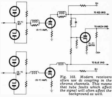
Hence, the (G - Y) matrix tube must be replaced anyhow, and the green background and screen controls must then be readjusted to neutralize the raster on black-and-white reception. Always assume at the start that the receiver is capable of normal operation if a faulty tube or two can be located and replaced. This approach will usually save a great deal of time.
