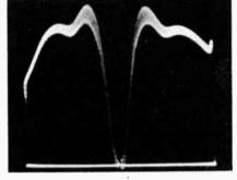
each square indicates an interval of 0.1 mc. Frequency points are then determined at any desired point along the response curve by counting squares and multiplying by 0.1 mc.
