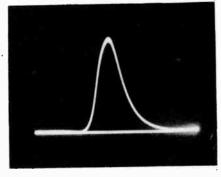
reference waveform drops to a small fraction of its former value (Fig. 813) and we conclude that, although the test with the signal-tracing probe suffices to show whether the signal is present or absent at this point, the test does *not* serve to show the stage gain.
