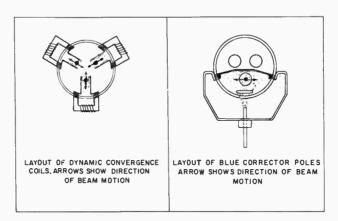
Fig. 709. Layout of dynamic convergence coils and magnetic vanes. (Courtesy of Motorola, Inc.)
