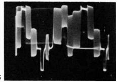
In adjusting bar widths, the controls may be set an the basis af a pattern an the screen af the calar picture tube. (See phatas 6 and 7).
