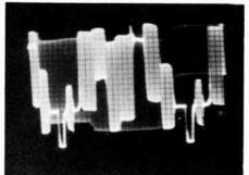
The correct height of the sync pulse is the some os the burst height.
