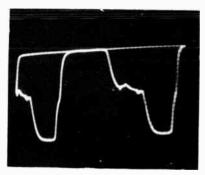
Output from Q detector; again, considerable contamination of Q output with I output. The Q bar is the longer of the twa downward excursions. Contamination is caused by misadjustment of the color phasing cantrol.
