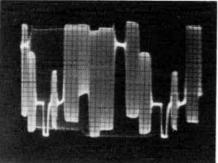
Photos 36, 37 and 38. The overall chroma gain control and overall Y gain control are adjusted to bring the peak of the subcarrier in the green bor exactly even with the blanking level.
