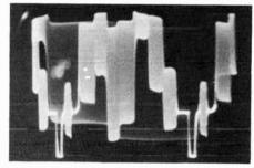
These photos (18, 19 and 20) show the effect on the white-bar subcarrier of varying the red-bar saturation contral.
