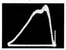
still remains the interleaved monochrome signal in this band from 2.1 to 4.2 mc. The output from the chroma bandpass amplifier accordingly consists principally of the mixed I and Q signal voltages.
