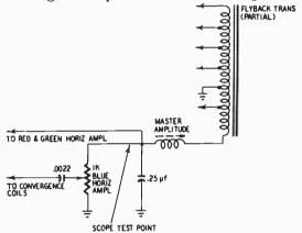
Fig. 705. Misadjustment of the master amplitude control may burn out the 1,000-ohm potentiometer.
