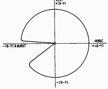
Now, consider the situation in which the quadrature transformer is misadjusted in the TV receiver so that the two subcarrier voltages fed to the color demodulators are no longer in quadrature. In such a case, the scope displays an elliptical pattern (Fig. 406), and no possible adjustment of the scope gain controls can make a circle out of it. This is the basis of the quadrature test with a linear phase sweep.
