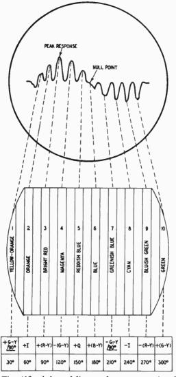
Fig. 412. A keyed linear phase sweep signal has the characteristics shown above. The scope pattern represents the (R-Y) detector output waveform.
