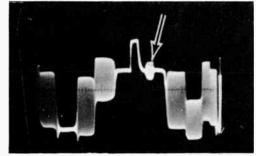
The burst signal shows a definite increase in amplitude.
