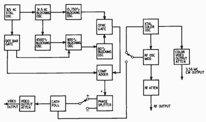
Fig. 908. Block diagram of a rainbow generator. (Courtesy of Hickok Electrical Instrument Co.).
