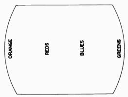
Fig. 116. A simple rainbow pattern is a spectrum of color-difference signals.
