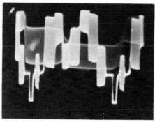
Note that when the saturation is varied, only the peak-to-peak voltage of the carresponding chrominance signal varies; the voltage of the Y component does not change.
