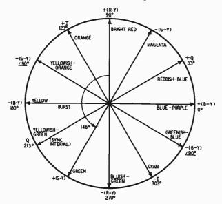
Fig. 402. As the linear phase sweep vector lags farther and farther behind the bursí phase, it progressively sweeps through all of the color-difference signals during a horizontal scan interval.
