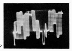
The bar sequence abserved here is: green, yellaw, red, magenta, white, cyan and blue. The bars have been adjusted to have approximately equal widths. Ta produce yellaw, the green and red bars are averlapped. Magenta is abtained by averlapping red and blue. Cyan is produced by overlapping green and blue. White requires three calars—red, green and blue. (See phatas 8, 9 and 10).
