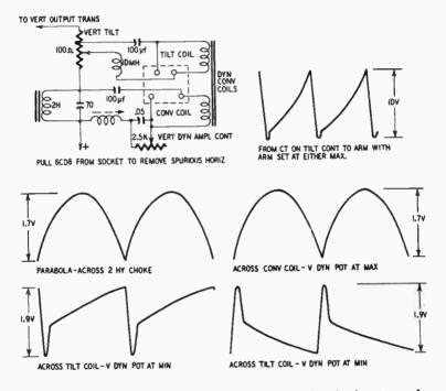
Fig. 711. Simplified dynamic convergence circuit in 60-cycle operation. (Courtesy of Motorola, Inc.)
