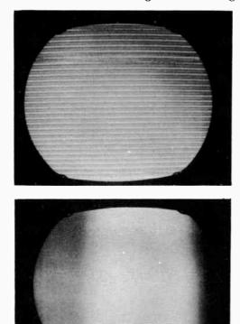
Fig. 220. Color subcarrier oscillator operating off frequency. (Above) Oscillator off frequency by 1,800 cycles. (Below) Oscillator off frequency by 15,750 cycles
