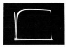
Fig. 321. (Left) With the power switch "on," the Y amplifier reflects into the contrast control, and residual ringing of the delay line is seen. (Right) With the power switch "off," plate resistance of Y amplifier tube becomes infinite, and reflection is no longer seen.
