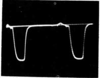
Output from Q detector, I signal nulled satisfactorily. Residual I signal is seen only as a small irregularity in the base line. The corners of the Q bars are rounded because of the relatively narrow bandpass of the Q demadulator circuit.
