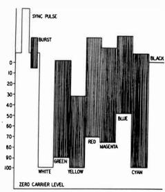
Fig. 611. The color signal places a greater demand on the dynamic range of the if amplifier than a black-and-white signal because the 3.58-component extends into the blacker-than-black region.
