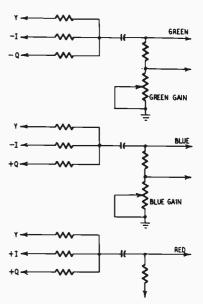
In a small number of sets (R-Y) and (B-Y) detectors are used, with a (G-Y) matrix, but the matrixing of the color-difference signals with the Y signal is not accomplished in the picture tube but in a separate resistive matrix similar to the I-Q matrix. When checked for proper matrix action, the scope is applied at the matrix input terminals instead of at the grids and cathode of the picture tube. The signals found in normal operation are the same as those of Fig. 502.
