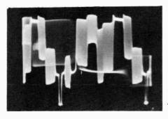
The colar bor generator usually has a sync-pulse width control. (See photos 1 and 2). This photo shows the pulse adjusted to narrow width.
