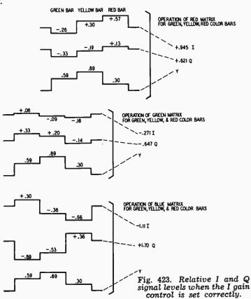
It is possible to adjust the chrominance gain controls upon the basis of color program material but again this is a poor procedure since the fidelity of a color transmission may vary somewhat from time to time and it is not possible to conclude that the gain controls are actually set exactly as they should be. Of course, when a color bar generator and scope are not available, adjustment upon the basis of the screen display is the next best procedure.
