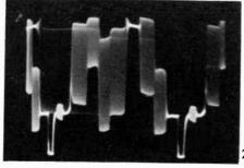
The amplitude of burst is approximately equal to one-half that of the red bar.
