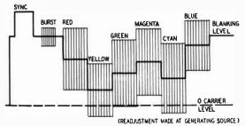
Fig. 804. Readjusted color signal for 100%-saturated color bars.
