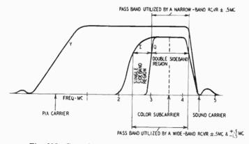
Fig. 602. Complete color signal has double- and single-sideband components within the chrominance region. Wideband receivers utilizing the single-sideband chrominance signal must be aligned to take the half-voltage level of the single sideband into consideration.
