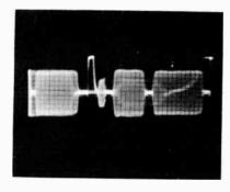
Applied color signal; this output from the color bar generator cansists of horizantal sync, burst, I and Q valtages. It is very useful in determining whether the color subcarrier is being applied in exact quadroture and whether the color subcarrier is being applied with I at 57° from burst.
