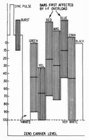
Fig. 341. Overload in if amplifier first distorts bar signals extending into black region.
