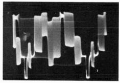
These phatos (11 and 12) show the result of varying the width of the red bar. The width of the white bar is changed, as well as the width of the cyan bar, due to the overlapping principle utilized to generate the complementaries and white.
