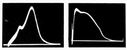
Fig. 318. (Left) Distortion of Q demodulator response when demodulator probe is applied directly at the output of the Q channel, instead of at the low-impedance point in the phase-splitter circuit following the Q channel (right).
