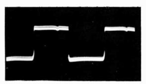
Fig. 336. Typical response of Q channel to 60-cycle square-wave voltage.
