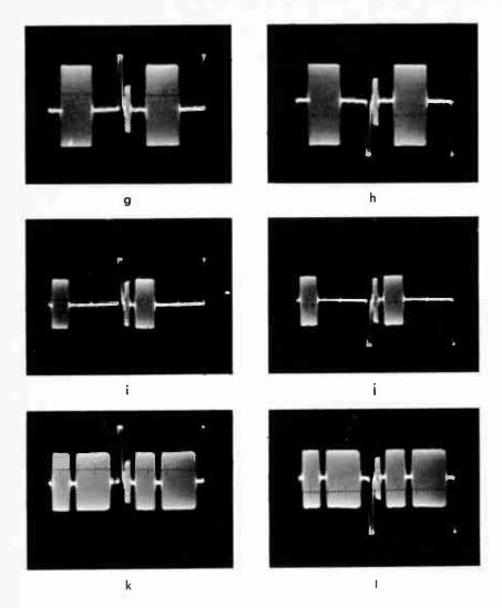
Fig. 211 (g to 1). Typical video-frequency outputs from an NTSC color-bar generator.
