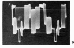
Since two green bars are utilized to synthesize the pattern, adjustment of the green bar width varies the widths of the yellow and cyan bars.
