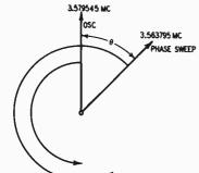
Fig. 401. A linear phase-sweep signal has a frequency which is lower than that of the color-subcarrier oscillator by 15,750 cycles. The phase-sweep vector falls farther and farther behind the oscillator, causing the angle between the two vectors to get larger and larger—thus forming a linear phase sweep.
