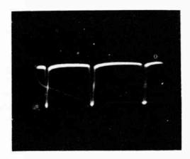
Fig. 706. Pulse excitation voltage from fly-back transformer to convergence circuits.
