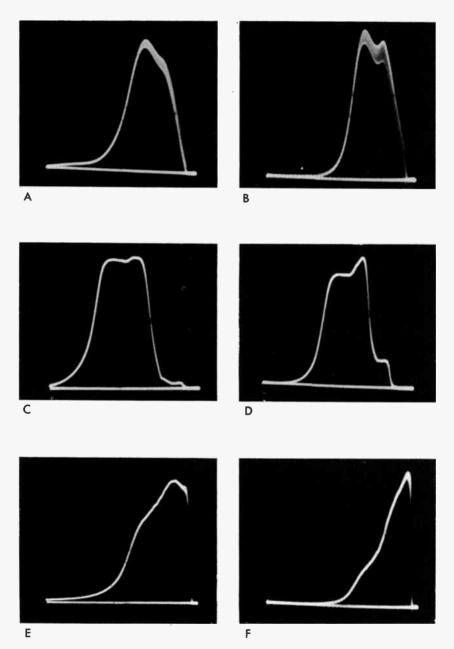
Fig. 320. (A) Response of Q demodulator at high signal level. (B) Same response curve at a low signal level. (C) Bandpass amplifier response at high signal level. (D) Same response at low signal level. (E) Green video-amplifier response at high signal level. (F) Same amplifier response at low signal level.
