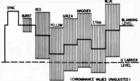
Fig. 803. Color signal corresponding to 100%saturated color bars.
