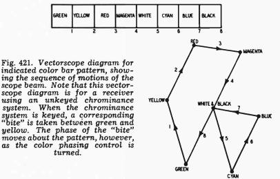
A vectorscope check of the color demodulators against a color bar signal is very informative and supplies a large amount of operating data in convenient form. When a color bar signal is applied to the receiver and the color demodulators are connected to a scope with the output from the (R-Y) demodulator energizing the vertical amplifier and the output from the (B-Y) demodulator fed into
