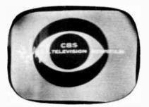
Fig. 3-L. Low-voltage B+ causes reduction in height and width.
