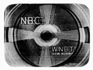
Fig. 1-J. Example of horizontal jitter.
