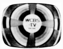
Fig. 5-P. Defect in video amplifier can produce poor-quality pix.
