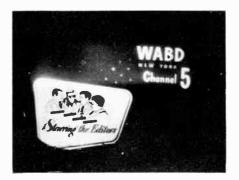
Fig. 1-D. Poor dc restoration results in a gray picture. Dc restorers are found in old receivers, many of which are still in use.
