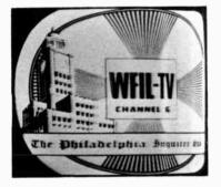
Fig. 7-H. Photo shows example of horizontal nonlinearity.
