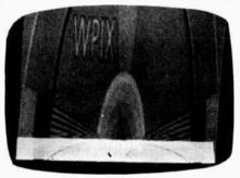
Fig. 6-F. Photo shows vertical foldover.
