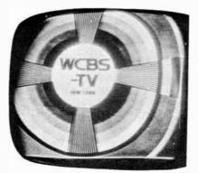
Fig. 4-C. Shifting of pix by misadjusted focus assembly.
