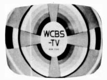
Fig. 8-D. Overdrive indicated by vertical white line.
