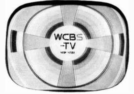
Fig. 5-R. Pix of test pattern shows echo.
