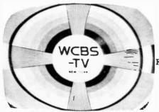
Fig. 1-L. Test pattern shows lefthand stretch.
