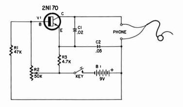
Resistors: R1-47,000 ohms; R3-4,700 ohms (both 1/2 watt); R2—50,000-ohm potentiometer. Capacitors: C1-.02 µf; C2-.05 µf (both poper tubulor). Transistor: V1-2N170, n-p-n.
