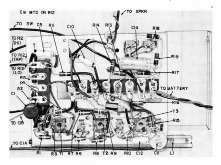
Fig. 514. Below chassis view-Basic Superhet Receiver.
