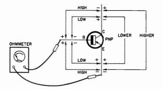
Fig. 607. Basic transistor tests with an ohmmeter.
