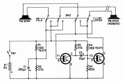
Resistors: R1, R4–1,000-ohm potentiometers; R2, R3–27 ohms, 1 watt; R5–82 ohms, 1 watt. Capacitors: C1–250  $\mu$ f; C2–20  $\mu$ f (both 6volt electrolytics). Switches: SW1–spst toggle; SW2–4 pdt, spring return, lever type. Transistors: V1, V2–2N301, p-n-p power type. Battery: B1—6 volts (4—1.5 volt cells in series).
