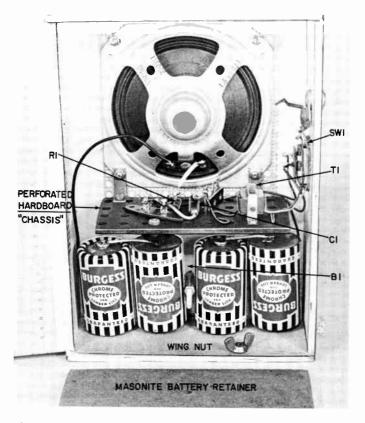
Fig. 219. Interior view of the unit shown in Fig. 218 . . . a perforated pressed-board chassis is used. Power is supplied by four flashlight cells connected in series.
