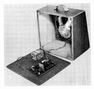
Fig. 507. Rear view of the Utility Amplifier.
