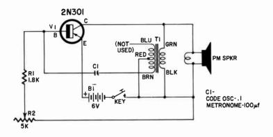
Resistors: R1-1,800 ohms,  $\frac{1}{2}$  watt; R2-5,000-ohm potentiometer. Capacitors: C1-.1  $\mu$ f, tubular (for Code Practice Oscillator) or 100  $\mu$ f (for Metronome), 6 volts, electrolytic (see text). Transformer: T1-500 ohms, CT pri, 8 ohms, sec (Argonne AR-164). Transistor: V1-2N301, p-n-p power. Battery: B1-6 volts (Burgess type Z4).
