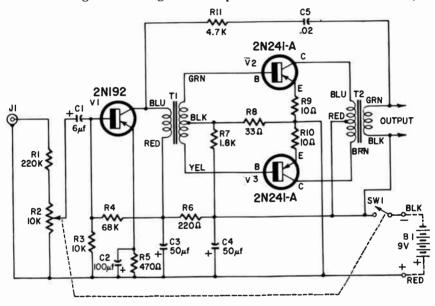
Resistors: R1-220,000 ohms; R3-10,000 ohms; R4-68,000 ohms; R5-470 ohms; R6-220 ohms; R7-1,800 ohms; R8-33 ohms; R9, R10-10 ohms; R11-4,700 ohms (all ½ watt); R2-10,000-ohm potentiometer, audio taper, with spst switch.
