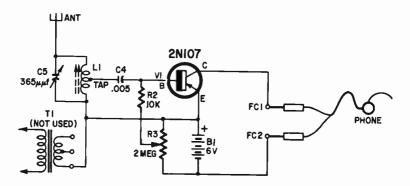
Resistors: R2—10,000 ohms, ½ watt; R3—2meg potentiometer. Capacitors: C4—.005  $\mu$ f; C5—365  $\mu\mu$ f (pf) variable.
