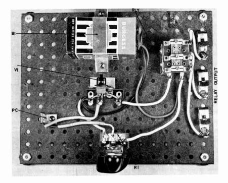
Fig. 410. The Electric Eye wired breadboard fashion.
