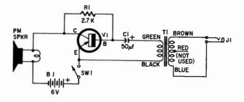
Resistor: R1-2,700 ohms, ½ watt. Capacitor: C1-50  $\mu$ f, 6-volt electrolytic. Switch: SW1-spst slide. Jack: J1-open circuit phone. Transformer: T1-500 ohms CT to 8 ohms (Argonne AR-164). Transistor: V1-2N301, p-n-p power type. Battery: B1-6 volts (4-1.5 volt' cells in series).
