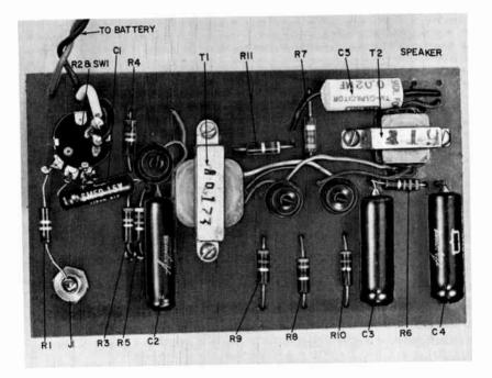
Fig. 503. Top view of the wired Basic Amplifier.
