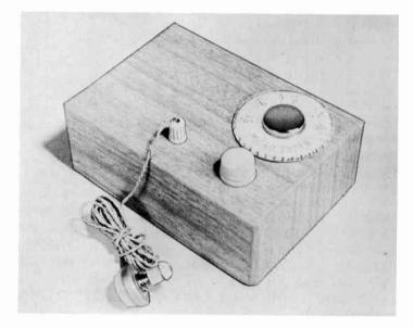
Fig. 319. The Pocket Superhet mounted in a small wooden box . . . if preferred, a plastic case may be used.
