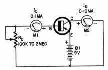
Resistor.  $R_b{--}100,000{-}ohm$  to 2-meg potentiometer. Meters:  $I_b{--}0$  to 1 ma dc;  $I_c{--}0$  to 10 ma dc.
