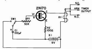
Resistors: R1-50,000-ohm potentiometer; R2-100 ohms, ½ watt. Copocitor: C1-100 μf, 15 volts, electrolytic. Switch: SWI-spdt, pushbutton (Switchcraft 103). Transistor: V1-2N170, n-p-n. Bottery: B1-9 volts (Burgess type 2N6). Reloy: RY-4,000-ohm coil, contact rating 1.5 amps, 28 vdc (Advance SO/1C/4,000D). Miscelloneous: perforated circuit board; knob; rubber feet; brackets; transistor socket; terminal strips; battery connectors; Fahnestock clips; machine screws and hex nuts; wire; solder; etc.
