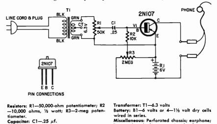
Fig. 106. Schematic of the circuit shown wired in Fig. 105. Only major components are detailed in the parts list.
