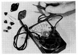
Fig. 606. Using an ohmmeter to check transistors.
