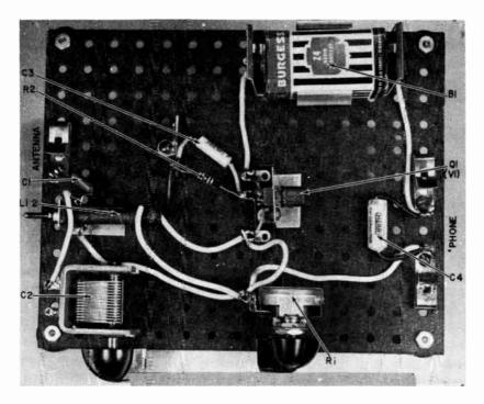
Fig. 305. The completed Regenerative Receiver, wired breadboard fashion.
