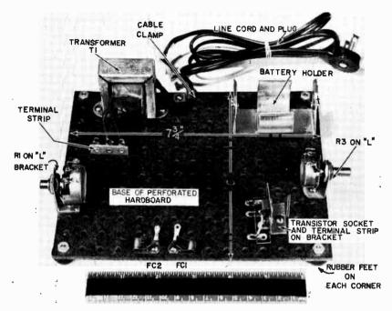
Resistors: R1—50,000-ohm potentiometer (linear taper); R2—10,000 ohms, ½ watt; R3— 2-meg potentiometer (linear taper).
