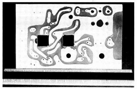
Fig. 315. Etched circuit board layout.
