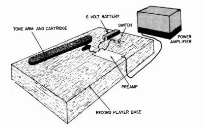
Fig. 207. How the hi-fi preamp is used. For a stereo installation, a pair of preamps is required . . . one for each channel.
