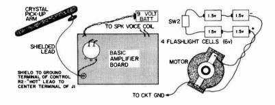
Fig. 510. Portable Phonograph wiring details-compare with Fig. 509.
