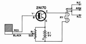
Resistor: R1-50,000-ohm potentiometer. Transistor: V1-2N170, n-p-n. Battery: B1-9 volts (Burgess type 2N6). Relay: RY-4,000-ohm coil, contact rating 1.5 amps, 28 vdc (Advance SO/1C/4,000D). Photocell: PC-Selenium photovoltaic cell (International Rectifier B2M). Miscellaneous: perforated circuit board; rubber feet; Fahnestock clips; battery connectors; brackets; knob; transistor socket; terminal strip; cardboard tube (for light shield); flashlight; machine screws and hex nuts; wire; solder; etc.
