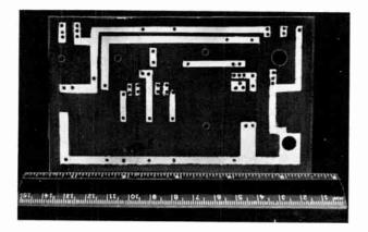
Fig. 502. Basic Amplifier circuit-board layout.
