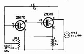
Resistor: R1-50,000-ohm potentiometer. Capacitor: C1-30  $\mu$ f, 6 volts, electrolytic. Transistors: V1-2N170, n-p-n; V2-2N301, p-n-p power. Battery: B1-6 volts, heavy duty (Burgess TW1). Lamp-6 volts (type No. 63). Miscelloneous: perforated circuit board; transistor sockets; brackets; knob; rubber feet; clearance lamp assembly (with lens and bracket); terminal strips; Fahnestock clips; machine screws and hex nuts; wire; solder; etc.
