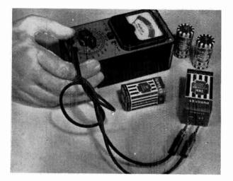
Fig. 603. Using a Battery Tester. Some internal load is placed across the battery when voltage measurements are being made.
