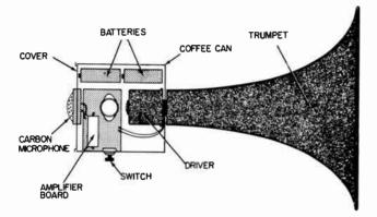
Fig. 211. Cross-section view of the Power Megaphone. Several loyouts are possible.
