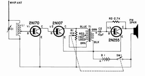
Resistors: R1-10,000-ohm potentiometer with spst switch; R2-2,700 ohms, ½ watt. Capacitors: C1-365 μμf (pf), variable (J. W. Miller 2111); C2-10 μf, 6-volt electrolytic. Coil: L1-ferrite antenna coil (J. W. Miller 2000). Transformer: T1-500-ohm CT pri, 8-ohm sec (Argonne AR-164). Switch: SW1-(on R1). Transistors: V1-2N170, n-p-n; V2-2N107,
