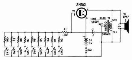
Resistors: R1-1,600 ohms; R2-to-R10 values determined experimentally (see text); (all ½ watt). Capacitors: C1-.1 µf tubular. Transformer: T1-500 ohms CT pri to 8 ohms (Argonne AR-164). Switches: SW1-spst toggle or slide; SW2 to SW10-spst spring return "key" type. Transistor: V1-2N301, p-n-p, power. Battery: B1-6 volts (Burgess F4P1 or 41.5 volt D-cells in series).
