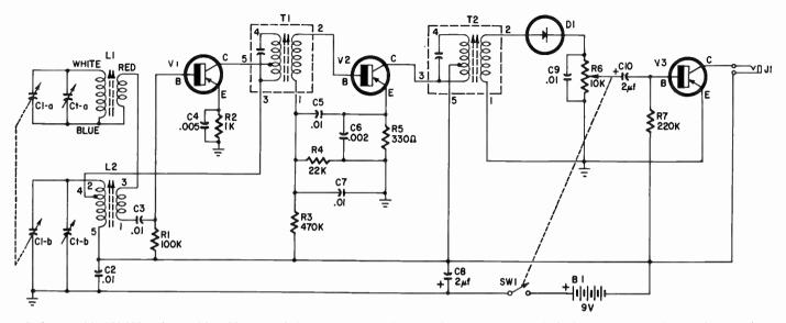
Resistors: R1-100,000 ohms; R2-1,000 ohms; R3-470,000 ohms; R4-22,000 ohms; R5-330 ohms; R7-220,000 ohms; (all  $\frac{1}{2}$  watt); R6-10,000-ohm potentiometer (audio taper) with spst switch. Capacitors: C1-2-gang variable (to match L1 and L2) (Argonne AR-93); C2, C3, C5, C7, C9-01  $\mu$ f; C4-.005  $\mu$ f; C6-.002  $\mu$ f; (all ceramic disc) C8, C10-2  $\mu$ f, 15 volts, electrolytic. Coils: L1—antenna coil to match C1-a (Argonne AR-69); L2—oscillator coil to match C1-b (Argonne AR-98).
