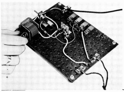
Fig. 303. Using the Light-Powered Receiver. Best results are obtained in full sunlight, but fair reception is obtained on overcast days. Use a moderate, to long, external antenna.
