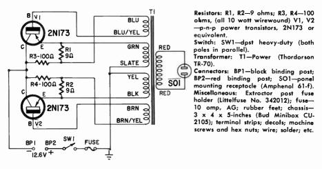
Fig. 519. Schematic of a useful auto accessory-a Power Inverter.
