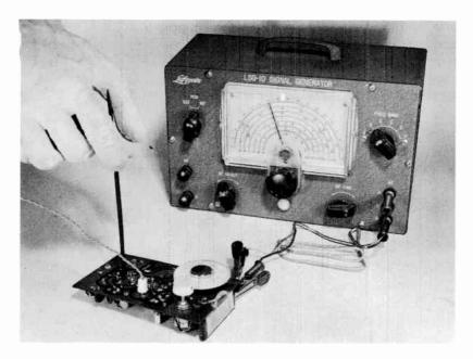
Fig. 318. Aligning the Pocket Superhet.
