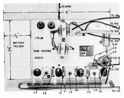
Fig. 513. Top of chassis view-Basic Superhet Receiver.
