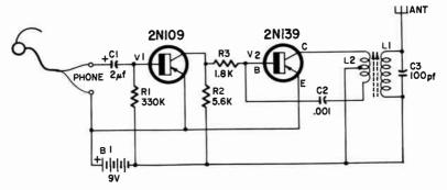
Resistors: R1-330,000 ohms; R2-5,600 ohms; R3-1,800 ohms; (all ½ watt). Copocitors: C1-2  $\mu$ f, 12 volts, electrolytic; C2-.001  $\mu$ f ceramic or paper; C3-100 pf ( $\mu\mu$ f) mica or ceramic. Coil: L1-L2-modified ferrite antenna coil (Superex VL) see text. Transistors: V1-2N109, p-n-p; V2-2N139, p-n-p, rf type. Bottery: B1—9 volts (Burgess type 2N6). Microphone: Phone—1,000 to 2,000 ohms, headphone.
