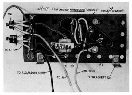
Fig. 311. The basic "chassis" used in the Cigar Box Portable-note that VI and V2 are soldered in position . . . sockets can be used if preferred, of course. Masonite, hardboard and pressed board are all name variations of the same material.
