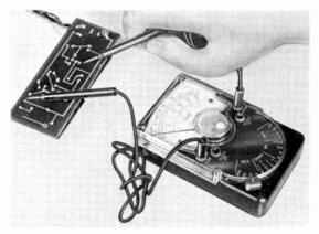
Fig. 605. Circuit-voltage tests help spot trouble.
