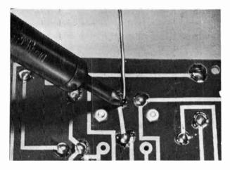
Fig. 708. Soldering connections on a circuit board.
