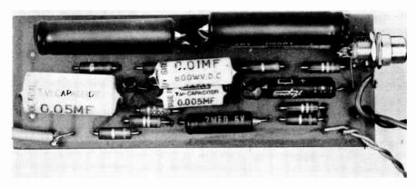
Fig. 206. Top view of wired hi-fi preamp. Although two capacitors are used in parallel for C5, a single unit of the right value is preferred.
