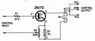
Resistors: R1—27,000 ohms, ½ watt; R2— 50,000-ohm potentiometer. Transistor: V1—2N170, n-p-n. Battery: B1—9 volts (Burgess type 2N6). Relay: RY—4,000-ohm coil, contact rating 1.5 amps, 28 vdc (Advance SO/1C/4,000D). Miscellaneous: perforated circuit board; rubber feet; transistor socket; brackets; knob; Fahnestock clips; battery connectors; machine screws and nuts; wire; solder; etc.
