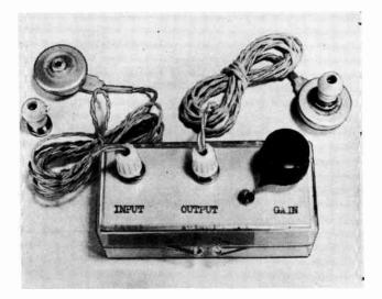
Fig. 225. The completed Detectaphone. The instrument is used with a standard high impedance dynamic earphones...one earphone serves as a microphone, the other as an output device.
