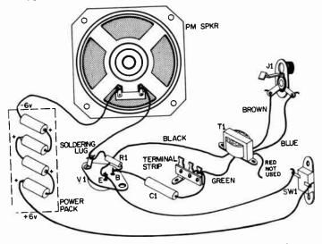
Fig. 220. Pictorial diagram for wiring the Audio Booster.
