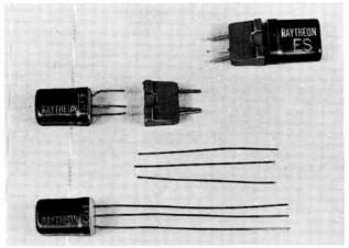
Fig. 104. Transistor leads must be cut short and, often, shaped to fit standard sockets.
