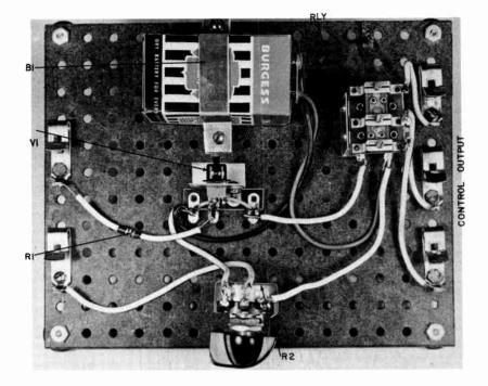
Fig. 302. The Light-Powered Receiver wired on a perforated board.
