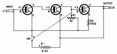
Resistors: R1-5,000 ohms (potentiometer with spst switch) R2-10D ohms, ½ watt. Switch: SW1-spst (on R1). Transistors: V1, V3-2N107, p-n-p; V2-2N170, n-p-n. Jacks: J1, J2-phone jacks, subminiature to match earobones. Battery: B1—6 to 9 volts. Miscellaneous: Small plastic box; small knob; perforated phenolic chassis; transistor sockets, hearing aid type earphones (2) with plugs to match J1 and J2; machine screws and hex nuts; wire; solder; spaghetti tubina: etc.
