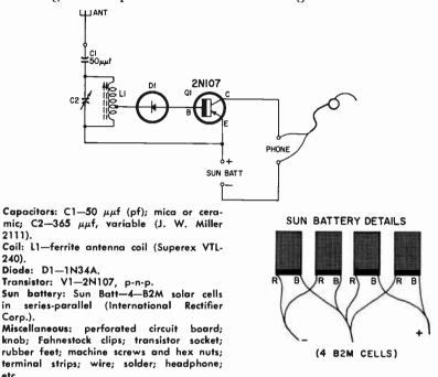
Fig. 301. Schematic of a simple Light-Powered Receiver.
