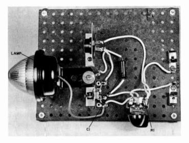
Fig. 415. Breadboard version of the Light Flasher.
