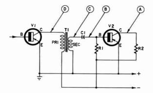
Fig. 611. Signal tracing techniques may be used to isolate component troubles. Tests at A and B check V2, tests at B and C check C1 and, finally, tests at C and D check T1.
