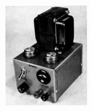
Fig. 520. Overall view of the completed Power Inverter.
