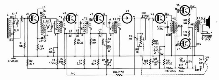
Resistors: R1, R8-10,000 ohms; R2-27,000 ohms; R3-1,500 ohms; R4, R10, R15-470 ohms; R5-68,000 ohms; R6-330 ohms; R7-3,300 ohms; R9-82,000 ohms; R11-2,700 ohms; R13-4,700 ohms; R14-56,000 ohms; R16-220 ohms; R17-33 ohms; R18, R19-10 ohms (all ½ watt); R12-5,000ohm potentiometer (audio taper), with spst switch (SW).
