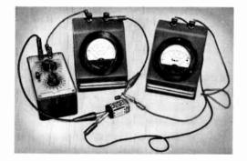
Fig. 101. Clip leads can be used to save time in an experimental setup. Test results can be erratic with this sort of arrangement.
