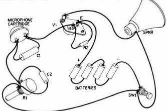
Fig. 210. Power Megaphone pictorial diagram.
