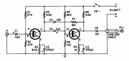
Resistors: R1, R2–27,000 ohms, R3, R8– 5,600 ohms, R4–8,200 ohms; R5–82,000 ohms; R6–10,000 ohms; R7–18,000 ohms; R8–5,600 ohms; R9–1,000 ohms; (all ½ watt). Capacitors: C1–10  $\mu$ f; C2, C3–250  $\mu$ f; C4– 2  $\mu$ f; (all 6-volt electrolytics) C5–015  $\mu$ f, paper or ceramic; C6–.05  $\mu$ f paper or ceramic.
