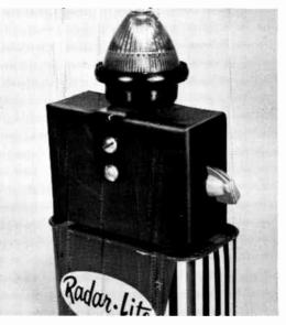
Fig. 417. The Light Flasher assembled in a small metal box and mounted on a heavy duty lantern battery.
