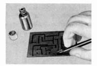
Fig. 706. Applying the resist to a cleaned board.
