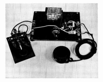
Fig. 420. With key and headphone connected, the Code Practice Oscillator is ready for use.
