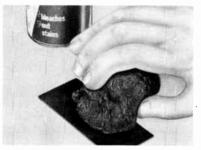
Fig. 705. Cleaning a copper-clad phenolic board.
