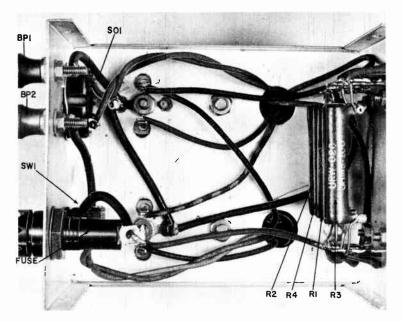
Fig. 521. Interior view of the Power Inverter. Resistors R1, R2, R3 and R4 are attached to terminal strips mounted on the rear apron.
