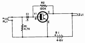
Fig. 201. Schematic of the Headphone Amplifier.
