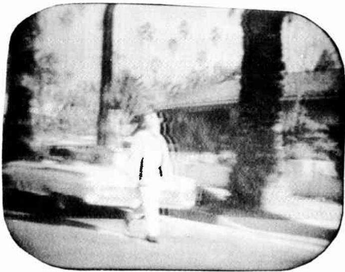
Fig. 507. The effects of overpeaking.
