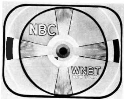
Fig. 208. Loss of fine detail in the vertical wedges is an indication of poor high-frequency response.
