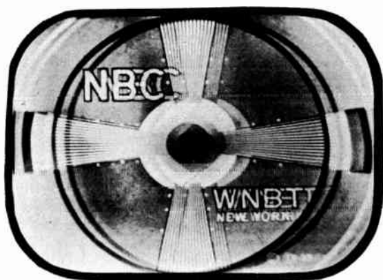
Fig. 108. Picture with widely displaced ghost.
