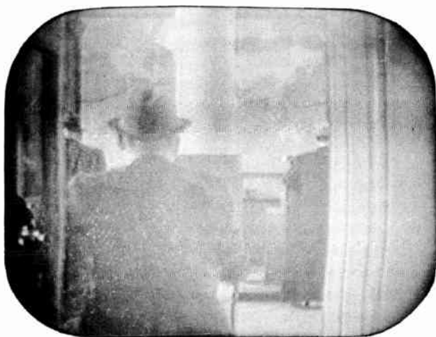
Fig. 505. Video if, detector or video amplifier trouble is indicated if a weak washed-out picture has no snow.
