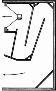
FIG. 8 (*above left*).—A SIMPLE HORN USED TO COUPLE A LOUD-SPEAKER TO THE AIR
