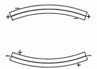
FIG. 9.—CRYSTAL "BIMORPHS" SUB-JECTED TO BENDING
