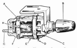
FIG. 10.—CUT-AWAY VIEW OF A CRYSTAL PICK-UP A crystal bimorph; B turnover knob; C plastic driving member; D stylus; E stylus arm; F plastic clamping block; G output terminal; H foil electrode connecting crystal and terminal.
