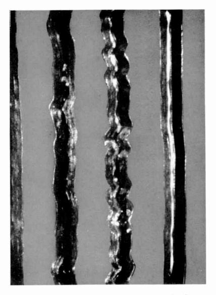
FIG. 17 (b).—The Microgrooves of Fig. 17 (a) After a Few Playings at Excessive Playing Weight and Without Attention to Dust Removal
