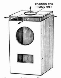
FIG. 11.—A SIMPLE TWO-SPEAKER SYSTEM The treble unit is mounted on an upward-facing baffle.
