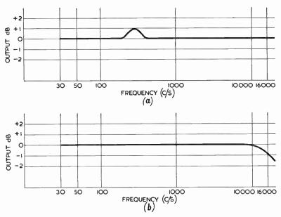
FIG. 2.—Two Illustrations of the Statement : Frequency Response 30–16,000  $c/s \pm 1dB$ .
