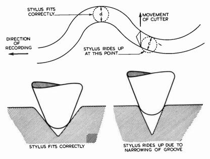
FIG. 11.—ILLUSTRATING THE "PINCH" EFFECT The stylus tip rises as the groove narrows—width c is smaller than d.
