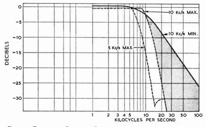
FIG. 3.—FREQUENCY RESPONSE CHARACTERISTICS OF LOW-PASS FILTER AND SLOPE CONTROLS
