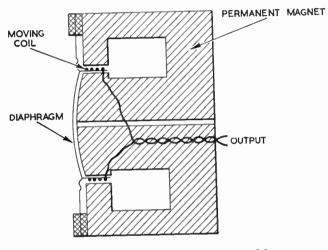
Fig. 6 (a).—Cross-sectional View of a Moving-coil Microphone
