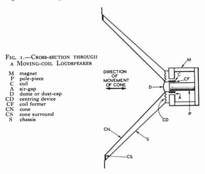
attraction and repulsion between these two fields moves the coil to and fro in the magnet gap, thereby driving the cone back and forth, as indicated by the arrow, to produce the sound waves.
