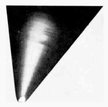
FIG. 18 (b).—EXCESSIVELY WORN STYLUS Note "flat" worn on the tip. (Courtesy E.M.I. Records Ltd.)
