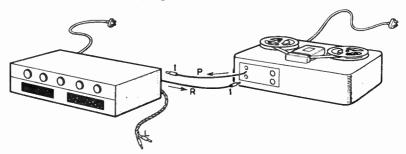
FIG. 2.—CONNECTIONS FOR AN AMPLIFIER AND TAPE RECORDER
