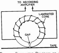
Fig. 3.—Schematic Diagram of a Tape Head
