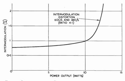
FIG. 4.—INTERMODULATION DISTORTION PLOTTED AGAINST OUTPUT Power
