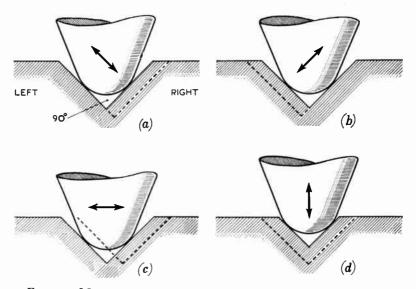
FIG. 2.—MOVEMENT OF STYLUS IN A COMPLEX-CUT GROOVE (a) Right-hand channel modulated, (b) left-hand channel modulated, (c) both channels modulated equally and in phase, (d) both channels modulated equally and in opposite phase.
