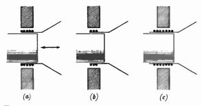
FIG. 2.—MEASURES TAKEN TO PREVENT THE COIL LEAVING THE MAGNETIC FIELD
