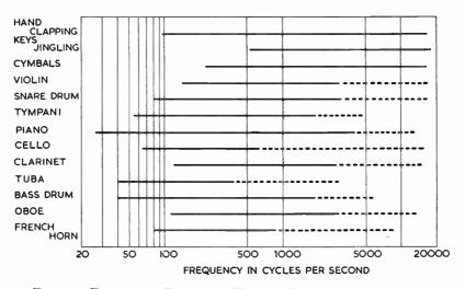
FIG. 1.—FREQUENCY RANGE OF VARIOUS MUSICAL INSTRUMENTS The solid lines show the range of fundamentals, the broken lines the harmonics.
