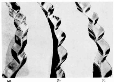
(a) Groove walls modulated equally and in phase, (b) right-hand groove walls modulated, (c) dissimilar modulation of groove walls. (Courtery N. V. Philips' Gloeilampenfabrieken, Holland.)
