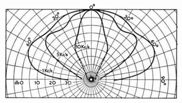
FIG. 4.—POLAR RESPONSE PATTERNS OF A TYPICAL LOUDSPEAKER AT VARIOUS FREQUENCIES
