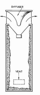
FIG. 7.—CROSS-SECTIONAL VIEW OF A COLUMN EN-CLOSURE The drive unit faces upwards into a diffuser.
