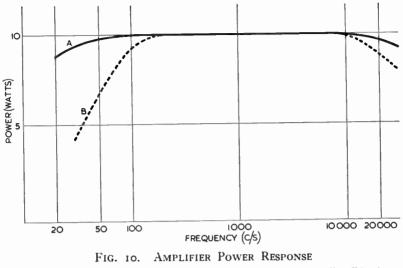
Curve A shows output reasonably maintained; in curve B it falls off in the bass and treble.
