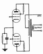
Fig. 5.—Simple Push-pull Output Stage with Triodeconnected Tetrode Valves
