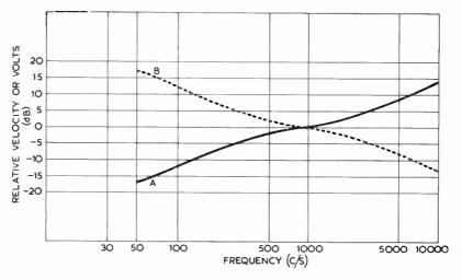
Fig. 2.—Microgroove Recording (A) and Playback (B) Characteristics
