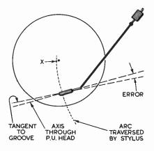
FIG. 13.—TRACKING ERROR The angle between a tangent to the groove and the axis through the pick-up head is a measure of tracking error.
