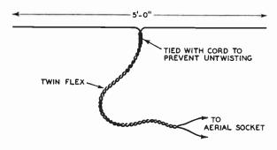
FIG. 14.—CONSTRUCTIONAL DETAILS OF A SIMPLE INDOOR DIPOLE AERIAL SUITABLE FOR USE IN AREAS WHERE SIGNAL STRENGTH IS GOOD
