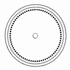
FIG. 16.—STROBOSCOPIC DISC
