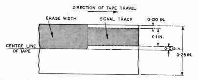
FIG. 2.—ARRANGEMENT AND DIMENSIONS FOR TWIN-TRACK RECORDING ON <sup>1</sup>/<sub>4</sub>-IN. TAPE
