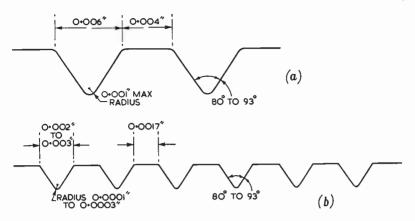
FIG. 1.—GROOVE CONTOURS (a) Coarse groove (78 r.p.m.), 90-120 grooves per inch. (b) Microgroove, 200-300 grooves per inch.
