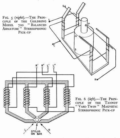
The principles of two types of stereo cartridge are shown in Figs. 5 and 6. The Goldring model 700 is very much like a pair of the variable reluctance pick-ups shown in Fig. 8, Chapter 2. As indicated in Fig. 5, the stylus S is mounted on a stylus bar extending between two pairs of poles and pivoted at P; hence the
