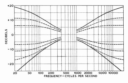
Fig. 2 (a).—Frequency Response Curves for a Passive Tone Control Circuit
