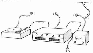
FIG. 1.—PRINCIPAL CONNECTIONS FOR AN INSTALLATION COMPRISING A TURNTABLE WITH PICK-UP, AN AMPLIFIER, AND AN F.M. RADIO TUNER
