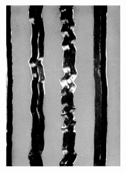
FIG. 17 (a).—PHOTOGRAPH OF UNPLAYED MICROGROOVES Compare with the photograph, Fig. 17 (b), of the same grooves after being played under bad conditions. (Courtesy E.M.I. Records Ltd.)
