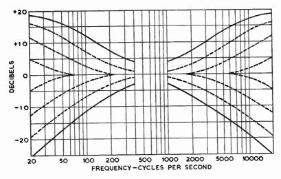
FIG. 2 (b).—FREQUENCY RESPONSE CURVES FOR A NEGATIVE FEEDBACK TONE CONTROL CIRCUIT (BAXANDALL CIRCUIT)
