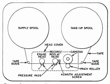
FIG. 4.—LAYOUT OF A TYPICAL TAPE DECK, SHOWING THE MAIN COMPONENTS
