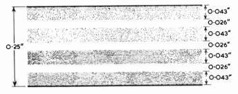
FIG. 8.—Arrangement of Four Tracks on a  $\frac{1}{4}$ -in. Tape
