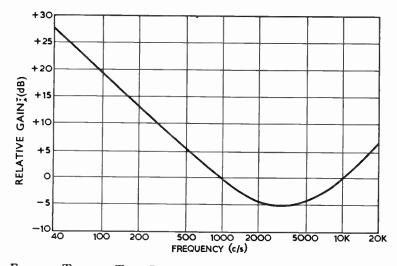
FIG. 5.—Typical Tape Playback Amplifier Response Curve for Playback at  $7\frac{1}{2}$  I.P.S. Speed
