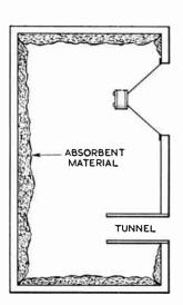
FIG. 6.—CROSS-SECTIONAL VIEW OF A VENTED ENCLOSURE WITH AN INTERNAL TUNNEL
