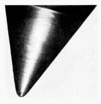
FIG. 18 (a).—New MICROGROOVE SAPPHIRE STYLUS (Courtesy E.M.I. Records Ltd.)
