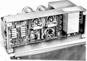
FIG. 1 (b).—UNDER CHASSIS VIEW OF QUAD H AMPLIFIER WITH BASE COVER REMOVED Note neat positioning of components and arrangement of wiring.
