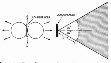
FIG. 15 (a).—SOUND RADIATION OF A DOUBLET There is no radiation in the plane of the loudspeaker (*i.e.* direction "x.").
