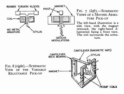
A big advantage is the ease of stylus replacement. The cantilever is cleated to the rod magnet, and this assembly is simply pulled from the pick-up and a new one pushed in. The Ferroxdure magnet is quite cheap and is therefore expendable. The magnets of replacement assemblies will not become demagnetised under normal storage conditions.
