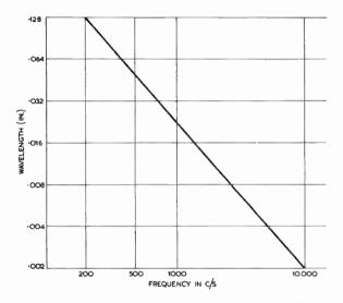
Fig. 12.—Relationship between Recorded Wavelength and Frequency for a 12-In.,  $33\frac{1}{3}$  R.P.M. Record
