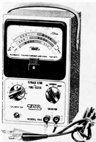
Fig. 1205. A shorted turn in a horizontal output transformer lowers the Q of the inductance, which is indicated by the frequency-generating circuits in testers of this type. It is often necessary to unsolder terminal connections and remove the high-voltage rectifier tube from its socket as even the shorted loop of the filament winding can give a REPLACE indication. (Electronic Instrument Co.)
