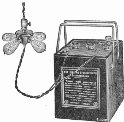
Charging Battery with Charging Plug.
