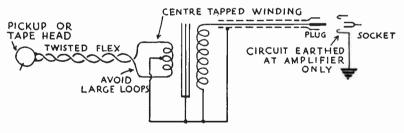
Fig. H/4. Input circuit with centre-tapped transformer arranged to avoid hum.
