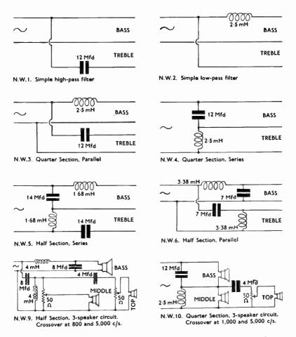
Fig. C/20. Typical Constant Resistance Crossover Circuits with values for 15 ohms speakers and 1,000 c/s crossover, except NW9 which is for 800 and 5,000 c/s and includes two volume controls.
