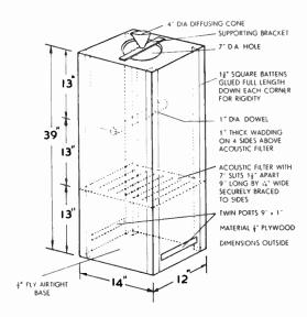
Fig. C/6. Plywood column (with solid wood corners) for 8" unit. Weight 30 lb. approx. Internal volume 3 cu.ft. approx. The dowel must be tightly wedged between the two panels to control resonance.
