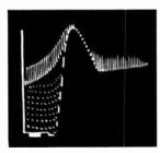
Fig. I/3. Picture of combined effect of motor-boating and parasitic oscillation on steady tone at 1,500 c/s, showing severe intermodulation.
