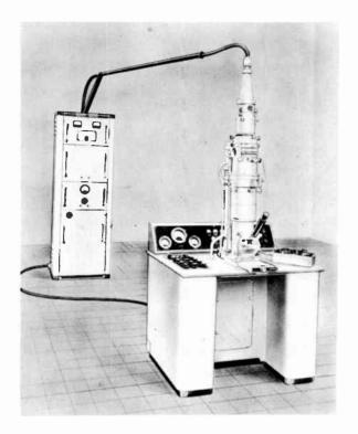
Fig. E/6c. A.E.I. Electron Microscope.
