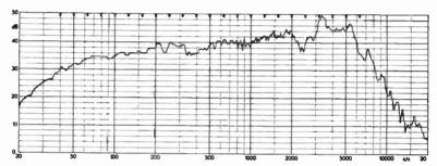
Fig. L/8. Axial response of modern 10" speaker. Bass resonance 35 c/s.
