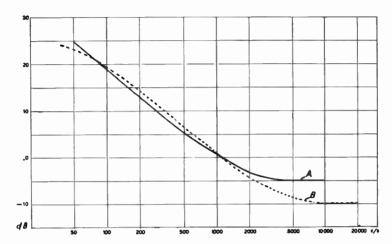
Fig. T/3. Standard replay characteristics for 7½"/sec tapes
