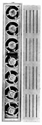
If all the units in a line source loudspeaker are fed with equal power, the radiation pattern will contain large spurious side lobes. Cleaner results can be obtained if the power input to each unit is attenuated progressively as its distance from the centre increases.
