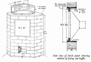
Fig. B/3. Brick corner enclosure, 9 cu.ft., used with no interior lining or absorbents.
