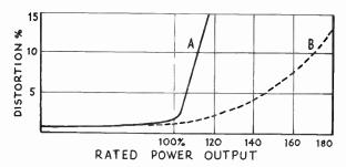
Fig. O/4. Amplifiers with different overload characteristics.
