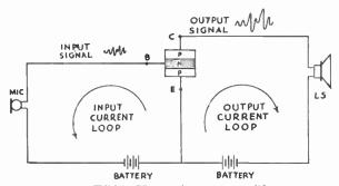
Fig. T/12. The transistor as an amplifier.
