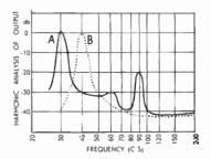
On a listening test, harmonic peaks which are 20 dB less than the fundamental are difficult to detect. A speaker system which is free from frequency doubling above about  $40~\mathrm{c/s}$  sounds smooth and warm in the bass and often quieter than a less linear set up.
