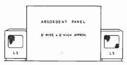
Fig. A/3. Absorbent surface placed between loudspeakers to improve stereo.
