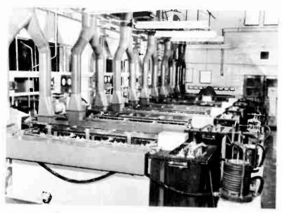
Fig. R/12. High peed nickel plating vats producing solid nickel stampers.
