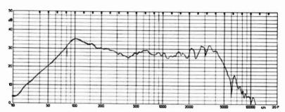
Fig. L/7. Axial response of 1930 model. Bass resonance 90 c/s.
