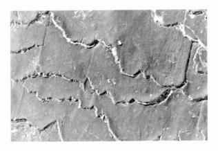
Fig. E/6B. Electron-microscopic view of human hair. Mag. 3,000x.
