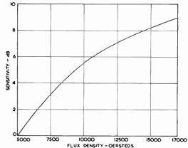
Fig. F/4. Speaker output related to flux density with white noise input.
