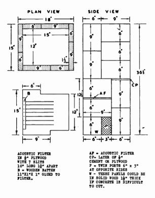
Fig. C/8. Concrete column, 4 cu.ft., using slabs 9" × 6" × 1½" and suitable for 8" and 10" units.
