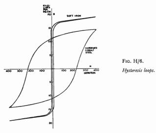
In materials such as transformer cores which are subjected to continual magnetic reversals, hysteresis accounts for a substantial portion of the wasted power.
