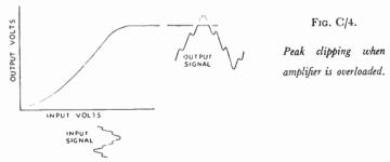
Moderate peak clipping does not cause serious audible distortion in a properly designed amplifier but there will be some roughness and hardening of tone quality. Distortion will be noticed however with poor quality amplifiers which produce parasitic oscillations when overloaded.
