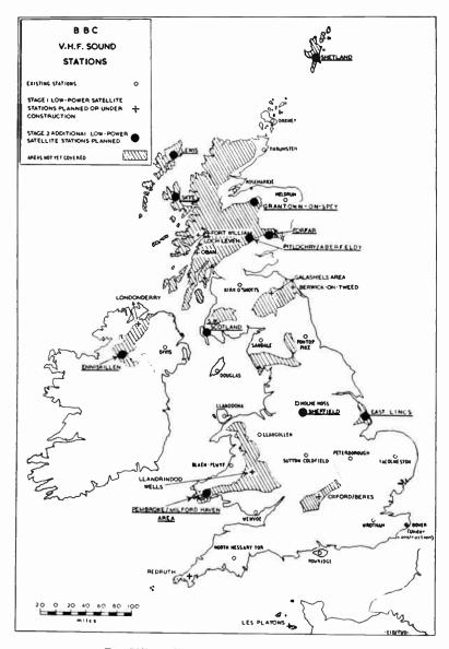
Fig. V/1. VHF coverage by B.B.C. transmitters.
