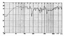
Fig. B/2. Response of 8" unit in 9 cu.st. corner brick enclosure.
