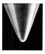
Fig. S/12. Typical ½ mil sapphire for stereo. Mag. 250x.
