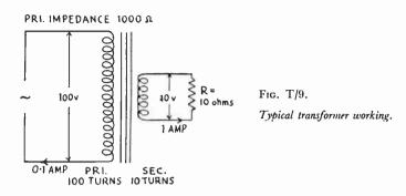
If the secondary is loaded with a resistance of 10 ohms and the current in the primary is 0.1 amp, the current in the secondary, neglecting the losses in the transformer, will be 1 amp. The primary circuit has an effective resistance of  $\frac{100}{0.1} = 1,000$  ohms, against 10 ohms in the secondary. The transformer has modified the impedance by 100 times, i.e. the square of the turns ratio.
