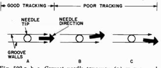
Fig. 502-a,-b,-c. Correct needle tangency (a) means good tracking. Poor tracking results from the conditions shown in b and c.
