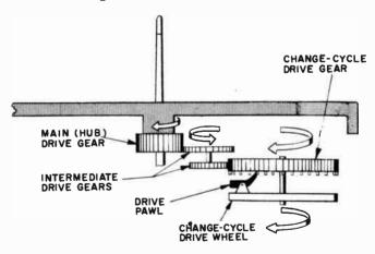
Fig. 603. Typical operation of pawl-latch drive.
