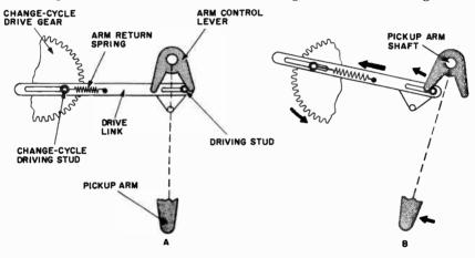
Fig. 1101-a,-b. Basic direct swing-in drive.
