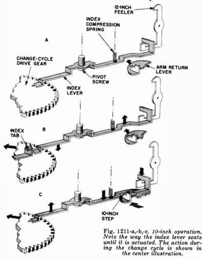
mined by the index lever contacting the first, second or third index step on the arm-return lever. The index lever, then, must be raised to a different position for each record size. With this device, 7-inch records cannot be intermixed in the stack for the same reasons given for the previous setdown index.
