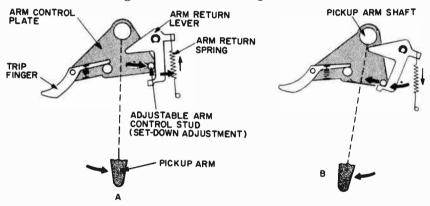
Fig. 1106-a,-b. Basic spring-loaded direct swing-in drive.
