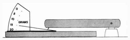
Fig. 511. Technique used for measuring needle pressure.
