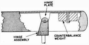
Fig. 513. Counterbalance is positioned as shown above.
