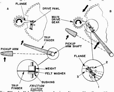
Fig. 705-a,-b. Velocity trip mechanism. It resembles the position type but differs in the use of a friction clutch.
