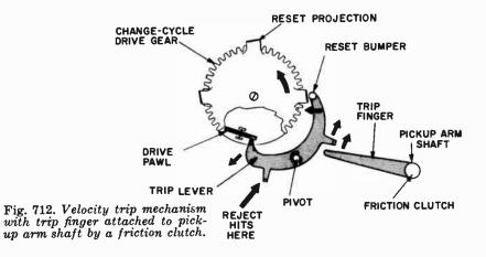
enters the runoff grooves, the trip finger moves the trip lever too fast for it to be reset. The trip lever then releases the drive pawl so that the pawl turns to latch the bosses (metal extensions) at the underside of the change-cycle drive gear; this starts the change cycle. During the cycle, the trip lever is reset by the reset projections on the change-cycle drive gear; it is put directly in the path of the drive pawl so that it will uncouple the pawl at the end of the cycle.
