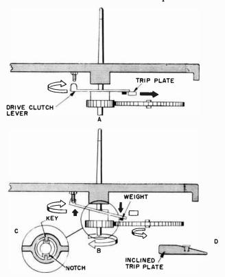
Fig. 608-a,-b,-c. Dog-latch keyed-lever clutch.
