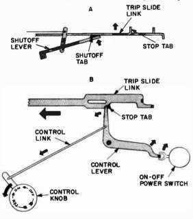
Fig. 1302-a,-b. Automatic control lever power shutoff.
