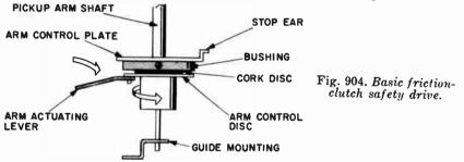
smooth. The arm swings to the position where the stop ear on the arm control plate hits the obstruction; then it stops, although the groove track and arm actuating lever keep driving it. This is possible because of the safety drive.
