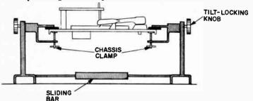
Fig. 102. Service stand facilitates repair of record changers.
