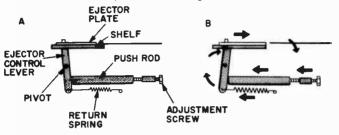
Fig. 1008-a,-b. These illustrations show the operation of a shelf plate ejector.
