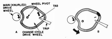
Fig. 606-a,-b. Turntable hub rim-drive clutch.
