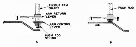
Fig. 1103-a,-b. The spring-loaded drive clutch.
