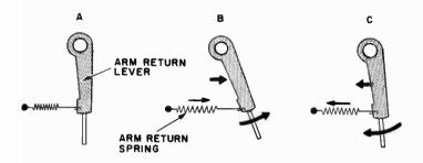
Fig. 1102-a,-b,-c. The spring-loaded arm return lever.
