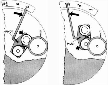
Fig. 311. Three-speed belt-drive assembly showing 33-1/3 and 45 r.p.m. positions.
