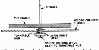
Fig. 402. The main drive gear is mounted on the turntable hub.
