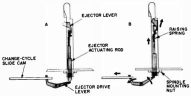
Fig. 1016-a,-b. Slide-cam-lever drive.
