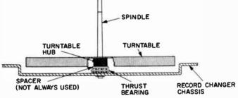
Fig. 404. The thrust bearing permits the turntable to turn smoothly.
