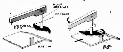
Fig. 901-a,-b. Slide-cam swing-out drive. Illustration at left shows parts at start of change cycle. Action during change cycle appears in drawing at the right.
