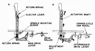
Fig. 1015-a,-b. Lateral-cam-lever drive.
