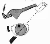
Fig. 910. Automatic (spring-loaded) safety drive. With this type of mechanism the motion of the pickup arm can be impeded, but the change cycle will continue.
