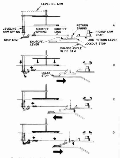
Fig. 1301-a,-b,-c,-d. Leveling arm automatic shutoff mechanism.
