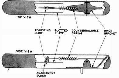
Fig. 518. Another adjustable spring counterbalancing method.
