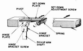
Fig. 1219. Admiral set-down adjustment.
