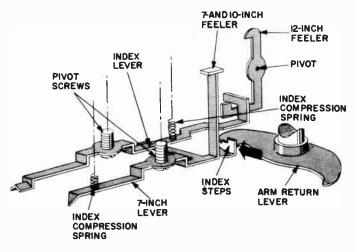
Fig. 1210. Basic V-M automatic random intermix index.
