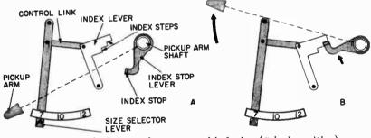
Fig. 1201-a,-b. Selector lever manual indexing (7-inch position).
