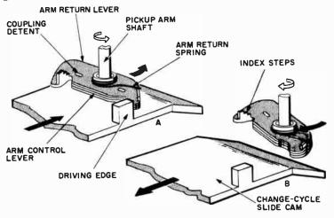
Fig. 1105-a,-b. Basic V-M 950 spring-loaded swing-in drive.
