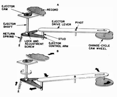
Fig. 1007-a,-b. Mechanism of a shelf cam ejector.
