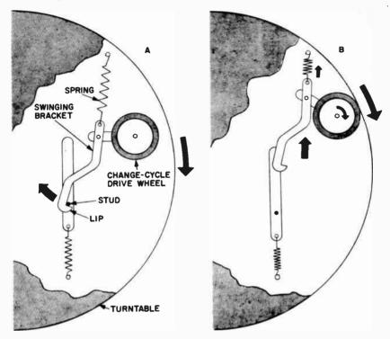
Fig. 605-a,-b. Illustrations show operation of rim-drive clutch.
