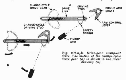
is held back, the driving stud will also be held back, as shown in Fig. 906-b. The safety arm will then pivot and the safety spring will stretch, permitting the rest of the change-cycle mechanism to go through the change cycle unhindered. But, if the pickup arm is then freed, the safety spring will pull in the safety arm, driving the pickup arm to its normal position.
