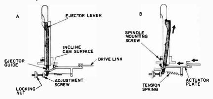
Fig. 1018-a,-b. Sliding-incline-cam drive.
