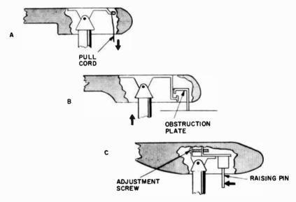
Fig. 802-a,-b,-c. Behind-the-hinge pickup arm raising methods.
