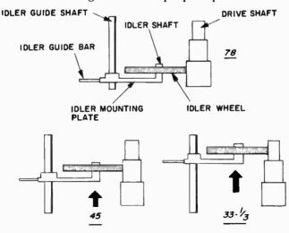
Fig. 313. Three-diameter drive shaft speed positions. The speed reduces as the drive-shaft diameter decreases.
