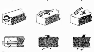
Fig. 521-a,-b,-c. Three methods of changing from 78 to 45 and 33<sup>1</sup>/<sub>3</sub> needles.
