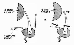
Fig. 1218-a,-b. Holding out the index arm.
