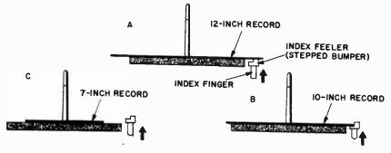
Fig. 1204-a,-b,-c. The basic automatic non-intermix index.
