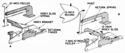
Fig. 1209-a,-b. 12-inch operation. This technique takes advantage of the striking action of the falling record.
