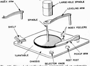
Fig. 101. View of above-the-chassis components of un automatic record changer.
