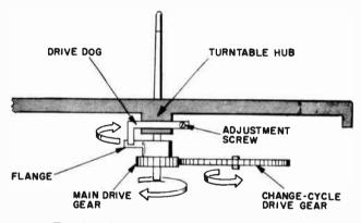
Fig. 601. Illustration shows dog-latch drive.
