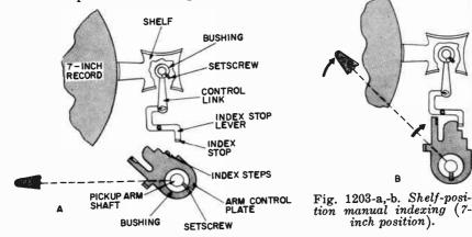
ing the index stop lever so that the stop will be put in the path of the proper index step. Unlike the previous setup, this index stop lever is stationary during the cycle and the index steps swing in with the pickup arm. The overall action, however, is the same.
