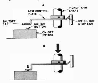
Fig. 1304-a,-b. Automatic control plate power shutoff.
