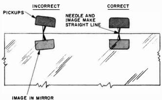
Fig. 525. Technique for checking needle alignment.
