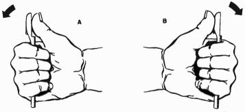
Fig. 1023-a,-b. Technique for adjusting the record guide.
