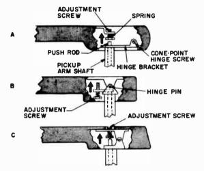
Fig. 801-a,-b,-c. Basic push rod arm-raising devices.
