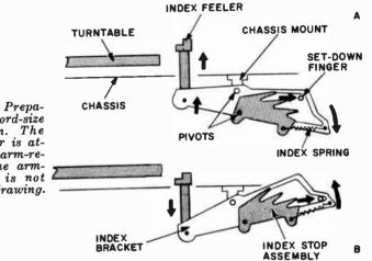
Fig. 1205-a,-b. Preparation for record-size determination. The set-down finger is attached to the arm-return lever. The arm-return lever is not shown in this drawing.
