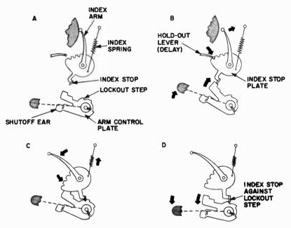
Fig. 1303-a,-b,-c,-d. Index arm automatic shutoff mechanism.
