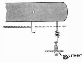
Fig. 517. Adjustable spring counterbalancing method.
