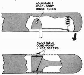
Fig. 516. This arm uses adjustable hinge screws.
