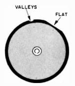
Fig. 322. Flats and valleys sometimes develop in the rubber edge or rim of the idler wheel. This can happen even if the record changer is not in use. Examine the wheel carefully to make sure that it is not out of round.
