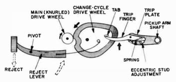
Fig. 708. Simple type of position trip mechanism used in automatic record changers.
