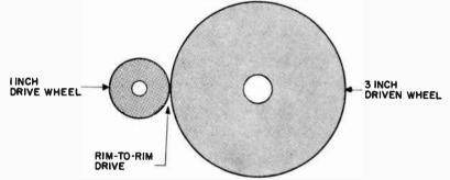
Fig. 303. Rim coupling makes use of rim-to-rim drive.
