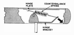
Fig. 515. Spring counterbalancing technique.
