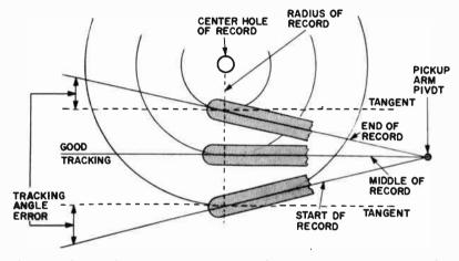
Fig. 503. Illustration above shows how tracking angle error is measured.
