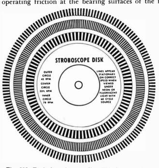
Fig. 202. Typical stroboscope disc. This is a simple and effective means for checking the speed of the motor.
