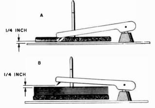
Fig. 808. Adjusting the pickup arm height.
