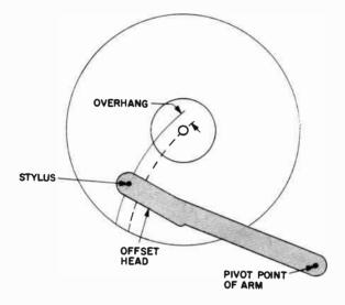
Fig. 504. Pickup arm with an offset head.
