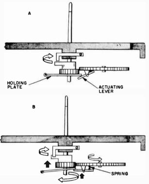
Fig. 607-a,-b. Dog-latch holding plate clutch.
