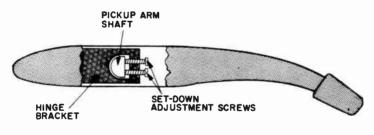
Fig. 1220. Collaro set-down adjustment.
