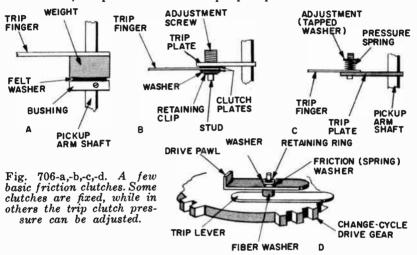
at the trip friction clutch for the trip mechanism to function properly. If the clutch is too tight, the record changer will trip too soon. If it is much too tight, it might kick the pickup arm back a groove or two whenever it is reset. If the clutch is too loose, the changer may not trip at all.
