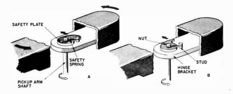
Fig. 902-a,-b. Basic hinge-bracket safety drive. The safety plate turns with the pickup arm shaft.
