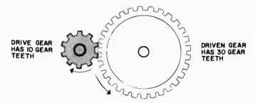
Fig. 301. Simple mechanical coupling using gears.
