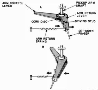
Fig. 1104-a,-b. Basic Admiral RC600 spring-loaded swing-in drive.
