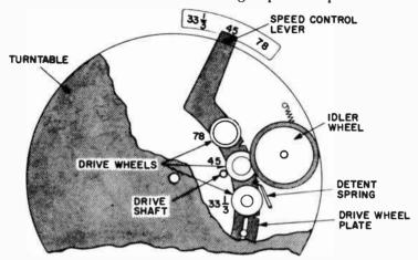
Fig. 306. Three-speed step-rim drive. Each drive wheel has a different upper diameter. The detent spring locks the drive wheel plate into position for any particular speed.
