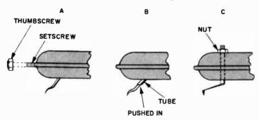
Fig. 526-a,-b,-c. Three methods of replacing a needle.
