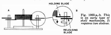
record could break in half. With this device, the spindle functions only as a guide and so it is not offset. It is a straight round rod, although it may sometimes appear with a taper.
