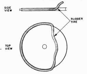
Fig. 318. The rubber tire seated in the groove of the idler wheel can be removed quite easily.
