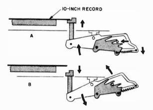
Fig. 1207-a,-b. 10-inch operation.
