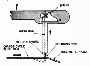
Fig. 803. Slide-cam push-rod technique.
