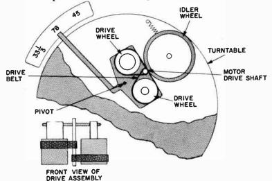
Fig. 310. Three-speed belt drive assembly. The unit is shown in the 78 r.p.m. position.
