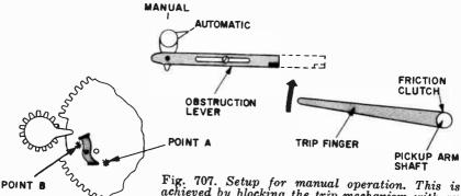
Fig. 707. Setup for manual operation. This is achieved by blocking the trip mechanism with an obstructing lever.
