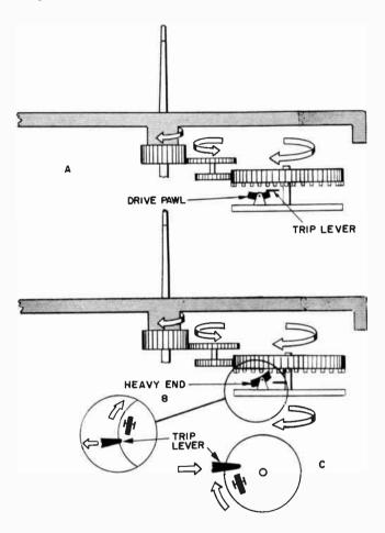
Fig. 609-a,-b,-c. Basic pawl-latch clutch method.
