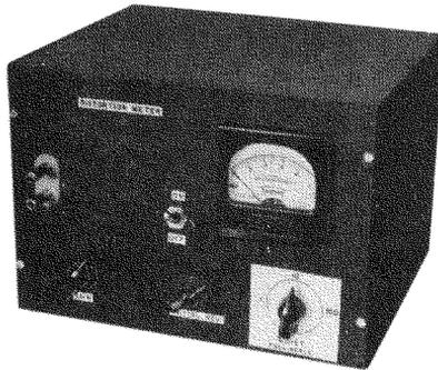
*Fig. 1804. A front view of the distortion meter.*
