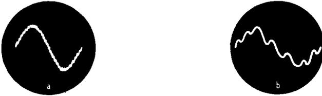
Fig. 1103. *Waveform a is distorted sine wave output. Waveform b is a 60-cycle sine wave modulated with 400 cycles.*
