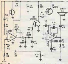
Fig. 1. The one-way intercom uses an omnidirectional electret microphone to pick up sound and convert it to an electrical signal. The resulting signal is used to activate the audio umplifier (U2) that drives the speaker (SPKRI), and is also the audio signal that is output by the speaker.
