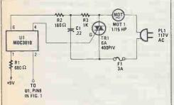
Fig. 2. The Triac Driver can be added to the proximity switch to control a small AC motor.
