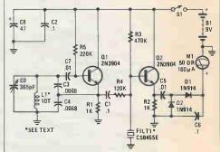
Fig. 3. The metal detector is little more than a simple oscillator circuit (built around QI), whose output is fed to a meter (MI), causing it to deflect to about mid-scale. When the sense coil (LI) is brought near metal, the oscillator frequency changes, and that change causes the meter needle to move either up or down the scale depending on the type of metal detected.
