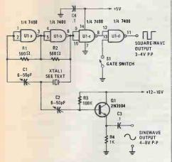
Fig. 1. Two gates (U1-a and U1-b) of a 7400 quad 2-input NAND comprise the actual oscillator circuit, with feedback controlled by a crystal (XTALI) and a variable capacitor (C1). Gate U1-c is used to buffer the output of the oscillator, while U1-d is used to turn the output on and off.
