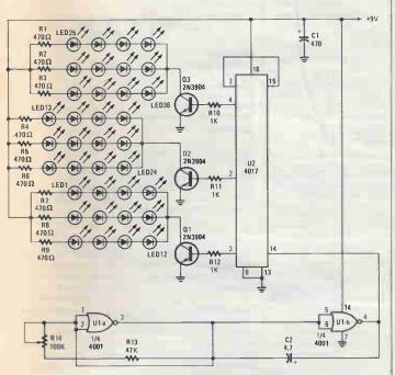
Fig. 1. The bell-unimation circuit contains 36 LED's that are controlled by a 4017 counter/divider, which is clocked by an astable multivibrator that consists of half of a 4001 quad 2-input NOR gate.
