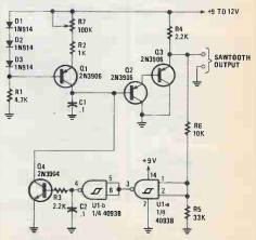
Fig. 4. The Sawtooth Generator's output frequency is controlled by R7, which provides a low end frequency of about 30 Hz and an upper end frequency of close to 3.3 kHz.
