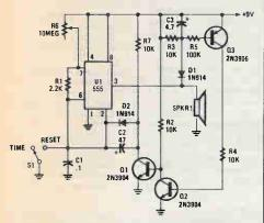
Fig. 1. This time-out circuit differs from conventional 555-timer applications in that this circuit has the 555 configured in the astable mode as opposed to the monostable, or one-shot mode.
