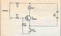
Fig. 3. The moisture detector is nothing more than a transistor (in a common-emitter configuration) that is used as a simple switch.
