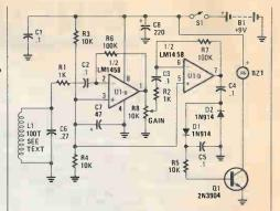
Fig. 4. The receiver portion of the metal detector is built around an LM1458 dual op-amp. a single 2N3904 general-purpose silicon transistor, and a 100-turn homebrew coil that's tuned to about 7 kHz via C6.
