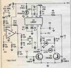
Fig. 2. The analog audio-frequency meter is actually made up of three simple sub-circuits; a conventional inverting amplifier, a phase-locked loop, and a nixer/LED driver.
