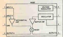
Fig. 1. Here's a block pinout diagram of Signetics' NE602 lowpower VHF double-balanced mixer, which contains a built-in local oscillator, an differential input amplifier, and a voltage regulator.
