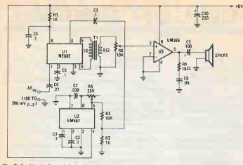
Fig. 2. In this single-mode inversion voice scramber/descrambler circuit, the NE602 is configured as a balanced modulator/demodulator.
