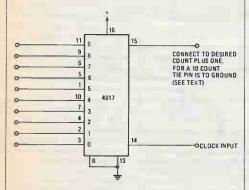
Fig. 3. Additional LED-bell outlines can be added to the circuit using this diagram as a guide. Simply connect pin 15 of the counter to the output that corresponds to the number of bells plus one. See the text for more information.
