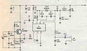
Fig. 4. Here is an unusual audio-frequency generator built around the NE602. It produces an audio sine-wave by mixing the outputs of two RF oscillators operating at about the same frequency.
