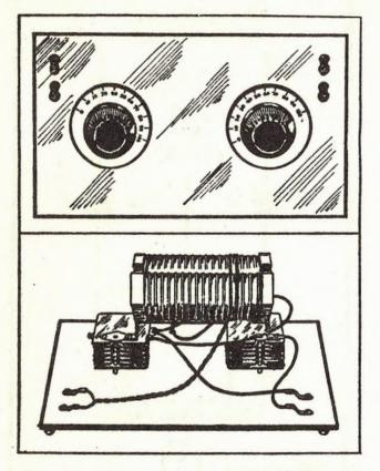
Fig. 14. General appearance of the inverted "L" antenna tuner.
