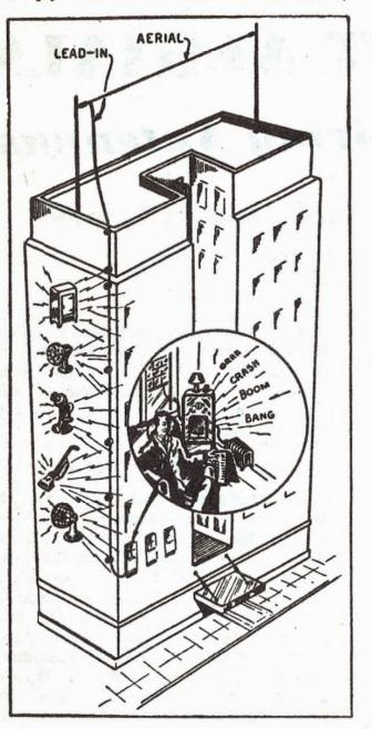
Fig. 1. Some of the sources of man-made static. Note the position of the lead-in wire in the field of noise.
