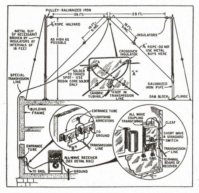
Fig. 17. Complete installation of a double doublet antenna system for "all wave" radio reception.
