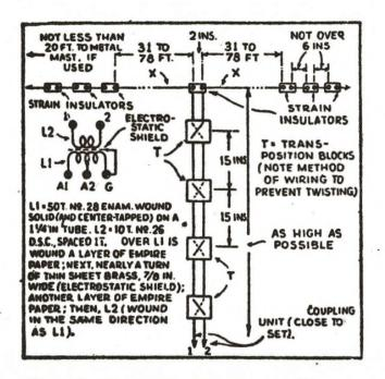
Fig. 16. Typical Doublet Antenna System.
