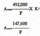
and C=75XD.  $K^{T}$ =.25 for frequencies below 3,000 kc., .24 from 3,000 to 28,000 kc., and .23 for all frequencies above 28,000 kc., and D is the diameter of the wire. In other words, the spacing between the two feeders should be equal to 75 times the diameter of the wire. This antenna
