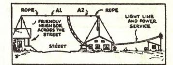
Fig. 19. Improved antenna, remote from power line. Note balance weight to keep aerial taut.
