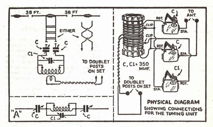
Fig. 10. A tuned doublet antenna. The antenna is "tuned" by varying condensers C, C1, and by shorting out turns on the coupling coil.
