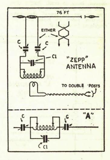
Fig. 11. Tuned "Zeppelin" Antenna. The tuning system is the same as that shown in figure 10.
