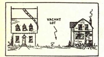
Fig. 24. Aerial construction where it has to be confined to the roof of your house. Erect aerial as high as possible and keep the feeders as far as possible from the side of the house.
