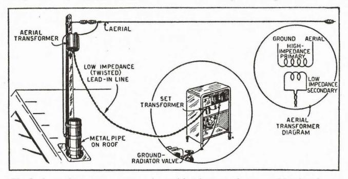
Fig. 6. A complete antenna system using aerial and set transformers and low-impedance transmission line.
