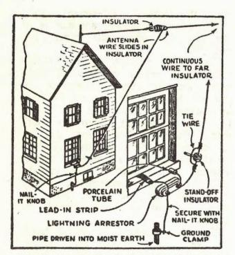
Fig. 5. Proper installation of an inverted "L" antenna.
