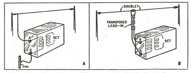
Fig. 4. Left, Marconi Inverted "L" Antenna. Right, Hertzian Doublet Antenna.
