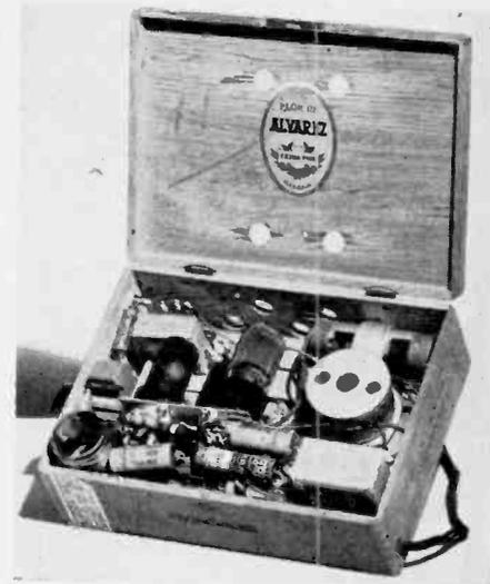
Layout of the three-tube broadcast receiver.
