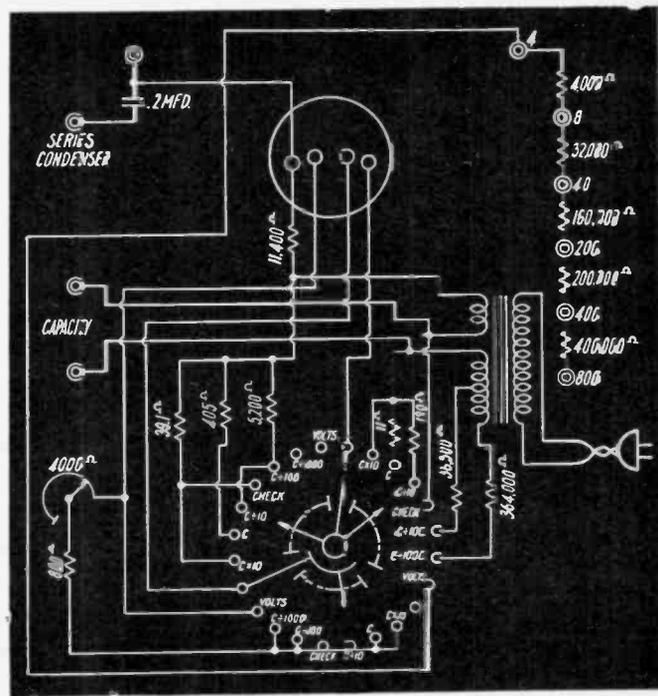
Fig. 7—The Weston 664, a wide-range commercial capacitance meter.
