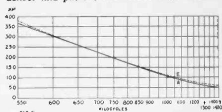
Fig. 5—Padder & Trimmer make a good curve
