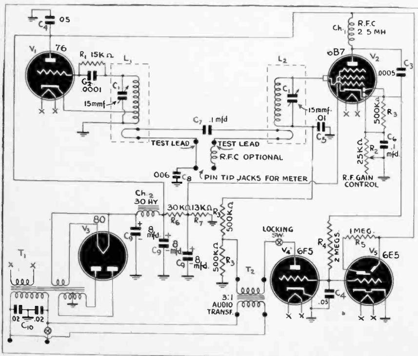
cycles. The link circuit is broken on one side and brought out to pin tip jacks. The tuned circuit is connected to a 6B7 pentode section. The output of the pentode section is rectified in the diode section and the negative potential developed is applied to
