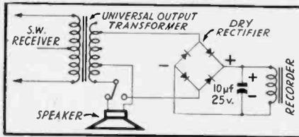
Fig. 2—Hookup for recording from receiver
