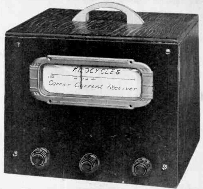
**V**ERY good "wired wireless" results are obtainable with the simple equipment described here. I have been experimenting with these circuits for some time, using approximately 200 Kc. as carrier. Communication has been carried on a distance of 6 blocks in a crowded residential district of Berkeley, and undoubtedly greater distances are easily possible. Either phone or C.W. signals may be transmitted.
