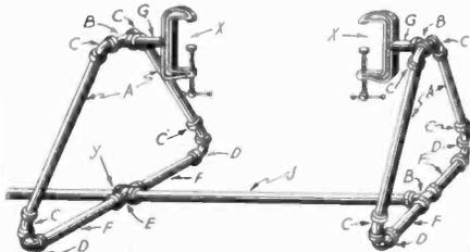
The chassis cradle above was built entirely of ready-cut easily-obtained pipe fittings
