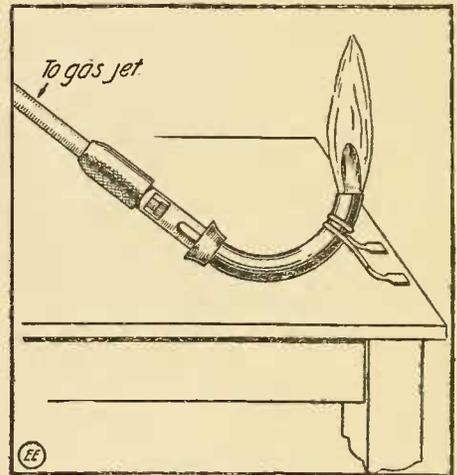
To Make This Gas Blow Torch You Will Require a Bicycle or Other Small Pump, a 1 to 5 Gallon Can, and Two Lengths of Rubber Tubing to Lead the Gas and Comprest Air to the Torch Handle.
