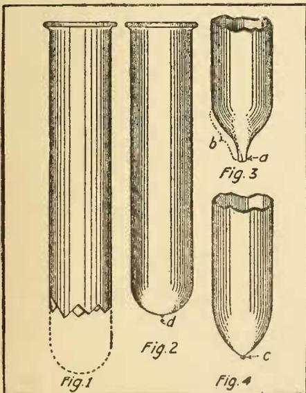
The broken test-tube was lowered into the Bunsen flame and the jagged edges, when soft enough, (still held in the flame) were pulled out with the aid of an ordinary pair of pliers. When the walls seemed thin enough, the jagged edges were drawn together thereby closing the end of the tube as in Fig. 3. The heat was concentrated on "b," Fig. 3, and when soft enough the tip "a" was drawn out (*while held in the flame*).
