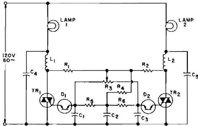
$R_1 = R_2 = 6800\Omega, 1\text{WATT}$
