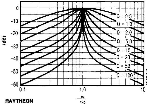
$$V_{BP} = \frac{\frac{\omega}{\omega_0} \frac{1}{Q}}{\sqrt{\left[1 - \left(\frac{\omega}{\omega_0}\right)^2\right]^2 + \left(\frac{1}{Q} \frac{\omega}{\omega_0}\right)^2}}$$
