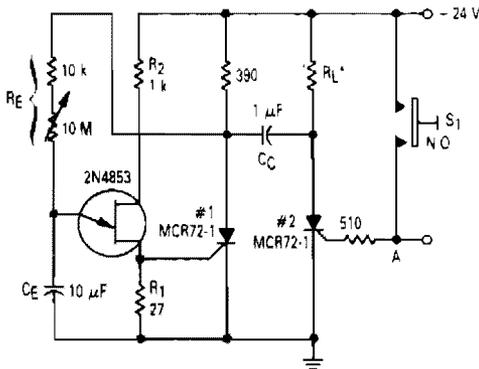
\*VALUE OF  $R_L$  MUST BE LOW ENOUGH TO ALLOW HOLD CURRENT TO FLOW IN THE SCR
