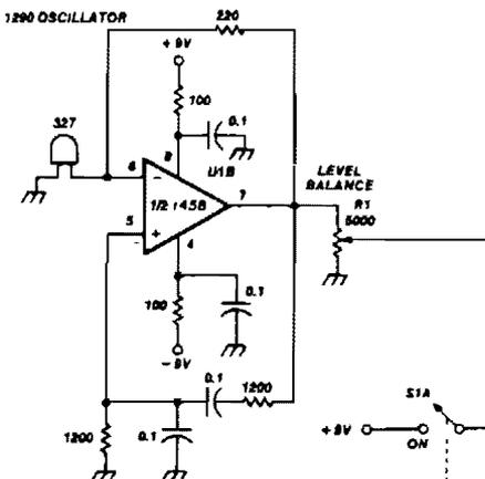
Except as indicated, decimal values of capacitance are in microfarads ( $\mu F$ ); others are in picofarads (pF); resistances are in ohms.  $k = 1,000$   $M = 1,000,000$
