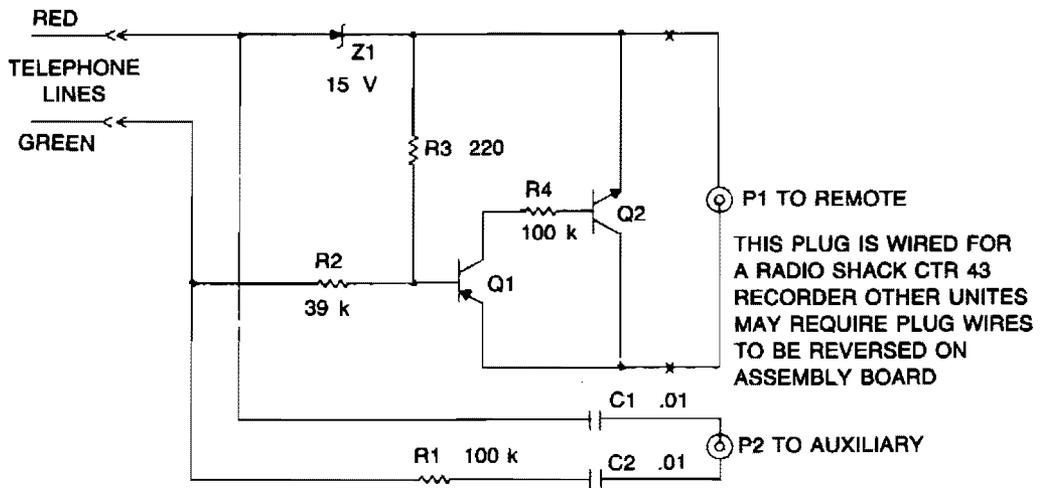
CONNECT TO ANY CONVENIENT PHONE JACK OR WHEREVER ACCESS TO WIRES IS AVAILABLE. MAY BE CONNECTED VIA ALLIGATOR CLIPS, PLUGS OR MODULAR PLUG.
