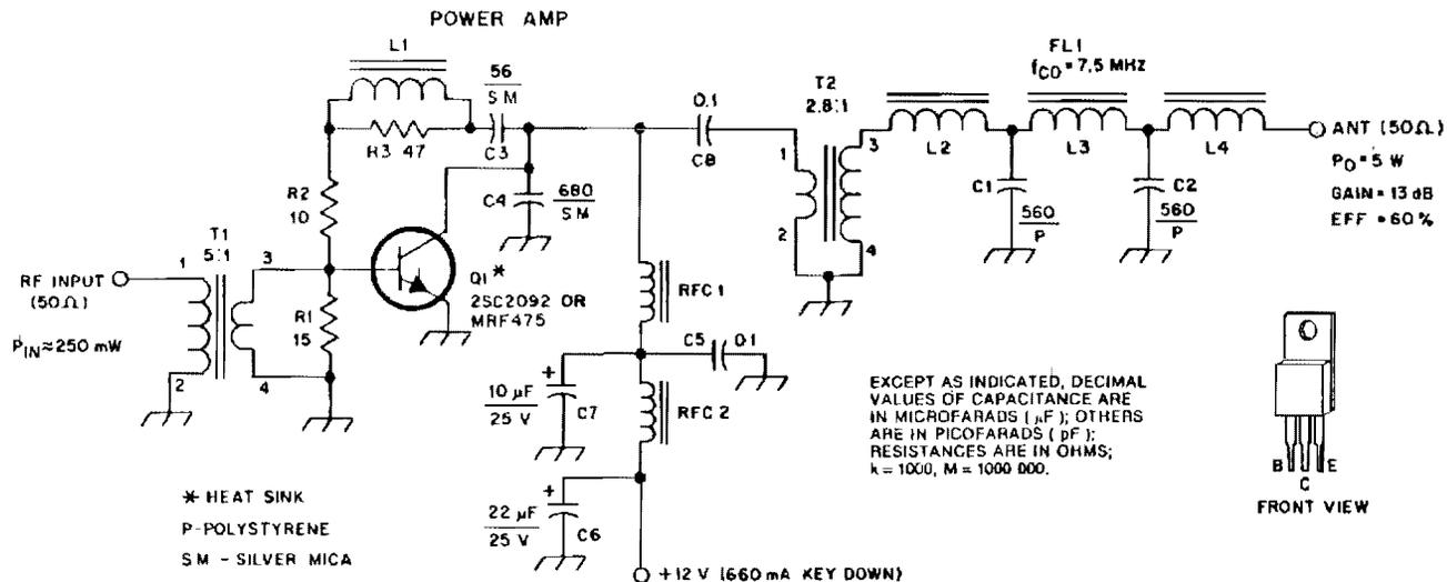
L1—0.22-μH inductor. Small RF choke or 8 turns of no. 24 enam wire on an Amidon T-37-6 toroid.
