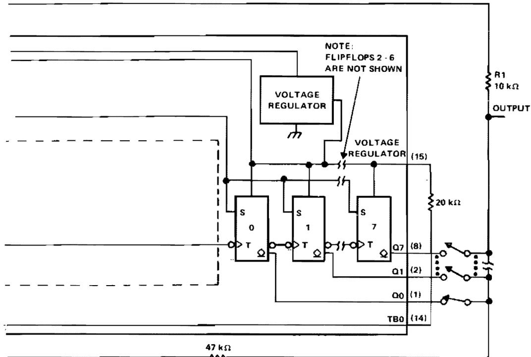
is connected to the regulator output via a 10 k ohm pull-up resistor. The output of the TBO drives the input to the 8-stage counter section.
