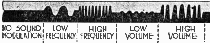
FIG. 4.—Changes in Variable Area Sound Track.
