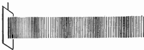
FIG. 1.—Radiation of Sound Waves from Vibrating Body.
