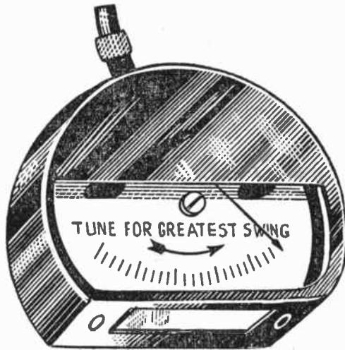
FIG. 11.—Reversed Scale Meter Tuning Indicator
