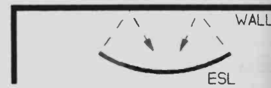
FIGURE 14-13: Poor position—rear wave reflects through dipole.
