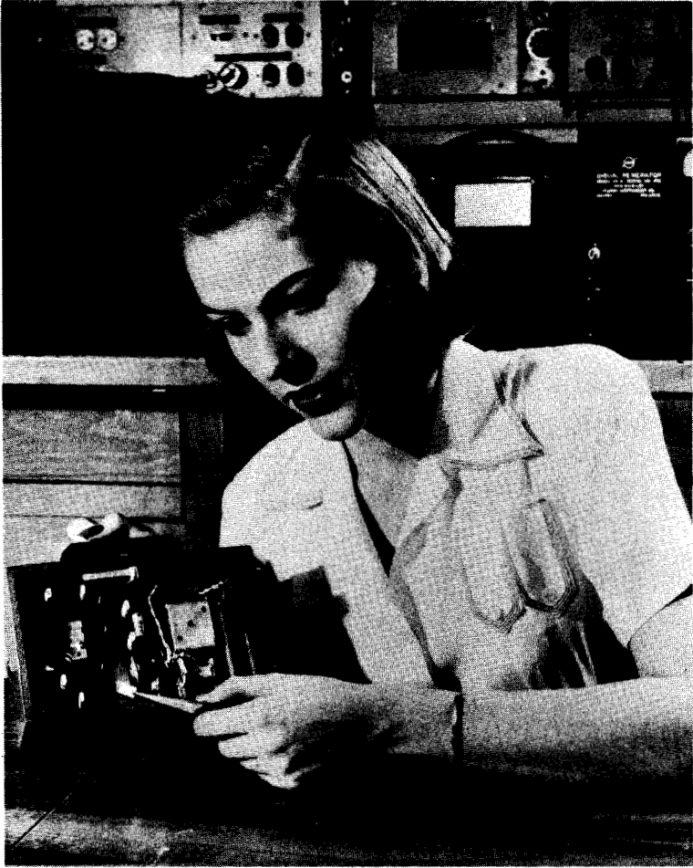
Figure 2. An experimental personal-type AM receiver in which transistors are used to permit a better than three-fold reduction in the size and weight of batteries needed to maintain a 100-hour operating life.
