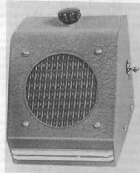
Fig. 424. Here, the circuit given in Fig. 421 has been assembled in a meter case, with a 3-inch speaker, for use as an Electronic Metronome. The SPST toggle switch on the side of the case is wired in series with the battery as an ON-OFF switch.
