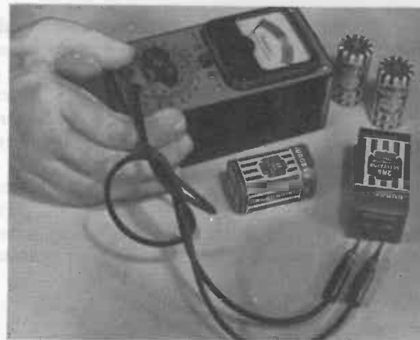
Fig. 603. Using a Battery Tester. Some internal load is placed across the battery when voltage measurements are being made.
