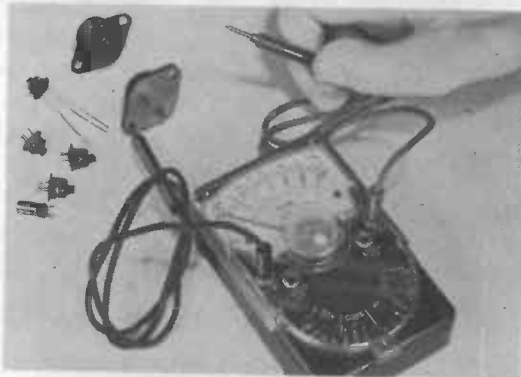
Fig. 606. Using an ohmmeter to check transistors.
