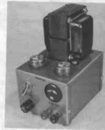
Fig. 520. Overall view of the completed Power Inverter.
