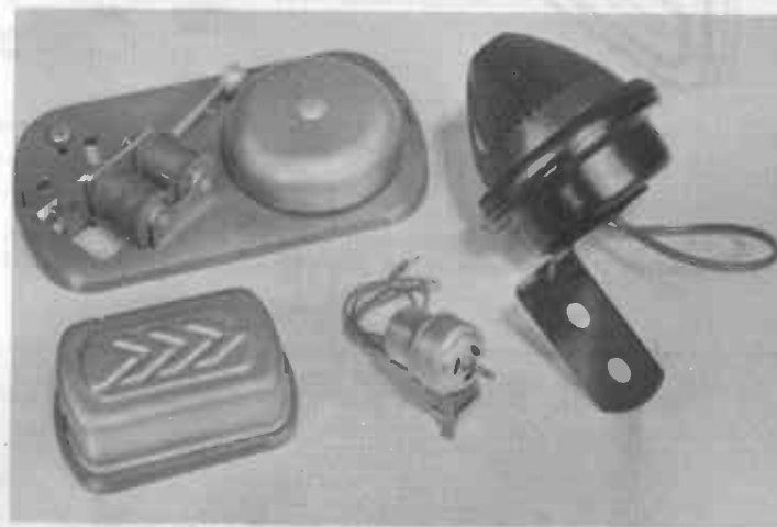
Fig. 405. Output devices that may be used with the Sensitive Relay . . . electric bell, buzzer, small motor, lamp. In each case, an external source of power (this can be either a heavy duty battery or step-down transformer) must be used to power the device.
