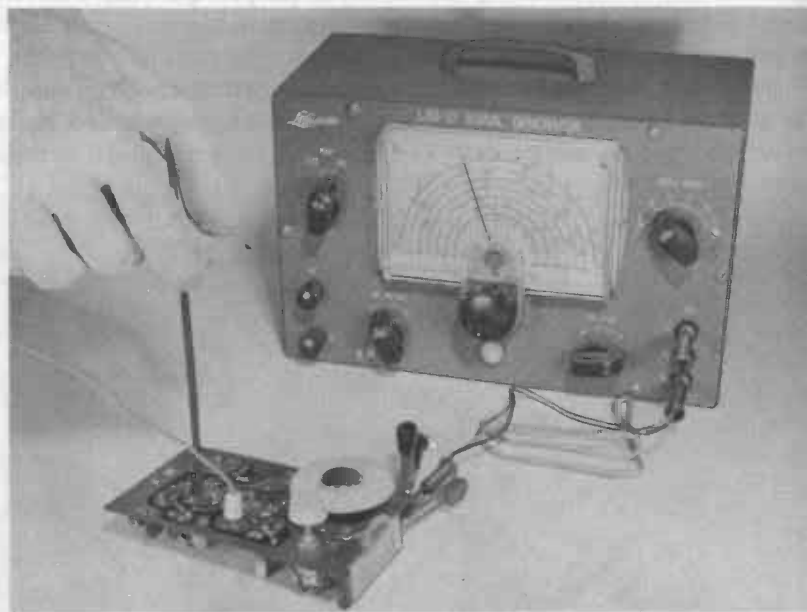
Fig. 318. Aligning the Pocket Superhet.
