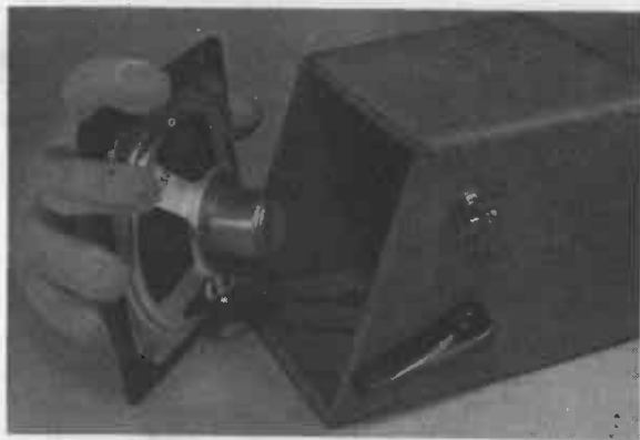
Fig. 214. The intercom Master, containing the amplifier, should be assembled in a wooden or metal cabinet of adequate size to hold the batteries as well as the electronic circuitry.
