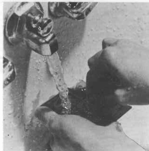
Fig. 1-16. Removing resist and deburring holes on completed board.
