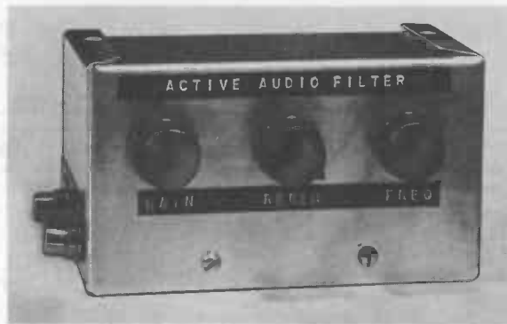
Fig. 3-12. The completed active filter unit.
