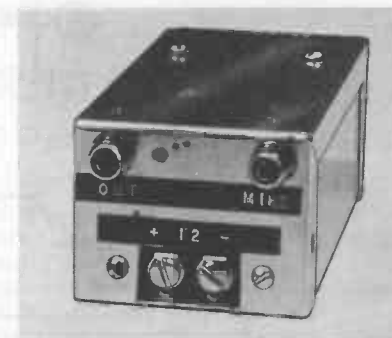
Fig. 6-6. Rear view of 50-mc vfo, showing connections.
