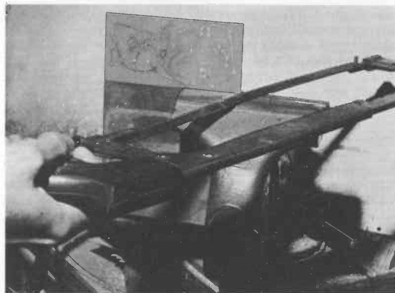
Fig. 1-15. Sawing the board to size.
