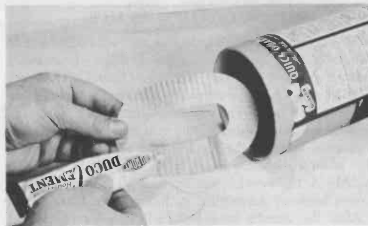
Fig. 9-5. Gluing the antenna.
