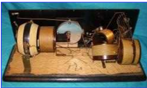
Figure 5 — This look inside the Paragon RA-10 shows why Paul Godley's skilled hands were needed in Scotland to detect the first transatlantic transmissions from American hams. The RA-10 was the tuning component in a complete receiver system. As evident in this photograph, tuning involved sensitive interplay between sensitivity, bandwidth and wavelength. [Photograph courtesy of Henry Rogers, W7HTR, photo]
