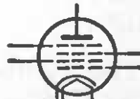
MULTI-GRID INDIRECTLY HEATED VACUUM-TUBE
