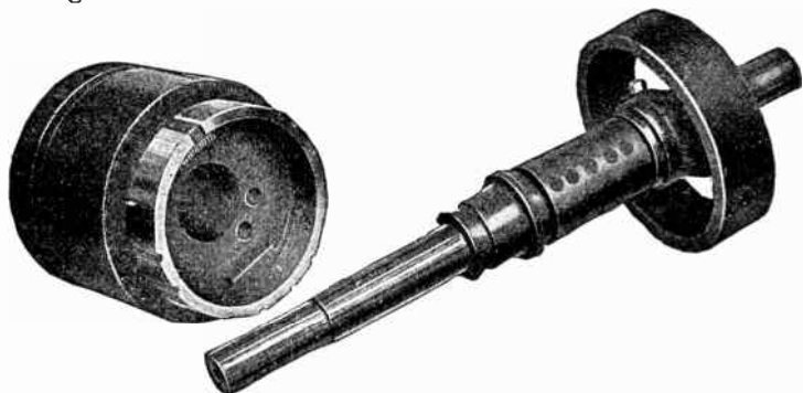
Figs. 1,867 and 1,868. —General Electric disassembled clutch as used on clutch type, single phase (KS) induction motor. In starting, the armature revolves freely on the shaft until approximately 75 per cent. of normal rated speed is reached. The load is then picked up by the automatic action of a centrifugal clutch, which rigidly engages an outer shell, keyed directly to the shaft. The brass friction band of the clutch is permanently keyed to the pulley end of the armature.
