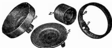
FIGS. 1,852 to 1,855.—Parts of General Electric centrifugal clutch pulley as used on clutch type, single phase induction motor. A, clutch; B, friction band; C, adjusting spring; D, outer clutch shell with pulley sleeve; E, solid removable pulley; F, internal mechanism comprising parts A; B. and C; G, outer shell and pulley comprising parts D and E.
