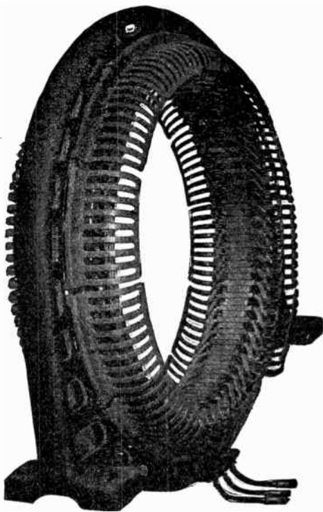
FIG. 1,395.—Western Electric stationary armature and frame of engine driven alternator. It is of cast iron and surrounds the laminated iron core in which the armature windings are embedded. Heavy steel clamping fingers hold the core punchings in place and numerous ventilating ducts are provided in the core at frequent intervals to allow free circulation of cool air. The armature coils are form wound, insulated, and retained in the core slots by means of wedges.
