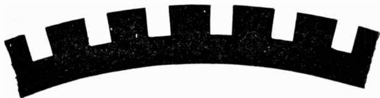
FIG. 1,518.—Style of armature core stamping used with bar wound machines. This construction, since there are no indentations in the teeth for wedges, makes it necessary to provide bands to hold the bars in place.
