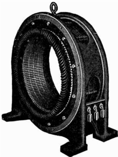
FIG. 1,474.—Western Electric stationary armature. In this type of armature, the core upon which the winding is placed, is built into the frame as shown, the core teeth projecting inwardly like internal gear teeth, forming a cylindrical chamber for the revolving field. The core is built up of iron, laminated and japanned to prevent eddy currents and hysteresis losses. The laminations are rigidly bolted between two heavy end plates. The armature coils are of copper bar impregnated with insulating compound. They are held in the slots by wedges which allow their ready removal for inspection or repairs.
