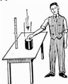
FIGS. 1.355 to 1.357.—Mechanical analogy of wattless current. If a man lift a weight any distance, as from the position of fig. 1.355 to position of fig. 1.356, he does a certain amount of work on the weight giving it potential energy. When he lowers it to its original position, as in fig. 1.357, the weight loses the potential energy previously acquired, that is, it is given back to the man, the "system" (man and weight) having returned to its original condition as in fig. 1.355. During such a cycle, the work done by the man on the weight is equal to the work done by the weight on the man and no useful external work has been accomplished.
