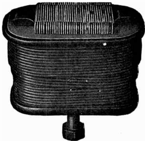
FIG. 1,467.—General Electric field coil, showing one method of winding. In the smaller machines the wire is wound on spools which are slipped over the pole pieces, which are built of sheet iron, spreading at the pole face so as to secure not only a wide polar arc for the proper distribution of the magnetic flux, but also to hold the field windings in place.
