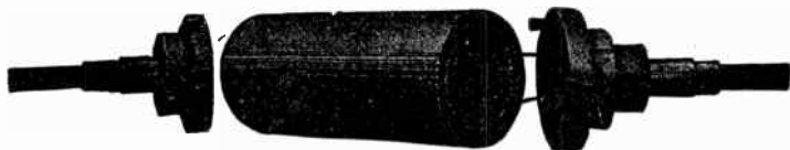
FIGS. 1,580 to 1,582.—Westinghouse two pole parallel slot field with ends removed showing construction. The parallel slot design of field construction is used in Westinghouse machines up to 10,000 kva. capacity. In fig. 1,581, the large holes at the end near the circumference of the cylinder are for the accommodation of the bolts that hold the bronze end discs and stub shafts. In winding, the cylinder is mounted on a horizontal turntable that rotates in a horizontal plane. The copper strap field coil winding is wound turn by turn under pressure and strip insulation is wound in between. When completed the turns are held rigidly in position with heavy brass wedges. An end disc made of bronze holds the stub shaft and is bolted to each end of the steel center. When the leads are attached to the collector rings the field is complete.
