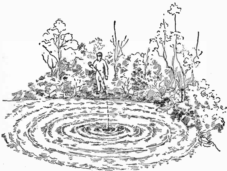
FIG. 4.—Effect of throwing a stone into still water; it produces waves which travel outwardly in expanding, concentric circles from the point where the stone enters the water or point of disturbance .
