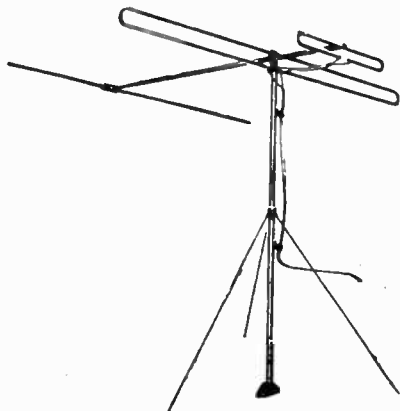
FIG. 40 —Double folded dipole antenna with reflector. An antenna of this type will give an excellent forward gain and high forward-to-back ratio. The antenna requires only one transmission line to receiver and requires no special matching network to give excellent performance on high and low bands. It is used preferably where transmitting stations are located not too far apart.
