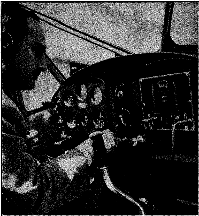
FIG. 2 —Illustrating aircraft radio receiver. The pilot receives code and messages through head phones which are interconnected to receiver as shown. (Courtesy Western Electric Co.)
