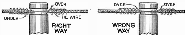
FIGS. 6,945 and 6,946.—Right and wrong methods of tying wires to grooved knobs, called tying in . In fig. 6,945, one end of the tie wire passes over the wire, the other passes under. Pliers must be used so that the wires will be firmly secured. In tying in the wires, the first and last knob should be tied in and the intermediate knobs tied in last. Where the wires are of a large size a block and tackle should be used, care being taken not to pull too tight as this will stretch the wire. The tie wires should be of solid wire and of the same size as the wire to be secured, one wire is passed underneath the wire and the other wire is passed over so that it is secured at both ends. Pliers should be used as tie wire cannot be properly secured by hand.
