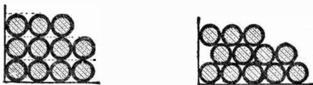
FIGS. 7,566 and 7,567.—Square and hexagonal order of "bedding." The term bedding is an expression used to indicate the relation between the cross sectional area of the winding when wound square, as in fig. 7,566, and when wound in some other way, as in fig. 7,567. In the square order of bedding, the degree of bedding equals zero.
