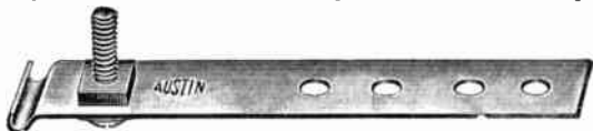
FIG. 7,281.—Austin tempered steel fish tape. It is made of flat tempered spring wire. The flat shape lends to its flexibility which is necessary for long runs of conduit having several bends. The tempering prevents the tape curling after long use. It comes in lengths, multiples of 25 feet.
