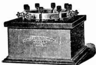
FIG. 6,832.—Standard resistance box: 100,000 ohms, in four units of 10,000, 20,000, 30,000, and 40,000 ohms. An "infinity" plug separates each coil from the ones adjacent. Segments are elevated from the hard rubber top by special washers in order to increase insulation. Binding posts are so arranged as not to be in the way when plugs are used.
