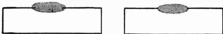
FIGS. 7,978 and 7,979.—Judging the arc length, 2. By appearance of the weld. Good penetration of the welding metal into the parent metal is not obtained with a long arc and there will be a bad overlap, as in fig. 7,978, while if the arc be short, there will be good penetration and a slight overlap, as in fig. 7,979. Another way to determine if the arc be too long is to examine the crater or depression in parent metal on breaking the arc, and see what the penetration looks like. If there be no penetration in the parent metal, then the arc is too long, providing of course, the proper electrode, current and correct polarity are used.
