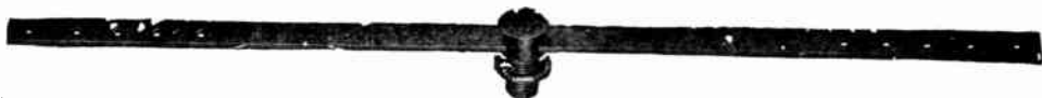
FIG. 7,264.—Austin straight bar hanger and stud. The stud is slotted allowing free movement along the bar, yet may be easily tightened by the locknut in any selected place, making it possible to set box at desired spot although conduit may bear a little off length.
