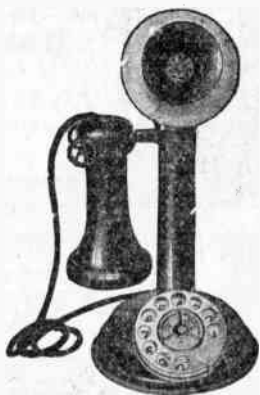
FIG. 8.420.—Automatic telephone wall type showing dial by which the subscriber makes calls without the aid of a central office operator.
