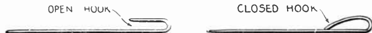
FIGS. 7,229 and 7,230.—Open and closed snake hooks. The open hook is used in hooking one snake to another. The closed hook is used for fishing.
