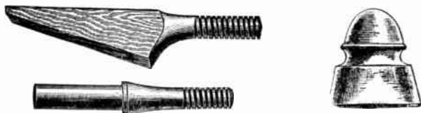
FIGS. 7,307 to 7,309.—Glass insulator and insulator pin in bracket. The insulator here shown is of the pony double petticoat type. Insulator pins are used with cross arms, brackets are attached direct to the pole.
