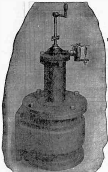
FIG. 8,956.—Sullivan unloading device with pilot valve for air intake conduit. It consists of a double beat valve, placed on the air inlet duct, and controlled by a pilot valve. The valve is set to shut off all the incoming air from the compressor when the receiver pressure rises above a predetermined point; that is, when the demand for air drops away. The compressor then runs under no load except that due to friction, compressing no air, and reducing the consumption of power to a very low factor. When the demand for air begins once more, that is, when the pressure in the receiver falls below the point at which the unloading device is set to act, the valve again opens fully, and the compressor automatically resumes its entire load until the demand for air again ceases, when the cycle of operation, just described, is repeated. The pilot valve may be adjusted to maintain any desired pressure in the air receiver.
