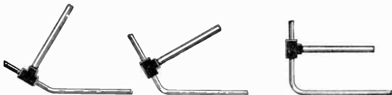
Figs. 7,148 to 7,150.—Correct method of making a quarter bend with a hickey. The pipe should be marked at the place where the bend is to be made, grasp pipe with hickey and raise pipe from floor a few inches, shift hickey and bend conduit a little more; keep shifting hickey until the proper bend is made. Unless hickey be shifted, the pipe will be kinked, thus making it difficult to pull the wires through the pipe; kinked bends will not pass inspection. To make an offset: Stand hickey on floor in an upright position with the bending part up, insert pipe into opening and pull down on the pipe, using the length of the pipe as a leverage, having made the bend as far as desired, turn the bend up and repeat as above.
