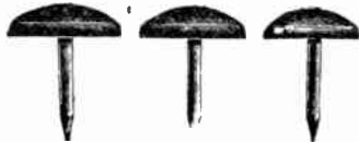
FIGS. 8.350 to 8.353.—Milonite nails and method of tacking two insulated wires. The heads are colored to match insulation and the wires can be tacked down without cutting or injuring the insulation.
