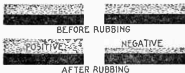
Figs. 6,109 to 6,112.—Positive and negative electricity. The rubbing process removes electricity from one body transferring it to the other.
