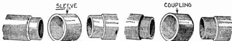
FIG. 7,355.—Sleeve joint type of fibre. Both the socket type and the sleeve type are easily aligned without the use of a mandrel.
