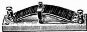
FIG. 7,440.—Thermal flasher. This simple flasher consists of a brass strip fixed at each end to a porcelain base and slightly arched upwards. The amount of this arching, however, is much less than is shown in the figure. The center of the strip carries a platinum contact on its upper surface, and opposite this is a platinum tipped contact screw which is carried in a brass angle piece fixed to the base. One terminal is fitted on one end of the strip, and the other is connected, through the angle piece, with the contact screw. The strip is wound from end to end with an insulated resistance wire, one end of this being soldered to the strip, and the other connected to the right hand terminal. When this device is switched into circuit with the lamps, the current first flows through the resistance, which cuts it down so much that the lamps are not visibly affected. The heat generated in the resistance causes the strip to curve still more, till at length contact is made, the resistance short circuited, and the lamps lighted.
