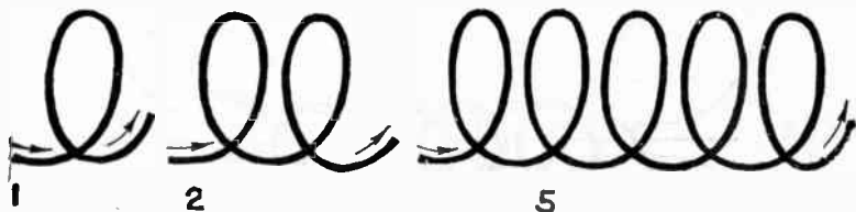
FIGS. 6,247 to 6,249.— Ampere turns. By definition the ampere turns is equal to the product of the current passing through a coil multiplied by the number of turns in the coil. Thus, in fig. 6,247, ampere \times 1 turn = 1 ampere turn; in fig. 6,248, 5 amperes \times 2 turns = 10 ampere turns; in fig. 6,249, 2 amperes \times 5 turns = 10 ampere turns.
