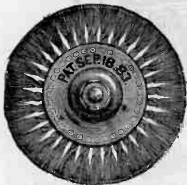
FIGS. 6.379 and 6.380.—Hanson and Van Winkle swing type, circular steel wire, casting brush. The steel wires are twisted in knots and the knots are hung on rods around the hub, as shown in fig. 6.379, so that they will turn around the rods if the work is held too close to the brush wheel. In using the brush the work should be held so as to be just in contact with the ends of the wires. The brush shown is about 15 inches in diameter, and should not be run much faster than 1,000 r.p.m.
