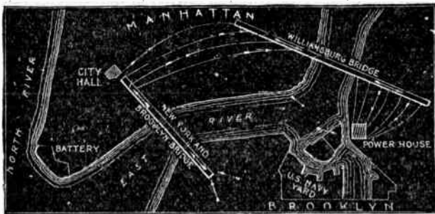
FIG. 6,359.—Electrolysis in lower New York. The figure illustrates current movements as discovered. The power house is located near the navy yard in Brooklyn. A portion of the returning currents, as shown by arrows, flows over the New York and Brooklyn bridge to Manhattan, thence north to Williamsburg bridge via underground mains, subway structures, and other metals, and passes over that bridge back to Brooklyn, thence through mains to rails and negatives, to power house. In this case damage may be expected at three points: 1, where currents leave bridge metals on the Manhattan side; 2, where they leave pipes to enter Williamsburg bridge; 3, where they leave same bridge for pipes in Brooklyn side. When the two bridge structures are connected in Manhattan as proposed, then there will be further changes in the direction of current. Before the Williamsburg bridge was built, these currents recrossed through the river bed, leaving mains all along the docks in the Manhattan side, for the river, and leaving the river for mains or other metals along the docks of the Brooklyn side. Traces of these currents have been found as far north as 23rd St., a distance of over two miles from the Brooklyn bridge. Since the Williamsburg bridge has been built, nearly all traces of these currents flowing north of it have disappeared, showing that the mass of metal composing the structure acts as a short circuit or path of lower resistance which carries practically all of the returning currents flowing from Manhattan back to Brooklyn.
