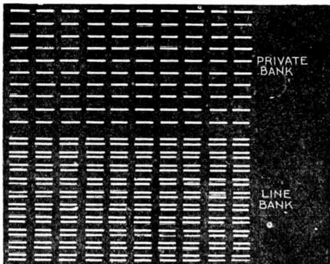
FIG. 8,434.—Diagram showing contacts of line and private banks of a 100 line system. These banks form a part of the connector switch.
