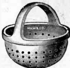
FIGS. 6.372 and 6.373.—Various dipping vessels. Fig. 6.372, deep glazed earthenware dipping basket; fig. 6.373, shallow glazed earthenware dipping basket. The aluminum basket is adapted for use in washing and dipping in all acid solutions, but cannot be used in potash solutions. Different shapes and sizes of basket are required for various kinds of work. Successful dipping depends, how-
