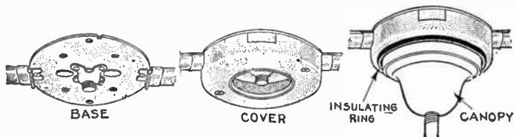
FIGS. 7,046 to 7,048.—Base, cover, and canopy for fixture outlets; note knock out holes in base for picking up concealed wiring.
