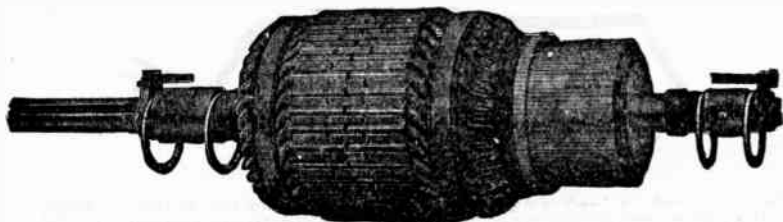
FIG. 7.829 —Fairbanks Morse type TR machine armature construction. The armature core is built up of thin sheet steel laminations with notches in the circumference, which, when the discs are placed together, form grooves or slots to receive the armature coils. With specially designed tools these notches are so accurately spaced that no filing of the slots is required. The armature cores for the Nos. 23, 24, 25, 26, 27, 28 and 29, machines are mounted on a cast iron spider, which also carries the commutator, making the two parts entirely self-contained, and with this construction, it is possible to remove the armature shaft, without disturbing the core, commutator or windings.
