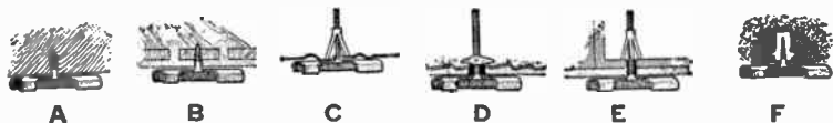
FIGS. 7,034 to 7,039.—Methods of supporting National metal molding. Fig. A, on wood surfaces use a No. 8 flat head wood screw; fig. B, on lath and plaster use a 1\frac{1}{4} in. No. 8 flat head wood screw; fig. C, on metal ceilings use one toggle bolts 2 ins. long; fig. D, on plastered ceilings of metal lath, use flat toggle bolt; fig. E, on tile use flat toggle or one toggle bolt; fig. F, on concrete use lead shields.
