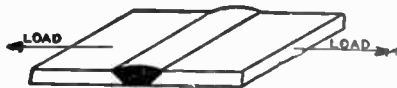
FIGS. 8,041 to 8,043.—Strength of welds. The table showing allowable strength of fillet welds applies to figs. 8,041 and 8,042. For figuring the strength of the butt weld shown in fig. 8,043, use the sectional area of the steel plate at a stress of 5,000 lbs. per sq. in. for dynamic or vibration load and 13,000 lbs. per sq. in. for static load in tension or 15,000 lbs. per sq. in. in compression.
