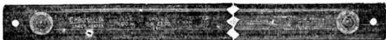
FIG. 8,233.—Wiegand one inch wide, strip heater designed for use in building special machinery where heat is required at some local point on the machinery as is the case in package forming and sealing machines, marking machines, and other manufacturing process equipment. These strip heaters are rated at comparatively high wattage per sq. in. They safely operate at red heat, not exceeding 1,300° Fahr. The single end strip heater shown has the usual advantage of bringing the terminals to one end which is often desirable in machine building.
