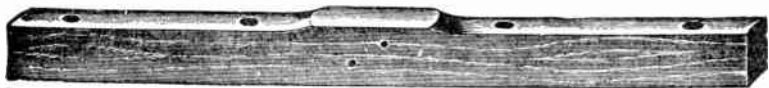
FIG. 7,310.—Cross arm which carries the insulator pins. The standard cross arm is 3\frac{1}{4} \times 4\frac{1}{4} inches, double painted, and bored for 1\frac{1}{2} inch pins and two \frac{1}{2} inch bolt holes. Telephone arms are 2\frac{3}{4} \times 3\frac{3}{4} inch, bored for 1\frac{1}{4} inch pins and two \frac{1}{2} inch bolts.
