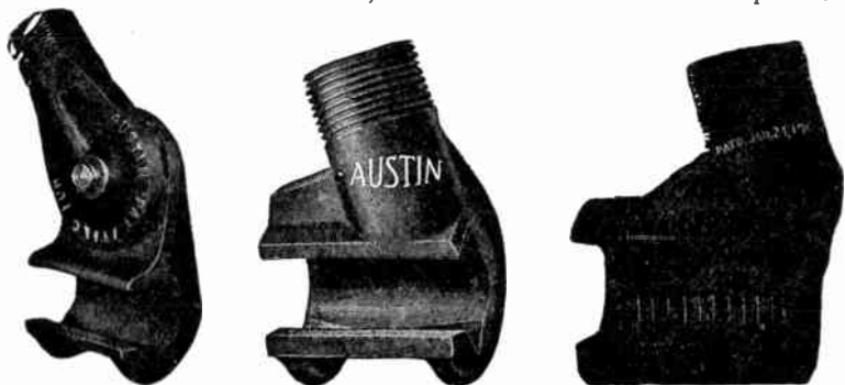
FIGS. 7,282 to 7,284.—Austin Hickeys. Fig. 7,282, adjustable; fig. 7,283, "bull dog" non-skid; fig. 7,284, Lakin for short bend in awkward positions.
