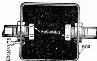
FIG. 7,158.—Method of securing conduit to outlet or junction boxes. Two locknuts and a bushing must be used as shown.
