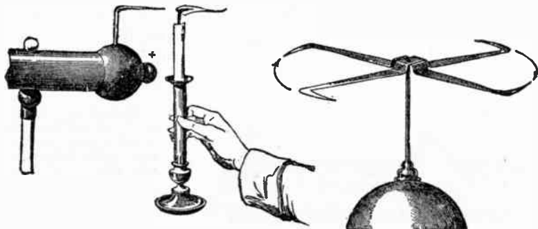
FIG. 6,131.—Experiment to illustrate the effect of pointed conductors.
