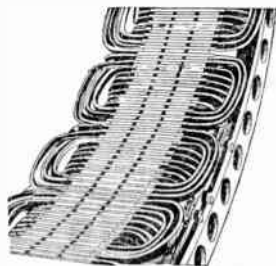
FIGS. 7,755 to 7,757.—Separate coils, and section of Allis-Chalmers alternator with coils in place.
