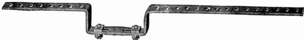
FIG. 7,265.—Austin universal box cleat used chiefly for side wall construction can also be used on ceiling work. By nailing across the front of joists a flush position for the box is obtained.
