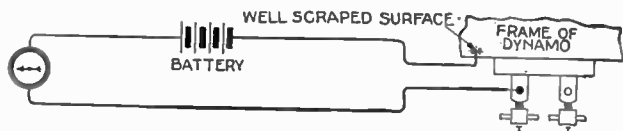
FIG. 7,652.—Method of testing dynamo for short circuits. T, T, are terminals under test. In testing, if a deflection of the needle be produced when the galvanometer terminal is in contact with either, the terminals are in contact with the frame, and they should then be removed, and the fault repaired by additional insulation or by reinsulating.
