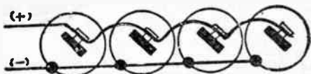
FIG. 6,179.—Multiple or parallel connection. The voltage is the same as that of a single cell, but the current is equal to the amperage of a single cell multiplied by the number of cells.
