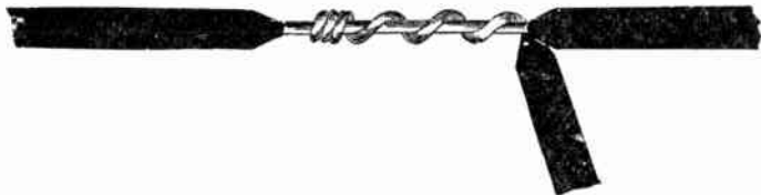
FIG. 7,292. —Tee or branch tap joint. This joint is used in junction boxes. The splice is made the same as the running butt splice only all the wires are wound around the same wire. In splicing , the wire to be tapped is skinned so that just enough insulation is removed so that the proper number of turns may be wound around it. Hold the new wire that is to be tapped parallel with the wire that is already installed, and with a pair of pliers wind the wire around 4 or 5 times and clinch end of wire so it will not protrude.
