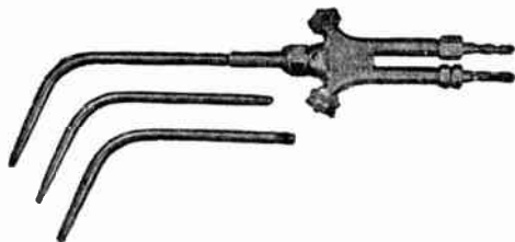
FIGS. 8,213 to 8,215.—Airco-Davis-Bournonville lead burning torch designed for "burning" or welding lead. By attaching a proper mixing head and using City gas instead of acetylene, this torch may be used for soldering. The temperature with gas is about 3,500° Fahr.
