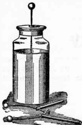
Figs. 6,107 and 6,108.—The Leyden jar and discharger. Its discovery is attributed to the attempt of Musschenbroek and his pupil Cuneus to collect the supposed electric "fluid" in a bottle half filled with water. The bottle was held in the hand and was provided with a nail to lead the "fluid" down through the cork to the
