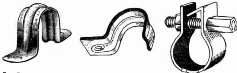
Figs. 7,164 and 7,165.—Conduit clamps. Fig. 7,164, old style requiring two screws; fig 7,165 new style, single screw.
