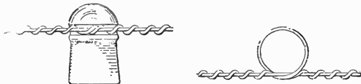
FIGS. 7,334 and 7,335.—Approved method of attaching wire to an insulator; elevation and plan of insulator and tie. The line wire is first laid in the groove of the insulator, after which a short piece of the same size of wire is passed entirely around to hold it in place, then it is twisted to the line at either side with pliers.
