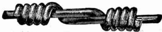
Fig. 7.331.—American wire joint. This is a simple method of connecting the ends of the sections of wire by tightly twisting the ends around each other for a few turns; it is the standard Western Union wire joint.
