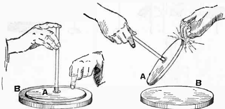
FIGS. 6,143 and 6,144.—The electrophorus and method of using. Charge B; place A, in contact with B, and touch A (fig. 6,143). The disc is now charged by induction and will yield a spark when touched by the hand, as in fig. 6,144.
