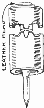
FIG. 6.939.—Knob complete with nail and leather head. The leather head is pinched over on the side so that nail cannot fall out.
