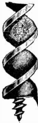
FIG. 7.114.—Boring machine for boring porcelain tube holes in knob and tube work. It will bore a hole parallel with the floor (avoiding slanting tubes) and in less time than with a brace.
