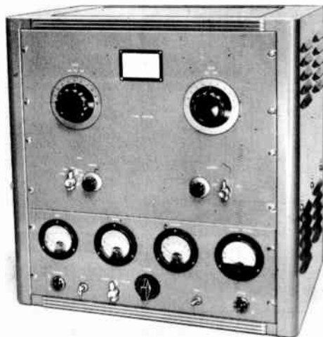
Fig. 6-72—The kilowatt 4-400A amplifier and its control unit are mounted in a 21-inch gray hammer-tone rack cabinet (Bud CR-1727). Shelf brackets (Bud SA-1350) are mounted on both sides of the cabinet to hold the amplifier chassis. Below the meters, from left to right: filament pilot light, key-type a.c. switch, Class AB 1 /C bias switch, screen autotransformer, plate switch and plate pilot light.
