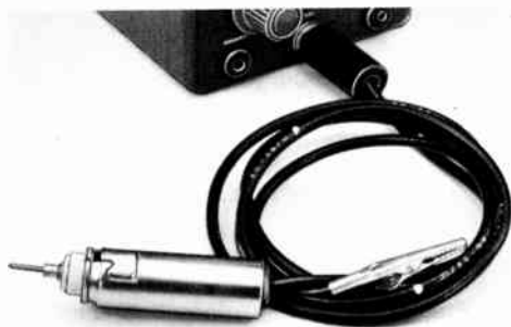
Fig. 21-35—The r.f. probe is used in conjunction with a vacuum-tube voltmeter. The case of the probe is constructed from a 7-pin ceramic tube socket and a 2\frac{1}{4} -inch tube shield. A half-inch grommet at the top of the tube shield prevents the output lead of the probe from chafing. The flexible copper-braid grounding lead and alligator clip provide a low-inductance return path from the test circuit. The d.c. output of the probe goes to the phone plug, which plugs into the d.c. input jack of the v.t.v.m.
