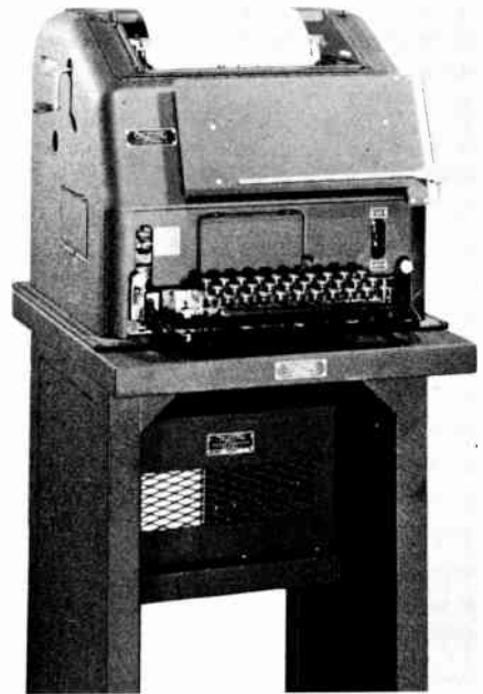
The Model 15 page printer, shown here with table, is used in a great many RTTY stations.
