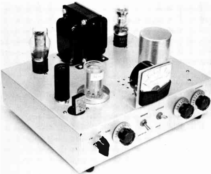
Fig. 6-40—The inexpensive 75-watt transmitter is a two-tube five-band crystal-controlled transmitter; v.f.o. control can be added at any time. To simplify construction and testing, plug-in coils are used, housed in the two shield cans (Millen 80011 or Miller S-42 with S-42C base). The crystal-oscillator tube, a 12BY7, is housed in the black tube shield at the left; the 1625 amplifier tube is mounted under the chassis.
