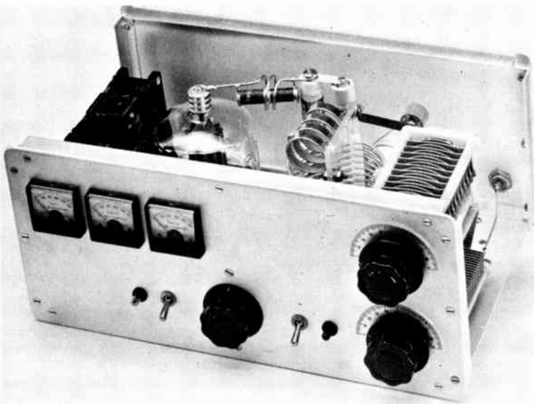
Fig. 6-68—The compact kilowatt amplifier with its perforated-metal cover removed. Using a 3-400Z in a grounded-grid circuit, it handles a kilowatt p.e.p. input at 3000 volts with ease. The (2-inch) meters monitor plate voltage, grid current and plate current. Panel is 7 x 15 inches; the bottom plate is 8 \frac{3}{4} inches wide. (Built by Robert Smith, WILLF, Simsbury, Conn.)
