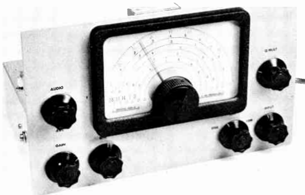
Fig. 5-38—This five-tube receiver is band switched, 3.5 through 30 Mc. The oscillator tuning dial (Miller MD-8) has a two-speed drive. Input stage is a 7360 mixer with r.f. Q multiplication.
