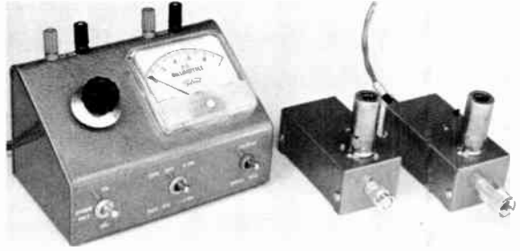
Fig. 21-27—Two diode noise generators and (left) their power supply. Useful generator range is (right) 7 to 90 Mc. and (center) 90 to 450 Mc.
