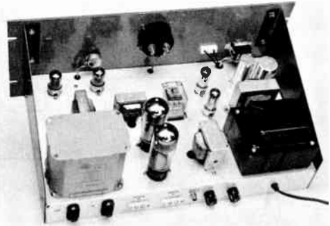
Fig. 8-15—A look at the top of the modulator chassis. The power supply is located on the right, the speech amplifier tubes are at the upper left, and the modulation transformer is at the lower left. The control relay, K_1 , is at the center of the chassis, just behind the meter.
