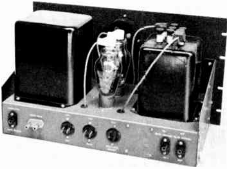
Fig. 8-18—A typical Class B modulator arrangement. This unit uses a pair of 811As, capable of an audio power output of 340 watts, and includes a splatter filter. The modulation transformer is at the left and the splatter choke at the right. All high-voltage terminals are covered so they cannot be touched accidentally.
