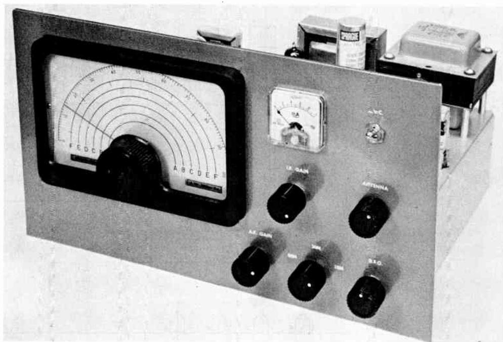
Fig. 5-55—The HB-67 is a five band receiver featuring a mechanical filter for selectivity. A two-speed dial (Miller MD-8) is fast enough for quick jumps around the band and slow enough for ease in tuning s.s.b. Audio-derived fast-attack slow-decay a.g.c. also contributes to ease of tuning.
