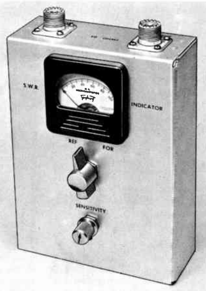
Fig. 13-20—The Monimatch, an s.w.r. monitor that can be left in the line at all times. The unit shown here will handle a kilowatt.
