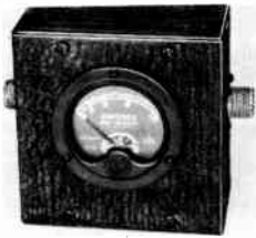
Fig. 21-31—R.f. ammeter mounted for connecting into a coaxial line for measuring power. A "2-inch" instrument will fit into a 2 × 4 × 4 metal box.
