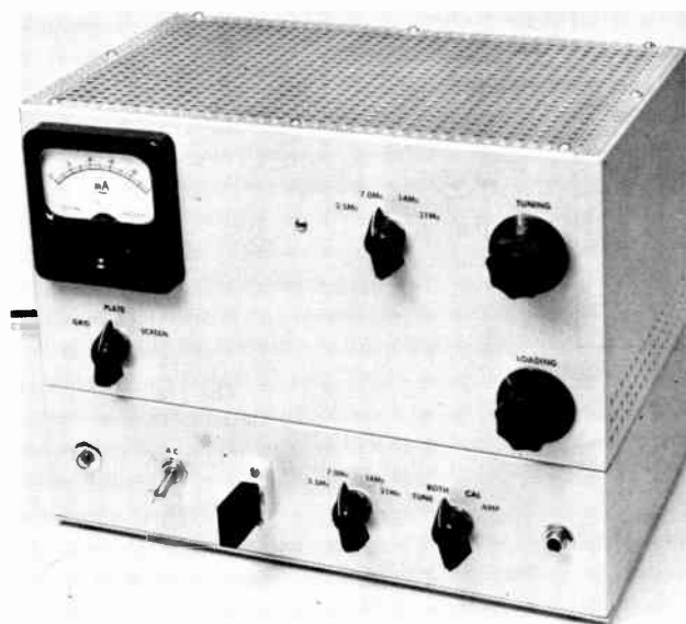
Fig. 6-35—The four-band 50-watt transmitter is a two-tube unit much superior to the "simple 1-tube" transmitters often recommended for newcomers to amateur radio. The cabinet combines a chassis and an aluminum "utility box."
