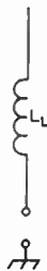
Fig. 19-34—Placing the loading coil at the center of the whip antenna, instead of at the base, increases the radiation resistance, although a larger coil must be used.
