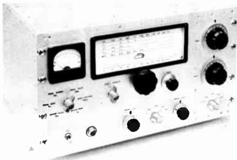
Fig. 6-60—The 450-watt c.w. transmitter is mounted on I beams of Reynolds T-shaped aluminum to allow air to be drawn in at the bottom and cool the 4E27A/5-125B final by convection. Controls along the bottom, from left to right, are the power switch and associated pilot light, driver plate tuning, exciter band switch, exciter tuning and final band switch. Above, from left to right, are the meter switch, spot-operate control, v.f.o. tuning, final drive control and final loading. Final plate tuning control is at the upper right. The v.f.o. dial is an Eddystone 898, the pointer knobs are National, and all other dials are Johnson. (Built by Walter Lange, W1YDS, West Hartford, Conn.)
