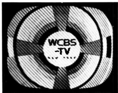
Fig. 23-5—"Cross-hatching," caused by the beat between the picture carrier and an interfering signal inside the TV channel.
