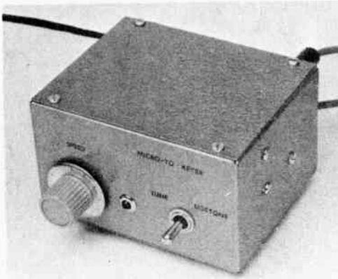
Fig. 1 — This electronic speed keyer is 100-percent solid state and uses both integrated circuits and bipolar transistors. It operates over a speed range of 10 to 50 wpm and contains its own built-in monitor. This circuit was originally described in QST , August, 1967, by K3CUW.
