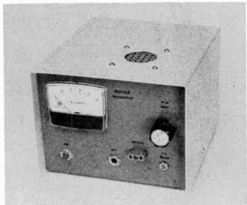
Fig. 1 — This is the completed transmitter for 160- to 20-meter operation. The plate tuning control is at the upper right, and just below, the loading capacitor, C2.
