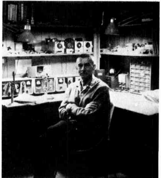
This modern-day operating position was built by KØGKB, of Boulder Colorado. Installing a desk in a corner allows a large amount of table-top area, to be within reach of the operator. Shelves mounted above the operating position provide convenient storage space for books and station accessories.
