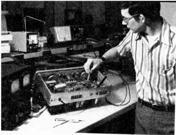
Fig. 8-42 — Receiver alignment requires a stable signal source (a signal generator) and voltmeter. Alignment of communications receivers should be checked at least once a year.
