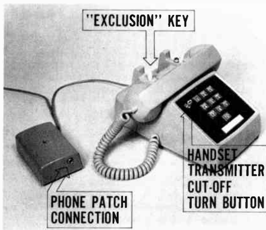
Fig. 15F-1 — The voice coupler, to the left of the touch-tone telephone, is supplied by the telephone company. The coupler is normally fixed to a wall or desk, and contains a jack for connection of the amateur's phone patch.
