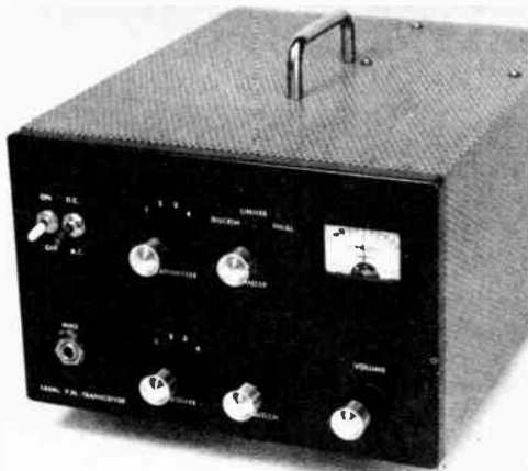
Fig. 14-25 — A homemade fm transceiver. The transmitter section uses the solid-state exciter and amplifier shown in Chapter 10.
