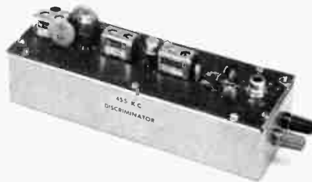
Fig. 14-23 — The solid-state fm adapter is constructed on a 6 X 2-inch etched-circuit board, mounted on a homemade chassis.
