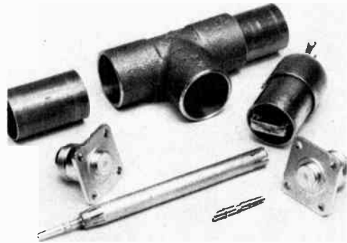
Fig. 22-24 — Major components of the line sampler. The brass T and two end sections are at the back of the picture. A completed probe assembly is at the right. The N connectors have their center pins removed. The pins are shown with one inserted in the left end of the inner conductor and the other lying in the right foreground.
