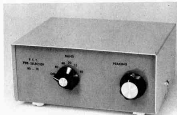
Fig. 8-36 – The 80- to 10-meter preselector is constructed in a cabinet made from two U-shaped pieces of sheet aluminum. Press-on feet are used. Panel decals (obtained from H. H. Smith) lend a "finished" appearance to the unit.
