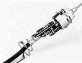
Fig. 17-54 — Inside the probe. The 1N34A diode, calibrating resistor, and input capacitor are mounted tight to the terminal strip with shortest leads possible. Spaghetti tubing is placed on the diode leads to prevent accidental short circuits. The tube-shield spring and flexible-copper grounding lead are soldered to the cable braid (the cable is RG-58/U coax). The tip can be either a phone tip or a short pointed piece of heavy wire.
