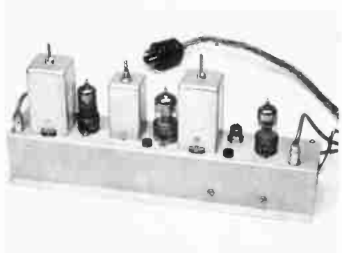
Fig. 14-20 — The fm adapter, wired for connection to a Collins 75A2.
