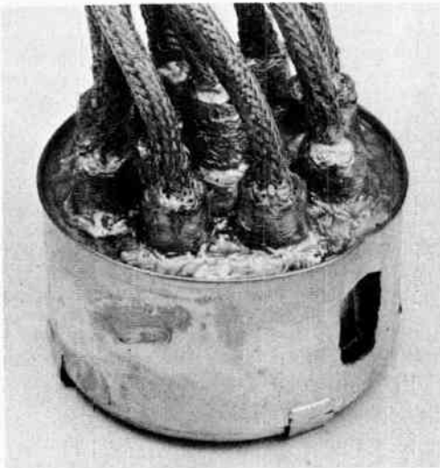
Fig. 10-4 — A close-up view of the distributor shield can. The shield braid over each spark-plug wire is soldered to the top of the can, and the can is grounded to the engine block.
