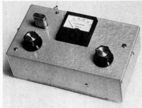
Fig. 17-56 — The deviation meter is constructed in a Calectro aluminum box. A four-position switch is at the lower right. The crystal plugs in on the left, with the frequency adjusting trimmer just below. A short whip or pickup wire can be plugged into the phono connector that is mounted on the back wall of the box.
