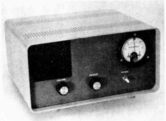
Fig. 14-39 — Front view of the complete receiver for 10-, 6-, or 2-meter fm. The unit is housed in an LMF 10 X 5 X 2-inch cabinet. Knobs are Kurz-Kasch S-748-1L.
