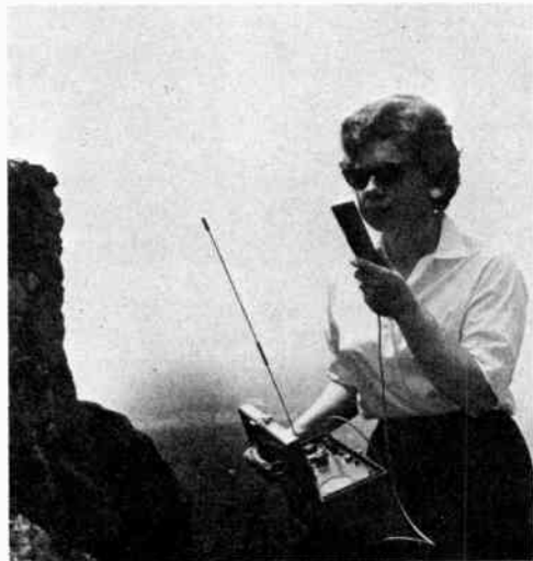
Fig. 10-1 – Effective portable operation can be realized when using lofty locations for vhf or uhf. Here, W1CCK is shown operating a battery-powered, 150-mW output, 2-meter transceiver. With only a quarter wavelength antenna it is possible to communicate with stations 25 miles or more away. Low-power transistor equipment like this unit will operate many hours from a dry-cell battery pack.
