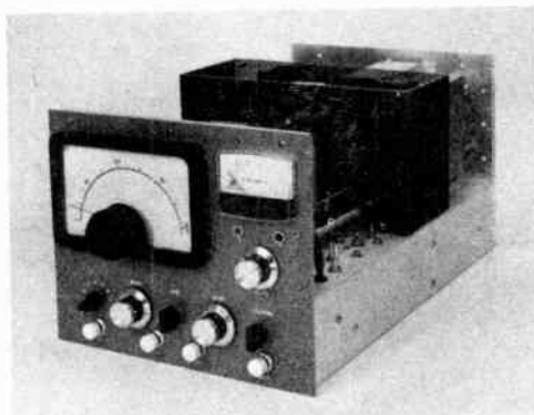
Fig. 1 — Front view of the cw transmitter. All metal work is done with sheet and cane-metal sections.
