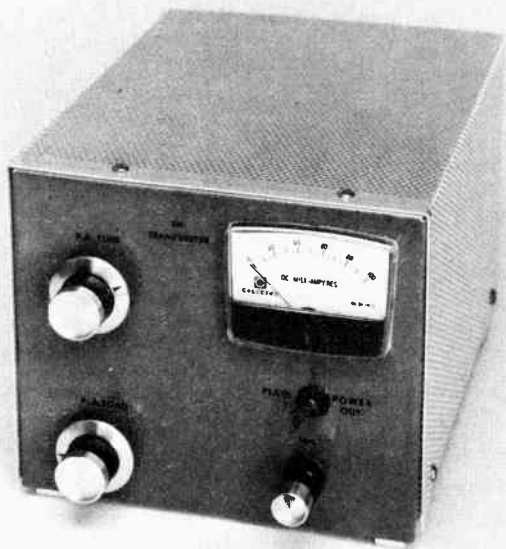
Fig. 7-3 — The 6-meter transverter, with shield cover in place. Large knobs are for amplifier tuning and loading. Small knob, lower right is for a meter sensitivity control. The meter switch is just above it.
