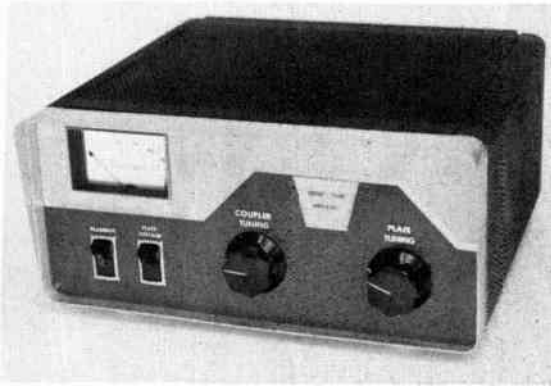
Fig. 1 — Front view of the 800-watt amplifier. An LMB CO-1 cabinet, Simpson 02640 meter, and Kurz-Kasch S-649-70L knobs are used, giving a modern appearance. Coils are changed through the door in the top of the cabinet.
