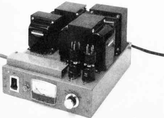
Fig. 1 — The Universal Power Supply is constructed on a standard-size aluminum chassis. Back-to-back plugs with appropriate jumper wires make changing from 117-V to 220-V input operation or from 6.3-V to 12.6-V filament operation a simple matter of reversing a plug.
