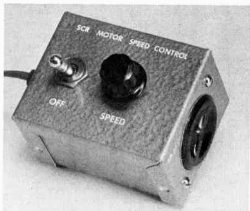
Fig. 18-1 — Small enough to fit in the palm of your hand, the SCR motor-speed control is housed in a small Minibox.
