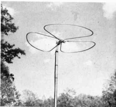
Fig. 10-18 — The Big Wheel, an omnidirectional horizontal antenna for the 144-MHz band designed by W1FVY and W1IJD. Radiating elements occupy an area approximately 40 inches in diameter.
