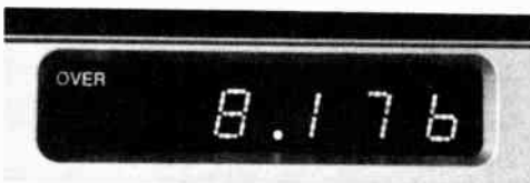
Fig. 6-12 — A 5-digit readout using light-emitting diodes.
