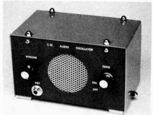
A cw code-practice oscillator along with a speaker may be mounted inside a homemade aluminum box. If desired, the battery could be mounted inside the enclosure also, thereby allowing easy portability of the unit.
