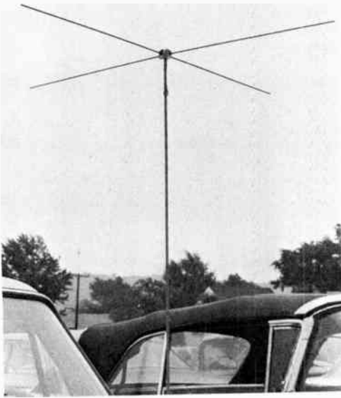
Fig. 10-20 — Two-meter turnstile antenna shown mounted on the front of an automobile. The miniature coax cable which feeds the antenna is taped to its 1/4-inch diameter steel supporting rod. The ends of the antenna elements should be flattened, or rounded, to make them safer in the event of accidental contact with the human body.
