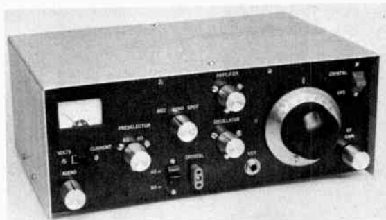
Fig. 10-33 — Front view of the cw transceiver. The chassis and cabinet are homemade, and consist of two U-shaped pieces of thick aluminum stock. The panel is painted dark green to permit the white decal labels to stand out prominently.
