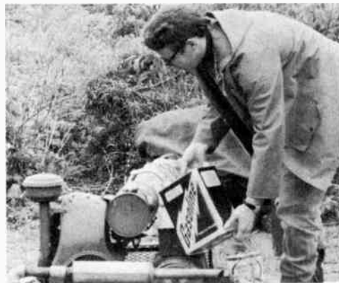
Fig. 10-5 — Gasoline-powered ac generators used for portable/emergency operation should be treated for ignition noise in the same manner as automobile engines are. The frame of the gas generator should be connected to an earth ground, and the entire unit should be situated as far from the operating position as possible. This will not only reduce ignition noise, but will minimize ambient noise from the power unit. (Shown here is K1GTK during Field Day operations.)
