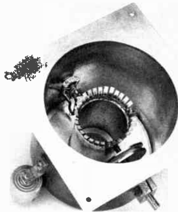
Fig. 7-47 — Interior of the plate circuit assembly, showing the center conductor with its ring of finger stock, the output-coupling loop, left, and the disk-type tuning capacitor, right.
