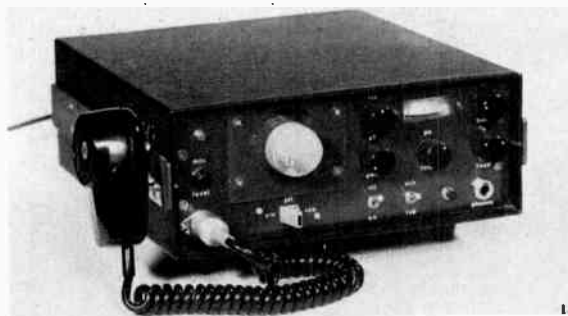
Fig. 1 — The transceiver is constructed in a homemade cabinet. A 36:1 gear reduction dial is employed. Other packaging arrangements may be used to fit a particular home- or mobile-station requirement.
