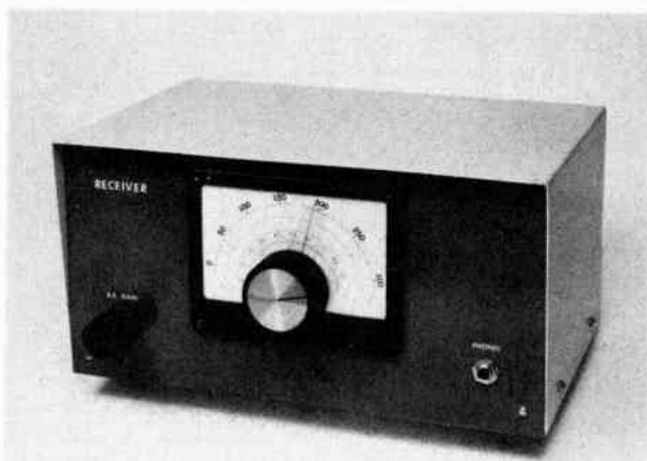
Exterior view of the three-band beginner's receiver. The dimensions are 11 × 5-1/2 × 7 inches. The vernier dial is calibrated for 10 kHz per division. The front panel is finished in dark blue. White press-on decals are used to identify the gain control and phone jack. The receiver was built by WA1CQW.
