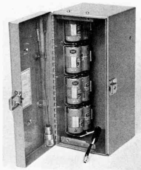
Fig. 6 — Eight size D cells are series connected to provide 12 volts. They are mounted in Keystone holders on the back wall of the bond box. The 1/4-inch diameter hole in the front of the cabinet (upper right of photo) permits final calibration of the receiver (C20) after the installation is completed. The hole is opposite the shaft of C20.
