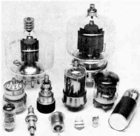
Transmitting tubes are in the back and center rows. Receiving tubes are in the front row (l. to r.): miniature, pencil, planar triode (two), Nuvistor and 1-inch diameter cathode-ray tube.
