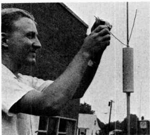
Fig. 10-15 — K1MET prunes a capacity hat for antenna resonance at the low end of the 160-meter band. The Webster Big-K antenna is first tuned for the high segment of the band. The capacity hat is clipped on when operation on the "low end" is desired. Fine adjustments can be made by increasing or decreasing the spacing between the two No. 10 wires.
