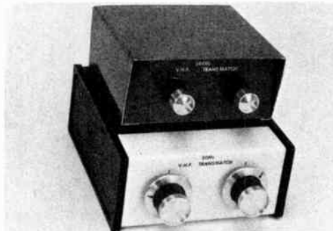
Fig. 22-21 — These 6- and 2-meter Transmatches may be used with powers up to 500 watts. They can be employed with either balanced or unbalanced feeders.
