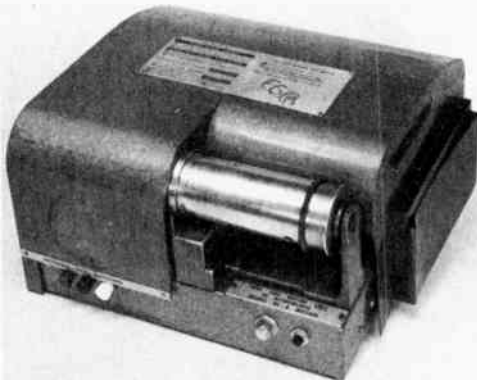
Western Union Telefax transceiver. Machines of this type are available as surplus for less than $20. The drum accommodates a sheet of paper measuring approximately 4 1/2 x 6 1/2 inches.
