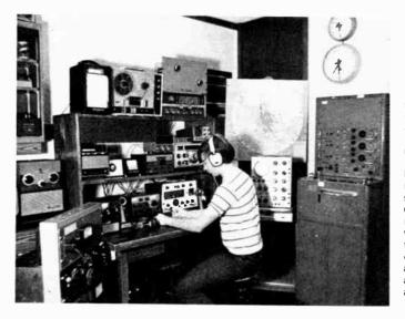
This station, owned by the Talcott Mountain UHF Society, WA1IOX, is designed expressly for moonbounce and advanced amateur satellite work. The operator (WA1JLD) is able to control simultaneously the several re-ceivers, "steer" the antennas, and still have access to the peripheral equipment for data recording and measurement.
