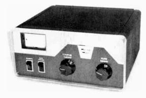
Fig. 1 – Front view of the 800-watt amplifier. An LMB CO-1 cabinet, Simpson 02640 meter, and Kirsh-Kash S-649-70L knobs are used, giving a modern appearance. Coils are changed through the door in the top of the cabinet.
