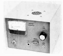
Fig. 1 – This is the completed transmitter for 160to 20-meter operation. The plate tuning control is at the upper right, and just below, the loading capacitor, C2. frequency crystals are required with the transmitter. The term "fundamental" means that the crystal frequency is the same as the desired output frequency. The transmitter will also cover 160 and 20 meters.
