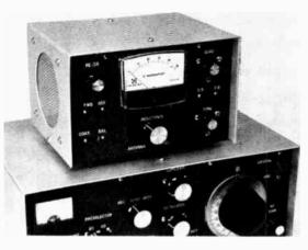
The QRP console is shown atop the QRP transceiver. These electrically compatible units have look-alike decor with green panels, white labels, and lye-bath finished aluminum covers. Kurz-Kasch 700 Series knobs are used on both pieces of gear (Catalog No. 112, Kurz-Kasch, Inc., Dayton, Ohio 45401).
