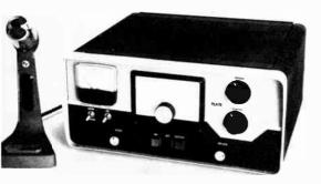
The ssb transmitter uses a minimum number of panel controls. Push-button switches activate the power supply and the output-metering function. A J. W. Miller MD-4 dial, LMB CO-1 cabinet and Simpson Wide-Vue meter lend a modern appearance to the unit.
