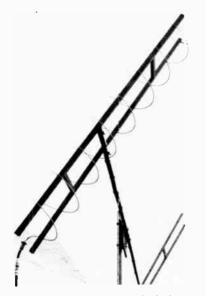
Fig. 22-20 – An 8-turn 432-MHz helical array, wound from aluminum clothesline wire. Left-hand polarization is shown. Each turn is one wavelength, with a pitch of 0.25 wavelength. Feed is with 50-ohm coax, through an 84-ohm Q section.
