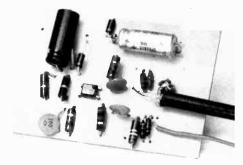
Fig. 1 – The solid-state T-R switch constructed on an etched circuit board of the pattern shown in QST for April, 1971, p. 32. The circuit could also be built on a piece of insulated or perforated board.
