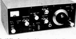
Fig. 10-33 – Front view of the cw transceiver. The chassis and cabinet are homemade, and consist of two U-shaped pieces of thick aluminum stock. The panel is painted dark green to permit the white decal labels to stand out prominently.
