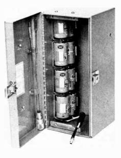
Fig. 10-59 – Eight size D cells are series connected to provide 12 volts. They are mounted in Keystone holders on the back wall of the bond box. The 1/4-inch diameter hole in the front of the cabinet (upper right of photo) permits final calibration of the receiver (C20) after the installation is completed. The hole is opposite the shaft of C20.
