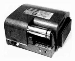
Fig. 15D-1 – Western Union Telefax transceiver. Some machines of this type have been made available to amateurs. The drum accommodates a sheet of paper measuring approximately  $4 1/2 \times 6 1/2$  inches.
