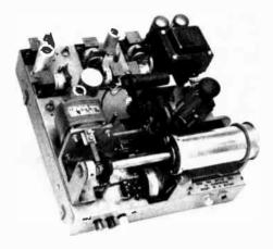
Fig. 15D-2 – The Telefax transceiver with cover removed. The shaft along which the drum traverses is visible at the left of the drum. The photo-optic assembly may be seen on the right-hand side of the chassis, just behind the drum. The lamp and its focusing lens system appear at the right, while the photoelectric cell is housed behind its lens system inside a light shield with appropriate opening.
