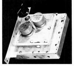
Fig. 7-42 — The 2-tube 1296-MHz amplifier. Two 2C39As are used in this grounded-grid setup. The 'arge square base unit houses the cathode input circuit. The plate cavity is not visible, as it is obscured by the plate-bypass assembly seen here. (Built by W6IOM)
