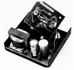
This 250-MHz prescaler uses the Fairchild U6895 H 9059X IC. A power supply and an output amplifier complete the device.
