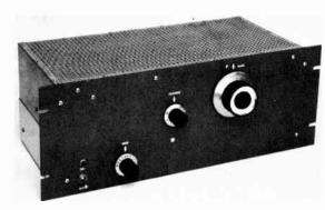
Fig. 7-31 — The 144-MHz amplifier is built in conventional rack-and-panel style, with the entire top of cane metal, to provide free air flow. Controls are grid-circuit tuning, C2, lower left; output loading capacitor, C5, center; and plate-circuit tuning, C4, with vernier dial, right. The slotted end of the Teflon shaft on C1 is visible as a white spot just below the loading control.
