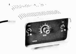
Fig. 13-23 — Front view of the rf speech clipper. The unit is built in an LMB CO-3 cabinet.
