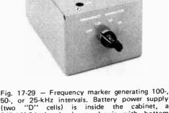
50-, or 25-kHz intervals. Battery power supply (two "D" cells) is inside the cabinet, a 3 X 4 X 6-inch aluminum chassis with bottom plate. The trimmer capacitor for fine adjustment of frequency is available through the hole in the top near the left front.
