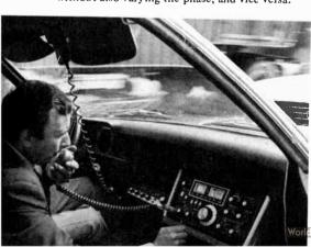
Fig. 14-1 — The use of vhf fm mobile rigs in conjunction with repeaters has improved the communications of many amateur emergency groups. Here F2BQ relays traffic being received via 2-meter fm on a 40-meter ssb link.
