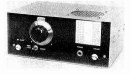
Fig. 8-52 — Front view of the direct-conversion receiver. The panel is finished in machine gray spray paint. The two controls are main tuning and audio gain.
