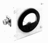
Fig. 17-10 – Rf ammeter mounted in a Minibox, with connectors for placing the meter in series with a coaxial line. A bakelite-case meter should be used to minimize shunt capacitance (which introduces error) although a metal-case meter can be used if mounted on bakelite sheet with a large cut-out in the case around the rim. The meter can be used for rf power measurements ( $P = 1^2R$ ) when connected between a transmitter and a nonreactive load of known resistance.
