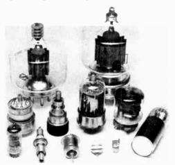
Transmitting tubes are in the back and center rows. Receiving tubes are in the front row (I. to r.): miniature, pencil, planar triode (two), Nuvistor and 1-inch diameter cathode-ray tube.
