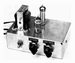
Fig. 11-11 — The single-tube keyer, housed in a  $4 \times 6 \times 2$ -inch aluminum chassis. Power switch, speed and weight controls are mounted along the front apron. On top are the power transformer, the 12AU7 and OB2 regulator.
