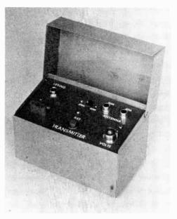
Fig. 1 – This version of the solid-state transmitter is housed in a small recipe box. All controls and jacks are accessible from the top panel.
