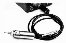
Fig. 17-56 – Rf probe for use with an electronic voltmeter. The case of the probe is constructed from a 7-pin ceramic tube socket and a 2 1/4-inch tube shield. A half-inch grommet at the top of the tube shield prevents the output lead from chafing. A flexible copper-braid grounding lead and alligator clip provide a low-inductance return path from the test circuit.
