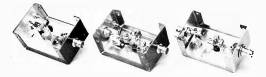
Fig. 9-22 – Interiors of the FET preamplifiers, in the same order as in Fig. 9-20. The input end is toward the right in each unit.
