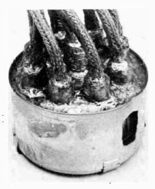
Fig. 10-4 — A close-up view of the distributor shield can. The shield braid over each spark-plug wire is soldered to the top of the can, and the can is grownded to the engine block.
