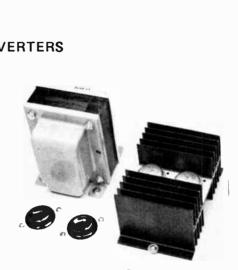
Fig. 10-29 - Top view of the dc-to-ac inverter. The transistors and their heat sink are at the right. Two ac outlets are used, offering greater convenience than would be possible with a single receptacle. A neon lamp lights when the unit is operation.
