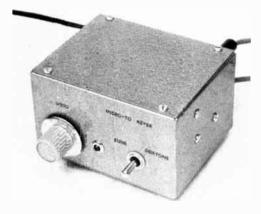
This Micro-TO keyer circuit is a modern version of a keyer that was invented by W9TO. It is compact; inexpensive to build (under 25), and easy to construct. It employs both integrated circuits (ICs) and bipolar transistors. The complete package measures  $4 \times 5 \times 6$  inches.
