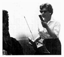
Fig. 10-1 — Effective portable operation can be realized when using lofty locations for vhf or uhf. Here, W1CKK is shown operating a battery-powered, 150-mW output, 2-meter transceiver. With only a quarter wavelength antenna it is possible to communicate with stations 25 miles or more away. Low-power transistor equipment like this unit will operate many hours from a dry-cell battery pack.
