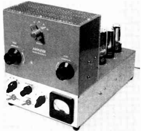
Fig. 6-49—Front view of the 6146 all-purpose amplifier. The upper panel is part of an 8 × 6 × 3½-inch Minibox (Bud CU-2109); the ventilated shielding of Reynolds Aluminum cane metal is fastened to the Minibox and base with sheet-metal screws.
