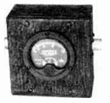
Fig. 21-25—R.f. ammeter mounted for connecting into a coaxial line for measuring power. A "2-inch" instrument will fit into a 2 \times 4 \times 4 metal box.
