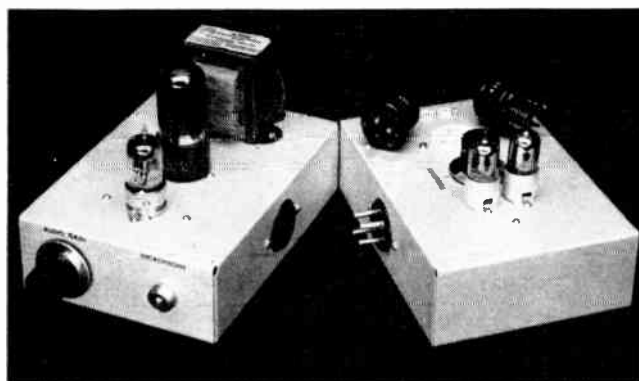
Fig. 17-26—The simple transmitter for 220 and 420 Mc. is made in two parts. The modulator, left, may be retained for use with more advanced r.f. sections than the simple oscillator shown on the right. The two units may be plugged together or connected by cable.
