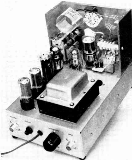
Fig. 6-50—Rear view of the 90-watt all-purpose amplifier with the cane-metal cover removed. One voltage-regulator tube has been removed from its socket (right edge of transformer) to allow the neutralizing capacitor and plate blocking capacitor to be seen. The plate r.f. choke ( RFC_3 in Fig. 6-51) is mounted on one side wall, and the load capacitor and safety choke ( C_4 and RFC_1 in Fig. 6-51) are mounted on the far side wall.
