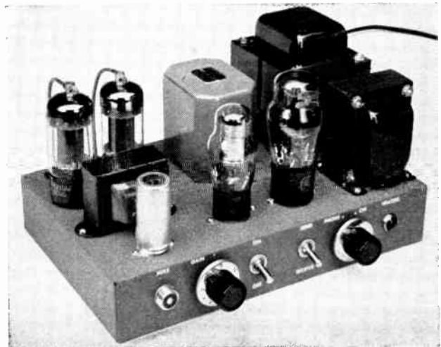
Fig. 9-17—A modulator for transmitters operating at plate inputs up to 50 watts. The speech amplifier and modulator are at the left in this view; power supply components are on the right. The chassis is 7 × 11 × 2 inches.
