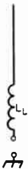
Fig. 19-30—The capacitive reactance at frequencies lower than the resonant frequency of the whip can be canceled out by adding an equivalent inductive reactance in the form of a loading coil in series with the antenna.
