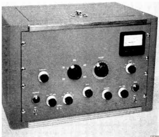
Fig. 6-55—A 500-watt transmitter. Power supplies and a differential keyer are included. It operates with the external v.f.o. tuner shown in Fig. 6-59. Controls along the bottom, from left to right, are for low-voltage power, v.f.o./crystals/s.s.b. switch, driver tank switch, driver tank capacitor, final loading, v.f.o. set switch, and high-voltage. Above, from left to right, are controls for excitation, final tank switch, final tank capacitor and meter switch. The band-switch pointer is made by cutting down the metal skirt of a dial similar to the one to the right.
