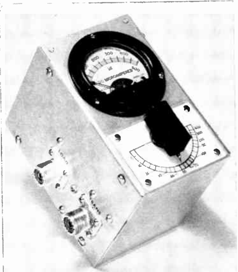
Fig. 21-45—An RC bridge for measuring unknown values of impedance. The bridge operates at an r.f. input voltage level of about 5 volts. The aluminum box is 3 by 4 by 5 inches.
