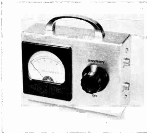
Fig. 19-40—A front view of the field-strength meter. Sensitivity control R_1 is to the right of the 0-1 indicating meter. Antenna input and output connectors are mounted on the right end of the box.
