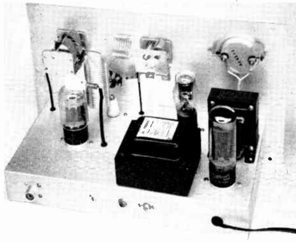
Fig. 6-37—Rear view of the transmitter showing the placement of components above chassis. The loading capacitor, C_5 , is at the left, L_3 is the vertical coil and L_2 the horizontal one. Rubber grommets are used to prevent chafing and to furnish additional insulation on the leads coming from below chassis.
