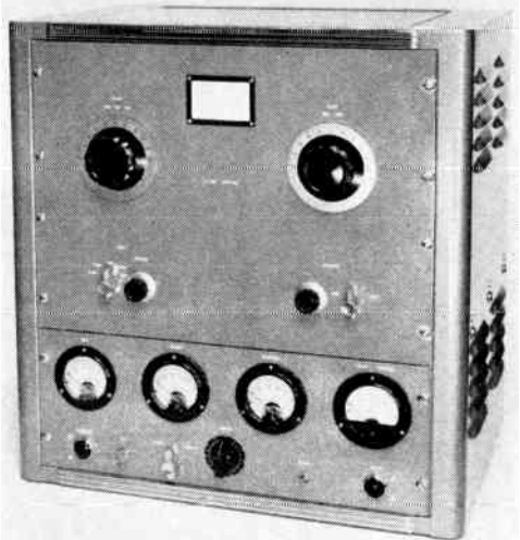
Fig. 6-78—The kilowatt 4-400A amplifier and its control unit are mounted in a 21-inch gray hammertone rack cabinet (Bud CR-1727). Shelf brackets (Bud SA-1350) are mounted on both sides of the cabinet to hold the amplifier chassis. Below the meters, from left to right: filament pilot light, key-type a.c. switch, Class AB 1 /C bias switch, screen autotransformer, plate switch and plate pilot light.
