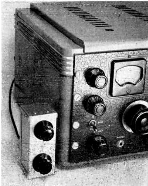
Fig. 5-62—View of the Q multiplier showing its single connecting cable to the receiver. The box can be placed in any convenient spot on or around the receiver.
