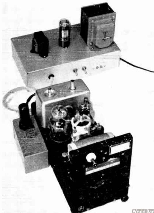
Fig. 6-90—The complete Novice setup, in this case using the 80-meter (BC-696) transmitter. Note the key jack at the lower-left corner of the transmitter panel. The crystal oscillator is connected to the transmitter oscillator-tube socket with a short length of cable terminating in an octal plug. A small notch should be cut in the transmitter cover to provide clearance for the cable when the cover is installed.
