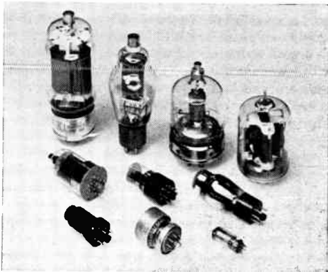
Representative tube types. Transmitting tubes having up to 500-watt capability are shown in the back row. The tube with the tap cap in the middle row is a low-power transmitting type. Others are receiving tubes, with the exception of the one in the center foreground which is a v.h.f. transmitting type.
