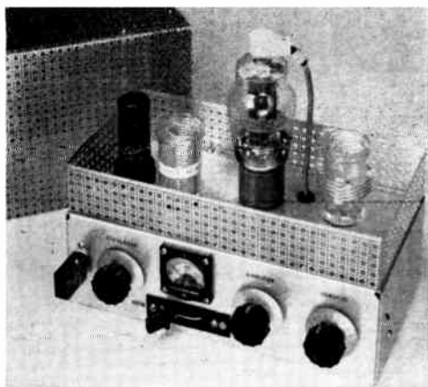
Fig. 6-41—The amplifier tuning and loading controls are to the right of the meter and meter switch. This view of the r.f. unit shows the construction of the "fence" around the top of the chassis. The cover, also made from perforated aluminum, is visible at the rear. The 6AG7 oscillator tube is at the left on the chassis with its plate coil beside it. The amplifier tank coil is at the right. The crystal socket is a Millen 33102 and the dials are Johnson type 116-222.
