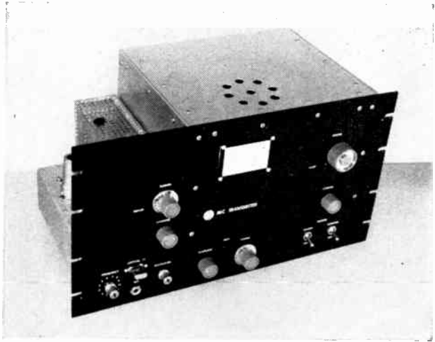
Fig. 17-2—The 50-Mc. r.f. unit. Exciter, left portion on the assembly, also serves on 144 Mc. Amplifier utilizes a 4-125A, 4-250A or 4-400A.
