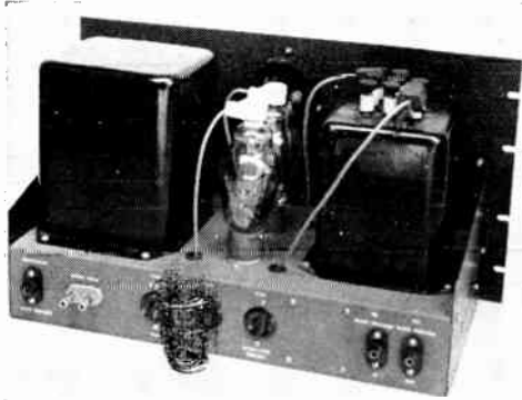
Fig. 9-26—A typical Class B modulator arrangement. This unit uses a pair of 811As, capable of an audio power output of 340 watts, and includes a splatter filter. The modulation transformer is at the left and the splatter choke at the right. All high-voltage terminals are covered so they cannot be touched accidentally.
