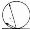
Fig. 14-6—Illustrating the importance of vertical angle of radiation in determining antenna directional effects. Off the end, the radiation is greater at higher angles. Ground reflection is neglected in this drawing of the free-space pattern of a horizontal antenna.
