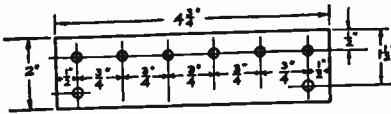
NOTE - Size of drill to agree with type of binding past used.
