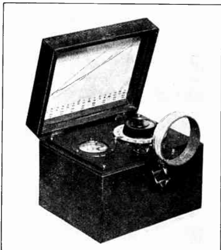
THE PICK-UP LAMP TO BE PROVIDED WHEN A WAVEMETER HAS NO RESONANCE INDICATOR
