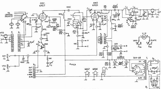
Fig. 6-44—Circuit diagram of the 75-watt 6DQ5 transmitter. Unless specified otherwise, capacitance is in picofarads (pf. or  $\mu\mu$ f.), resistance is in ohms, resistors are  $\frac{1}{2}$  watt.
