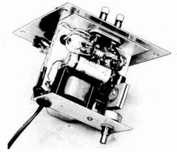
Fig. 21-20—Bottom view of the audio oscillator, showing the power-supply components and amplitude-control lamp, I<sub>1</sub>. The lamp is mounted by wires soldered to its base. The selenium rectifier is supported by a tie-point strip. Placement of resistors, which are hidden by the other components, is not critical. The unit fits in a 4 × 5 × 6 inch box.
