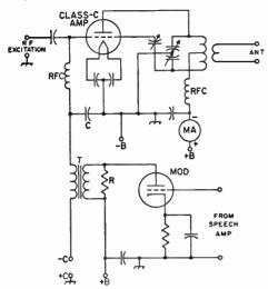
Fig. 10-14—Contral-grid modulation of a Class C amplifier. The r.f. grid bypass capacitar, C, should have high reactance at audia frequencies (0.005 μf.
