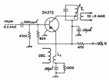
Fig. 5-13—Typical transistor mixer circuit. L1-Low-impedance inductive coupling to oscillator. T<sub>1</sub>-Transistor i.f. transformer. Primary impedance of 50,000 ohms, secondary impedance of 800 ohms (Miller 2066).
