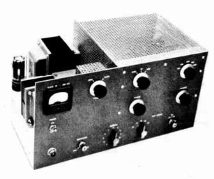
Fig. 6-43—This 75-watt crystal-cantrolled transmitter has provision for the addition of v.f.o. cantrol. A 6AG7 oscillator drives a 6DQ5 amplifier on 80 through 15 meters.
