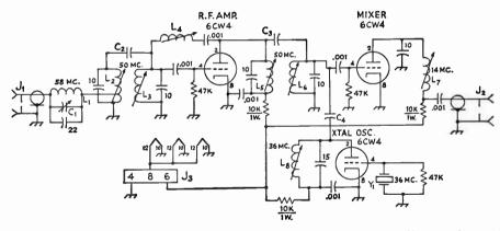
Fig. 16-9—Schematic diagram and parts information for the 50-Mc. converter. Resistors  $\frac{1}{2}$  watt unless specified. Fixed capacitors are ceramic; decimal values in  $\mu$ f., others in  $\mu$  $\mu$ f.
