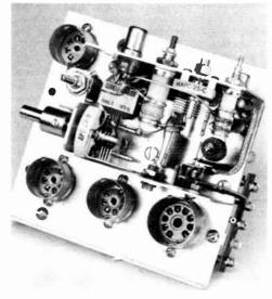
Fig. 19-22—The v.f.o. section is built in the U-shaped portion of a  $31/4 \times 21/6 \times 11\%$ -inch Minibox (Bud CU-2101-A) mounted on a sheet of aluminum; the other half of the Minibox serves as the cover. The Nuvistor socket and the oscillator coils are mounted on one side of the Minibox. Jack  $J_1$  is mounted on the other side of the Minibox and is visible between the two right-hand tube sockets.
