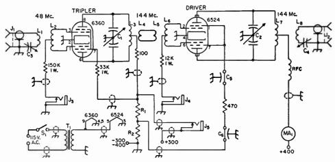
Fig. 17-25—Schematic diagram of the tripler and driver stages of the high-powered 2-meter transmitter.
