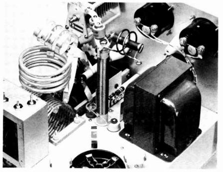
Fig. 6-83—Another of the VIAW grounded-grid amplifier, showing the output voltmeter (shield cover removed) components mounted on a multiple tie point strip. The cone insulator between the meters receives the screw that holds down the meter shield (chassis).
