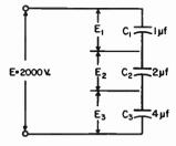
Fig. 2-11—An example of capacitors connected in series.
