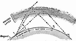
Fig. 15-4—Refraction of sky waves, shawing the critical wave angle and the skip zane. Waves leaving the transmitter at angles above the critical (greater than A) are not bent enough to be returned to earth. As the angle is decreased, the waves return to earth at increasingly greater distances.
