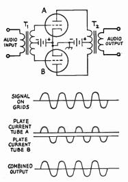
Fig. 3-13—Class B amplifier operation.
