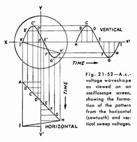
For many amateur purposes a satisfactory horizontal sweep is simply a 60-cycle voltage of adjustable amplitude. In modulation monitoring (described in the chapter on amplitude modulation) audio-frequency voltage can be taken from the modulator to supply the horizontal sweep. For examination of audio-frequency wave forms, the linear sweep is essential. Its frequency should be adjustable over the entire range of audio frequencies to be inspected on the oscilloscope.
