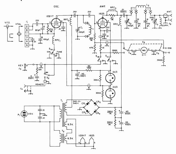
Fig. 6-40—Circuit diagram of the inexpensive 75-watt transmitter. Unless indicated otherwise, all resistors are ½-watt, all resistances are in ohms, all capacitances are in μf. Electrolytic capacitors are marked with polarity, mica capacitors are marked with \*, other fixed capacitors under 0.1 μf. are ceramic.
