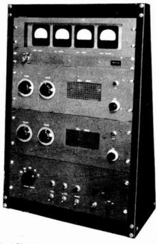
Fig. 6-73—Individual kilowatt amplifiers for two bands plus complete metering and all control circuits and power supplies (except plate) fit handily into a table rack. Amplifiers for five bands plus the plate supply will mount in floor rack. Band switch at lower left (S<sub>8</sub> in Fig. 6-74) switches filament supply, excitation and output connections to all amplifiers in use; screen and plate supplies are connected to all amplifiers at all times.
