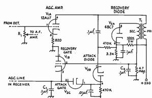
Fig. 5-18—Audio "hang" a.g.c. system. Resistors are ½ watt unless specified otherwise. R<sub>1</sub>—Normal audio volume control in re-
