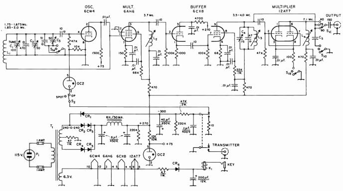
Fig. 6-89—Circuit diagram of the two-band v.f.o. Unless otherwise specified, all capacitances are in picofarads (pf. or μμf.), resistances are in ohms, resistors are ½-watt. Capacitors marked with polarity are electrolytic, those marked with asterisk are silver mica.
