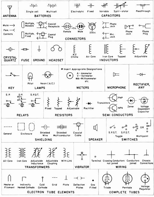
Where it is necessary or desirable to identify the electrodes or capacitors, the curved element represents the *outside* electrode (marked "outside foil," "ground," etc.) in fixed paperand ceramic-dielectric capacitors, and the *negative* electrode in electrolytic capacitors. In variable or adjustable capacitors (regardless
