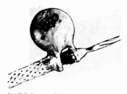
Fig. 23-9—Proper method of bypassing the end of a shielded lead using disk ceramic capacitor. The 0.001μf. size should be used for 1600 volts or less; 500 μμf. at higher voltages. The leads are wrapped around the inner and outer conductors and soldered, so that the lead length is negligible. This photograph is about four times actual size.
