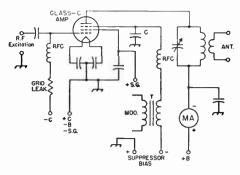
Fig. 10-13—Suppressor-grid modulation of an r.f. amplifier using a pentode-type tube. The suppressorgrid r.f. bypass capacitor, C, should be the same as the grid bypass capacitor in control-grid modulation.
