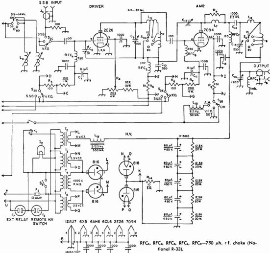
$L_{10}$ —7-hy. 150-ma. filter choke (Stancor C-1710).  $L_{11}$ —15-hy. 75-ma. filter choke (Stancor C-1002).  $L_{12}$ —5/25-hy. 300-ma. swinging filter choke (Triad C-33A).
