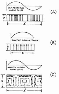
Fig. 2-63—Field distribution in a rectangular waveguide. The TE<sub>2-0</sub> mode of propagation is depicted.
