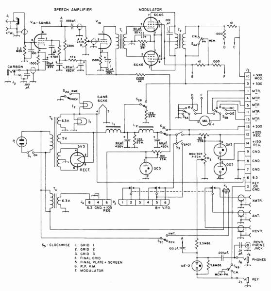
Fig. 17-14—Circuit diagram of the power supply, modulator and control unit. Unless specified otherwise, resistances are in ohms, resistors are ½ watt, capacitors marked with polarity are electrolytic.
