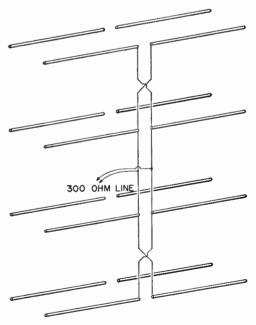
Fig. 18-15—Schematic drawing of a 16-element array.
