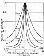
Fig. 2-39—Current in series-resonant circuits having different Qs. In this graph the current at resonance is assumed to be the same in all cases. The lower the Q, the more slowly the current decreases as the applied frequency is moved away from resonance.
