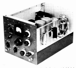
above a small CAL control knob that sets the signal level into the receiver when the function switch (left, below VXO control) is on "calibrate." Small knob at lower left is sideband-selector switch. Switch to left of meter switches meter to grid or cathode of output tube or to r.f. voltmeter on output line; knob just below adjusts sensitivity of r.f. voltmeter.
