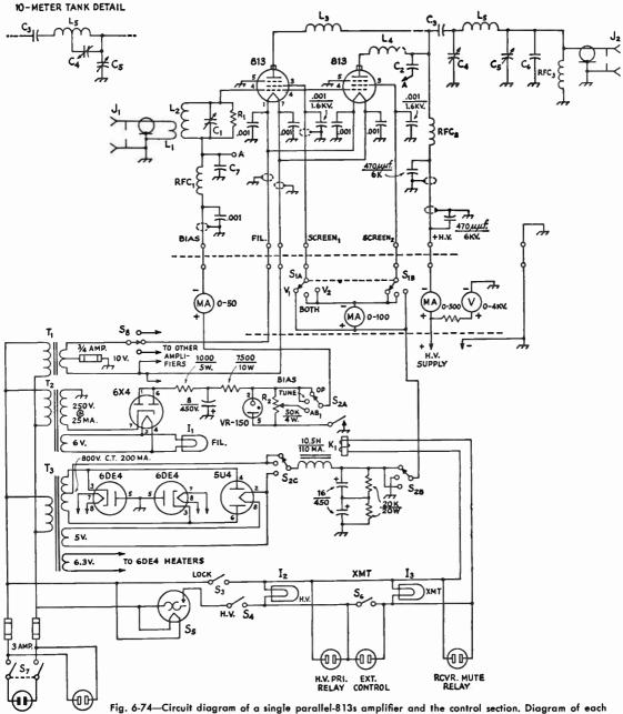
amplifier is similar, except as noted belaw. Unless specified otherwise, capacitances are in  $\mu$ f., capacitars marked with palarity are electralytic, fixed capacitors are ceramic, resistances are in ahms.
