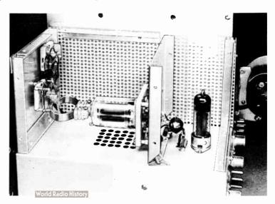
The final chassis is aluminum, 10 by 12 by 3 inches, matching up with the driver chassis to fit into a standard 10½-inch rack panel. Complete enclosure is a must for TVI prevention, and it pays dividends in improved stability by providing effective isolation of circuits that tend to give trouble in open layouts.
