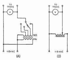
Fig. 7-33—Two methods of transformer primary control.
