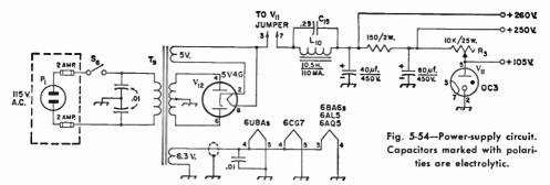
C<sub>18</sub>—0.25-µf. paper, 600 volts. L<sub>10</sub>—Filter choke, 10.5 henry, 110 ma. (Knight 62 G 139). P<sub>1</sub>—Fuse plug.
