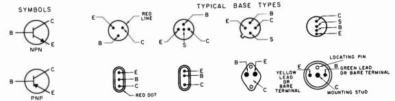
Code for identifying typical junction transistors. The leads are marked C-collector, B-base, E-emitter and S-interlead shield and metal case.
