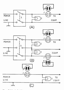
Fig. 7-35—Reliable arrangements for cutting aff all power to the transmitter. S is an enclosed double-pole knife-type switch, J a standard a.c. outlet. P a shorted plug to fit the outlet and I a red lamp.
