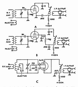
Fig. 16-5—Typical v.h.f. mixer circuits for triode (A), pentode (B) and push-push triode (C). Circuits A ond B may be used with one portion of various dual-purpose tubes, Plate current of pentode (B) should be held at lowest usable value if no r.f. stage is used.
