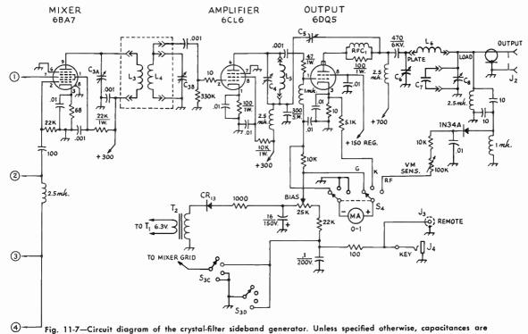
in  $\mu\mu$ f., decimal capacitances are in  $\mu$ f., resistors are  $\frac{1}{2}$  watt, resistances are in ohms. Copacitors marked with polarity are electrolytic.
