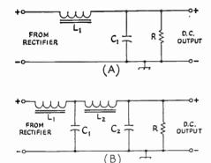
Fig. 7-10—Choke-input filter circuits. A—Single-section.
