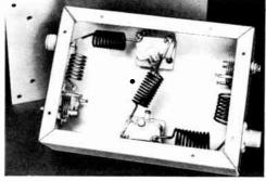
Fig. 23-23—Low-pass filter using variable air capacitors. The box is a 2 by 5 by 7 aluminum chassis, fitted with a bottom plate of similar construction to the one used in Fig. 23-21.
