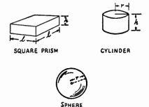
Fig. 2-64—Forms of cavity resonators.
