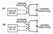
Fig. 21-36—Setups for measuring inductance and capacitance with the grid-dip meter.
