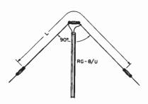
Fig. 14-13—The inverted V antenna is a dipole with the ends lower than the center. It is convenient to use because it requires only one high support, which also supports the weight of the coaxial transmission line. Shown here in its simplest form, with a glass insulator in the center, a deluxe version can be made with a waterproof fitting (Cesco Dri-Fit).
