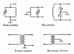
Fig. 2-59—Single-ended and balanced circuits.
