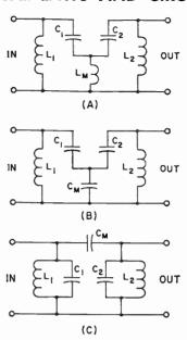
Fig. 2-46—Three methods of circuit coupling.
