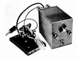
Fig. 8-12—This electrronic speed key has a range of approximately 8 to 35 w.p.m., set by the speed control at top center. It has relay output and can be used with any transmitter that can be keyed by a hand key. The key (left) is made from two telegraph keys and a pair of 1/2-inch thick sheet plastic paddles.
