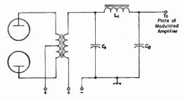
Fig. 9-13—Splatter-suppression filter for use at high level, shown here connected between a Class B modulator and plate-modulated r.f. amplifier. Values for  $L_1$ ,  $C_1$  and  $C_2$  are determined as described in the text.
