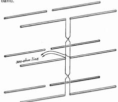
Fig. 18-14—Element arrangement and feed system of the 12-element array. Reflectors are spaced 0.15 wavelength behind the driven elements.
