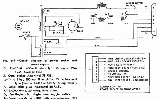
T<sub>2</sub>--Filament transformer, 6.3 volts, 3 amp. (Triad F-16X, Knight 62-G-031, or equivalent).
