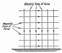
Fig. 15-1—Representation of electric and magnetic lines of farce in a radia wave. Arraws indicate instantaneous directions of the fields far a wave traveling toward the reader. Reversing the direction of one set of lines would reverse the direction of travel.
