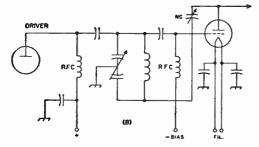
Fig. 6-25—When a pi-network output circuit is used with a triode, a balanced grid circuit must be provided for neutralizing. A—Inductive-link input, B—Capacitive input coupling.
