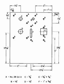
Fig. 16-22—Location of holes on the panel. The panel is part of a  $4 \times 5 \times 6$ -inch Minibox (Bud CU-3007A). The square hole, E, takes the 4-pin connector (Cinch-Jones S-304-AB) used to connect the handset to the transceiver.
