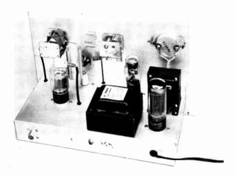
Fig. 6-37—Rear view of the transmitter showing the placement of components above chassis. The loading capacitor,  $C_8$ , is at the left,  $L_8$  is the vertical coil and  $L_2$  the horizontal one. Rubber grommets are used to prevent chafing and to furnish additional insulation on the leads coming from below chassis.
