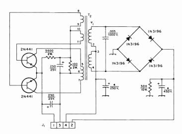
Fig. 19-20—Circuit diagram of the power supply. Capacitances are in μf., resistances are in ohms.
