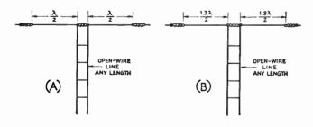
Fig. 14-29—Collinear antennas in phase. The system at A is known as "two half waves in phase" and has a gain of 1.8 db. over a half-wave antenna. By lengthening the antenna slightly, as in B, the gain can be increased to 3 db. Maximum radiation is at right angles to the antenna. The antenna at A is sometimes called a "double Zepp" antenna, and that at B is known as an "extended double Zepp."
