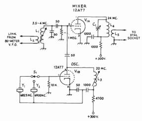
L<sub>2</sub>—12 turns Na. 32 enam.,  $3_{16}$  inch long on %-inch iron-slug form, approx 5  $\mu$ h.
