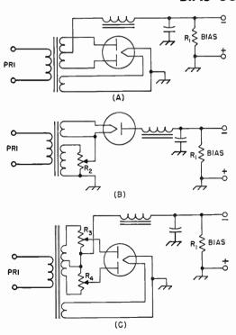
As discussed in Chapter 6 on high-frequency transmitters, the chief function of a bias supply for the r.f. stages of a transmitter is that of providing protective bias, although under certain circumstances, a bias supply, or pack, as it is sometimes called, can provide the operating bias if desired.
