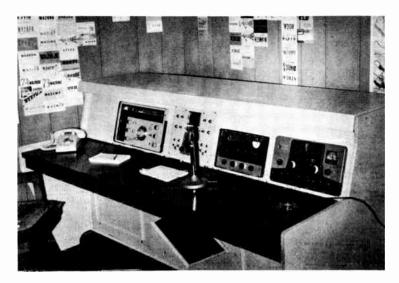
This homemade console, built of plywood and finished with light tan speckled spray paint, effectively conceals all power and antenna leads. The top of the console lifts off for access to the equipment.
