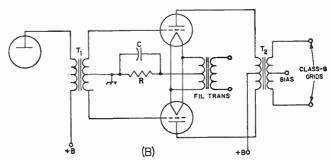
Fig. 9-7—Triode driver circuits for Class B modulators. A, resistance coupling to grids; B, transformer coupling. R<sub>1</sub> in A is the plate resistor for the preceding stage, value determined by the type of tube and operating conditions as given in Table 9-1. C- and R<sub>2</sub> are the coupling capacitor and grid resistor, respectively; values also may be taken from Table 9-1.
