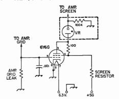
Fig. 6-18—Screen clomper circuit for protecting screen-grid power tubes. The VR tube is needed only for complete screen-voltage cut-off.
