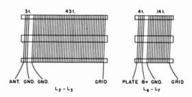
Fig. 5-38—Details of the coil construction. Each one is made from B & W 3012 Miniductor or Illumitronic 632 stock, which is wound 32 t.p.i. and %-inch diameter. The separation between  $L_2$  and  $L_3$  is 1 turn; the separation between  $L_6$  and  $L_7$  is 1 turn.  $L_6$  is 43 turns of the same stock.
