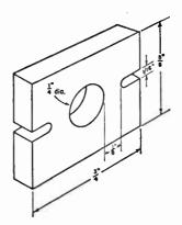
Fig. 13-20—Dimensions of the insulating spacers used to hold the pick-up wires in place in the Monimatch.
