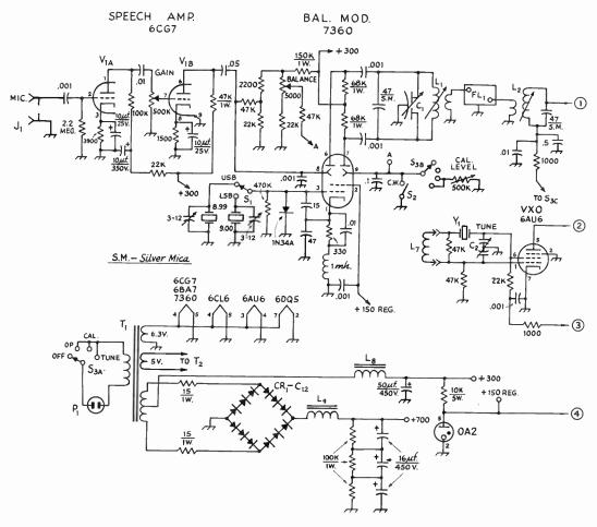
determination of the coupling is a job for an impedance bridge, it is suggested that the builder use the coil specified for  $L_2$  unless he has facilities for designing his own.
