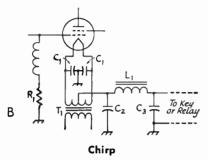
The frequency-stability reference in the opening paragraph refers to the "chirp" observed on many signals. This is caused by a change in frequency of the signal during a single dot or dash.
