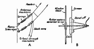
dow sash, as shown in Fig. 14-51, or by using weatherstrip material where necessary.
