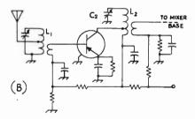
Fig. 5-27—Transistor r.f. amplifier circuit. The low-impedance connections to the base and collector can be (A) taps on the inductors or (B) low-impedance coupling links. L<sub>1</sub>C<sub>1</sub>, L<sub>2</sub>C<sub>2</sub>—Resonant at signal frequency.
