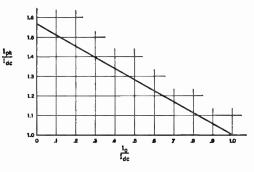
Fig. 11-21—When the two-tone test signal is used for checking the linearity of an amplifier, the peak current is higher than the current indicated by the plate meter. The ratio of these values depends upon the ratio of the idling (no-signal) current to the indicated current.
