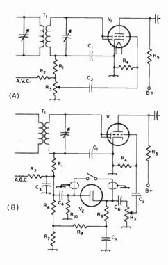
Fig. 19-3—Diagrams showing addition of noise limiter to car receiver. A—Usual circuit, 8—Modification.
