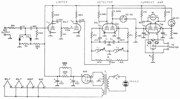
Fig. 12-12—Receiving converter for f.s.k. teletype signals (W2PAT). Unless otherwise indicated, capacitances are in μf. resistances are in ohms, resistors are ½ watt. Capacitors of 0.01 μf. or less may be mica or ceramic; larger values may be paper. Capacitors with polarities indicated are electrolytic.
