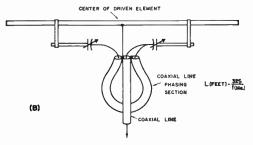
Fig. 14-37—The most popular methods of feeding the driven element of a beam antenna are (A) the gamma match and (B) the T match. The aluminum tubing or rod used for the matching section is usually of smaller diameter than the antenna element; its length will vary somewhat with the spacing and number of elements in the beam. The coaxial line in the phasing section can be cailed in a 2- or 3-foot diameter coil instead of hanging as shown.
