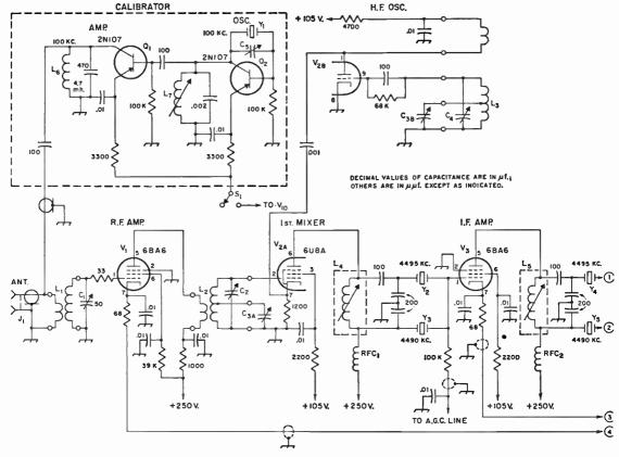
Fig. 5-52—Front-end circuit of the receiver. Unless otherwise specified, resistars are ½ watt; 0.01 and 0.02-μf. capacitors are disk ceramic, 600 volts; 0.5 capacitors are tubular paper or Mylar; capacitars below 0.01 μf. are mica; capacitors marked with polarities are electrolytic.
