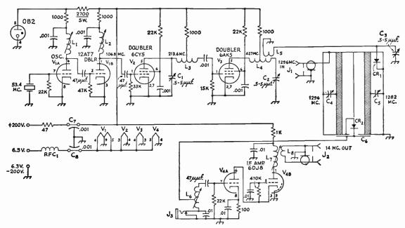
Fig. 16-28—Circuit diagram and parts information for the 1296-Mc. converter. Decimal values of capacitors are in  $\mu f$ .
