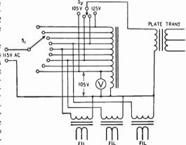
Fig. 7-34—With this circuit, a single adjustment of the tap switch  $S_1$  places the correct primary voltage on all transformers in the transmitter.
