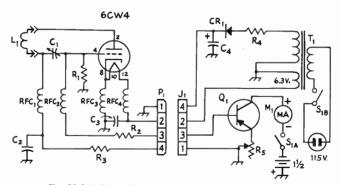
Fig. 21-18—Circuit diagram of the u.h.f. grid-dip meter.
