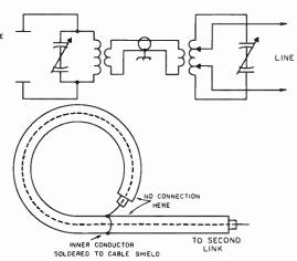
Fig. 23-19—Shielded coupling coil constructed from coaxial cable. The smaller sizes of cable such as RG-59/U are mast convenient when the coil diameter is 3 inches or less, because af greater flexibility. Far larger coils RG-8/U or RG-11/U can be used.
