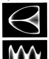
Fig. 10-22—Upper photo—Audio phose shift in coupling circuit between transmitter and harizantal deflection plotes. Lower photo—Hum on vertical deflection plotes.
