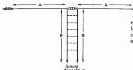
Fig. 14-19—Practical arrangement of a shortened antenna. When the total length, A+B+B+A, is the same as the antenna length plus twice the feeder length of the center-fed antennas of Table 14-I, the same type of coupling circuit will be used. When the feeder length or antenna length, or both, makes the sum different, the type of coupling circuit may be different but the effectiveness of the antenna is not changed, unless A+A is less than a quarter wavelenath.
