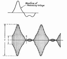
Fig. 10-2—Modulation by an unsymmetrical wave form. This drawing shows 100% downward modulation along with 300% upward madulation. There is no distartian, since the modulation envelape is an accurate reproduction of the wave form of the modulating voltage.
