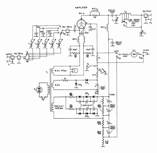
Fig. 6-54—Circuit diagram of the 200-watt grounded-grid linear amplifier. Unless specified, all capacitances are in picofarads (pf. or μμf.), all resistors are ½ watt, all resistances are in ohms. Capacitors marked with polarity are electrolytic; 0.01-μf. capacitors are 1200-volt disk ceramic.
