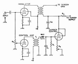
Fig. 10-12—Circuit for carrier control with screen madulation. A small triode such as the 6C4 can be used as the control amplifier and a 6Y6G is suitable as a carrier-control tube,  $T_1$  is an interstage audio transformer having a 1-to-1 or larger turns ratio,  $R_4$  is a 0.5-megohm volume control and also serves as the grid resistor for the modulator. A germanium crystal may be used as the rectifier. Other volues are discussed in the text.
