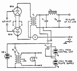
Fig. 9-27—Circuit diagram of the Class B modulator. C<sub>1</sub>, C<sub>2</sub>, L<sub>1</sub>—See text. ( $L_1$  is Chicago Transformer type SR-300).
