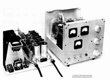
Fig. 6-78—The 3-1000Z grounded-grld linear is mounted on short legs to allow air to be drawn in at the bottom and blown up past the tube. The meters indicate grid (left) and plate current and relative output (below). Knobs at right (B & W 901) control plate (top), band switching and loading.
