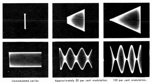
Fig. 10-20—Oscilloscope patterns showing praper modulation of a plate-and-screen modulated tetrode r.f. amplifier. Upper row, trapezoidal patterns; lower row, corresponding wave-envelope patterns. In the latter a linear sweep having a frequency one-third that of the sine-wave audio modulating frequency was used, so that three cycles of the modulation envelope show in the pattern.
