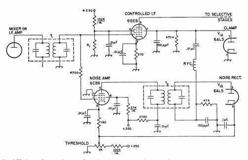
Fig. 5-22—Practical circuit diagram of an i.f. noise silencer. For best results the silencer should be used ahead of the high-selectivity portion of the receiver. T<sub>1</sub>—Interstage i.f. transformer
