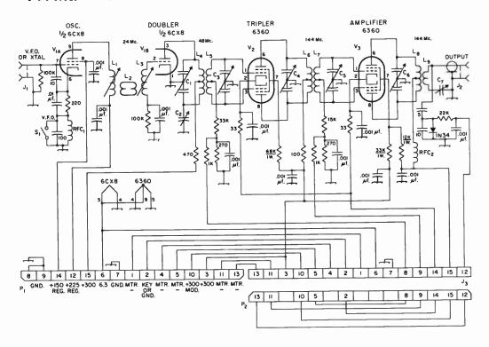
Fig. 17-7—Circuit diagram of the 144-Mc. transmitter. Unless specified otherwise, capacitances are in picofarads (pf. or  $\mu\mu$ f.), resistances are in ohms, resistors are  $\frac{1}{2}$  watt.  $P_2$  plugs into  $J_3$  for 144-Mc. operation.
