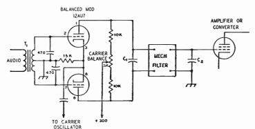
Fig. 11-4—One type of balanced-modulator circuit that can be used with a mechanical filter (Collins F455-31 or F500-31 series) in the i.f. range. The filters are furnished in various types of mountings, and the volues of C<sub>1</sub> and C<sub>2</sub> will depend upon the type of filter selected.
