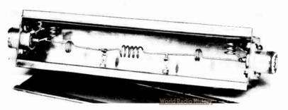
Fig. 23-26—A 52-ohm law-pass filter for 144-Mc. Transmitters. Case is made from flashing copper and is 1½ inches square by 7½ inches long. Cover slips on flanges falded out at the bottam; ends are folded down and soldered.
