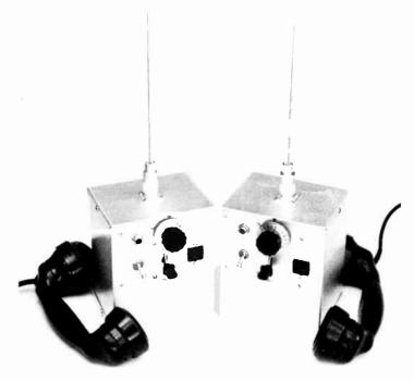
Fig. 16-17—This pair of 420-Mc. transceivers will be all ready to go as soon as the handset connectors are plugged in the panel sockets. Each handful is a complete station, built around the 6CW4 Nuvistor and a pair of transistors.
