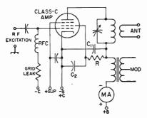
Fig. 10-6—Plate and screen modulation of a Class C r.f. amplifier using a screen-grid tube. The plate r.f. bypass capacitor, C<sub>1</sub>, should have reasonably high reactance at all audio frequencies; a value of 0.001 to 0.005  $\mu$ f. is generally satisfactory. The screen bypass, C<sub>2</sub>, should not exceed 0.002  $\mu$ f. in the usual rate
