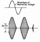
Fig. 10-3—An overmodulated signal. The madulation envelope is not an accurate reproduction of the wave form of the modulating voltage. This or any type of distortion occurring during the modulation process generates spurious sidebands or "splatter."
