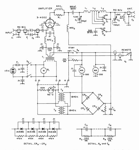
Fig. 6-64—Circuit diagram of the 900-watt p.e.p. grounded-grid amplifier. Unless specified otherwise, capacitances are in μf., resistances are in ohms, resistors are ½ watt.
