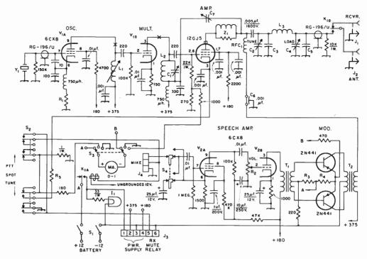
Fig. 19-16—Circuit diagram of the 40-watt "extended-band" mobile transmitter. Unless noted otherwise, resisttances are in ohms, resistors are ½ watt, capacitances are in picofarads.
