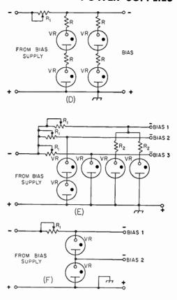
Each VR tube will handle 40 ma. of grid current. If the grid current exceeds this value under any condition, similar VR tubes should be added in parallel, as shown in Fig. 7-29B, for each 40 ma., or less, of additional grid current. The resistors  $R_2$  are for the purpose of helping to maintain equal currents through each VR tube, and should have a value of 50 to 1000 ohms or more.
