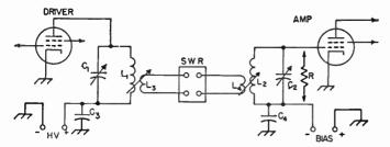
Fig. 6-19—Coupling excitation to the grid af an r.f. power amplifier by means of a low-impedance coaxial line.
