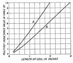
Fig. 2-15—Factor to be applied to the inductance of coils listed in the table below, as a function of coil length.
