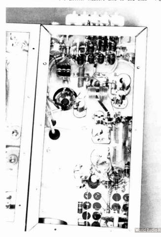
Fig. 17-19—Bottom view of the 50-Mc. exciter, showing bondpass circuits and TVI protective measures.
