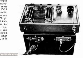
sible to dissipate a large part of the transmitter output in the tuner itself, and for this reason an output indicator is highly desirable, at least for the initial tune-up. Either an r.f. ammeter in the output lead or an r.f. voltmeter from it to chassis will be satisfactory. Under some conditions a neon bulb will serve as an r.f. voltmeter.
