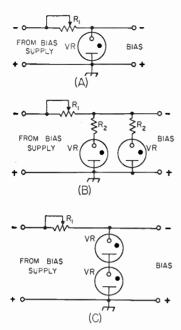
Fig. 7-29—Illustrating the use of VR tubes in stabilizing protective-bias supplies.  $R_1$  is a resistor whose value is adjusted to limit the current through each VR tube to 5 ma. before amplifier excitation is applied. R and  $R_2$  are current-equalizing resistors of 50 to 1000 ohms.
