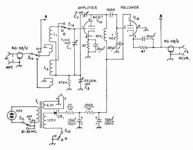
Fig. 5-50—Circuit diagram of the regenerative preselector. Unless otherwise specified, resistors are  $\frac{1}{2}$  watt, capacitors are in  $\mu\mu$ t., capacitors marked in polarity are electrolytic.
