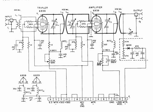
Fig. 17-12—Circuit diagram of the 432-Mc. tripler/amplifier shown in Fig. 17-13. Unless specified otherwise, capacitances are in picofarads, resistances are in ohms, resistors are ½ watt.
