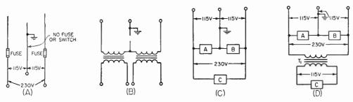
Fig. 7-32—Three-wire power-line circuits. A—Normal 3-wire-line termination. No fuse should be used in the gounded (neutral) line. B—Showing that a switch in the neutral does not remove voltage from either side of the line. C—Connections for both 115- and 230-volt transformers. D—Operating a 115-volt plate transformer from the 230-volt line to avoid light blinking. I<sub>1</sub> is a 2-to-1 step-down transformer.
