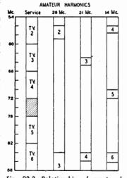
Fig. 23-3—Relotionship of omateur-band harmonics to v.h.f. TV channels. Harmonic interference from transmitters operating below 30 Mc. is most likely to be serious in the low-channel group (54 to 88 Mc.).
