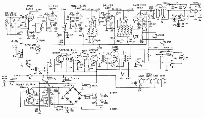
Fig. 19-26—Circuit diagram of the mobile transmitter. Unless specified otherwise, capacitances are in  $\mu\mu$ f., decimal values are in  $\mu$ f., resistances are in ohms, resistors are ½ watt.
