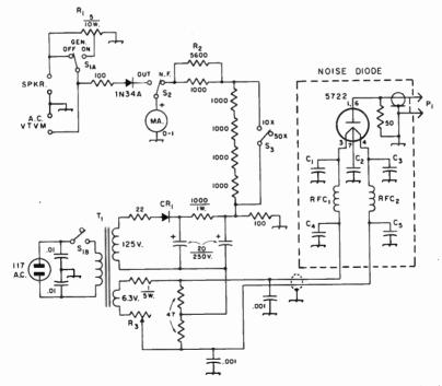
Fig. 21-25—Circuit diagram of the diode noise generators and power supply. Unless indicated otherwise, resistances are in ohms, resistors are ½-watt, capacitances are in μf.
