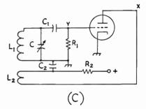
Fig. 5-14—High-frequency oscillator circuits. A, pentode grounded-plate oscillator; B, triode grounded-plate oscillator; C, triode oscillator with tickler circuit. Coupling to the mixer may be taken from points X and Y. In A and B, coupling from Y will reduce pulling effects, but gives less voltage than from X; this type is best adapted to mixer circuits with small oscillator-voltage requirements. Typical values for components are as follows:
