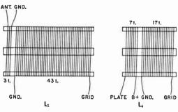
Fig. 5-32—Details of the coil construction. Each one is made from B & W 3012 Miniductor or Illumitronic 632 stock, which is wound 32 t.p.i. and  $\frac{3}{4}$ -inch diameter. The separation between coils in  $L_1$  is  $1\frac{1}{2}$  turns; the separation between coils in  $L_4$  is 1 turn.  $L_5$  is 43 turns of the same stock.
