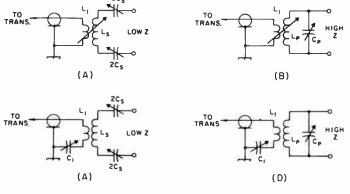
Coupling systems that will deliver power into a flat line are readily designed. For all practical purposes the line can be considered to be flat if the s.w.r. is no greater than about 1.5 to 1. That is, a coupling system designed to work into a pure resistance equal to the line  $Z_0$  will have enough leeway to take care of the small variations in input impedance that will occur when the line length is changed, if the s.w.r. is higher than 1 to 1 but no greater than 1.5 to 1.
