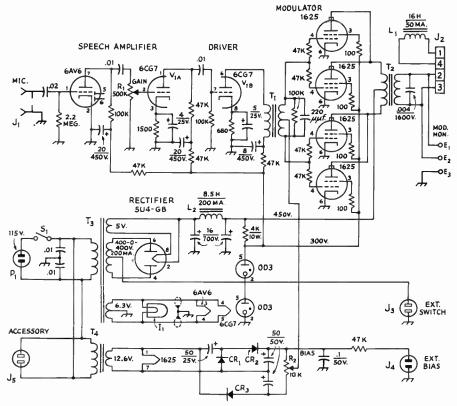
Fig. 9-21—Circuit diagram of the 50-watt modulatar. Unless specified atherwise, capacitances are in  $\mu$ f., resistances are in ahms, resistars are  $\frac{1}{2}$  watt.
