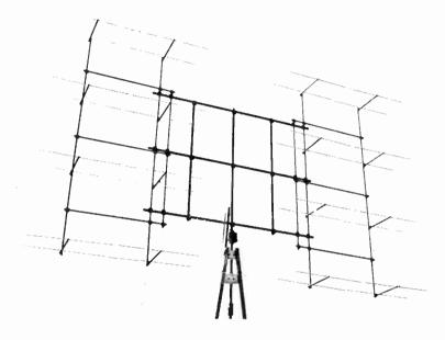
Fig. 18-18—Two 16element arrays spaced % wavelength and fed in phase.
