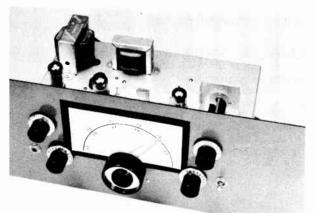
Fig. 5-30—The SimpleX Super receiver uses three dual tubes and a crystal filter to cover the 80- and 40-meter bands, and it can tune to 5 Mc. for copying WWV. The dial scale is made from white paper held to the panel by black tape; the index is clear plastic.
