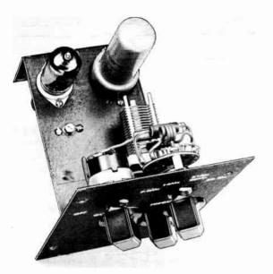
Fig. 21-14—A 100-kc, frequency standard and harmonic amplifier. The crystal in this unit is in the metal-tube type envelope. Pawer and r.f. autput connectians are taken thraugh the rear chassis lip.
