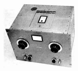
Fig. 6-69—This view of the amplifier shows the bandswitch trap door, air-exhaust port and hole for adjusting neutralization, all in the top of the shielding enclosure. The large knob on the left of the panel is for the 20/15/10-meter plate tuning capacitor, and the matching knob adjusts the capacitor used on 80 and 40. Farther down, from left to right: grid BAND switch, grid TUNING control, variable LOADING adjustment and LOADING switch.
