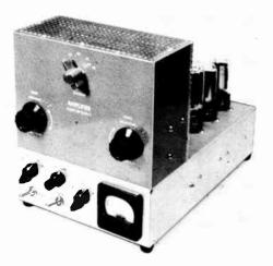
Fig. 6-47—Front view of the 6146 all-purpose amplifier. The upper panel is part of an  $8\times6\times31/2$ -inch Minibax (Bud CU-2109); the ventilated shielding of Reynolds Aluminium cane metal is fastened to the Minibox and base with sheet-metal screws.
