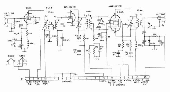
Fig. 17-4—Circuit diagram of the 50-Mc. transmitter. Unless specified otherwise, capacitances are in picofarads (pf. or μμf.), resistances, are in ohms, resistors are ½ watt. Fixed capacitors are ceramic.
