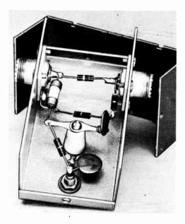
Fig. 21-43—An inexpensive bridge for matching adjustments using the circuit of Fig. 21-42. It is built in a  $1\% \times 2\% \times 4$ -inch "Channel-lock" box. The standard resistor,  $R_3$ , bridges the two coax connectors. A pin jack is provided for connection to the d.c. meter, 0-1 ma. or 0-500  $\mu$ a.; the meter negative can be connected to the case or to one of the coax fittings.
