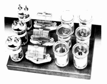
Fig. 11-13—Plug-in coils and r.f. phase-shift networks for the sideband generator. Output tank coils (right) include additional padding capacitor for C<sub>7</sub>, as given in the coil table. Polystyrene coil forms are 4-pin (Allied Radio 24-4P) and 5-pin (Allied Radio 24-5P).
