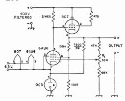
Fig. 7-22—Electronic voltage-regulator circuit. Resistors are ½ watt unless specified otherwise.
