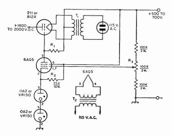
obtained with a regulation better than 1 per cent over a current range of 0 to 100 ma.
