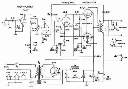
Fig. 9-15—Circuit of the speech amplifier and modulator. All capacitances are in  $\mu f$ .; capacitors with polarities marked are electrolytic, others are ceramic. Resistors are  $\frac{1}{2}$  watt except as nated below. Voltages measured to chassis with v.t. valtmeter.
