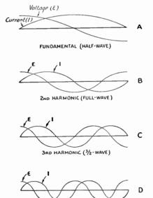
Fig. 14-14—Standing-wave current and voltage distribution along an antenna when it is operated at various harmonics of its fundamental resonant frequency.
