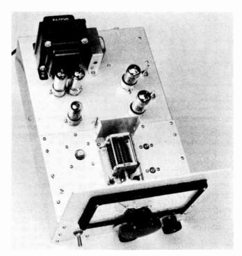
Fig. 6-87—The two-band v.f.o. uses a 6CW4 Nuvistor triode (left front) in the oscillator circuit. In this view the tube shields have been removed from the r.f. tubes (tubes in front of transformer are voltage regulators), and the Minibox cover has been lifted to show the tuning capacitor. The front half of the chassis is reinforced with a plate of ½-inch thick aluminum, to eliminate microphonics.
