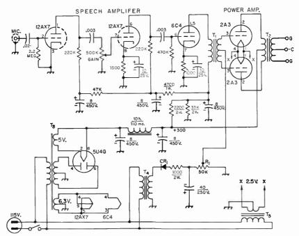
Fig. 9-8—Typical speech-amplifier driver for 10-15 watts output. Capacitances are in #f. Resistors are ½ watt unless specified otherwise. Capacitors with polarity indicated are electrolytic.
