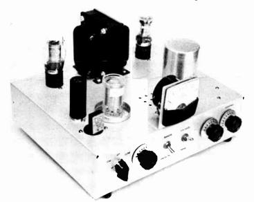
Fig. 6-39—The inexpensive 75-watt transmitter is a two-tube five-band crystal-controlled transmitter; v.f.o. control can be added at any time. To simplify construction and testing, plug-in coils are used, housed in the two shield cans (Millen 80011 or Miller S-42 with S-42C base). The crystal-oscillator tube, a 12BY7, is housed in the black tube shield at the left; the 1625 amplifier tube is mounted under the chassis.
