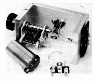
sible to determine the band edges very accurately. This is an important consideration in amateur frequency measurement, since the only regulatory requirement is that an amateur transmission be inside the assigned band, not on a specific frequency.
