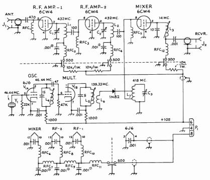
Fig. 16-24—Wiring diagram of the 432-Mc. converter. Capacitance values are in  $\mu\mu f$ ., except decimal values which are in  $\mu f$ . Resistors are  $\frac{1}{2}$  watt unless specified otherwise. All 0.001- $\mu f$ . capacitors marked \* are button-type (Centralab ZA-102); other 0.001- $\mu f$ . capacitors are disk ceramic. All 500- $\mu\mu f$ . feedthrough capacitors are Centralab FT-500.
