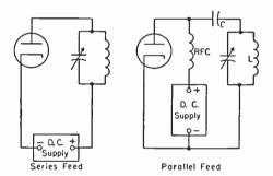
Fig. 2-57—Illustrating series and parallel feed.
