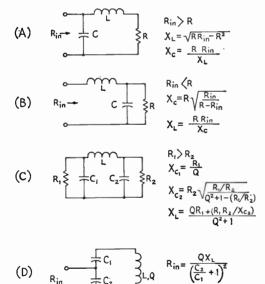
Fig. 2-52—Impedance-matching networks adaptable to amateur work. (A) L network for transforming to a higher value of resistance. (B) L network for transforming to a lower resistance value. (C) Pi network. R<sub>1</sub> is the larger of the two resistors; Q is defined as R<sub>1</sub>/Xc<sub>1</sub>. (D) Tapped tuned circuit used in same receiver applications. The impedance of the tuned circuit is transformed to a lawer value, R<sub>1n</sub>, by the capacitive divider.
