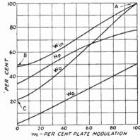
Fig. 10-16—Cathode-modulation perfarmance curves, in terms of percentage af plate madulation platted against percentage af Class C telephony tube ratings.
