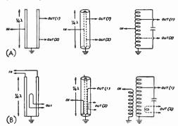
Fig. 2-60—Equivalent caupling circuits far parallel-line, caaxial-line and canventianal resanant circuits.
