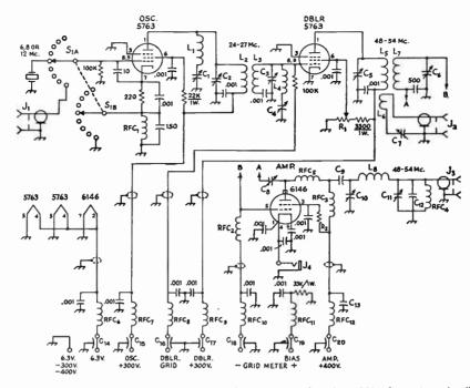
Fig. 17-18—Schematic diagram of 48-54-Mc. exciter. All capacitances less than .001 μf. are in μμf. All .001-μf. capacitors are disk ceramic. All resistors are ½ watt unless otherwise specified.
