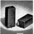
TONE MODULATOR .. The No. 90751 Tone Modulator is a small package containing a transistar audio ascillator and its mercury bottery, which plugs into the phone jack of a Grid Dip Meter to modulate the signal at approximately 800 cycles for applications requiring a modulated signal. Dimensions: only  $2\frac{1}{4} \times 1\frac{1}{16} \times 1\frac{1}{16}$  in.
