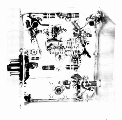
Fig. 16-12—Interior of the 144-Mc. converter. Details of parts arrangement are given in the text. The i.f. output from the mixer plate coil, L<sub>5</sub>, (upper right) is brought through a shielded lead down the side and across the bottom to the output connector, J<sub>2</sub>, at the lower left.
