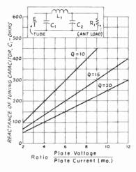
Fig. 6-13—Reoctance of input capacitor, C<sub>1</sub>, as a function the ratio of plate voltage to plate current.
