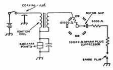
Fig. 19-1—Ignition system with recommended suppression methods.
