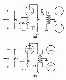
Fig. 9-3—Transformer-coupled amplifier circuits for driving a push-pull amplifier. A is for resistance-transformer caupling; B for transformer coupling. Designations correspond to those in Fig. 9-2. In A, values can be taken from Table 9-1. In B, the cathode resistor is calculated from the rated plate current and grid bias as given in the tube tables for the particular type of tube used.
