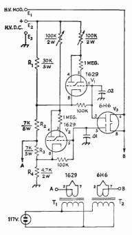
Fig. 10-24—Circuit diagram of the modulation monitor. Unless specified otherwise, resistors are ½ watt, resistances are in ohms, capacitances are in μf. C<sub>1</sub>, C<sub>2</sub>—Disk ceramic.
