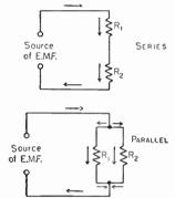
Fig. 2-4—Resistors connected in series and in parallel.
