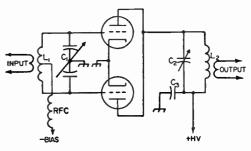
Fig. 6-30—Circuit af a push-push frequency multiplier far even harmanics.
