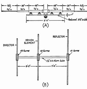
Fig. 14-57—Dimensions of a compact 14-Mc. beam. A—Side view of a typical element. TV-antenna "U" clamps hold the support arms to the boom. Birnbach 4176 insulators support the elements. B—Top plan of the beam showing element spacing and loading-coil dimensions. Elements are made of aluminum tubing. Construction of the loading coils and adjustment of the elements are discussed in the text. End-section lengths of 41 inches for the reflector, 40 inches for the director will be close to optimum.
