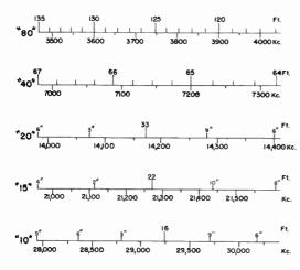
Fig. 14-4—The above scales, based on Eq. 14-B, can be used to determine the length of a half-wave antenna of wire.
