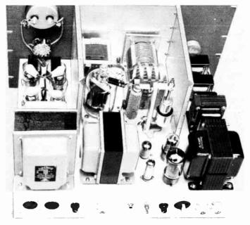
tween the outer end of the low-frequency section and the plate cap of the 2E26. Coil-tap leads run through small feed-through points or grommeted clearance holes in the side of the box.
