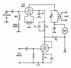
Fig. 10-11—Screen modulation by a "clamp" tube. The grid leak is the normal value for c.w. operation and  $C_2$  should be  $0.002~\mu f$ . or less. See text for discussion of  $C_1$ ,  $R_1$ ,  $R_2$  and  $R_3$ .  $R_3$  should have the proper value for Class A operation of the modulator tube, but cannot be calculated unless triode curves for the tube are available.
