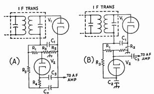
Fig. 5-21—Self-adjusting series (A) and shunt (B) noise limiters. The functions of V<sub>1</sub> and V<sub>2</sub> can be combined in one tube like the 6H6 or 6AL5.
