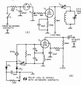
Fig. 12-14—Frequency-shift keyer circuits. Unless otherwise indicated, capacitances are in μμf., resistances are in ohms, resistors are ½ watt. A—Reactance-tube keyer for use with variable-frequency oscillator (W6OWP). B—Crystal oscillator circuit (W2PAT). It is essential that all leads associated with the crystal portion of the circuit be held to a small fraction of an inch in length if maximum shift is desired.
