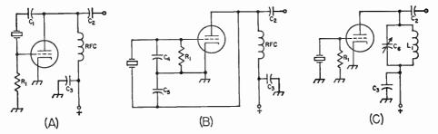
Fig. 6-2—Simple crystal oscillator circuits. A—Pierce. B—Equivolent of circuit A. C—Simple triode oscillotor.  $C_1$  is a plate blocking capacitor,  $C_2$  an output coupling capacitor, and  $C_3$  a plate byposs.  $C_4$  and  $C_5$  are discussed in the text.  $C_6$  and  $L_1$  should tune to the crystal fundamental frequency.  $R_1$  is the grid leak.
