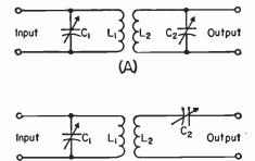
Fig. 2-48—Inductively-coupled resonant circuits. Circuit A is used for high-resistance loads (load resistance much higher than the reactance of either  $L_2$  or  $C_2$  at the resonant frequency). Circuit B is suitable for low resistance loads (load resistance much lower than the reactance of either  $L_2$  or  $C_2$  at the resonant frequency).
