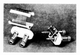
Fig. 21-37—A convenient mounting, using binding-post plates, for L and C standards made from commerciallyavoilable parts. The capacitor is a 100- $\mu\mu$ f. silver mica unit, mounted so the lead length is as nearly zero as possible. The inductance standard, 5  $\mu$ h., is 17 turns of No. 3015 B & W Miniductor, 1-inch diameter,
