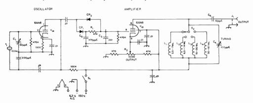
Fig. 21-13—Circuit of the 100-kc. crystal calibrator. Unless otherwise indicated, capacitances are in μf., resistances are in ohms, resistors are ½ watt.
