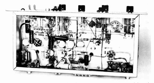
Fig. 11-11—View underneath the chassis of the sideband generator. Tuning capacitors are mounted close under the sockets for the associated plug-in coils. At rear of the chassis (bottom in this view), two terminals are used for bias measurement, and the 4-terminal barrier strip is for making connection to remote control and v.f.o. on-off circuits. Two inductors, part of the low-pass audio filter that protects the audio phase-shift network, are mounted near the r.f. input jack (lower left).
