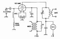
Fig. 10-10—Screen-grid madulation of beam tetrade. Capacitar C is an r.f. bypass capacitar and shauld have high reactance at audia frequencies. A value of 0.002 μf. is satisfactary. The grid leak can have the same value that is used far c.w. aperation of the tube.
