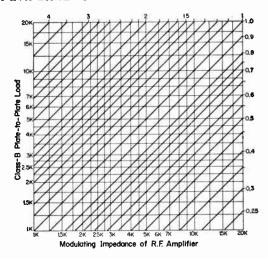
Fig. 9-6—Transformer ratios for matching a Class C modulating impedance to the required plate-to-plate load for the Class B modulator. The rotios given on the curves are from total primary to secondary. Resistance values are in kilohms.
