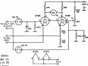
The zero-center meter,  $M_1$ , is not a necessity but is a convenience in making adjustments.  $R_1$  should be adjusted on receiver noise for zero reading. With a 2125-cycle tone the pointer will swing to the left and  $L_1$  should be adjusted for maximum deflection. With a 2975-cycle tone the pointer will swing to the right and  $L_2$  should be adjusted for maximum deflection. Equal deflections should be obtained from both channels.
