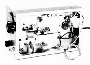
Fig. 5-41—Bottom view of the converter showing placement of parts. The coil at the lower left is  $L_3$ , and the input coil,  $L_1L_3$ , is just to the right of  $L_3$ . The oscillator coil  $L_1L_3$ , is at the left near the center. The output coil,  $L_0$ , is near the top center.
