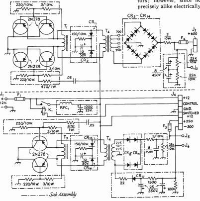
Fig. 19-48—Circuit diagram of the triple transistorized power supply. Capacitances are in μf., resistors are ½ watt unless specified otherwise. Capacitors marked with polarity are electrolytic; others are paper.
