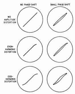
Fig. 9-33—Typical patterns obtained with the connectians shawn in Fig. 9-32. Depending an the number of stages in the amplifier, the pattern may slape upward to the right, as shawn, or upward to the left. Also, depending on where the distartian ariginates, the curvature in the second row may appear either at the tap ar battom of the line ar ellipse.
