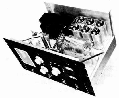
Fig. 6-63—A 900-watt grounded-grid linear amplifier, complete with silicon-diode power supply. Two transformers with secondaries connected in parallel furnish the plate power. Panel controls are bandswitch (to left of meters), loading (upper) and plate tuning. Switches control filament power, plate power and standby-operate.
