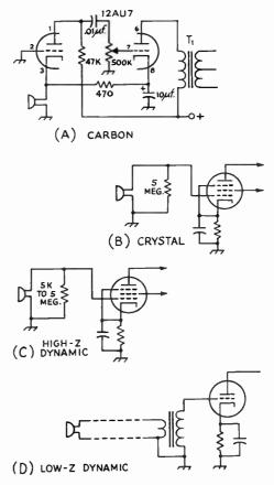
Fig. 9-1—Speech input circuits used with vorious types of microphones.
