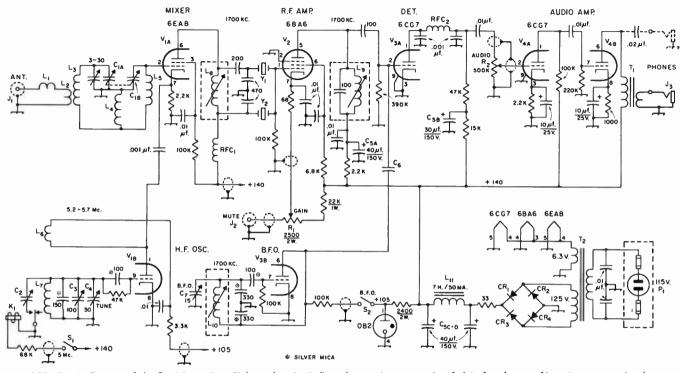
Fig. 5-37—Circuit diagram of the  $2\times4+$  receiver. Unless otherwise indicated, capacitances are in pf. (picofarads or  $\mu\mu$ f.), resistances are in ohms, resistors are  $\frac{1}{2}$ -watt. Capacitors marked with polarity are electrolytic; those marked with asterisk are silver mica.
