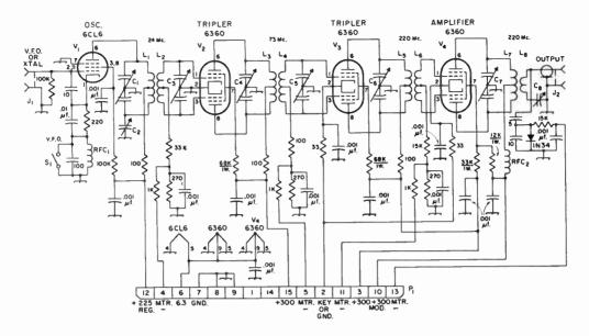
Fig. 17-10—Circuit diagram of the 220-Mc. transmitter. Unless specified otherwise, capacitances are in picofarads (pf. or  $\mu\mu f$ .), resistances are in ohms, resistors are ½ watt.
