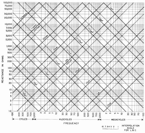
Fig. 2-28—Inductive and capacitive reactance vs. frequency. Heavy lines represent multiples of 10, intermediate light lines multiples of 5; e.g., the light line between 10  $\mu$ h. and 100  $\mu$ h. represents 50  $\mu$ h., the light line between 0.1  $\mu$ f. and 1  $\mu$ f. represents 0.5  $\mu$ f., etc. Intermediate values can be estimated with the help of the interpolation scale shown.
