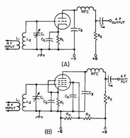
Fig. 5-4—Circuits for plate detection. A, triode; B, pentode. The input circuit,  $L_zC_1$ , is tuned to the signal frequency. Typical values for the other components are:
