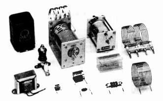
Inductors for power and radio frequencies. The two iron-core coils at the left are "chokes" for power-supply filters. The mounted air-core coils at the top center are adjustable inductors for transmitting tank circuits. The "pie-wound" coils at the left and in the foreground are radio-frequency choke coils. The remaining coils are typical of inductors used in r.f. tuned circuits, the larger sizes being used principally for transmit-
