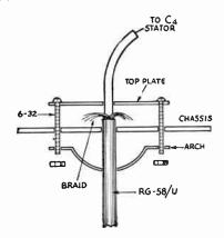
Fig. 6-52—Exploded view of the coble clamp used to hold the coaxiol cable running to  $J_2$ . The top plote is a  $1\frac{1}{2}$ -inch square of sheet aluminum with holes at the four corners for 6-32 screws. The arch is a  $\frac{1}{2}$ -inch wire strop that mounts diagonally under the chassis. When tightened, the top plote clamps the coble broid to the chassis; the arch lends support to the cable.
