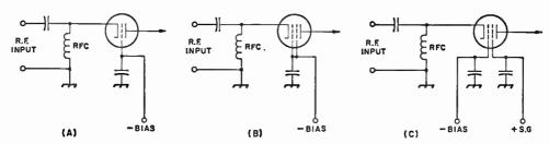
Fig. 6-27—A—Graunded-grid triade input circuit. B—Tetrade input circuit with grid and screen directly in parallel. C—Tetrade circuit with d.c. valtage applied to the screen. Plate circuits are conventional.
