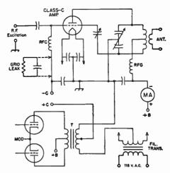
Fig. 10-15—Circuit arrangement for cathode modulation of a Class C r.f. amplifier. Values of bypass capacitors in the r.f. circuits should be the same as for other madulation methods.
