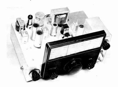
Fig. 5-35—The  $2\times4+$  receiver uses four tubes and tunes 3.5 to 4.0 Mc. and 6.9 to 7.4 Mc.; the range is selected by the setting of a two-section input tuning capacitor housed in a Minibox (extreme right). The toggle switches under the input tuning knob turn on (top) a 5-Mc. range for reception of WWV and (bottom) the b.f.o. Knobs either side of the central main tuning knob control (left) audio gain and (right) i.f. gain. B.f.o. frequency is set by the knob at the left.
