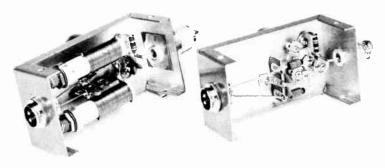
Fig. 21-26—Each diode noise generator is housed in a  $4\times2\%\times1\%$ -inch "Minibox" (Bud CU-2102-A). Power connections are made through double-pin male receptacles (Amphenol 80 PC2M), and the r.f. connection is made to the receiver or converter by a suitable plug. The plug on the 7- to 90-Mc. generator (left) is a PL-259 held to the face of the "Minibox" by a small copper plate and a UG-176/U reducing adapter.
