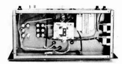
Fig. 9-28—The relay and filament transformer are mounted below the chassis. C<sub>2</sub>, C<sub>2</sub> and K<sub>1</sub> are mounted on small stand-off insulators.
