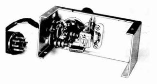
Fig. 6-93—This bottom view of the crystal oscillator shows the arrangement of components. Terminal strips are used for the cable connectians and alsa as a support for C<sub>1</sub>, the feedback capacitor.
