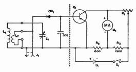
Fig. 21-39—Transistor d.c. amplifier applied to the wavemeter of Fig. 21-10 to increase sensitivity. Components not listed below are the same as in Fig. 21-10. B<sub>1</sub>—Small flashlight cell.
