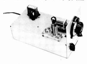
Fig. 5-48—The regenerative preselector covers the range 7 to 30 Mc.; it can be used ahead of any receiver to improve gain, image rejection and, in many cases, sensitivity. A dual triode 6CG7 is used as r.f. amplifier and cathode follower.
