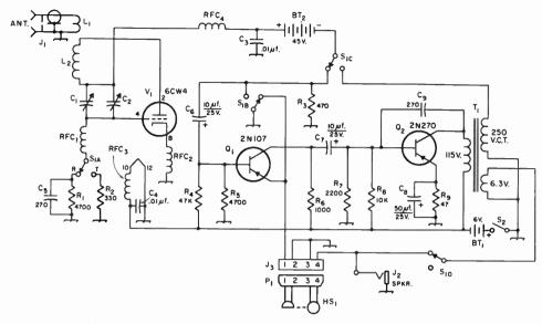
Fig. 16-18—Circuit diagram of the 420-Mc. transceiver. Unless specified otherwise, capacitances are in picofarads (pf. or  $\mu\mu$ f.), resistances are in ohms, resistors are  $\frac{1}{2}$  watt. Capacitors marked with polarity are electrolytic.
