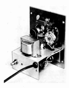
Fig. 21-22—Inside view of the audio oscillator. The a.c. switch,  $S_3$ , is mounted on the OUTPUT control at the left on the panel. The ceramic capacitors in the frequency-determining circuits are mounted on the rotary switch,  $S_1$ , at the right.  $S_2$  is above the tube, and  $I_1$  is on the near edge of the chassis, which is a U-shaped piece of aluminum  $3\frac{1}{2}$  inches deep with  $1\frac{1}{2}$ -inch lips.  $R_1$  is mounted on the near lip at the left.
