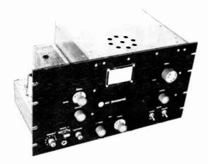
Fig. 17-16—The 50-Mc, r.f. unit. Exciter, left portion on the assembly, also serves on 144 Mc. Amplifier utilizes a 4-125A, 4-250A or 4-400A
