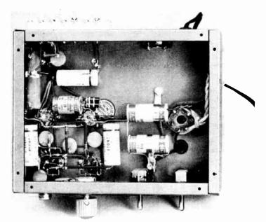
9-16-Below-chassis Fig. view of the modulator. The rectifier tube socket and electrolytic filter capacitors are at the right in this view. The 12AX7 socket is at the lower left. Bleeder resistor Rs is at the upper left, near the 6-terminal connection strip on the rear edge of the chassis. Placement of components is not critical, but the leads in the first two stages should be kept short and close to the chassis to minimize hum troubles.
