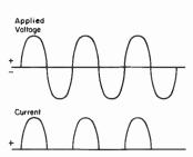
the polarity of the current through the load is as indicated. If the diode were reversed, the polarity of the voltage developed across the load R would be reversed.
