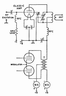
Fig. 10-5—Plate modulation of a Closs C r.f. amplifier. The r.f. plate bypass capacitor, C, in the amplifier stage should have reasonably high reactance at audio frequencies. A value of the order of 0.001  $\mu$ f. to 0.005  $\mu$ f. is satisfactory in practically all cases. (See chapter on modulators.)
