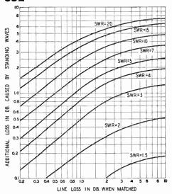
Fig. 13-9—Effect of standing-wave radio on line loss. The ordinates give the additional loss in decibels for the loss, under perfectly matched conditions, shown on horizontal scale.
