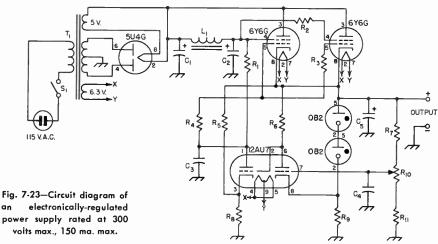
$\begin{array}{l} C_1,\ C_2,\ C_5-16-\mu f.\ 600\text{-volt electrolytic.}\\ C_3-0.015-\mu f.\ paper.\\ C_4-0.1-\mu f.\ paper.\\ R_1-0.3\ megohm,\ \frac{1}{2}\ watt.\\ R_2,\ R_3-100\ ohms,\ \frac{1}{2}\ watt.\\ R_4-510\ ohms,\ \frac{1}{2}\ watt.\\ R_5,\ R_8-30,000\ ohms,\ 2\ watts.\\ R_6-0.24\ megohm,\ \frac{1}{2}\ watt. \end{array}$
