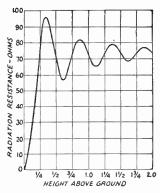
Fig. 14-2—Theoretical curve of variation of radiation resistance for a very thin half-wave horizontal antenna as a function of height in wavelength above perfectly reflecting graund.
