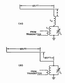
Fig. 14-28—Bent antenna for the 160-meter band. In the system at A, the vertical portion (length X) should be made as long as possible. In either antenna system, L<sub>1</sub>C<sub>1</sub> should resonate at 1900 kc., roughly. To adjust  $L_2$  in antenna A, resonate  $L_1C_1$  alone to the operating frequency, then connect it to the antenna system and adjust L2 for maximum loading. Furthur loading can be obtained by
