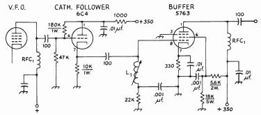
Fig. 6-6—Circuit of an isolating amplifier for use between v.f.o. and first tunable stage. Unless otherwise specified, all capacitances are in picofarads, all resistors are  $\frac{1}{2}$  watt.  $\frac{1}{2}$ , for the 3.5-Mc. band, consists of 100-140  $\mu$ h. adjustable inductor. RFC<sub>1</sub> is 100  $\mu$ h. All capacitors are disk ceramic.
