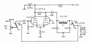
Fig. 9-12—Practical speech clipper circuit with low-pass filter. Capacitances below 0.001  $\mu$ f. are in  $\mu\mu$ f. Resistors are  $\frac{1}{2}$  watt. L<sub>1</sub>—20 henrys, 900 ohms (Stancor C-1515). S<sub>1</sub>—D.p.d.t. toggle or rotary.
