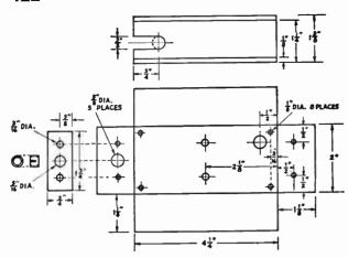
Fig. 16-29—Details of the sheet-metal parts of the trough-line tank circuits. The small plate at the left is insulated from the end of the trough assembly with thin sheet teflon. Slot in the partition, upper portion of drawing, provides space for the mixer crystal, as shown in Figs. 16-30 and 16-31.
