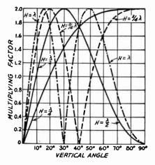
Fig. 14-1—Effect of ground on radiation of horizontal antennas at vertical angles for four antenna heights.
