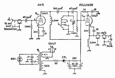
Fig. 8-17—Circuit diagram of the electronic t.r. switch. Unless otherwise specified, resistances are in ohms, resistors are ½ watt, capacitances are in μf.
