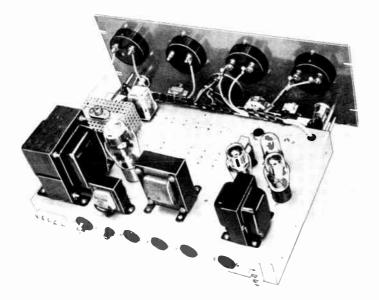
Fig. 6-70—Top view of the control unit. The voltmeter multiplier resistors are housed in a cane-metal protective shield (upper left). Resistors  $R_8$  and  $R_9$  are mounted under the sets of ventilation holes (center near panel).
