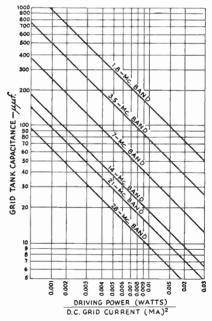
Fig. 6-20—Chart showing required grid tank capacitance far a Q of 12. To use, divide the driving power in watts by the square of the d.c. grid current in milliamperes and proceed as described under Fig-6-9. Driving power and grid current may be taken from the tube tables. When a split-stator capacitor is used in a balanced grid circuit, the capacitance of each section may be half that shown.
