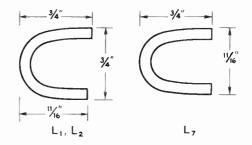
Fig. 16-26—Details of "coils" L<sub>1</sub>, L<sub>2</sub> and L<sub>7</sub>. Material is No. 10 tinned copper wire. Taps on L<sub>1</sub> and L<sub>2</sub> are ½ up from ground end; taps on L<sub>7</sub> are ½ and ½ up from ground end.
