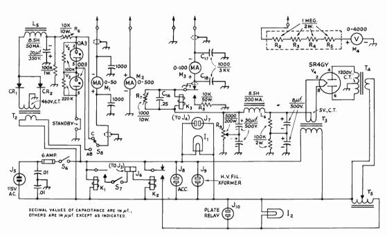
Fig. 6-68—Circuit diagram of the 4-400A amplifier (above the dashed line) and power supply/control unit.
