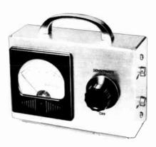
Fig. 19-41-A front view of the field-strength meter. Sensitivity control R<sub>1</sub> is to the right of the 0-1 indicating meter. Antenna input and ouput connectors are mounted on the right end of the box.
