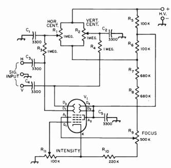
Fig. 21-54—Oscilloscope circuit for modulation monitoring. Constants are for 1500- to 2500-volt high-voltage supply. For 1000 to 1500 volts, omit R<sub>8</sub> and connect the bottom end of R<sub>7</sub> to the top end of R<sub>9</sub>.
