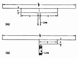
Fig. 14-45-The "T" match and "gamma" match.
