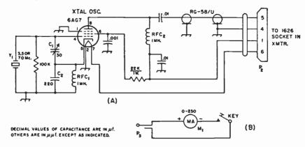
Fig. 6-92—(A) Circuit diagram of external crystal-controlled oscillator. Unless otherwise specified, resistances are in ohms, resistors are  $\frac{1}{2}$  watt. The 0.01- and 0.001- $\mu$ f. capacitors are disk ceramic. (B) Method of connecting the milliammeter in series with the key.
