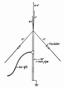
Fig. 14-27—The 14-, 21- and 28-Mc. ground-plane antenna uses wire elements. Vertical elements are taped to a cane pole; the four radials also serve as guy wires. The radials "droop" a little, making a 40-degree angle with the supporting 1-inch pipe.
