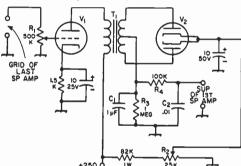
Fig. 9-11—Speech-amplifier output compression cir-
