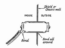
Fig. 23-13—The best method of using the "Hypass" type feed-through capacitor. Capacitances of 0.01 to 0.1 µf. are satisfactory. Capacitors of this type are useful for high-current circuits, such as filament and 115-volt leads, as a substitute for the r.f. choke shown in Fig. 23-11, in cases where additional lead filtering is needed.
