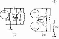
Fig. 6-33—Diagrams showing the peak voltage for which the plate tank capacitor should be rated for c.w. operation with various circuit arrangements. E is equal to the d.c. plate valtage. The values should be doubled for plate modulation. The circuit is assumed to be fully loaded. Circuits A, C and E require that the tank capacitor be insulated from chassis or ground, and from the control.
