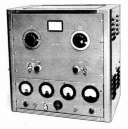
Fig. 6-67—The kilowatt 4-400A amplifier and its control unit are mounted in a 21-inch gray hammertone rack cabinet (Bud CR-1727). Shelf brackets (Bud SA-1350) are mounted on both sides of the cabinet to hold the amplifier chassis. Below the meters, from left to right: filament pilot light, key-type a.c. switch,
