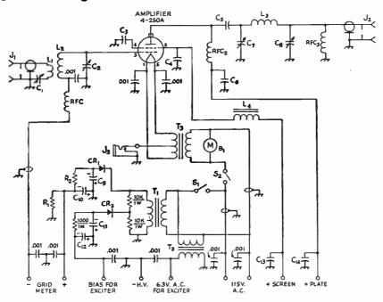
Fig. 17-21—Schematic diagram and parts list for the 4-250A amplifier. All capacitors marked .001 μf. are 600-volt disk ceramic.
