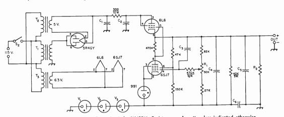
Fig. 7-24—High-voltage regulator circuit by W4PRM. Resistors are 1 watt unless indicated otherwise.
