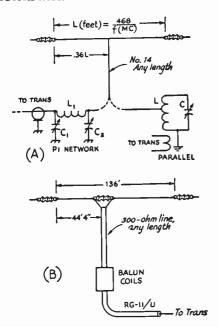
Fig. 14-21—Two versions of the off-center-fed antenna.
