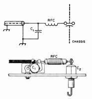
Fig. 23-12—Additional lead filtering for harmonics or other spurious frequencies in the high v.h.f. TV band (174-216 Mc.)
