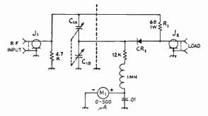
Fig. 21-46—Circuit of the impedance bridge. Resistors are composition, ½ watt except as noted. Fixed capacitors are ceramic.
