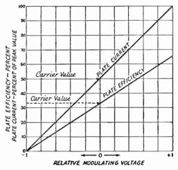
Fig. 10-9—In a perfect grid-madulated amplifier bath plate current and plate efficiency would vary with the instantaneous madulating valtage as shawn. When this is so the madulatian characteristic is as given by curve A in Fig. 10-4, and the peak envelope autput pawer is faur times the unmadulated carrier pawer. The variatians in plate current with madulatian, indicated above, da not register on a d.c. meter, so the plate meter shaws no change when the signal is madulated.
