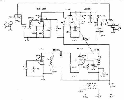
Fig. 19-13—Schematic diagram for the 144-Mc. converter. All resistors  $\frac{1}{2}$  watt unless otherwise specified. Capacitor values below 0.001  $\mu$ f. are in  $\mu\mu$ f. All 1000- $\mu\mu$ f. capacitors are disk ceramic. Other fixed capacitors are tubular ceramic.
