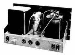
Fig. 9-26—A typical Class B modulatar arrangement. This unit uses a pair of 811As, capable of an audio power output of 340 watts, and includes a splatter filter. The modulation transformer is at the left and the splatter choke at the right. All high-voltage terminals are covered so they cannot be touched accidentally.
