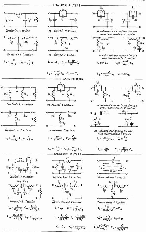
Fig. 2-53—Basic filter sections and design farmulas. In the above farmulas R is in ahms, C in farads, L in henrys, and f in cycles per second.
