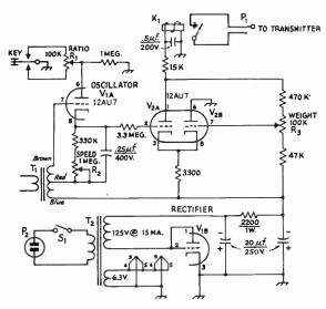
Fig. 8-13—Circuit diagram of the electronic speed key. Unless otherwise specified, resistors are ½ watt. Polarity-marked capacitors are electrolytic, others are tubular paper.
