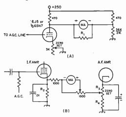
Fig. 5-23—Tuning indicator or S-meter circuits for superheterodyne receivers.
