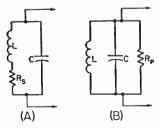
Fig. 2-41—Series and parallel equivalents when the two circuits are resonant. The series resistor,  $R_s$ , in A can be replaced by an equivalent parallel resistor,  $R_p$ , in B and vice versa.
