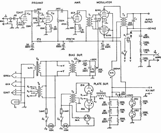
Fig. 9-24—Circuit diagram of the 6146 modulator and power supply. Capacitances are in μf. unless indicated otherwise; capacitors marked with polarity are electrolytic, others may be paper or ceromic as convenient.
