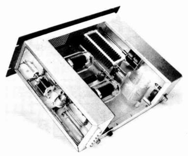
Fig. 6-75—View of the 80-meter amplifier with its cane-metal cavering remaved. As in each amplifier, the chassis is made from two  $5\times13\times3$ -inch chassis and a  $13\times17$ -inch base plate. Input and law-valtage leads make up to terminals and jack in center foreground.
