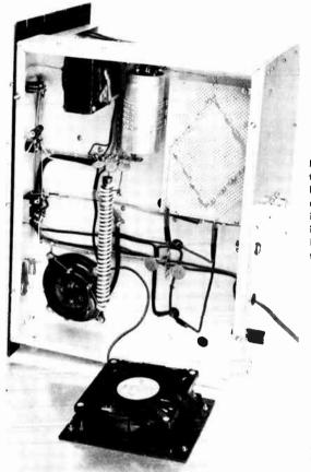
Fig. 6-66—A view underneath the chassis of the amplifier. Protective capacitors and balancing resistors for the diodes are mounted on the other side of the perforated insulating board. The seventh filter capacitor is held to the chassis by a metal clamp. Homemade filament r.f. choke can be seen to the right of the tube socket. It is supported by two plastic cable clamps.
