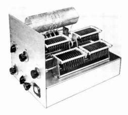
Fig. 13-16—This wide-range antenna coupler can be used with parallel-line or coaxial transmissian lines, as well as with a wire of random length. The capacitors at the center of the chassis are insulated from the chassis and from each other; the near capacitor is a normal split-stator capacitor and is maunted on the chassis. The cail at the far side is supported by its leads above the band switch.
