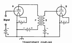
Fig. 3-10—Three basic forms of coupling between vacuum-tube amplifiers.
