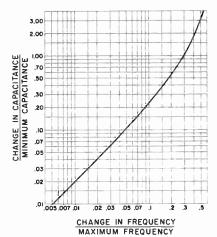
Fig. 5-10—Minimum circuit capacitance required in the circuit of Fig. 5-9A as a function of the capacitance change and the frequency change. Note that maximum
