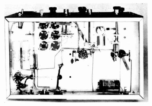
Fig. 6-46—Group of six octal sockets (upper left) serves as crystal sockets. Socket at center of chassis holds 6AG7 oscillator tube; the 3—30-pf. mica compression trimmer mounted alongside is excitation control for oscillator stage. Small midget capacitor above coil is neutralizing capacitor adjusted from above chassis; this capacitor and arid tuning capacitor to right must be insulated from chassis.
