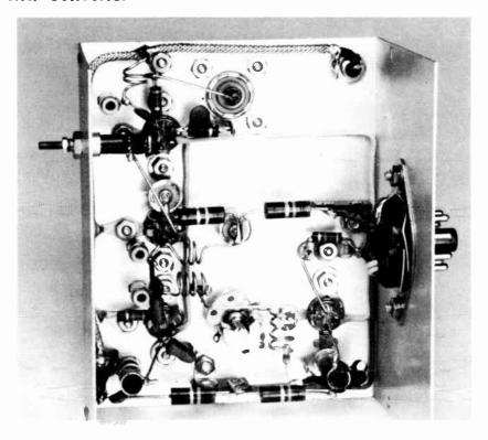
Fig. 16-15—View underneath the chassis of the 220-Mc, converter. The long shielded wire runs from  $L_5$  at the lower left to the output jack. Silver-button mica capacitors (Centralab ZA-102) that bypass the plate coil and the control grid of the second 6CW4 (center left) are also used to support several resistors. Coil  $L_8$  is supported by the terminals of  $C_5$  (bottom center). Chassis is part of  $3\times4\times5$ -inch Minibox.
