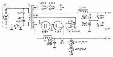
Fig. 6-51—Power supply section of the all-purpose omplifier.
