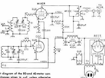
Fig. 5-40—Circuit diagram of the 80-and 40-meter converter. All capacitances given in  $\mu\mu f$ , unless otherwise noted.
