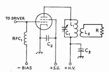
Fig. 6-10—Inductive-link output coupling circuits.
