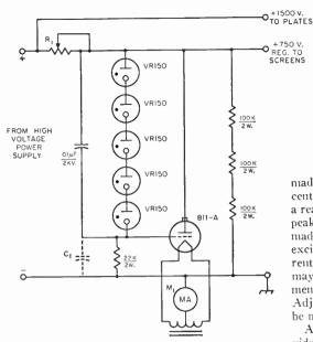
the amplifier screen. This provides a constant load for the scries resistor  $R_1$ .
