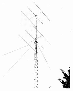
Fig. 18-13—Stacked array for 50 Mc. using two of the 3-element bays of Fig. 18-7. Phasing system and flexible section for rotation are of coaxial line, A "Q" section matches this to 450-ohm open-wire line for run to the station,
