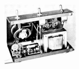
Fig. 21-27—Power supply for the noise generators is housed in a 7-inch wide sloping-panel cabinet (Bud AC-1613). Switches, from left to right, are (referring to Fig. 21-25) S<sub>2</sub>, S<sub>1</sub> and S<sub>2</sub>.
