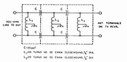
Fig. 23-30—Another type of high-pass filter for 300ohm line. The coils may be wound on ½-inch diameter plastic knitting needles, *Important*: Do not use a direct ground on the chassis of a transformerless receiver. Ground through a 0.001-μf. mica capacitor.
