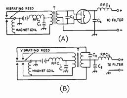
Fig. 19-44—Basic types of vibrator power-supply circuits.
