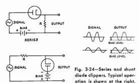
tion of single-frequency oscillations. Of particular interest is the clipper or limiter circuit, because of its several applications in receiving and other equipment.
