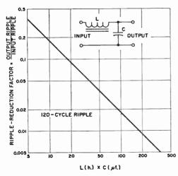
Fig. 7-9—Ripple-reduction factor for various values of L and C in filter section. Output ripple = input ripple × ripple factor.
