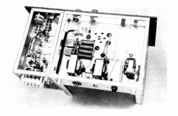
adjustment of the amplifier grid circuit, insert an s.w.r. bridge unit such as a Micromatch in the coax connecting the driver and amplifier, and tune  $C_1$  and  $C_2$  in the amplifier alternately for minimum reflected power. Adjust the driver tuning for maximum forward power.
