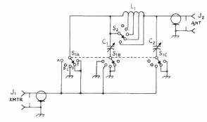
Fig. 13-13—Circuit diagram of an antenna coupler for "rondom" antennas. All contacts of  $S_2$  ore not shown.
