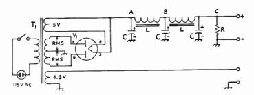
Fig. 7-14—Typical a.c. powersupply circuit for receivers, exciters, or low-power transmitters. Representative values will be found in Table 7-II. The 5-volt winding of T<sub>1</sub> should have a current rating of at least 2 amp. for types 5Y3-GT and 5V4-GA, and 3 amp. for 5U4-GB.
