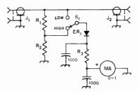
Fig. 21-30—Dual-range r.f. voltmeter circuit. Capacitances are in  $\mu\mu f$ ; capacitors are disk ceramic.
