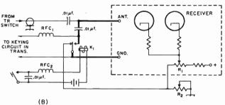
Fig. 8-9—Two variations of a circuit for smooth break-in operation, using (A) separate receiving antenna or (B) an electronic TR switch. The leads shown as heavy lines should be kept as short as possible, to minimize direct transmitter pick-up.
