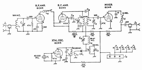
Fig. 16-11—Schematic diagram and parts information for the 144-Mc. converter. Resistors ½ watt unless specified. Fixed capacitors are ceramic unless specified. Decimal values in  $\mu f_{**}$ , others in  $\mu \mu f_{**}$
