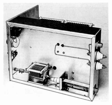
Fig. 13-18—The link capacitar and the Manimatch are maunted underneath the chassis.
