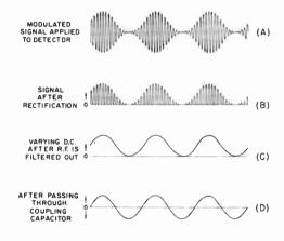
Fig. 5-3-Diagrams showing the detection process.
