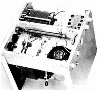
Fig. 6-80—Rear view of the 3-1000Z amplifier with the back wall and SK-516 chimney removed. The 4  $\times$  4  $\times$  2-inch box in the foreground houses the pi-network input circuits and bandswitch sections. S<sub>1A-B</sub>. The antenna changeover relay is mounted directly belaw.
