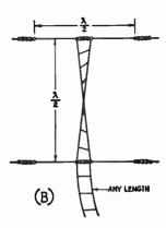
Broadside arrays may be fed either by tuned open-wire lines or through quarter-wave matching sections and flat lines. In Fig. 14-30B, note the "crossing over" of the phasing section, which is necessary to bring the elements into proper phase relationship.
