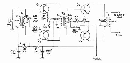
Fig. 19-28—Circuit of the 25-watt transistor madulator. Resistances are in ohms. Capacitors are electralytic.
