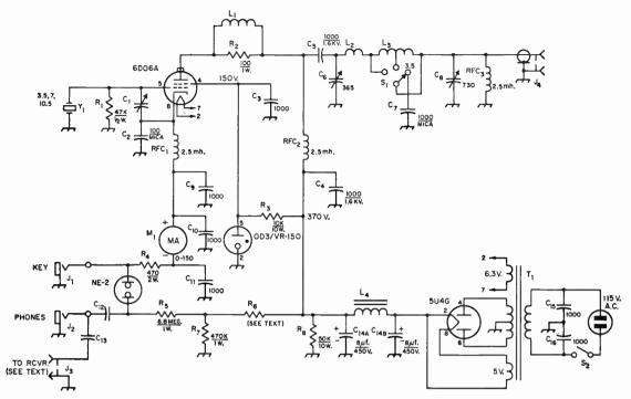
Fig. 6-36—Circuit diagram of the three-band transmitter. Unless otherwise specified, capacitances are in  $\mu\mu$ f. Resistances are in ohms (K=1000).
