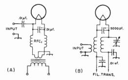
Fig. 6-29—Methods of isolating filament from ground.
