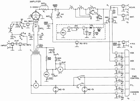
Fig. 6-79—Circuit diagram of the 3-1000Z amplifier. Unless specified otherwise, capacitances are in picotarads (pf. or  $\mu\mu$ f.). For simplicity, only one set of components is shown at  $S_{1A-B}$ .
