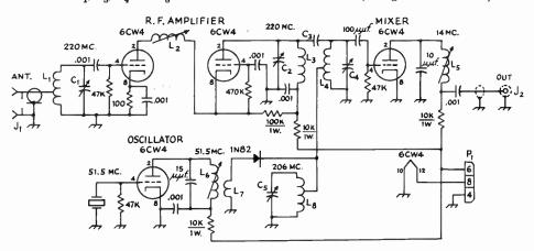
Fig. 16-14—Circuit diagram of the 220-Mc. crystal-controlled converter. Unless specified otherwise, resistors are ½ watt, resistances are in ohms, capacitances in μf.
