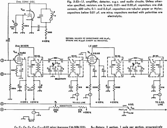
C<sub>6</sub>, C<sub>7</sub>, C<sub>8</sub>, C<sub>0</sub>, C<sub>10</sub>, C<sub>11</sub>—0.01 mica (Aerovox CM-30B-103). C<sub>12</sub>—9-180-µµf, mica compression trimmer.
