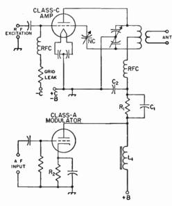
Fig. 10-8—Chake-caupled Class A madulatar. The cathade resistar,  $R_2$ , shauld have the narmal value far aperatian af the madulatar tube as a Class A pawer amplifier. The madulatian chake,  $L_1$ , shauld be 5 henrys ar mare. A value af 0.001 ta 0.005  $\mu$ f. is satisfactory at  $C_2$ , the r.f. amplifier plate bypass capacitar. See text far discussian af  $C_1$  and  $R_1$ .
