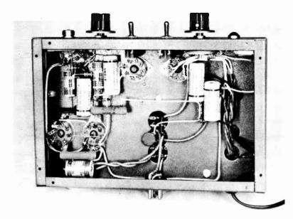
Fig. 9-19-Underchassis view of the 6BQ6GT modulator. The two large capacitors at the right are the filter capacitors in the power supply. The madulator bias resistor and bypass capacitor  $(R_1C_3)$  ore at lower left. Leads from the modulation transformer go through the three holes in the chassis. Shielded wire is used for heater, microphone input, and gaincontrol leads.
