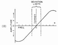
Fig. 12-7—F.m. or p.m. detection characteristics. A—"Slope detection," using the sloping side of the receiver's selectivity curve to convert f.m. or p.m. to a.m. for subsequent rectification. B—Typical discriminator characteristic. The straight portion of this curve between the two peaks is the useful region. The peaks should always lie outside the pass band of the receiver's selectivity curve.
