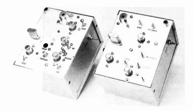
Fig. 16-8—The 50- and 144-Mc. crystal-controlled converters are built in 3 imes 4 imes 5-inch Miniboxes and are designed to work into a receiver that tunes 14 to 18 Mc. Plate voltage required is +150, and use of a 0D3-stabilized supply is suggested.
