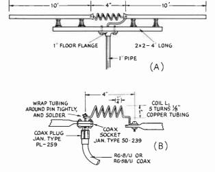
necessary to rotate it 180 degrees. It can be rotated by hand, as will be described, or by a small TV antenna rotator. A 28-Mc. antenna should be made full size (14-C) and fed at the center with RG-11/U.
