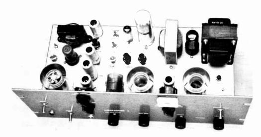
Fig. 11-10—This phasing-type single (and double) sideband generator features the 7360 beam-deflection tube in the balanced-modulator section. The 6CL6 output amplifier (behind meter) delivers sufficient output to drive ane or mare 6146 amplifier tubes in Class AB<sub>1</sub>. Plug-in coils are used to simplify construction.
