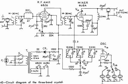
Fig. 5-43—Circuit diagram of the three-band crystalcontrolled converter. Unless indicated otherwise, capacitances are in  $\mu\mu f$ ., resistors are  $\frac{1}{2}$  watt.
