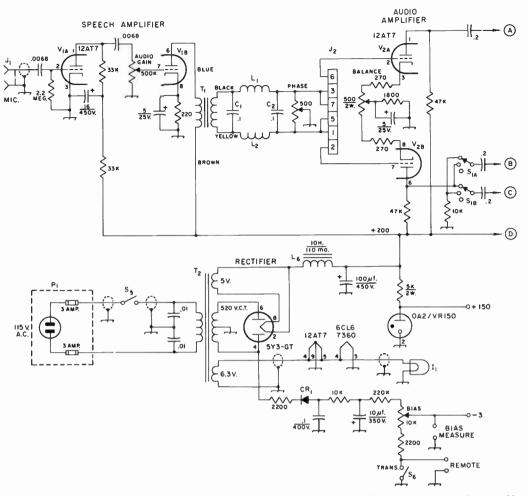
Fig. 11-12—Schematic diagram of the sideband generator. Unless specified otherwise, resistors are ½-watt, .01and .002-μf. capacitors are disk ceramic, 600 volts; .1- and .2-μf. capacitors are tubular paper, 400 volts; capacitors marked with polarities are electrolytic.
