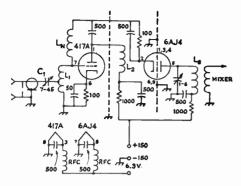
Fig. 16-2—Circuit of the cascode r.f. amplifier. Coupling capacitor,  $C_1$ , may be omitted if spurious receiver responses are not a problem. Neutralizing winding,  $L_{\rm N}$  should resonate at the signal frequency with the gridplate capacitance of the first tube. Base connections are for 417A and 6AJ4, but other small triodes mgy be used.
