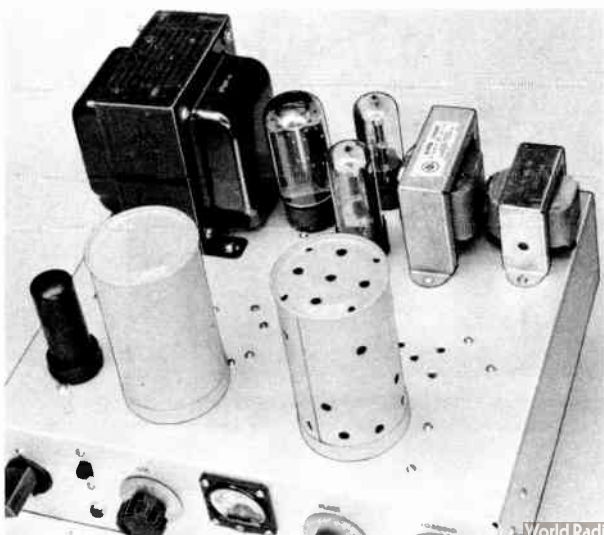
Fig. 6-39—An inexpensive 75-watt transmitter using plug-in coils and an "economy" power supply. The oscillator (left) is a 6AG7; the 1625 output tube is mounted underneath the chassis. Shield cans are baking-powder tins painted gray; the can for the output coil (right) is ventilated for better cooling, as is the chassis behind the can.
