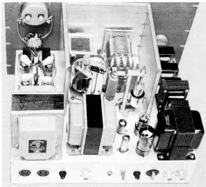
Fig. 6-55—The only shielding required on top of the chassis is the amplifier enclosure shown. A perforated cover for the enclosure is not shown.
