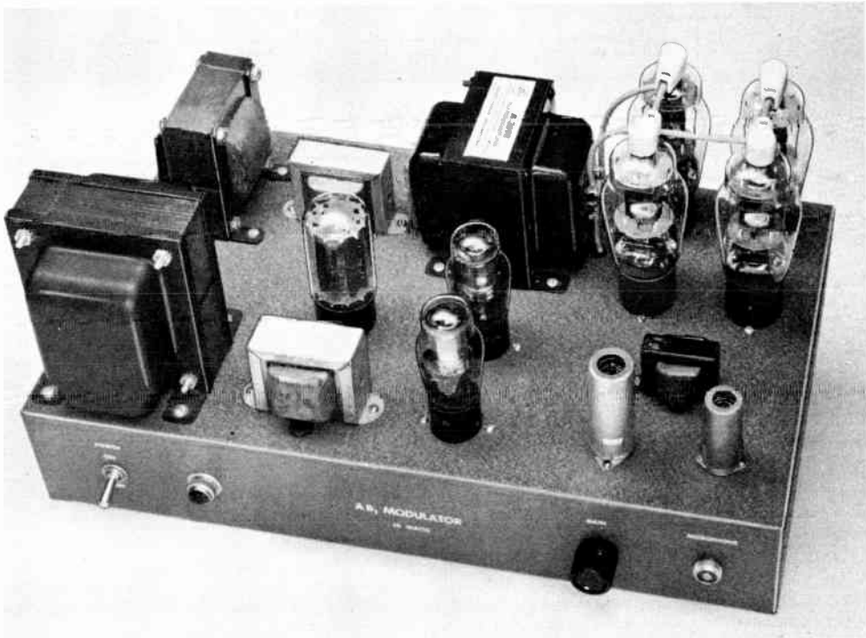
Fig. 9-20—A 50-watt modulator, using four 1625-type tubes in Class AB 1 . With higher plate voltage and a larger modulation transformer, the tubes can deliver up to 140 watts of audio power.
