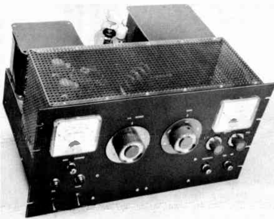
Fig. 6-69—This amplifier operates at a plate input of approximately 500 watts, uses a pair of 811As in grounded-grid, and is complete with power supply on a 13 \times 17 \times 4 -inch chassis. The rack panel is 10\frac{1}{2} \times 19 inches. Front-panel controls include the plate tuning capacitor and band switch in the center, filament and plate power switches with their pilot lights at the lower left, sensitivity control and forward-reflected power switch for the directional coupler at the lower right, variable loading capacitor and auxiliary loading-capacitor switch underneath the 0-1 milliammeter at the right, and the grid-cathode milliammeter with its switch at the upper left. The filter choke, 866As and plate transformer occupy the rear section of the chassis.
