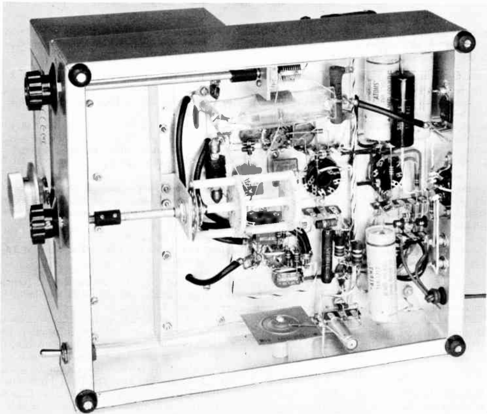
Fig. 6-85—Under the chassis of the two-band v.f.o. Fixed capacitors at the upper right are filter capacitors for the power supply and a 0.5- \mu f. capacitor used in the differential keying circuit. The socket for the relay connections mounted on the back wall of the chassis (right in this view), and the filter capacitor for the negative supply is at the bottom right. The lengths of coaxial cable running to the oscillator tube socket (seen below ceramic switch at center) are pieces of RG-58/U coming from the oscillator tuning compartment above the chassis. Their outer conductors are grounded to the chassis near the tube socket.
