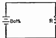
Fig. 2-3—A simple circuit consisting of a battery and resistor.
