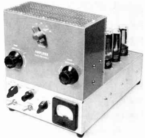
Fig. 6-48—Front view of the 6146 all-purpose amplifier. The upper panel is part of an 8 × 6 × 3½-inch Minibox (Bud CU-2109); the ventilated shielding of Reynolds Aluminium cane metal is fastened to the Minibox and base with sheet-metal screws.
