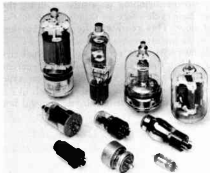
Representative tube types. Transmitting tubes having up to 500-watt capability are shown in the back row. The tube with the top cap in the middle row is a low-power transmitting type. Others are receiving tubes, with the exception of the one in the center foreground which is a v.h.f. transmitting type.
