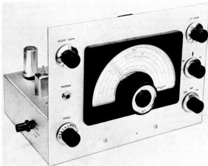
Fig. 5-35—The 2X4 + 1 superheterodyne is a four-tube receiver with 7-tube performance. It tunes the 80- and 40-meter amateur bands, and provision is included for receiving WWV on 5 Mc. A built-in crystal oscillator provides 100-kc. frequency markers throughout the bands. Black knob on the left-hand side controls the calibration oscillator and the WWV reception.
