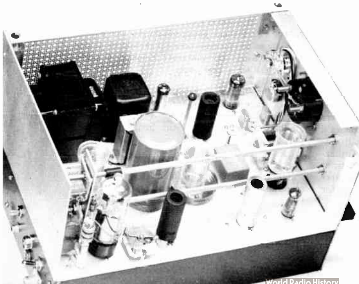
Fig. 11-8—Another view of the top of the filter sideband exciter. The variable capacitor in the VXO circuit is under the meter; the small box to the right of this capacitor is the crystal filter, and the two matched oscillator crystals supplied with the filter are near the panel. The 7360 beam-deflection modulator is in the black tube shield near the filter; a grommet on the shaft (next to the 7360) of the balance potentiometer serves as a knob.
