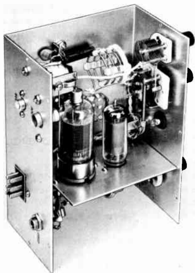
Fig. 19-21—View of the 50-Mc. transmitter showing the r.f. amplifier tank circuits and output loading control. C_3 is on the top right of the panel with C_2 just below it. Output indicator I_1 is below C_2 . This view also shows the two antenna connectors, power plug and grid current jack which are mounted on the rear surface.
