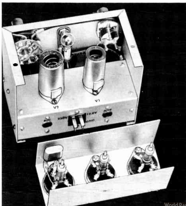
Fig. 19-7—Homemade L-shaped chassis, mounted on small brackets fastened to the side walls of the converter housing, is 4\frac{15}{16} inches long, 2 inches wide and 1\frac{1}{2} inches deep. V_1 is mounted on the chassis to the right of V_2 as seen in this rear view. J_3 , J_2 and J_1 are in line in that order from right to left across the rear wall of the chassis. An interior view of a coil compartment is shown in the foreground. Terminals of the coils are soldered directly to the socket terminals. Notice that the crystal for the oscillator is mounted adjacent to L_4 .
