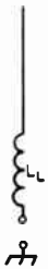
Fig. 19-31 — The capacitive reactance at frequencies lower than the resonant frequency of the whip can be canceled out by adding an equivalent inductive reactance in the form of a loading coil in series with the antenna.
