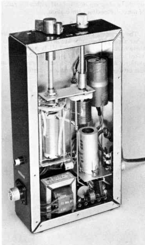
Fig. 8-16—The electronic t.r. switch is built in a 5 X 9 X 2½-inch chassis; the bottom plate has been removed to show the placement of parts. Although two receiver outlets are shown on the near face (a phono jack and a coaxial receptacle), only one is required, depending upon one's choice of cable termination.
