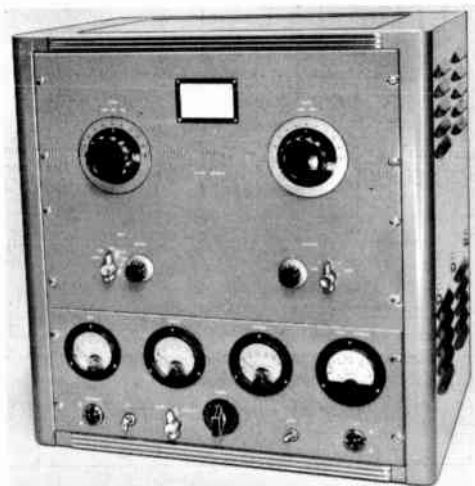
Fig. 6-77—The kilowatt 4-400A amplifier and its control unit are mounted in a 21-inch gray hammer-tone rack cabinet (Bud CR-1727). Shelf brackets (Bud SA-1350) are mounted on both sides of the cabinet to hold the amplifier chassis. Below the meters, from left to right: filament pilot light, key-type a.c. switch, Class AB 1 /C bias switch, screen autotransformer, plate switch and plate pilot light.
