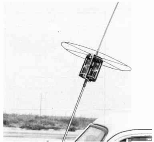
Fig. 19-35—The top-loaded 4-Mc. antenna designed by W6SCX. The loading coil is a B & W transmitting coil. The coil can be tuned by the variable link which is connected in series with the two halves of the coil.
