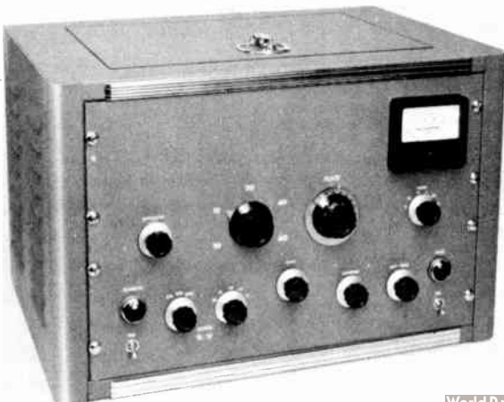
Fig. 6-54—A 500-watt transmitter. Power supplies and a differential keyer are included. It operates with the external v.f.o. tuner shown in Fig. 6-59. Controls along the bottom, from left to right, are for low-voltage power, v.f.o./crystals/s.s.b. switch, driver tank switch, driver tank capacitor, final loading, v.f.o. set switch, and high-voltage. Above, from left to right, are controls for excitation, final tank switch, final tank capacitor and meter switch. The band-switch pointer is made by cutting down the metal skirt of a dial similar to the one to the right.
