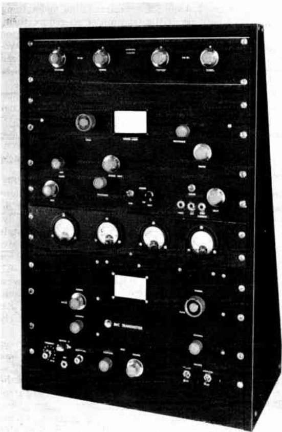
Fig. 17-1—A high-power r.f. section for a 50- and 144-Mc. station. Equipment includes a band-pass exciter for both bands, a 50-Mc. r.f. amplifier built on the same panel, a tripler-driver-amplifier for 144 Mc., and a dual antenna coupler for both frequencies. Units can be operated with a single set of power supplies, and with common speech equipment and meters.
