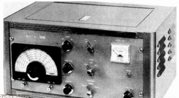
Fig. 5-51—The DCS-500 double-conversion superheterodyne. Left bottom, antenna trimmer, 100-kc. calibrator switch; center, left, top to bottom, noise-limiter switch, volume control, sensitivity control; center, right, b.f.o. switch, a.g.c. speed, selectivity; right, headphone jack, b.f.o. pitch control. The dial is a National ICN. Front panel is 8¾ inches high; the receiver is mounted in a Bud CR-1741 rack cabinet.
