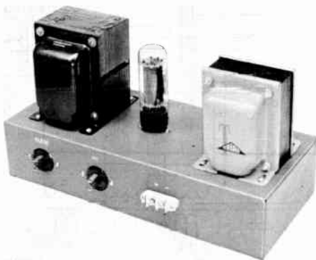
Fig. 7-33—A typical low-voltage power supply. The two a.c. connectors permit independent control of filament and high voltage.
