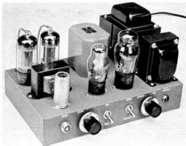
Fig. 9-17—A modulator for transmitters operating at plate inputs up to 50 watts. The speech amplifier and modulator are at the left in this view; power supply components are at the right. The chassis is 7 × 11 × 2 inches.
