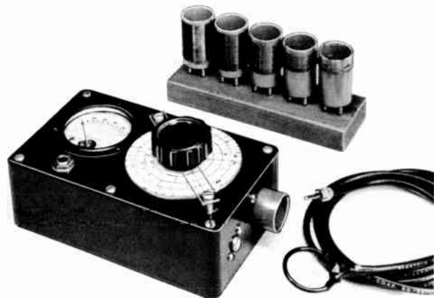
Fig. 21-11—The indicating frequency meter, plug-in coils, and pick-up cables. The meter is built in a bakelite meter case measuring 6 1/4 x 3 3/4 x 2 inches. The 3-inch dial is cut from a piece of aluminum and has a paper hand-calibrated scale cemented on. Hairline indicators are clear plastic mounted on small metal pillars. A 2-inch d.c. instrument is used. Pick-up loops are one turn of No. 14, spaghetti covered, soldered to the ends of the cables. The longer cable (5 feet) is useful to 30 Mc.; the shorter (13 inches) can be used for the full frequency range.
