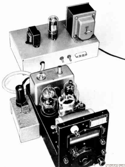
Fig. 6-87—The complete Novice setup, in this case using the 80-meter (BC-696) transmitter. Note the key jack at the lower-left corner of the transmitter panel. The crystal oscillator is connected to the transmitter oscillator-tube socket with a short length of cable terminating in an octal plug. A small notch should be cut in the transmitter cover to provide clearance for the cable when the cover is installed.
