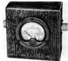
Fig. 21-25—R.f. ammeter mounted for connecting into a coaxial line for measuring power. A "2-inch" instrument will fit into a 2 \times 4 \times 4 metal box.
