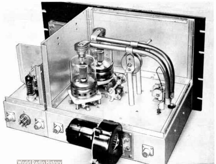
Fig. 17-10—Rear view of the 4-125A final stage. The split-stator capacitor near the middle of the picture is the screen neutralizing adjustment. The plate line is tuned with a capacitor made from parts of a neutralizing unit, mounted on ceramic stand-offs.
