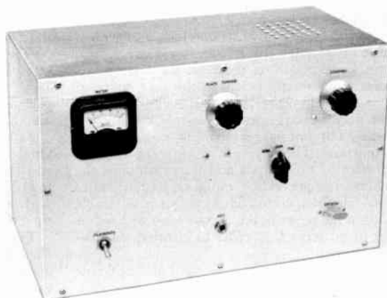
Fig. 6-35—This 30-watt three-band Novice transmitter is enclosed in a 7 \times 9 \times 15 -inch aluminum box. A group of \frac{1}{4} -inch-diameter holes should be drilled in the top of the box over the oscillator tube, as shown, to provide ventilation. A similar set of holes should be drilled in the back cover behind the oscillator circuit.
