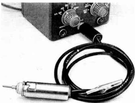
Fig. 21-29—The r.f. probe is used in conjunction with a vacuum-tube voltmeter. The case of the probe is constructed from a 7-pin ceramic tube socket and a 2¼-inch tube shield. A half-inch grommet at the top of the tube shield prevents the output lead of the probe from chafing. The flexible copper-braid grounding lead and alligator clip provide a low-inductance return path from the test circuit. The d.c. output of the probe goes to the phone plug, which plugs into the d.c. input jack of the v.t.v.m.
