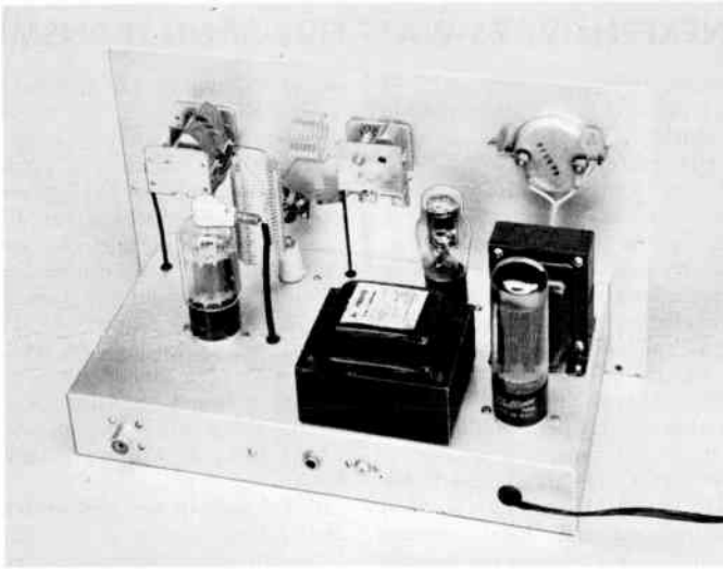
Fig. 6-37—Rear view of the transmitter showing the placement of components above chassis. The loading capacitor, C_8 , is at the left, L_3 is the vertical coil and L_2 the horizontal one. Rubber grommets are used to prevent chafing and to furnish additional insulation on the leads coming from below chassis.
