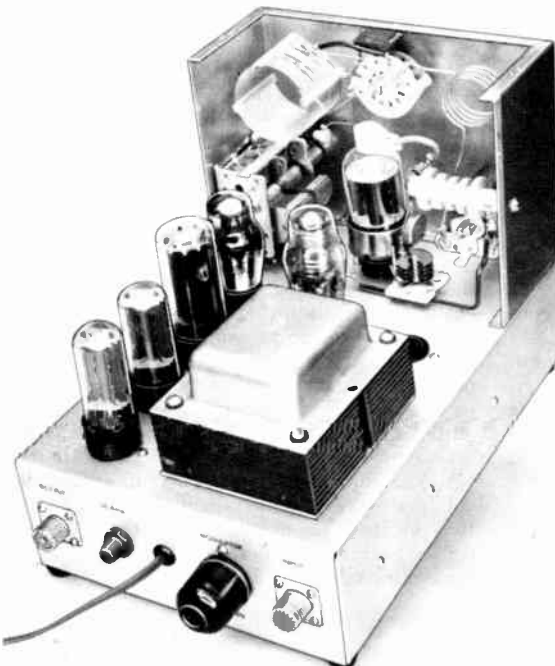
Fig. 6-49—Rear view of the 90-watt all-purpose amplifier with the cone-metal cover removed. One voltage-regulator tube has been removed from its socket (right edge of transformer) to allow the neutralizing capacitor and plate blocking capacitor to be seen. The plate r.f. choke ( RFC_3 in Fig. 6-50) is mounted on one side wall, and the load capacitor and safety choke ( C_1 and RFC_4 in Fig. 6-50) are mounted on the far side wall.
