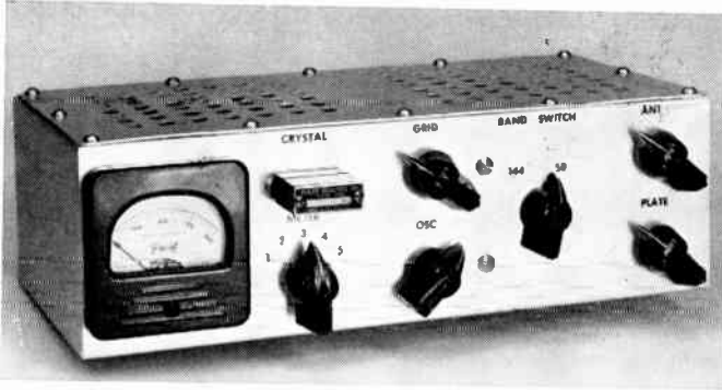
Fig. 19-31 — The crystal is mounted above the meter switch, to the left of the amplifier grid-tuning control. The tuning knob for the oscillator is at the lower left-hand side of the output switch, S_1 . Controls for the output and amplifier plate circuits are at the right. The unit may be used vertically by orientating the meter. Ventilating holes should be drilled in the end used as the top.
