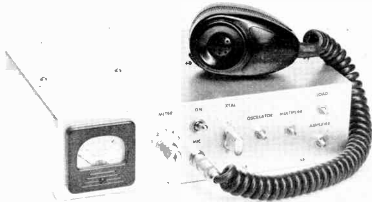
Fig. 19-26—The 50-Mc. mobile transmitter is built into a 7 × 11 × 3-inch aluminum chassis (Premier ACH-125). S_1 on the front wall is flanked by the meter at the left and J_1 and S_2 at the right. The control shaft for C_1 is centered in between the crystal socket and the multiplier tuning control, C_2 . The amplifier tuning capacitor, C_3 , is at the lower right-hand corner directly below the output capacitor, C_4 .
