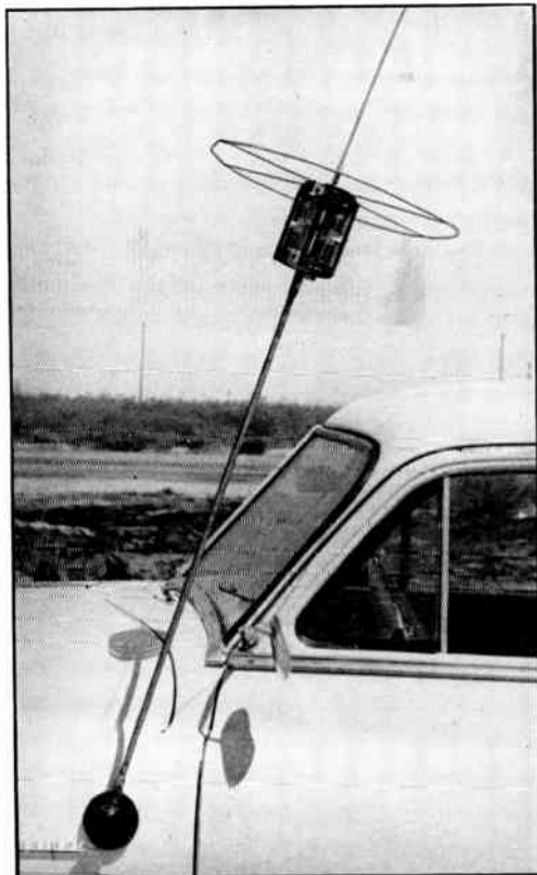
Fig. 19-43 — The top-loaded 4-Mc. antenna used by W6SCX. The loading coil is a B & W transmitting coil. The coil can be tuned by the variable link which is connected in series with the two halves of the coil.
