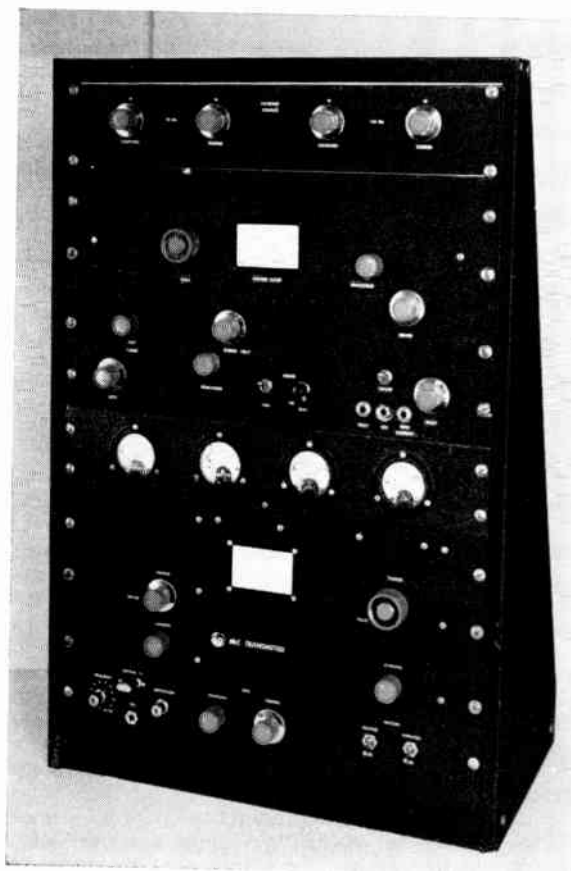
Fig. 17-1 — A high-power r.f. section for a 50- and 144-Mc. station. Equipment includes a band-pass exciter for both bands, a 50-Mc. r.f. amplifier built on the same panel, a tripler-driver-amplifier for 144 Mc., and a dual antenna coupler for both frequencies. Units can be operated with a single set of power supplies, and with common speech equipment and meters.
