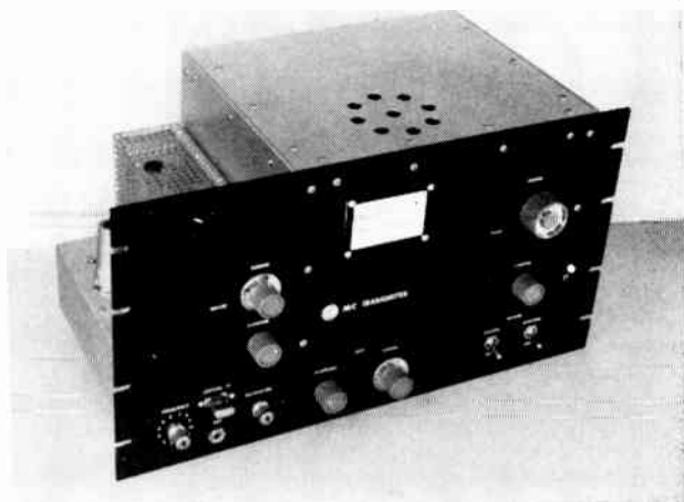
Fig. 17-2 - The 50 Mc. r.f. unit. Exciter, left portion on the assembly, also serves on 144 Mc. Amplifier utilizes a 4-125A, 4-250A or 4-100A.
