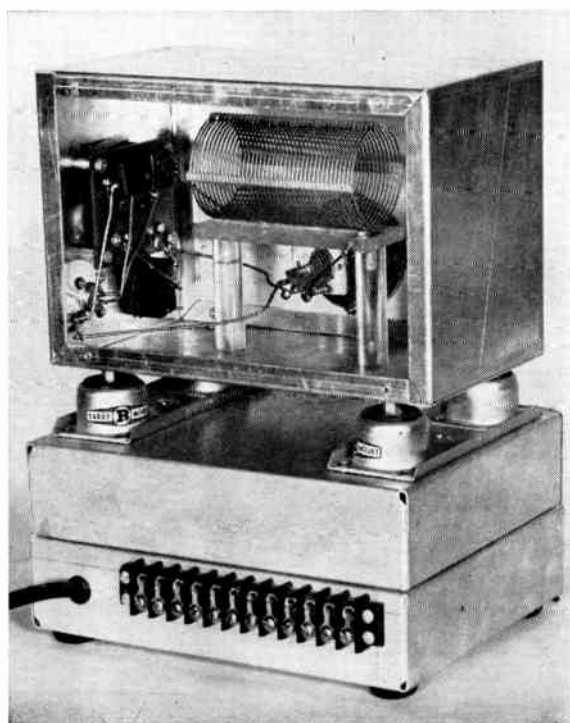
Fig. 6-62 — Rear view of the tuning unit showing the mounting of the inductor on polystyrene sheet and rods and the arrangement of other components. Ceramic trimmers, mounted on the insulating panel at the left, were later replaced with air trimmers ( C_2 and C_3 ).
