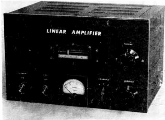
Fig. 12-17 — This linear amplifier uses four parallel-connected tetrodes in a grounded-grid circuit. It can be driven by an s.s.b. exciter capable of 20 watts peak envelope power output. The cabinet is 14½ by 9 by 10 inches deep.
