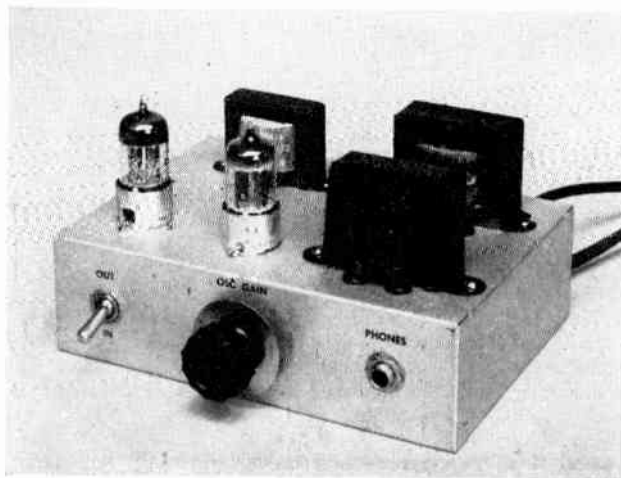
Fig. 8-10 — A combination c.w. monitor and code-practice oscillator that can be used without modification of the receiver or transmitter.
