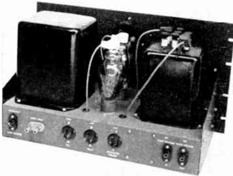
Fig. 9-29 — A typical Class B modulator arrangement. This unit uses a pair of 811 Vs, capable of an audio power output of 310 watts, and includes a splatter filter. The modulation transformer is at the left and the splatter choke at the right. All high-voltage terminals are covered so they cannot be touched accidentally.
