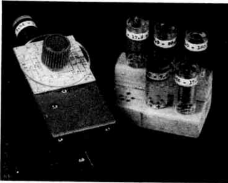
Fig. 21-19 — A compact and light-weight grid-dip meter for one-hand operation. It is built in a 1\frac{5}{8} \times 2\frac{1}{4} \times 4 -inch "Channel-lock" box and uses six plug-in coils to cover the range 1600 kc. to 160 Mc. The power supply and milliammeter for reading grid current are in a separate unit.
