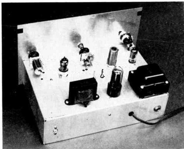
Fig. 5-30 — The miniature tubes, from left to right, are 6U8, 6BD6 (in shield) and 12AX7. The left-hand variable capacitor tunes the mixer input circuit, and the small one in the center tunes the high-frequency oscillator. Note the phono-jack antenna terminal and headphone output jack on the wall of the chassis. The tuning capacitor at rear center is mounted on an aluminum bracket.
