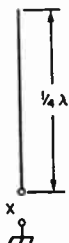
Fig. 19-36 — The quarter-wave whip at resonance will show a pure resistance at the feed point X.
