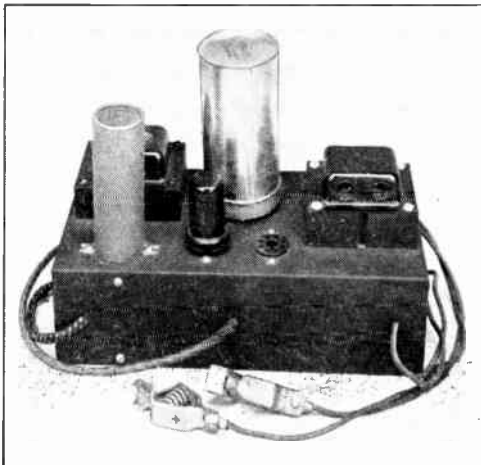
Fig. 19-54 — A typical combination a.c.-d.c. power pack for low-power emergency work. The two transformers are mounted at either end of the chassis. The filter capacitor is at the left, the two rectifier sockets at the center and the vibrator to the rear. The circuit is shown in Fig. 19-53.
