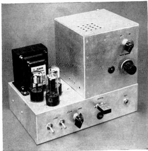
◆ ◆ Fig. 6-38 — Pictured is the completed 6146 rig. The plate-current indicator lamp is to the left of the tuning knob. In areas where TVI is likely to be a problem, a metal bottom plate should be used on the chassis in addition to the 6 \times 6 \times 6 aluminum box shown.
