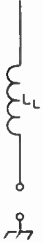
Fig. 19-41 — Placing the loading coil at the center of the whip antenna, instead of at the base, increases the radiation resistance, although a larger coil must be used.
