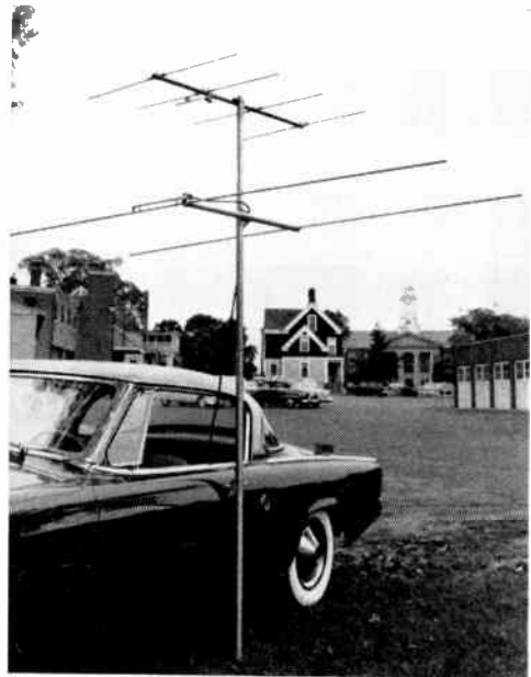
Fig. 18-5 — Two-element 50-Mc. and four-element 144-Mc. arrays designed for portable use. Support is sectional TV masting clamped to car door handle. Elements of 50-Mc. array are made in three sections, for stowing in back of car. Antenna for 144 Mc. is cut-down TV array. Both use gamma match, as shown in Fig. 18-6.
