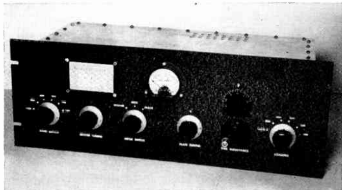
Fig. 6-47 — Controls, from left to right, are for band switch, exciter tuning, meter switch, pi-section tank capacitor, rotary inductor and turns counter, and output-capacitor switch. The panel is 7 by 19 inches. The top cover (a chassis bottom cover) is in place in this view.
