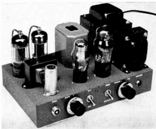
Fig. 9-13 — A modulator for transmitters operating at plate input up to 50 watts. The speech amplifier and modulator are at the left in this view; power supply components are at the right. The chassis is 7 × 11 × 2 inches.
