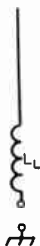
Fig. 19-38 — The capacitive reactance at frequencies lower than the resonant frequency of the whip can be canceled out by adding an equivalent inductive reactance in the form of a loading coil in series with the antenna.
