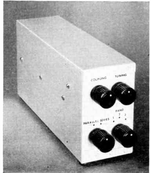
Fig. 5-49 — Front view of the antenna tuner.
