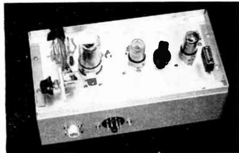
Fig. 17-21 — Top rear view of the 144-Mc. exciter-transmitter, showing power and output connectors on back of the chassis.
