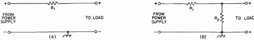
Fig. 7-15 -- A -- Series voltage-dropping resistor. B -- Simple voltage divider. C -- Multiple divider circuit.
