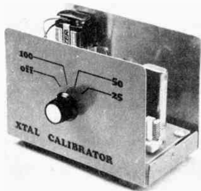
Fig. 26 — The marker generator is housed in a 4-1/2 x 3 x 2-1/2 inch (114 x 76 x 64 mm) aluminum cabinet. A 9-volt battery makes the instrument completely self-contained.
