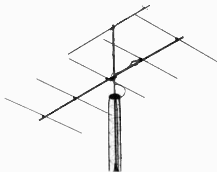
Fig. 6 — Photograph of the 5-element, 50-MHz Yagi. A 432-MHz beam is mounted above.
