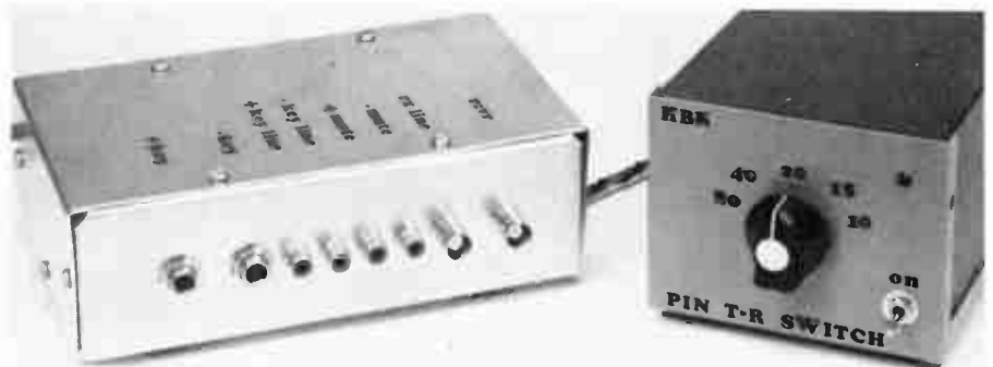
Fig. 29 — Exterior view of the PIN Diode T-R Switch. The box at the right is mounted at the operating position. The box at the left can be mounted remotely.
