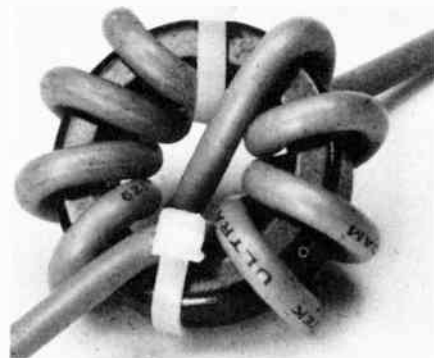
Fig. 11 — Winding the cable on a ferrite toroid is a highly effective shield current suppressor in some cases. Reversing the winding as pictured allows more turns with less shunt capacitance. RG-8X is used in this model, but RG-58 will suffice for moderate power applications. The most important property of the cable is complete shielding — avoid "bargain" cable having less than 95-percent braid coverage.
