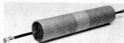
Fig. 10 — This coax shield decoupler is made with steel wool stuffed into an IBM copier tube. This size was selected for photographic purposes, but to be truly effective, the device should be about twice as long.
