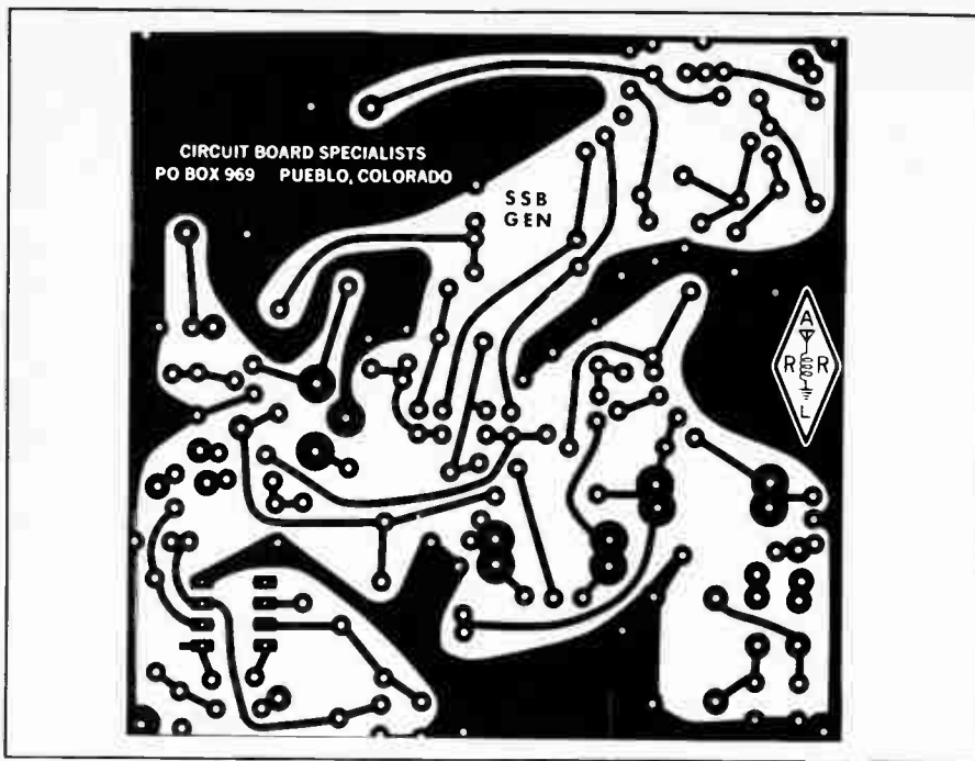
Fig. 46 — Full-scale etching pattern for the ssb generator pc board, shown from the foil side. Black represents unetched copper.
