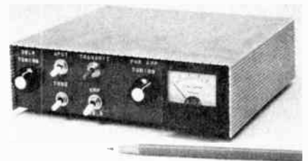
Fig. 53 — Exterior of the W1FB VMOS transmitter. The basics of this unit were treated in May 1979 QST.
