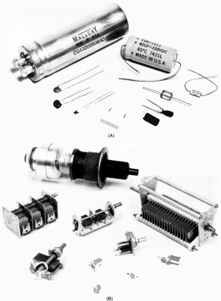
Fig. 15 — Fixed-value capacitors are seen at A. A large computer-grade unit is at the upper left. The 40- \mu\text{F} unit is an electrolytic capacitor. The smaller pieces are silver-mica, disk-ceramic, tantalum, polystyrene and ceramic chip capacitors. The small black unit (cylindrical) is a pc-board-mount electrolytic. Variable capacitors are shown at B. A vacuum variable is at the upper left.
