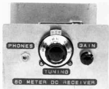
Fig. 49 — Front view of the beginners receiver. The panels are made from double-sided pc board material.
