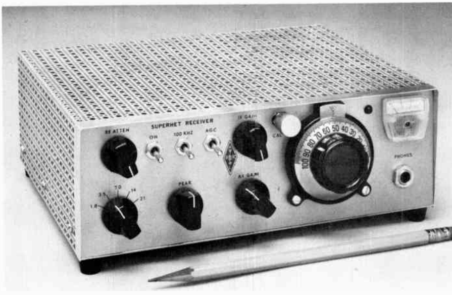
Fig. 58 — Photograph of the miniature 5-band superheterodyne receiver. This layout arrangement was developed by WA0UZO of Circuit Board Specialists.
