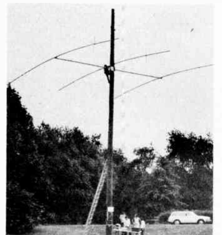
Fig. 50 — The shortened 40-meter Yagi beam closely approximates the size of a standard 20-meter Yagi. It is shown on a 60-foot (1.8-m) telephone pole.
