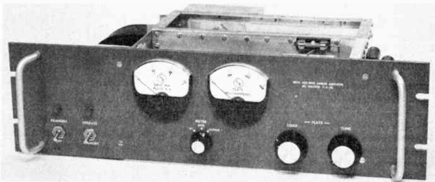
Fig. 44 — The high-power uhf amplifier. The toggle switches control filament power and stand-by/operate functions respectively. Multimeter function is selected with the switch located between the meters, while the plate tuning and loading controls are at the right. Modern knobs and homemade meter faces give the amplifier a commercial appearance.
