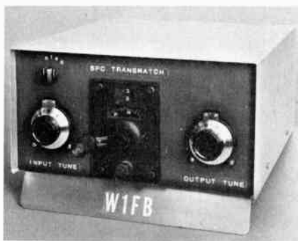
Fig. 22 — Exterior view of the SPC Transmatch. Radio Shack vernier drives are used for adjusting the tuning capacitors. A James Millen turns-counter drive is coupled to the rotary inductor. Green paint and green Dymo tape labels are used for panel decor. The cover is plain aluminum with a lightly grooved finish (sandpapered) which has been coated with clear lacquer. An aluminum foot holds the Transmatch at an easy access angle.
