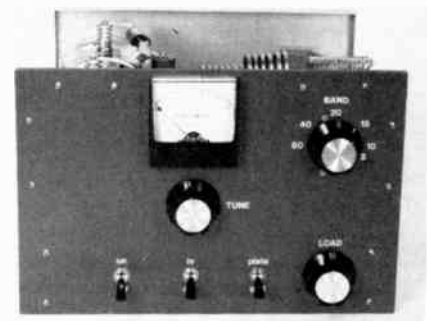
Fig. 75 — This is a photograph of the front panel of the 4-400A amplifier. The amplifier is relatively compact, measuring 10 x 14 x 10 inches (254 x 356 x 254 mm). The PEP input for this amplifier is 2 kW.
