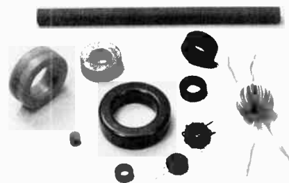
Fig. 45 — An assortment of toroid cores. A ferrite rod is placed at the top of the picture for comparison. The two light-colored, plastic-encased toroids at the upper left are tape-wound types (Hypersil steel) are suitable for audio and dc-to-dc converter transformers. The wound toroid at the right center contains two toroid cores which have been stacked atop one another to increase the power capability.
