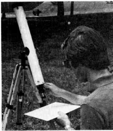
Fig. 2 — A simple sunspot projection system, demonstrated by ARRL staffer AC1Y. The cardboard baffle at the top provides a shaded area for viewing the sun's image. Sunspots large enough to affect radiowave propagation can be seen quite easily with this simple set-up. The best time to look for sunspots is the early morning.
