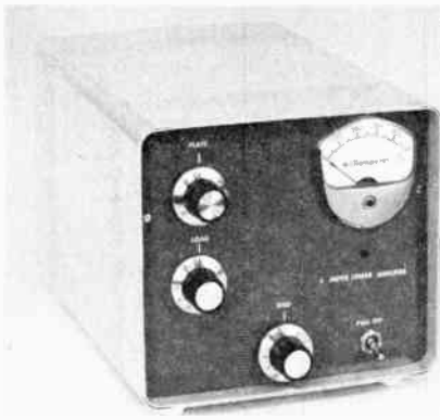
Fig. 11 — Designed and built by Dick Stevens, W1QWJ, this amplifier fills the need for a low-drive model usable with 10-watt exciters.
