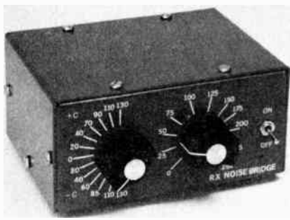
Fig. 66 — Exterior view of the noise bridge. The unit is finished in red enamel. Press-on lettering is used for the calibration marks.
