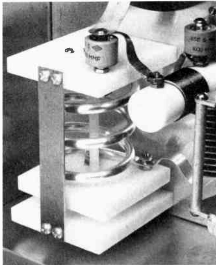
Fig. 20 — Photograph of the assembled adjustable inductor. Make certain to use only plated brass hardware for pieces that come into contact with the coil.
