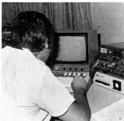
The modern RTTY position at W1AW. Note the neat order of equipment. This permits the operator to select all RTTY converter functions while tuning the transceiver. The proximity of the keyboard to transmit controls and the visibility of the equipment operating parameters (plate current and frequency) make for convenient operating. The required cw identification is accomplished by changing mode on the HAL keyboard at the end of transmissions. Many stations have an fsk identification technique that uses a very small shifting network across the keyboard contacts.
