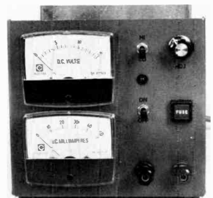
Fig. 38 — A simple 1.2- to 15-volt, 5-ampere power supply. All controls are mounted on the front panel for easy access. The milliammeter reading is multiplied by 100 to obtain the true output current.
