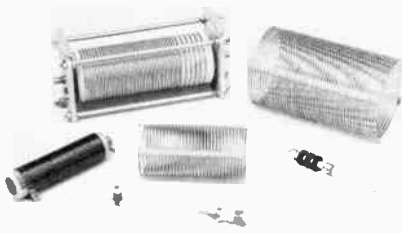
Fig. 18 — Assorted inductors. A rotary (continuously variable) coil is at the upper left. Slug-tuned inductors are visible in the lower foreground. An rf choke (three pi windings) is seen at the lower right.
