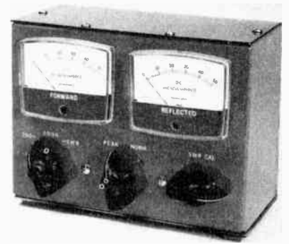
Fig. 62 — Front view of the 2-30 MHz rf wattmeter/VSWR indicator.
