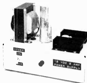
Fig. 31 — Exterior view of the 12-volt, 3-ampere, no-frills power supply.
