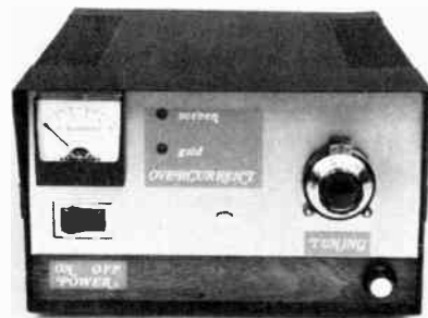
Fig. 25 — A 500-watt amplifier for the 2-meter band, complete with power supply, is housed in this cabinet. The hole plug covers a former location of a control.
