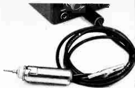
Fig. 19 — Rf probe for use with an electronic voltmeter. The case of the probe is constructed from a seven-pin ceramic tube socket and a 2-1/4-inch (57-mm) tube shield. A half-inch (13-mm) grommet at the top of the tube shield prevents the output lead from chafing. A flexible copper-braid grounding lead and alligator clip provide a low-inductance return path from the test circuit.
