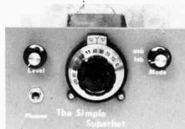
Fig. 52 — Outside view of the simple superhet receiver. The front and rear panels are made from double-sided circuit board.
