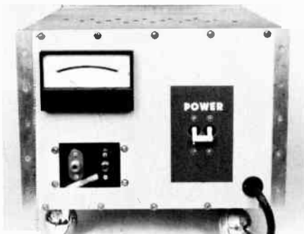
Fig. 46 — Front view of the heavy-duty, 3400-volt power supply.
