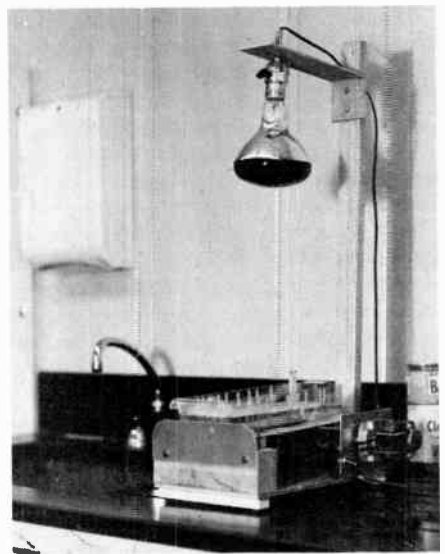
Fig. 15 — A homemade stand for processing etched-circuit boards. The heat lamp maintains the etchant-bath temperature between 90 and 115° F (32 and 46° C) and is mounted on an adjustable arm. The tray for the bath is raised and lowered at one end by the action of a motor-driven eccentric disc, providing the necessary agitation of the chemical solution. A darkroom thermometer monitors the temperature of the bath.
