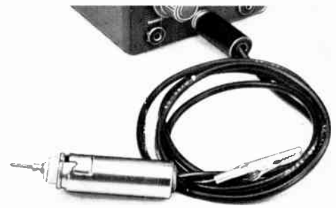
Fig. 19 — Rf probe for use with an electronic voltmeter. The case of the probe is constructed from a seven-pin ceramic tube socket and a 2-1/4-inch (57-mm) tube shield. A half-inch (13-mm) grommet at the top of the tube shield prevents the output lead from chafing. A flexible copper-braid grounding lead and alligator clip provide a low-inductance return path from the test circuit.
