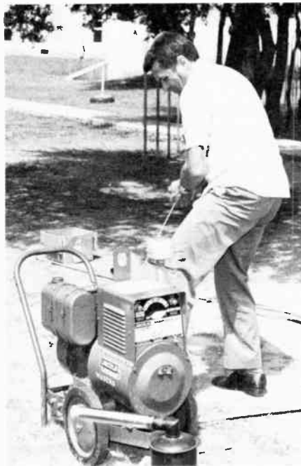
Fig. 5 — Gasoline-driven alternators are excellent as sources for 117 or 235 volts ac during field operations. In this picture is WB5YWQ yanking the starter rope of the WA5CXG power plant.
