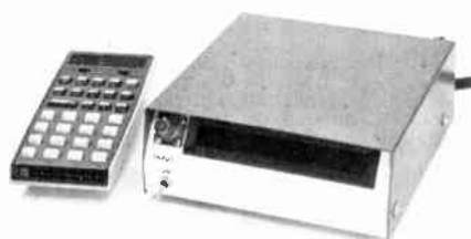
Fig. 30 — The counter is built into a homemade enclosure that measures 2 × 6 × 6 inches (50 × 153 × 153 mm).
