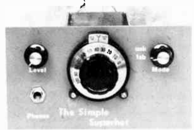
Fig. 52 — Outside view of the simple superhet receiver. The front and rear panels are made from double-sided circuit board.
