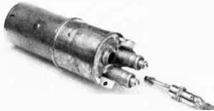
Fig. 6 — The automobile ignition coil should be shielded as shown here. A small tin can has been soldered to the metal coil case, and coaxial feed through capacitors have been soldered to the top of the can. The "hot" lead of the coil enters the shield can through a modified audio connector.
