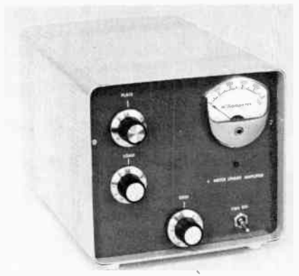
Fig. 37 — Designed and built by Dick Stevens, W1QWJ, this amplifier fills the need for a low-drive model usable with 10-watt exciters.
