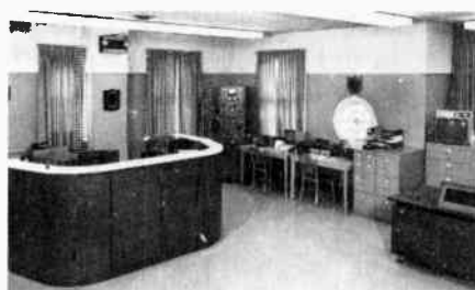
An overview of the W1AW station. The main operating console on the left houses the control equipment for simultaneous code practice/bulletins transmissions on eight bands. Two visitor operating positions are on the right.
