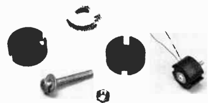
Fig. 46 — Breakaway view of a pot-core assembly (left) and an assembled pot core (right).
