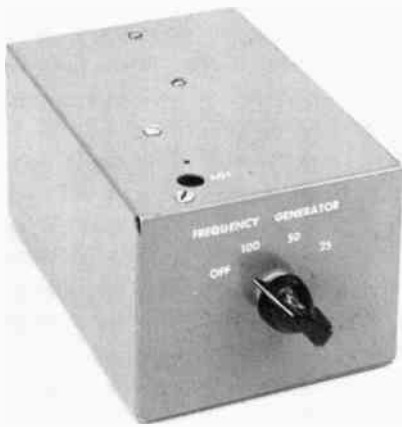
Fig. 26 — Frequency marker generating 100-, 50- or 25-kHz intervals. Battery power supply (two "D" cells) is inside the cabinet, a 3 × 4 × 6-inch (17 × 102 × 152 mm) aluminum chassis with bottom plate. The trimmer capacitor for fine adjustment of frequency is available through the hole in the top near the left front.
