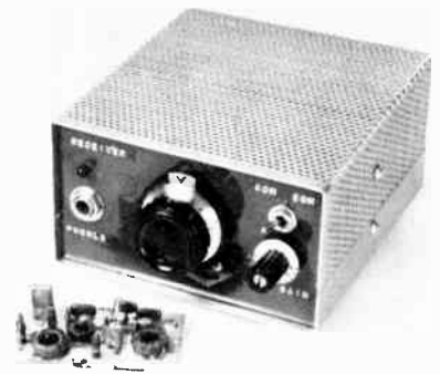
Fig 29 — Front view of the assembled 40-meter miniature receiver. A 20-meter converter is shown in the foreground. Pc boards and parts kits for this project are available from Circuit Board Specialists, Box 969, Pueblo, CO 81002. Boards and kits for a matching transmitter (May 1978 QST, page 16) are available from the same supplier.
