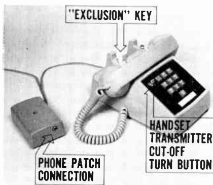
Fig. 35 — The voice coupler, to the left of the Touch-Tone telephone, is supplied by the telephone company. The coupler is normally fixed to a wall or desk, and contains a jack for connection of the amateur's phone patch.
