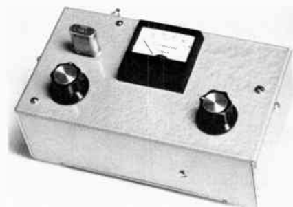
Fig. 63 — The deviation meter is constructed in a Calectro aluminum box. A four-position switch is at the lower right. The crystal plugs in on the left, with the frequency adjusting trimmer just below. A short whip or pickup wire can be plugged into the phono connector that is mounted on the back wall of the box.
