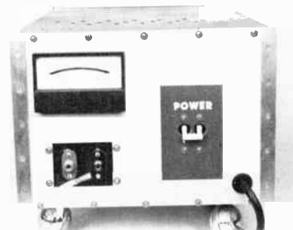
Fig. 40 — Front view of the heavy-duty, 3400-volt power supply.
