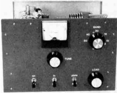
Fig. 78 — This is a photograph of the front panel of the 4-440A amplifier. The amplifier is relatively compact, measuring 10 × 14 × 10 inches (254 × 356 × 254 mm). The PEP input for this amplifier is 2 kW.
