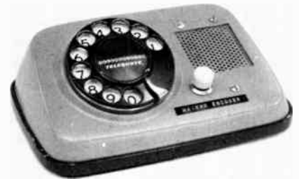
Fig. 57 — This dual-tone encoder is built in a surplus housing which was sold with the rotary dial no. TEL from John Meshna, P. O. Box 62, E. Lynn, MA 01904.
