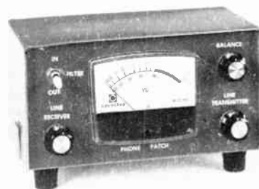
Fig. 37 — The phone patch unit is built into a homemade aluminum enclosure measuring 3 x 3 x 6 inches. A coating of spray-on enamel, rubber feet, and wet-transfer decal labels plus shiny knobs give the unit a professional appearance.
