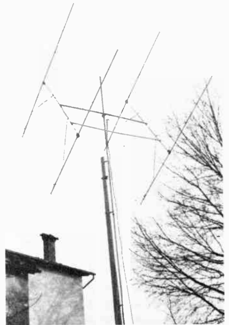
Fig. 16 — An efficient EME antenna system can be built around four long-boom Yagis like this setup at I4EAT.
