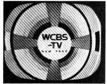
Fig. 3 — "Cross-hatching," caused by the beat between the picture carrier and an interfering signal inside the TV channel.
