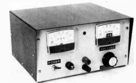
Fig. 34 — Front view of the 0-to 25-volt, 1.5-ampere power supply.
