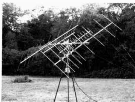
Fig. 11 — A circularly-polarized antenna system for satellite communications on 144 and 432-MHz. The array is assembled from KLM log-periodic yagis.
