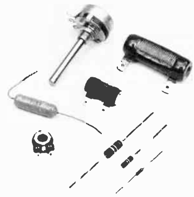
Fig. 7 — Examples of various resistors. In the foreground are 1/4-, 1/2- and 1-watt composition resistors. The three larger cylindrical components at the center are wirewound power resistors. The remaining two parts are variable resistors, pc-board mount at the lower left and panel mount at the upper center.
