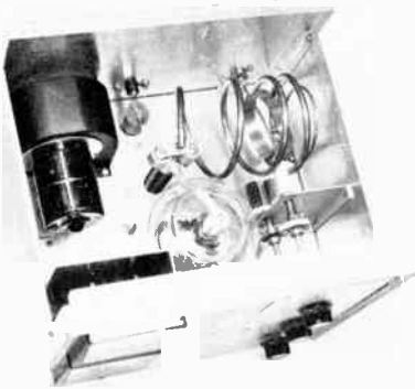
Fig. 23 — Interior view of the 50-MHz amplifier shows the shorted-turn tuning system, plate coil and output coupling, upper right. The tuning and loading controls are mounted on a bracket to the right of the 3-500Z tube and chimney. Meter shielding is partially visible in the left front corner.
