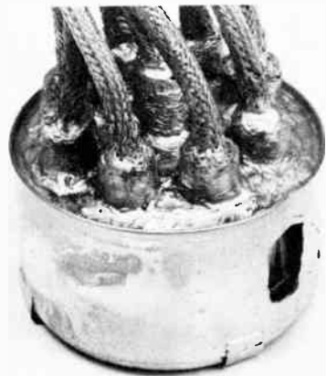
Fig. 4 — A close-up view of the distributor shield can. The shield braid over each spark-plug wire is soldered to the top of the can, and the can is grounded to the engine block.
