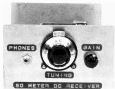
Fig. 49 — Front view of the beginners receiver. The panels are made from double-sided pc board material.
