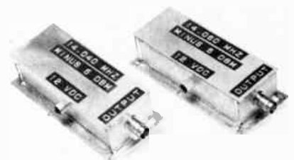
Fig. 65 — Exterior view of the two signal generators suitable for use in receiver performance measurements. Each uses an OE-10 oscillator available from International Crystal Mfg. Co., Inc.
