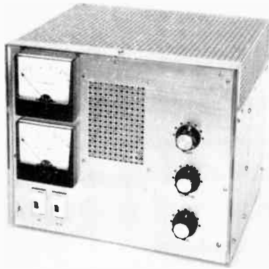
Fig. 22 — Table-top 50-MHz amplifier of grounded-grid design, only 10 × 12 inches (254 × 305 mm) in size. Grid and plate current are monitored simultaneously. Knobs at the right are for input tuning, bottom; amplifier loading, center; and plate tuning, top.
