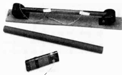
Fig. 47 — A bc-band ferrite rod loop antenna is at the top of the picture (J. W. Miller Co.) A blank ferrite rod is seen at the center and a flat bc-band ferrite loop antenna is in the lower foreground.
