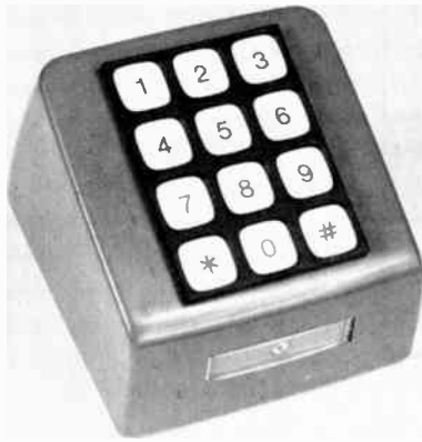
Fig. 50 — This homemade Touch-Tone generator is housed in a Western Electric sloping-front plastic box.
