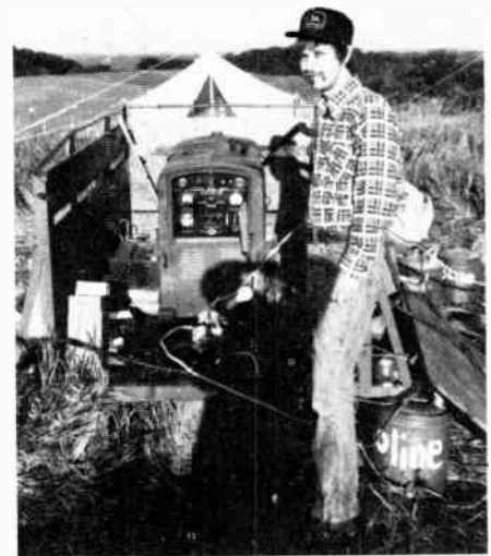
Fig. 12 — Large gasoline generators of the kW and higher class are excellent for powering several amateur stations from a complex field site. Maintenance, as discussed in the text, is a vital matter to ensure reliable operation. Here, WB9QPI has just finished a maintenance check of the group's Field Day power plant.
