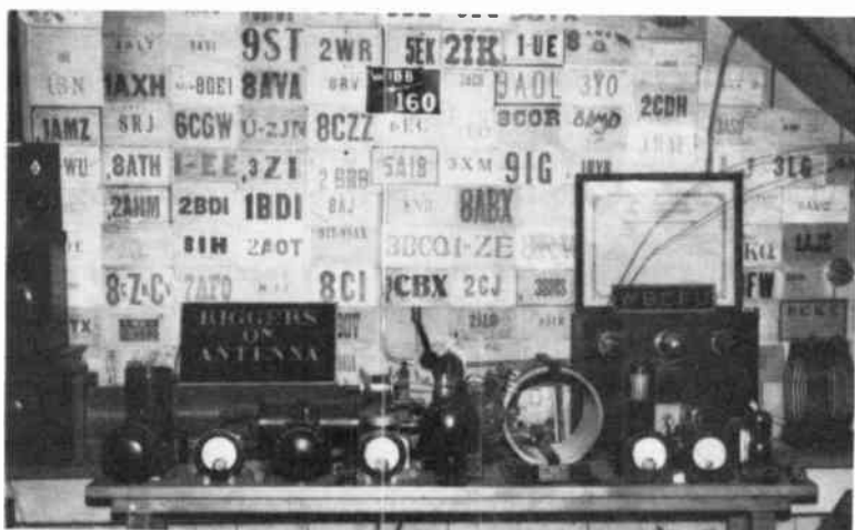
Early-1920's transmitter with a priceless collection of early QSL cards. R-F tube lineup is 202-202-203; modulator is 301-202-203. Antique Wireless Association Museum, Holcomb, N.Y.
