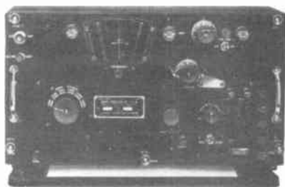
BC-312 RECEIVER AM-CW 12 VERSIONS VEHICLE, PORTABLE OR FIXED.
