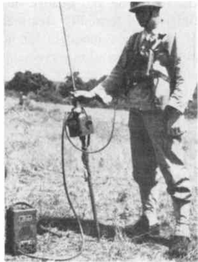
SCR-511, designed for cavalry in 1940, was the only light Walkie-Talkie when WW II broke out, and saw wide use by infantry.
