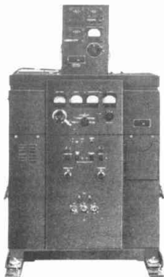
BC-610 TRANSMITTER WITH BC-939 ANTENNA TUNER. SIX VERSIONS.
