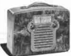
Model 37-G6—6 tube AC-DC or 1½ volt battery operated superhet with tuning range 540 to 1550 K. C.
