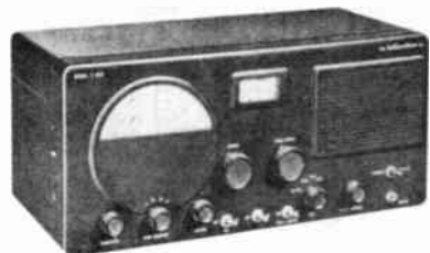
S-40B/S-77 S-40B is IMPROVED S-40 S-77 is AC-DC VERSION .54-44MC 8 TUBES $79.95 AUG '50 / DEC '50
