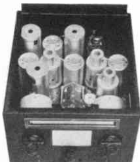
◇ AGS SUPERHET 2.4-15 MC 11 TUBES OCTOBER 1932 (AGS-X with crystal filter, AGU with single-unit plug-in coils, and AGL long-wave model all introduced July 1933)
