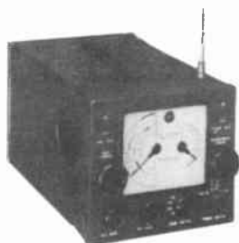
R-80 Receiver, showing design changes made on Hallicrafters S-29 Sky Ranger for military use. Used for troop information and entertainment. 9 tubes. AC-DC-BATT.
