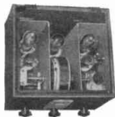
NC-5 S-W CONVERTER 15-185M 5 TUBES NOVEMBER 1931
