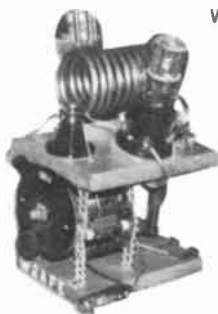
◇ UNITY-COUPLED PUSH-PULL CRYSTAL OSCILLATOR 80M 210's --45's W2AFE 1934 ARRL HND BK.
