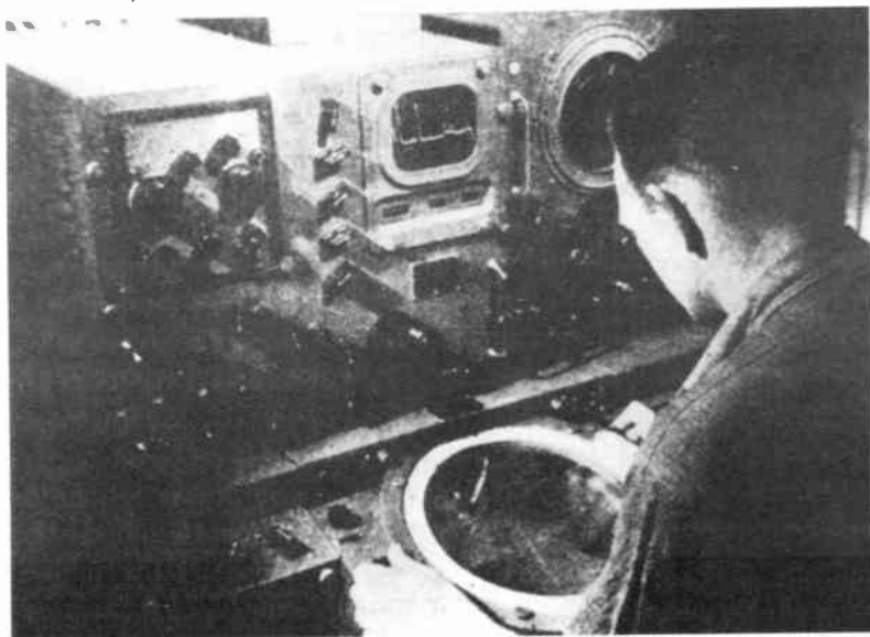
SC-2 air search radar for early warning of enemy air attack and for controlling friendly planes. 200-250 Mc. Larger version on aircraft carriers and battleships was the SK radar.
