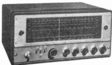
SX-62 .54-110MC 16 TUBES BUILT-IN FREQ. CALIBRATOR APRIL '49
