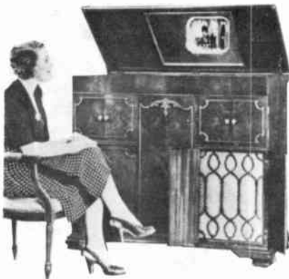
MODEL B-F-12 "SHARP-FOCUS" TV-RADIO-PHONO 43 TUBES 12" PICTURE ◊ 1939
