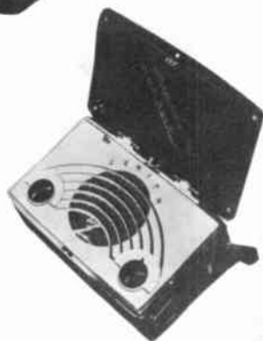
◇ 7G605 TRANS-OCEANIC (FIRST OF A QUALITY ALL-WAVE SERIES. McMILLAN USED PROTOTYPE IN ARTIC EXPLORATION) 7 TUBES AC-DC-BATT 1941
