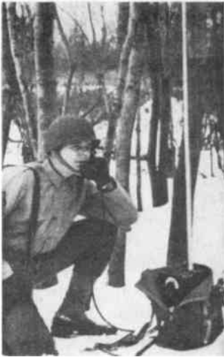
SCR-195 (infantry) and SCR-194 (field artillery) were the first Walkie-Talkies. brought out in 1936. SCR-195 is shown.
