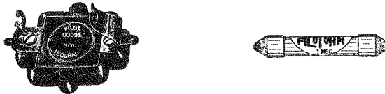
Fig. 238—Grid condenser with clips into which the grid leak resistor at the right may be snapped.
