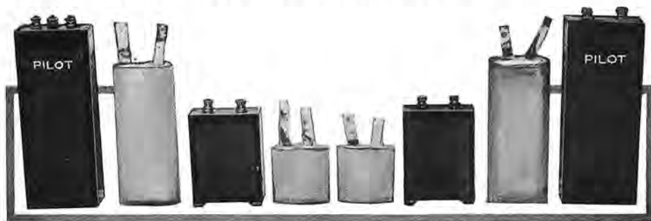
Fig. 91—A Group of Fixed Paper-type Condensers, showing the Wound Units before being sealed, and the completed Condensers in the Metal Cans. Notice the copper connection strips projecting from the tops.
