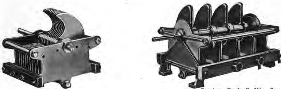
Fig. 86—Two Condensers which illustrate the effect of thickness of the Dielectric on the Breakdown Voltage of a Condenser. The Plates in the Radio Receiving Circuit Condenser at the left have a separation of .03 inches. The Breakdown Voltage is 1500 Volts. The Transmitter Condenser at the right has Plates separated .75 inches. Its Breakdown Voltage is 26,000 Volts.
