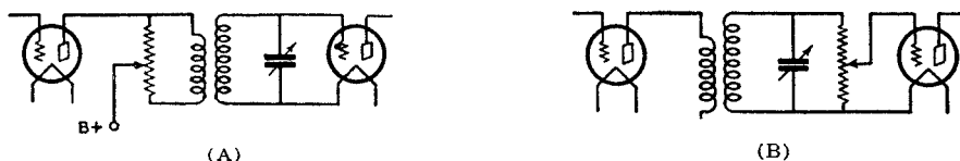
Fig. 271—(A) Volume control by means of a potentiometer connected in the plate circuit of an r-f amplifier tube. (B) Volume control by means of a potentiometer connected across the secondary of an r-f transformer.
