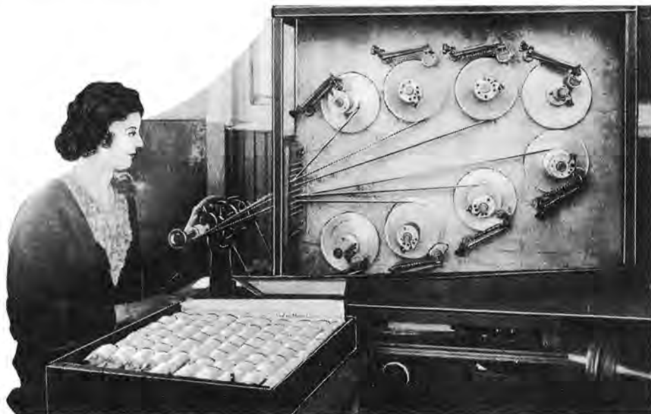
Fig. 89—Side View of a Condenser Winding Machine. The sheets of Paper Dielectric and Metal Foil Plates feed through the end of the dust-proof case on to the rotating mandrel. The Alternate Layers of Paper and Metal-Foil feed off from the rolls shown.
