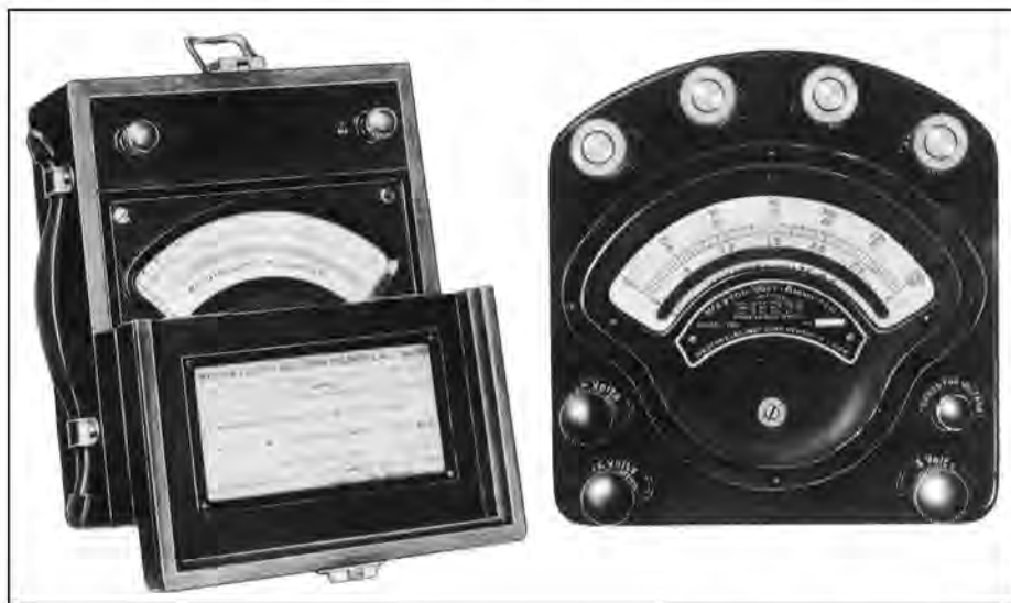
Fig. 139—A portable 0-2 thermo-milliammeter is shown at the left. At the right is a portable precision type d-c volt-ammeter having three current ranges and three voltage ranges. Its circuit diagram is shown in Fig. 145.
