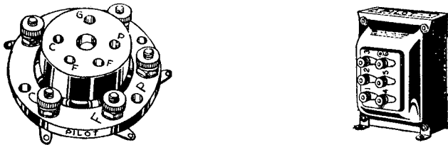
Fig. 222—Left: A 5-prong socket for separate heater type tubes. Right: A small transformer designed to deliver low-voltage a-c current for the filaments of a-c operated tubes.
