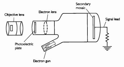
Figure 14. The Image Iconoscope
