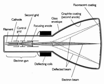
Figure 10. The Kinescope
