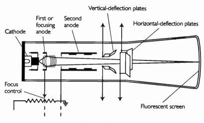
Figure 7. The Cathode-Ray Tube
