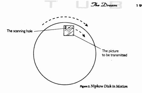
mitted by making the holes smaller and more numerous, each hole would allow even less light to come through, necessitating even greater illumination. Taken altogether, these problems called for a significant number of improvements to be made before any real results could be achieved.
