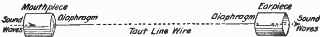
FIG. 11: An Acoustic Telephone. — The tension at both ends of the line wire bends the diaphragms outward from the cylindrical casings used for mouthpiece and earpiece.
