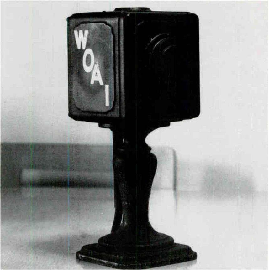
An original RCA Model 4-A-1 condenser microphone installed at WOAI, San Antonio, in December, 1929. Courtesy Hoxie Mundine
