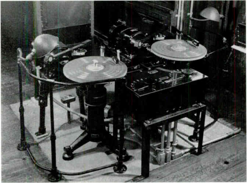
Two Western Electric vertical and lateral turntables installed at WOAI, San Antonio, in December, 1930. They played and “cut,” or recorded, radio programs to make electrical transcriptions (ETs). Years earlier these two machines had been the turntables that furnished sound for the first talking motion pictures. Courtesy Hoxie Mundine
