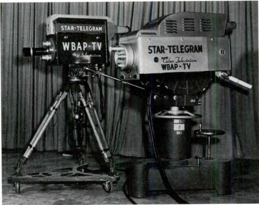
The cameras that helped establish television: WBAP-TV's RCA TK-10A, the predecessor to the TK-11, the workhorse of black-and-white television; and Channel 5's RCA TK-40A, the predecessor to the TK-41, the workhorse of color television. Courtesy KXAS-TV, Fort Worth, Texas
