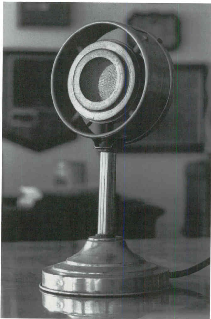
An original Western Electric Double Button carbon microphone first used at WJAD, Waco, in the early 1920s. Courtesy Robert E. Weathers, former owner, president, and general manager, WACO Radio Inc.
