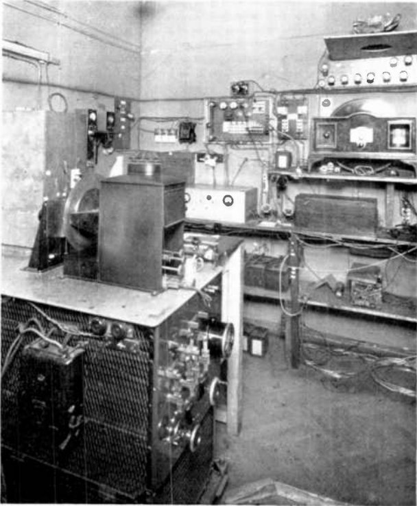
THE OLD CONTROL ROOM AT LONG ACRE FROM WHICH THE DAILY BROADCASTS OF BAIRD TELEVISION WERE SENT THROUGH TO THE B.B.C. THE PROJECTOR STAND IS SEEN ON THE LEFT
