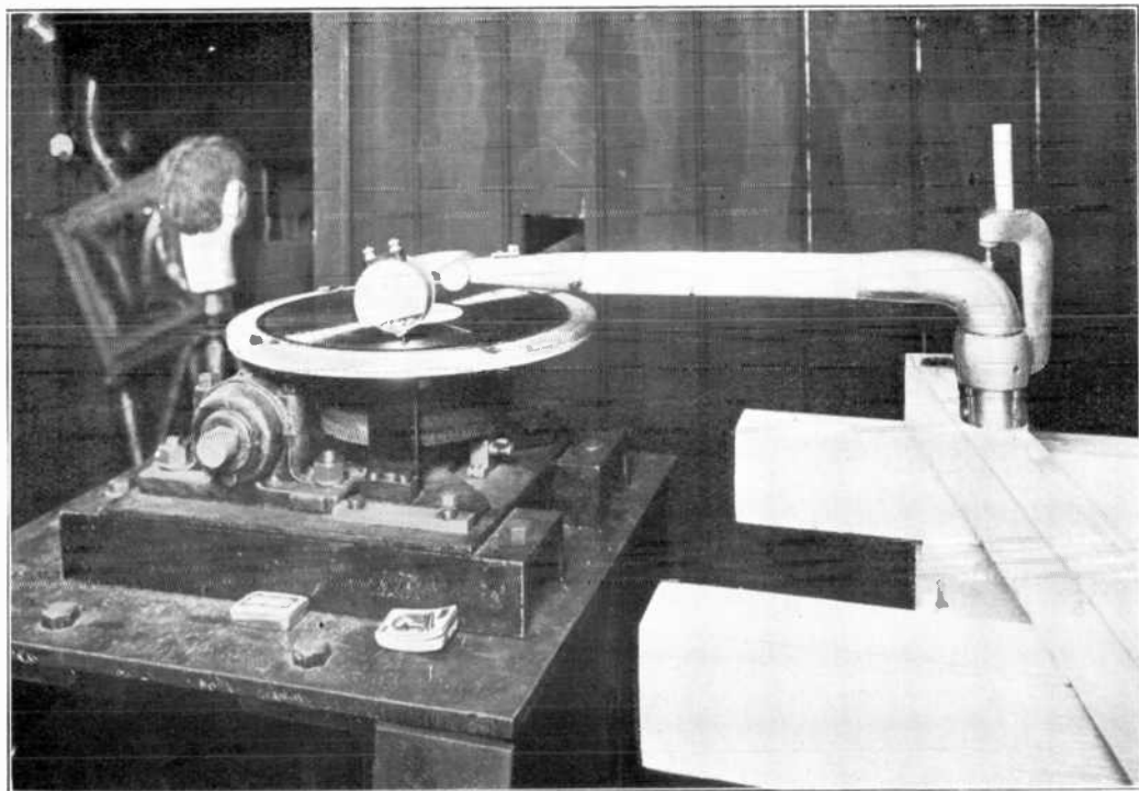
THE TRANSMITTING END OF THE PHONOVISION PROCESS RECORDING A DUMMY'S HEAD ON AN ORDINARY RECORD
