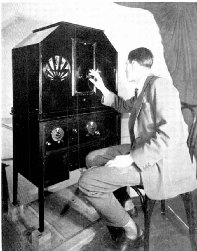
A BAIRD DUAL RECEIVER MODEL WHICH CONTAINS TWO RECEIVING SETS, ONE FOR SPEECH AND ONE FOR VISION
