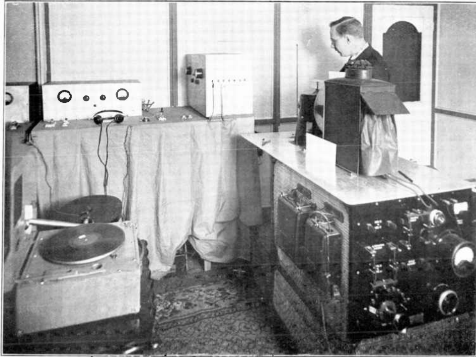
A PHOTOGRAPH OF A DISC TRANSMITTER WITH THE AMPLIFIER BOXES AND CONTROLS HOUSED ON AN ADJOINING TABLE
