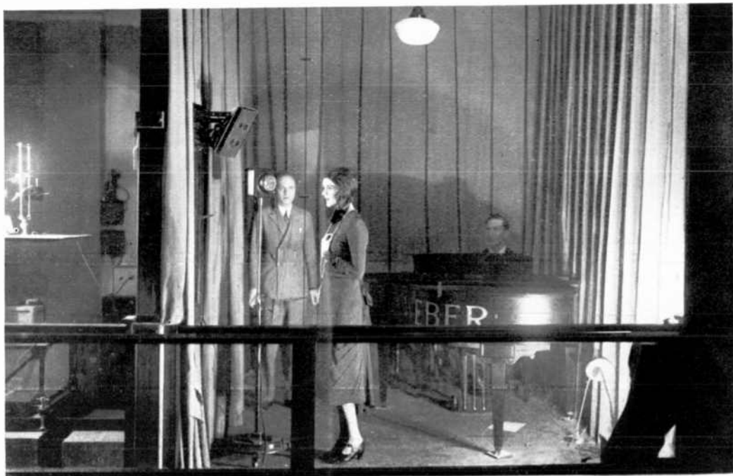
THE POSITION OF THE PHOTO-ELECTRIC CELLS IS CLEARLY SHOWN IN THIS EARLY PICTURE OF MISS JUNE COLLYER BEING TELEVISED AT THE STUDIO OF THE BAIRD TELEVISION CORPORATION OF AMERICA
