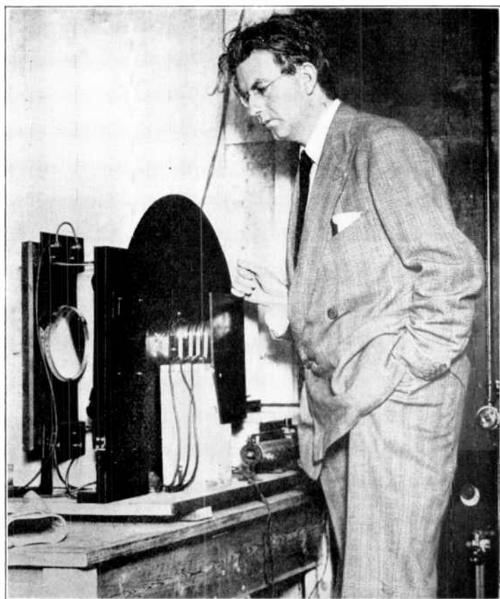
THE COMMUTATOR NECESSARY FOR CHANGING OVER TO EACH LIGHT SOURCE IN TURN IS CLEARLY SEEN IN THIS PHOTOGRAPH
