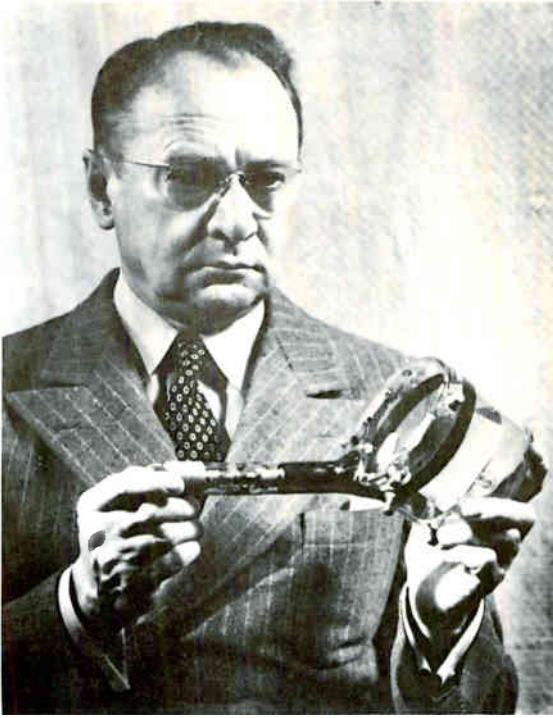
Dr. Vladimir Zworykin holding his iconoscope, the television pickup system he developed in the nineteen twenties for David Sarnoff. Courtesy RCA.
