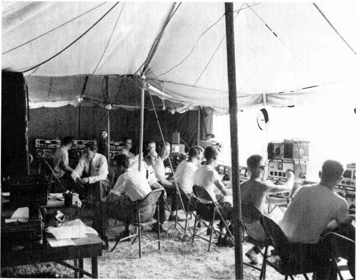
Above photo shows complex mobile coverage at Jamboree '55, the International Scout Rally. This was a good layout for multiple-language broadcasting. The CBC supplied technical know-how and equipment, and the visiting broadcasters did their own commentary. Events were recorded as they happened and the tracks were mixed with each language. CBC.
