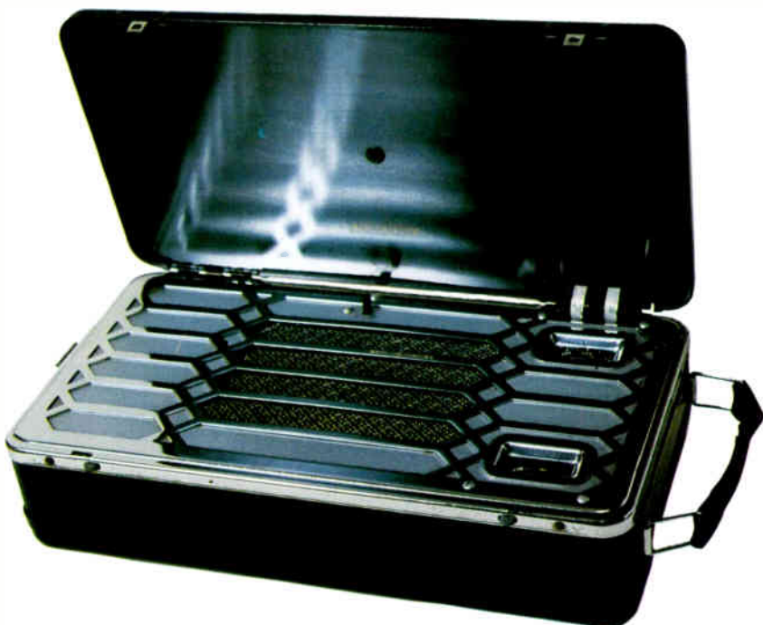
1947 British Marconiophone P17B four-valve battery personal portable in black plastic and chromium. 6.5cm x 22.8cm x 12.7cm (2½" x 9" x 5").
