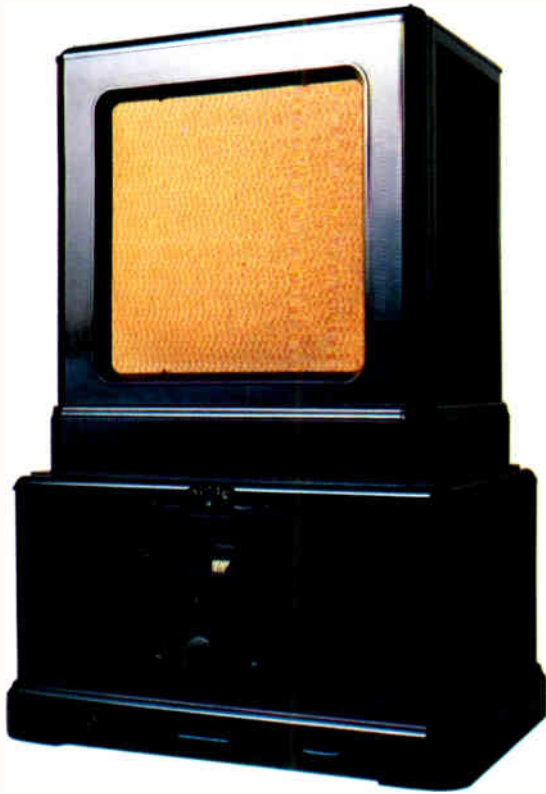
1950 Ekco British All Electric 315 two-valve mains receiver 20.5cm × 45.1cm × 22.8cm (8" × 17" × 9"), with matching moving-coil loudspeaker 41.9cm × 56.8cm × 20.5cm (16½" × 14½" × 8"), made of bakelite, but imitating the traditional wood cabinet style, rather than exploiting the design possibilities of plastic material.
