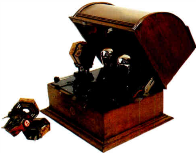
1926 British Edison-Bell Bijou two-valve battery receiver using plug-in coils to change waveband. Solid oak, ebonite panel and celluloid window in the lid, of similar design to one of the company's cabinets for a coin-slot phonograph. 27.9cm × 50.4cm × 25.4cm (11" × 12" × 10").
