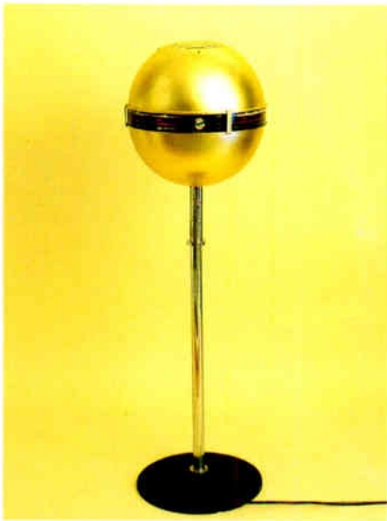
(Above) The Space Age did not officially begin until the launch of the Russian Sputnik in 1957, but the imagery of spaceships had begun to influence designers long before that. The British 1947 Emor Globe four-valve mains radio pictured here is a 50.4cm (12") diameter gold metal sphere on a 152.4cm (60") stand. It has no control knobs but is tuned by rotating the sphere.
