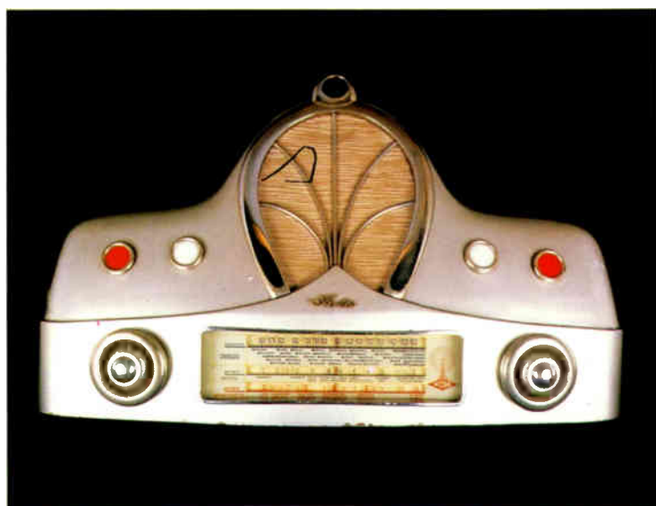
The automobile influence is evident in this plastic and chrome Spanish Artes AR-3 mains valve set of 1955. 51.7cm x 55.8cm x 26.6cm (12½" x 22" x 10½").
