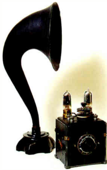
Polar Twin two-valve battery receiver with plug-in coils for changing wavelengths. Cabinet assembled from black crystalline-finish stamped panels clipped to a diecast skeleton. Shown here with a moulded ebonite loudspeaker. British. 1925. 15.2cm × 12.7cm × 12.7cm (6" × 5" × 5").
