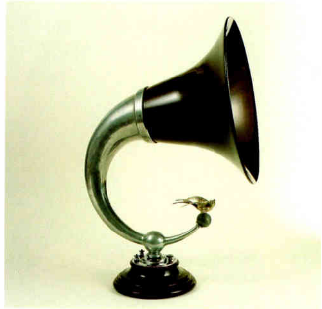
Brown's Q horn loudspeaker in aluminium with silver-plated bird ornament, turned wood base and flare in mahogany. British. 1924. 60.9cm (24") high with 35.5cm (14") flare.
