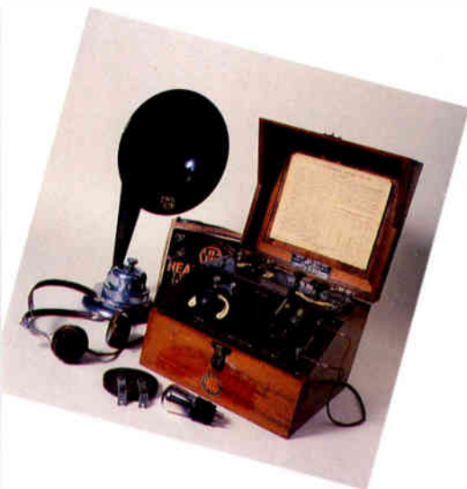
Stages in the evolution of the radio cabinet. (Left): The Wireless Set – a 1923 BTH crystal-valve receiver in solid walnut case 22.8cm × 29.2cm × 26.6cm (9" × 11½" × 10½"), with metal horn speaker 45.7cm (18") high. (Centre): The
