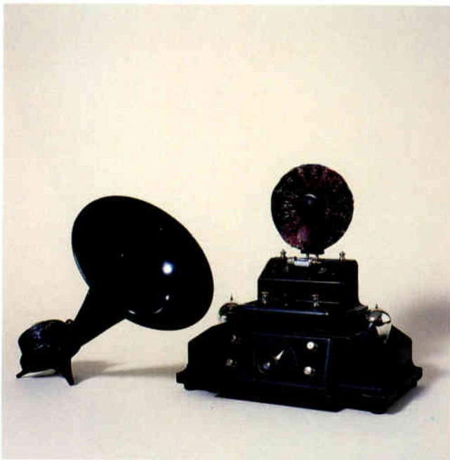
Brownie crystal set placed on top of its matching two-valve amplifier which made it capable of operating a loudspeaker instead of earphones. The moulded ebonite (vulcanized rubber) cases were mass-produced cheaply. 1925/6. 20.52cm × 29.5cm × 21.59cm (8" × 12" × 8½") (less coil).
