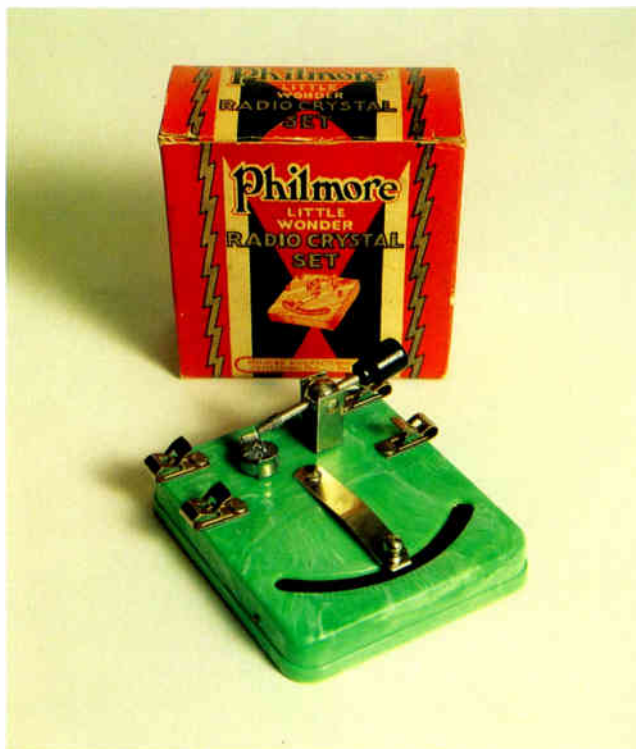
The American Philmore Little Wonder crystal set, manufactured between 1938 and 1945, might just as well have been made in the first few years of the Twenties. However, it distanced itself from the old 'instrument-look' by the use of mottled green plastic instead of black ebonite. 7.6cm x 8.2cm (5" x 3 1/4") base, 5.8cm (1 1/2") high.
