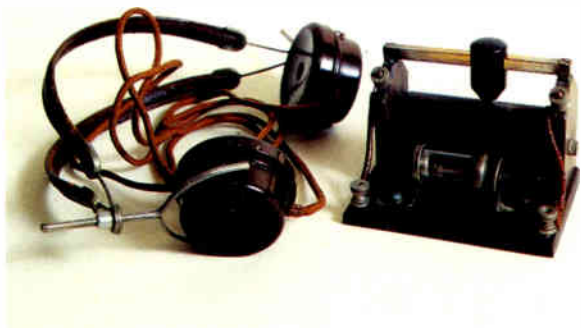
Miniature Wyncrystal receiver. Ebonite, brass and nickel, with cat's whisker-and-crystal and slide tuning. British. c. 1922. 10.7cm × 7.6cm × 7.6cm (4 1/4" × 3" × 3").
