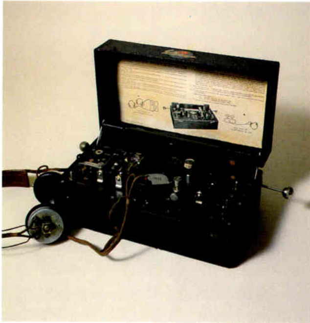
Marconiphone valve/crystal battery receiver RB10, tuned by sliding knobs at the sides and with plug-in coils to cover various wavebands. Really an amplified crystal-set but only capable of driving earphones. Imitation leather covered plywood box, ebonite panel and nickelled fittings. British. 1925. 15.5cm × 29.2cm × 15.8cm (5/4" × 11/2" × 6/4").
