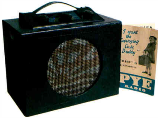
The 1958 British Pye Baby Q four-valve mains portable was produced in a blue leathercloth-covered plywood case with bakelite top-panel and the company's famous 'rising sun' logo behind the loudspeaker grille. 25.4cm × 50.4cm × 17.7cm (10" × 12" × 7").
