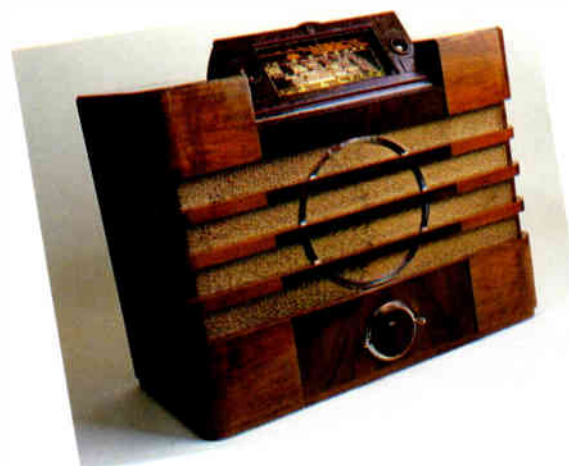
The British 1936 Philips five-valve Model 795A had a single control-knob which operated like a joystick. 45.1cm × 55.8cm × 27.9cm (17" × 22" × 11").
