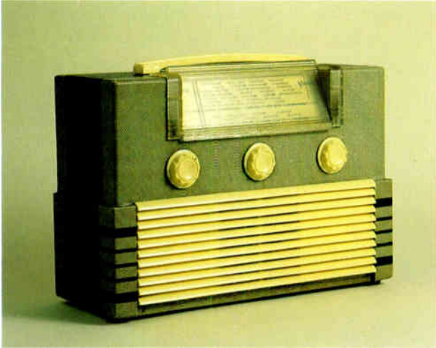
This British Vidor mains/battery four-valve portable of the Fifties in its cloth-covered wooden case 24.1cm × 33.5cm × 8.8cm (9½" × 14" × 3½") recycled the stepped design and louvres of the deco period.
