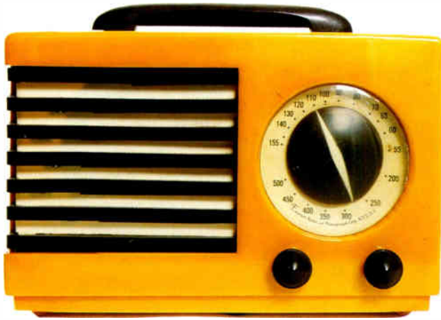
This American Emerson 400 midget main Aristocrat radio was produced in a variety of colour-combinations by the use of interchangeable sections, hand-cast in brilliant semi-transparent Catalin plastics. c. 1940. 20.5cm × 26.6cm × 12.7cm (8" × 10½" × 5").
