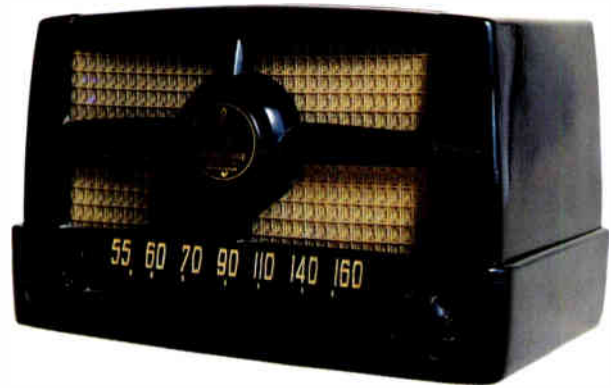
A cross between deco and automobile styling, this plastic Emerson mains valve radio of c. 1950 also makes a feature of its slide-rule style dial, borrowed from a dashboard speedometer of the day. 15.2cm × 22.8cm × 12.7cm (6" × 9" × 5").
