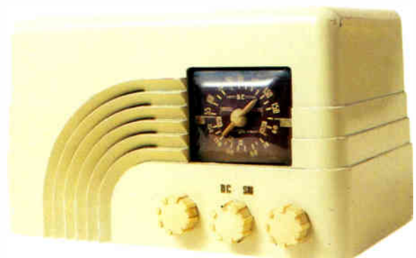
A deco Canadian Westrex midget mains radio, actually made in ordinary brown bakelite but marketed in several sprayed paint colours. c. 1940. 27.9cm x 17.7cm x 15.2cm (11" x 7" x 6").
