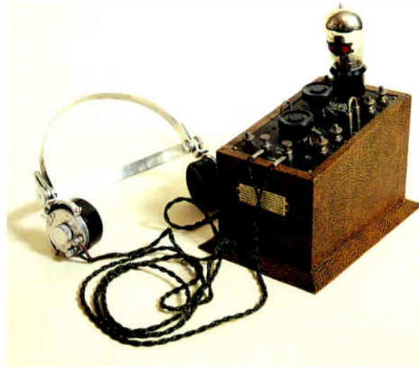
Fellows one-valve battery receiver suitable for earphone only use unless teamed with matching amplifier. Imitation leather case, ebonite panel and nickel fittings. British. 1925. 59.5cm × 15.9cm × 22.8cm (15½" × 5½" × 9").
