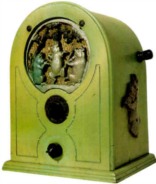
American Emerson Three Little Pigs four-valve mains receiver in green-painted bent plywood cabinet 22.8cm × 17.7cm × 12.7cm (9" × 7" × 5") with 'plastic wood' carving on the loudspeaker opening. 1951.
