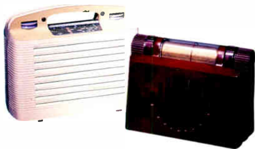
(Above) These small valve radios were typical of portables, often both battery and mains powered, of around the 1950s. Both are British and made by Murphy. The 144 of 1949 (left) is of cream-sprayed brown bakelite and the A100 of 1946 is of a later plastic.
