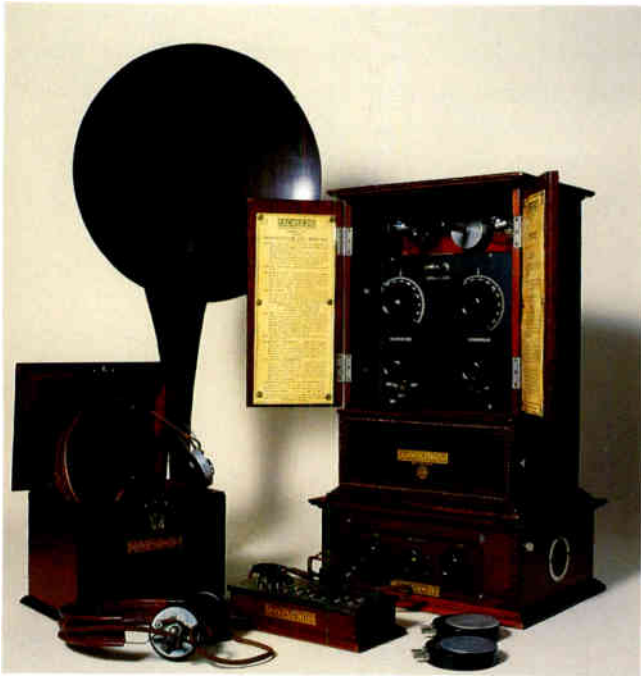
Large Gecophone battery set outfit, all in solid mahogany, comprising Smoker's Cabinet HF-Det set, matching amplifier, earphone box, distributor board and ebonite horn loudspeaker. British. 1922. 45.1cm × 50.4cm × 22.8cm (17" × 12" × 9").
