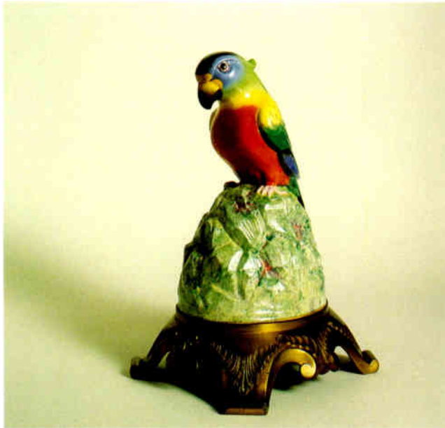
ArtAndia loudspeaker in the form of a parrot. Decorated china with ormolu base, made by Doulton potteries and concealing an Amplion drive-unit reflecting sound into an inverted cone and from beneath the base. British. 1927. 56.8cm (14½") high.
