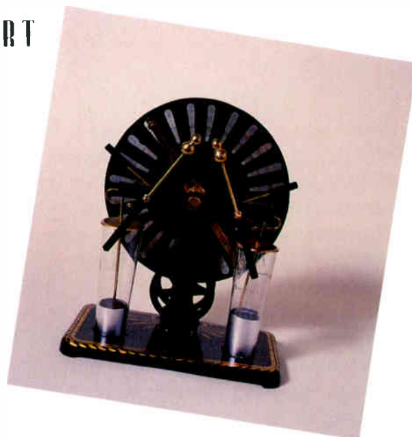
An ornate German Wimshurst machine c. 1890, an electrostatic induction generator – a kind of spark transmitter – although nobody had at the time devised a suitable receiver. 27.9cm × 22.8cm × 12.7cm (11" × 9" × 5").
