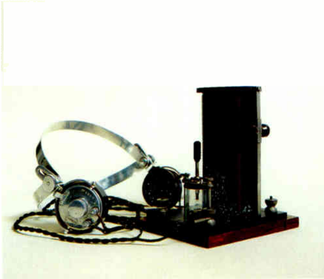
Crystal set sold by Gamages department store, London. Wood/ebonite base, nickel fittings, slide tuning. This simple earphone set needed a long aerial. British. 1923. 15.8cm × 12cm × 14.6cm (6¼" × 4¾" × 5¾").
