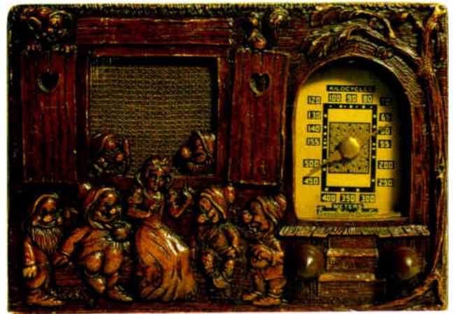
An imitation wood carving in a plastic material called 'repwood' was used for this American Emerson Snow White and the Seven Dwarfs main radio, intended to exploit the children's market. 17.7cm × 27.9cm × 15.2cm (7½" × 11" × 6").
