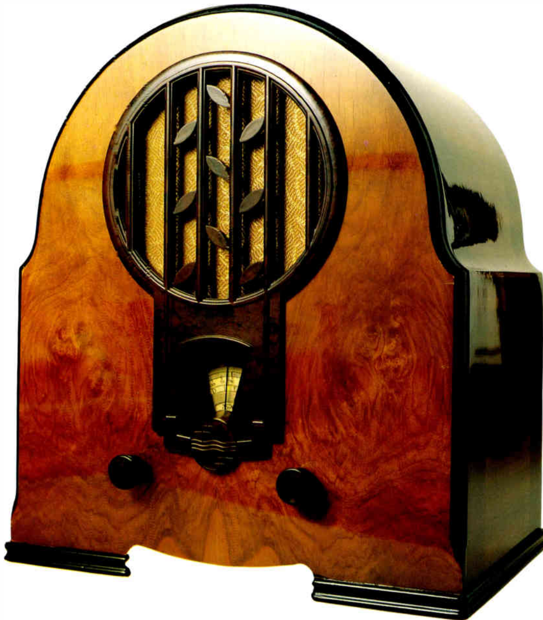
Philips Superinductance 634A five-valve mains receiver in bent walnut plywood case with bakelite decoration. Technologically a dinosaur, it used a TRF circuit at a time when the much better Superhetrodyne was being universally adopted. British. 1955. 48.2cm × 40.6cm × 26.6cm (19" × 16" × 10½").
