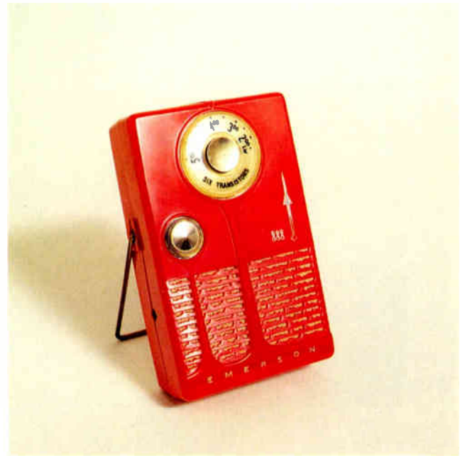
A Sixties American Emerson six-transistor radio in a decorative plastic case with folding stand.
