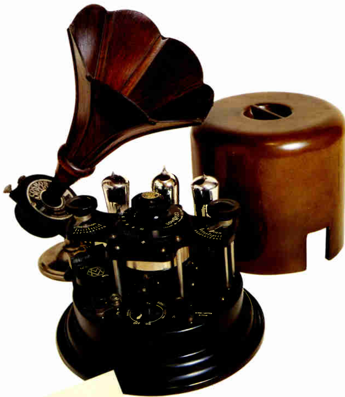
Met-Vick Cosmos three-valve battery set with plug-in waverange coils and matching oak-horned loudspeaker. Moulded in black ebonite, the set had a cover to keep dust out when not in use. British. 1925. 22.8cm (9") high × 24.1cm (9½") diameter.
