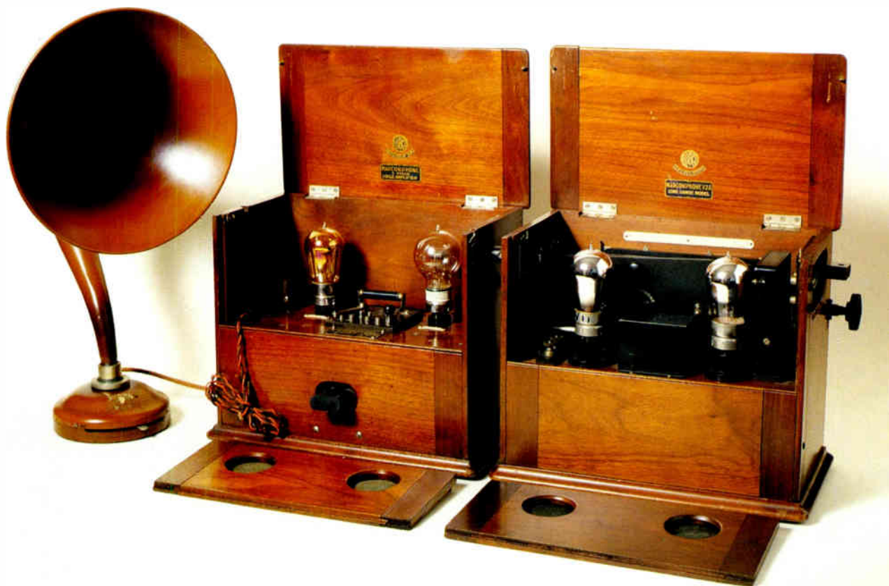
One of the first commercial valve receivers to appear on the British market was the Marconiphone V2 of 1922. The one pictured (right) is a slightly later model. It had plug-in coils for different wavebands and is shown here with matching amplifier for use with a loudspeaker (here a Sterling). Battery operated. Solid walnut cabinets. 26.6cm x 55cm x 20.3cm (10½" x 15" x 8").
