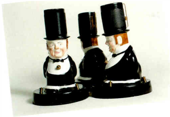
Uncle Tom Grafton china crystal sets, British made in 1924. A coil is wound on the top hat, the cat's whisker protrudes from the bow tie and the crystal is a diamond stud on the shirt-front. 22.8cm (9") high.
