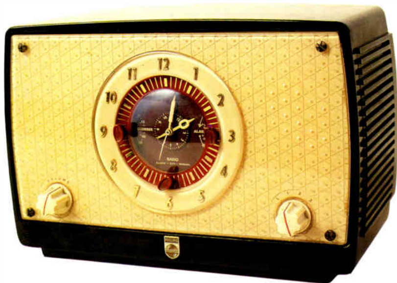
Several manufacturers produced mains valve clock-radios in the mid-Fifties, intended for bedrooms. They looked like the conventional cabinets of the period but stations were switched-in so that tuning-dials could be omitted and replaced by clock dials. The plastic-cased British Philips of 1954, which had the increasingly popular television-screen shape, is illustrated. 20.5cm x 51.7cm x 15.2cm (8" x 12½" x 6").
