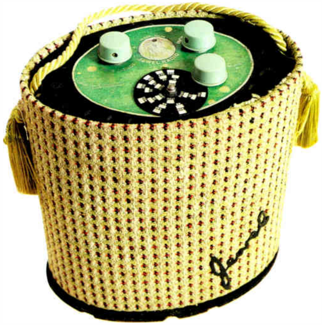
The 1957 British Jewel four-valve handbag radio had a fibre case covered in furnishing fabric with a tasselled handle. It bears a medallion depicting a girl with an illuminated 'jewel' in her hair. For the fashionable young lady on the move, it worked from the car cigarette lighter socket as well as from internal batteries. 22.8cm × 20.5cm × 12.7cm (9" × 8" × 5").
