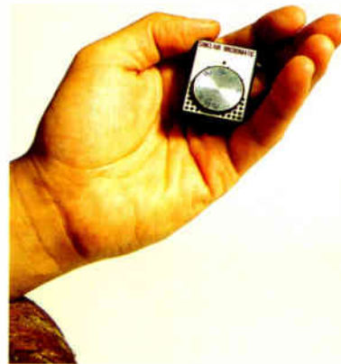
Marketed as 'Britain's smallest radio' in 1960; the Sinclair Micromatic was smaller than a matchbox, could be built from a DIY kit and was powered by a tiny hearing-aid battery, but would only work an earphone. 4.4cm × 5.1cm × 1.27cm (1¾" × 1¼" × ½").
