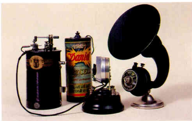
A tubular Brownie crystal set of 1924 with a Wilson Magnetic Bar amplifier (1925), and an Amplion Dragonfly horn loudspeaker (1924). British. Set 16.5cm (6½") high.
