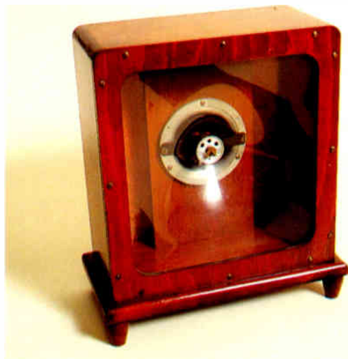
Moving-iron loudspeaker in plywood case with transparent membrane to radiate sound. Probably German. c. 1926. 22.8cm × 17.7cm × 12.7cm (9" × 7" × 5").
