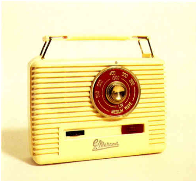
The 1957 British Marconi P60B (also HMV 1410G) used a combination of two of the old-fashioned valves and two of the new transistors. 15.2cm x 19cm x 7.6cm (6" x 7½" x 3").
