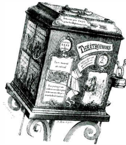
Théâtrophone coin-box which enabled the listener to choose from various relays from theatres.
