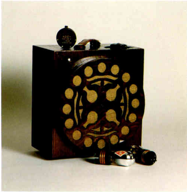
1951 British Adey four-valve battery portable radio with internal frame aerial and patent plug-in key. This performed various functions including prevention of unauthorized use. Walnut plywood. 25.4cm × 25.4cm × 17.7cm (10" × 10" × 7").
