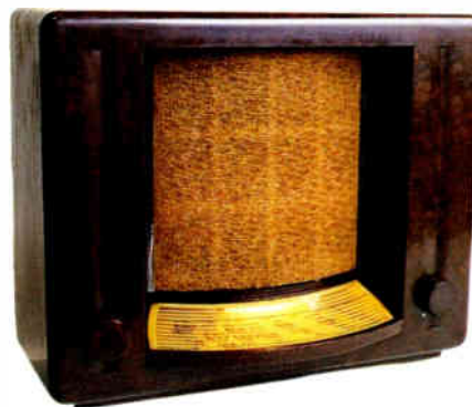
To fight price competition in 1956, Philips produced this V5A receiver without a conventional metal chassis. The 'works' were assembled in the form of a loom of wire and components which were then coiled-up into the one-piece bakelite cabinet. Four-valve. British. 54.2cm × 45.1cm × 26.5cm (15½" × 17" × 8").
