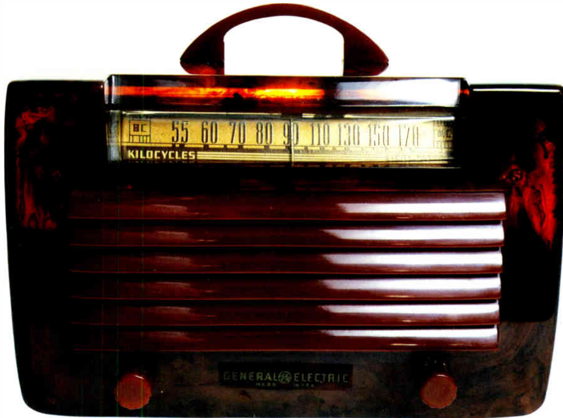
(Above) Craftsmen swirled colours into liquid Catalin plastic to produce the beautiful translucent tortoiseshell cabinet for this American GEC 1941 mains radio. 15.2cm × 24.1cm × 15.2cm (6" × 9½" × 6").
