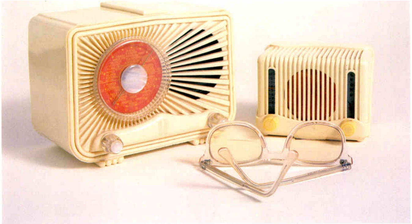
Two plastic-cased mains battery radios from the Fifties. The five-valve model on the left is by Madrid Radio and measures 12.7cm x 17.7cm x 8.8cm (5" x 7" x 3½"). The tiny one is the Gnomo by Era of Milan and was probably one of the smallest mains radios ever made, at 8.2cm x 10.9cm x 6.9cm (3¼" x 4¾" x 2¾").
