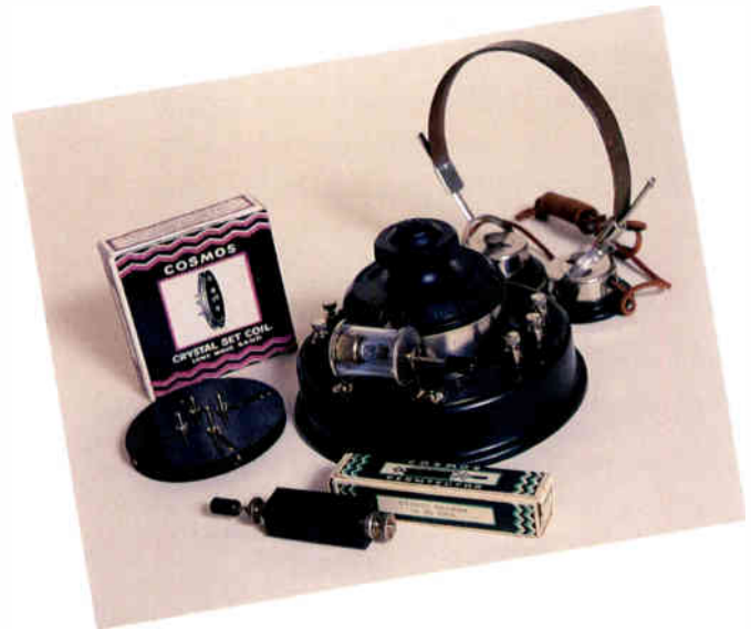
A crystal set of the early 1920s: it is called the Cosmos but the listener would have been unlikely to detect more than a local station, even with a 100-foot aerial. British made. 16.5cm (6½") diameter.
