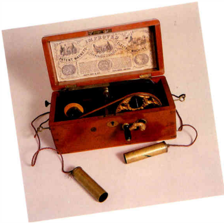
Improved Patent Magneto-Electric Machine c. 1890 in mahogany and brass, its driving wheel imitating a gold chariot wheel. Such 'shock machines' were promoted as magical cure-alls by late nineteenth-century medical men. If the machine is placed close to a radio receiver, turning the handle transmits sparking noises, showing that it actually produced wireless waves. 12.7cm x 25.4cm x 12.7cm (5" x 10" x 5").
