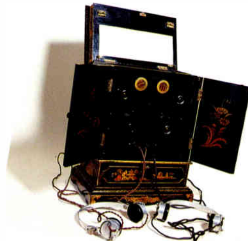
The interior of a two-valve set made by Sterling Telephone and Electric Company. It could operate two pairs of earphones but was not powerful enough to drive a loudspeaker.
