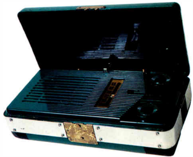
American Emerson 'handbag style' four-valve battery portable c. 1947. Approx. 6.5cm x 22.8cm x 12.7cm (2½" x 9" x 5").
