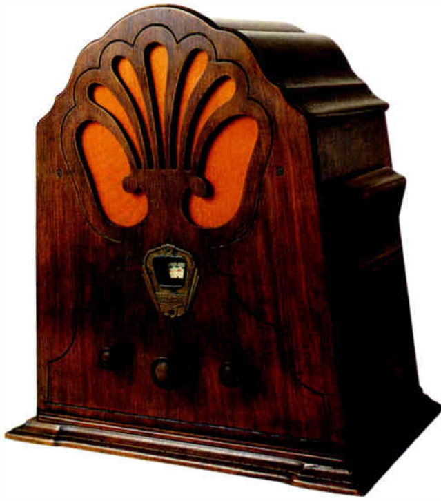
Ultra Tiger three-valve mains receiver with walnut-stained case built up from plywood and solid wood; bronze dial. British. 1951. 45.1cm × 40.6cm × 21.5cm (17" × 16" × 8½").
