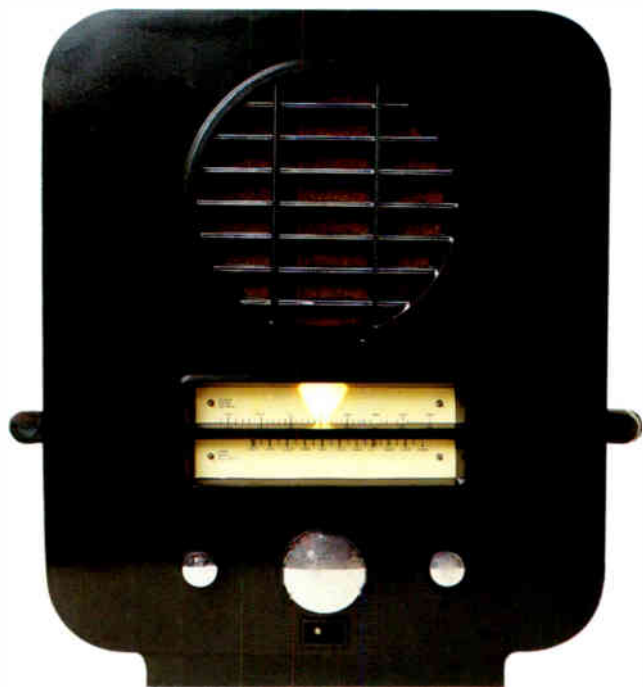
The Eico model AC7A four-valve mains receiver in Serge Chermayeff's 1955 cabinet. In black bakelite and chromium with a light-beam tuning indicator, it was obviously influenced by the semi-anthropomorphic robot designs of the day, and is a celebration of the Machine Age and the fast-developing technology of electronic communication. At a time when the general public still seemed to prefer decorative wooden cabinets which fitted in with their furniture, it was startlingly innovative, but outwld by a cheaper toned-down brown bakelite version that imitated real wood. 45.7cm x 58.1cm x 25.4cm (18" x 15" x 10").
