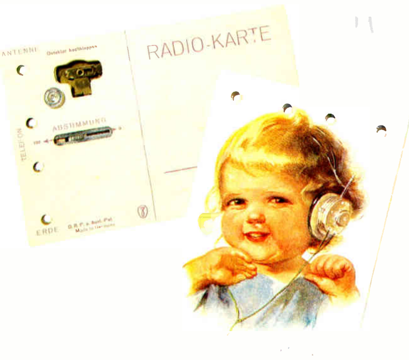
A 1922 postcard crystal set which appeared with a variety of picture fronts. Made by both German and English firms, it is 0.5cm (1/8") thick and contains a slider-tuned coil sandwiched between cards. It works with a good aerial, but nowadays brings in several stations on top of each other.
