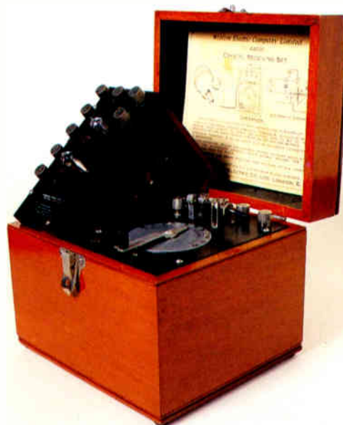
Western Electric crystal set, also sold as the Met-Vick Cosmos which operated only earphones unless a Weconomy amplifier was slotted into the compartment normally provided for earphones, when it would work a born loudspeaker. Mahogany. British. 1922/3. 17.7cm x 21.5cm x 19cm (7" x 8 1/2" x 7 1/2").
