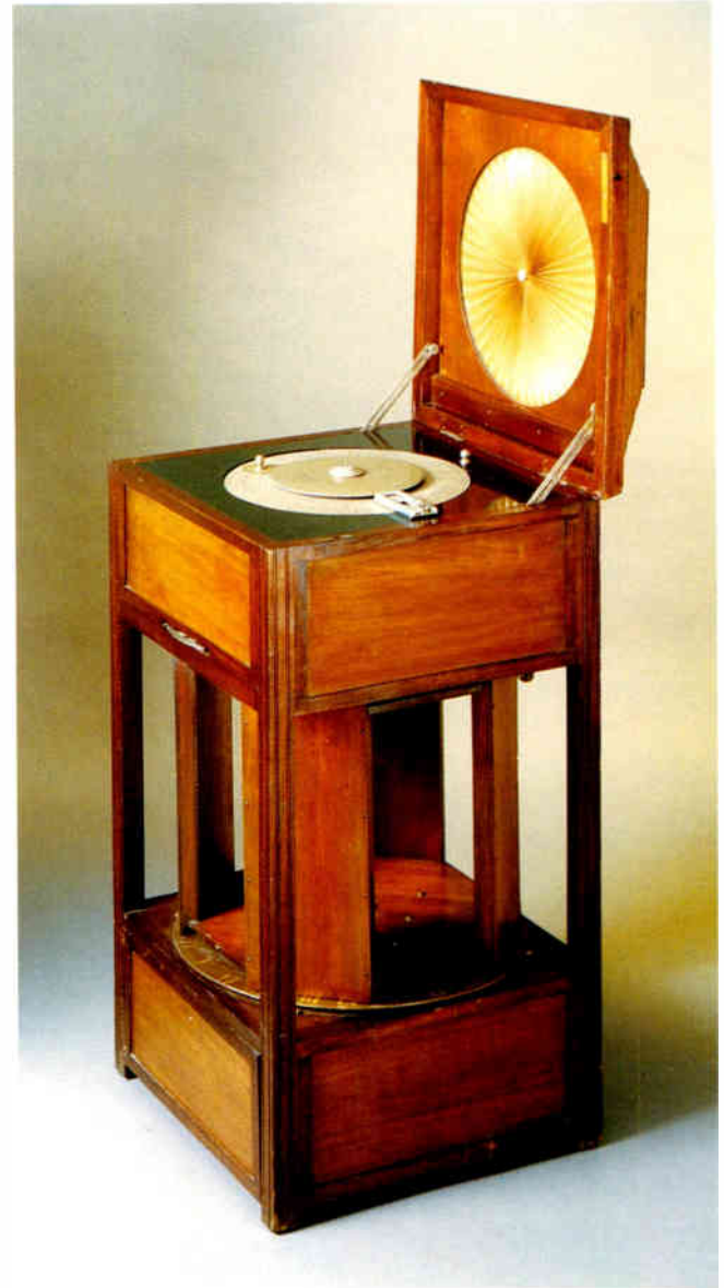
Gaumont Elgédynes six-valve grand luxe battery receiver in a walnut stand fitted with a rotatable frame aerial. In the lid is a moving-iron loudspeaker with a pleated-paper cone. French. 1928. 119.3cm × 50.8cm × 50.8cm (47" × 20" × 20").
