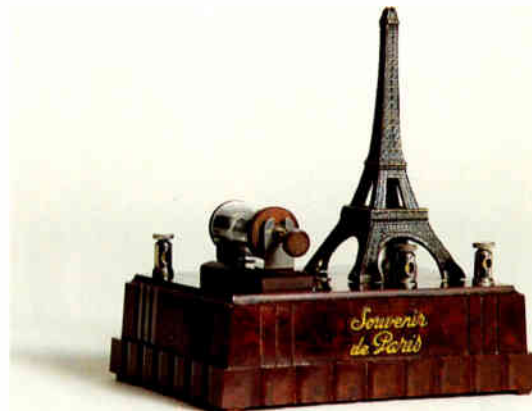
French crystal set, c. 1925, with sliding-plate tuning and glass-enclosed crystal and cat's whisker. The diecast metal model of the Eiffel Tower mounted on the bakelite base is just an ornament to enhance its attractiveness as a souvenir from Paris. 11.4cm × 10.1cm × 7.6cm (4½" × 4" × 5").
