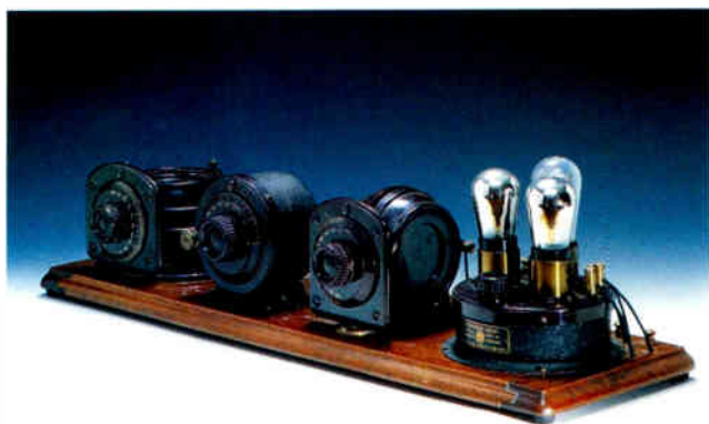
Atwater-Kent Breadboard, the Meccano set of American radio, consisting of separate units which can be assembled in various combinations on a simple wooden board to construct a variety of different receivers. American. 1924.
