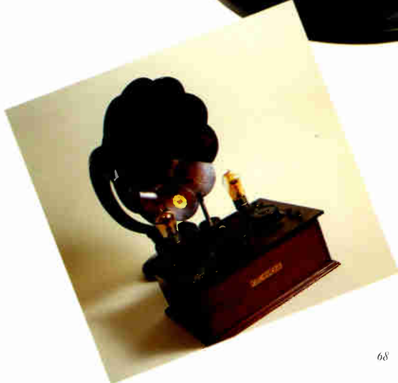
Met-Vick Cosmos three-valve battery set with plug-in waverange coils and matching oak-horned loudspeaker. Moulded in black ebonite, the set had a cover to keep dust out when not in use. British. 1925. 22.8cm (9") high × 24.1cm (9½") diameter.
