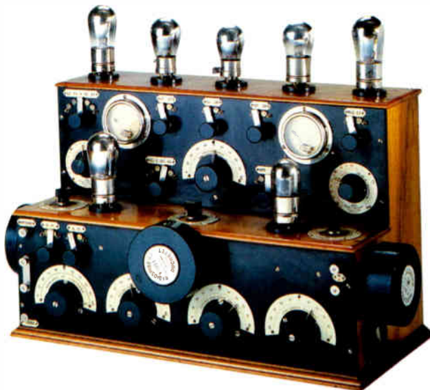
Ducretet F seven-valve receiver, usually supplied with a frame aerial and horn loudspeaker. Walnut cabinet with ebonite (imitation ebony) front panel and nickel-plated fittings. French. c. 1925.
