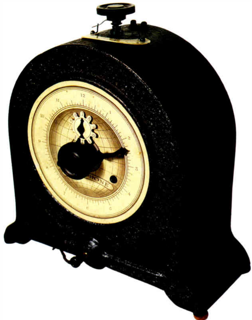
British Europhone two-valve battery receiver in the form of a mantel clock: black crystalline finish, pressed metal case with wood base, and imitation ivory dial. 1928. A separate loudspeaker had to be connected to enable it to work. 27.9cm × 25.4cm × 11.4cm (11" × 10" × 4½").
