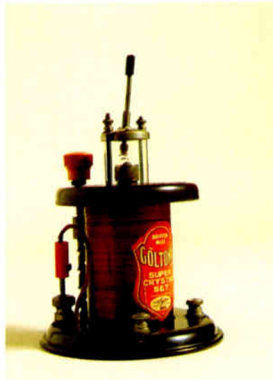
Goldtone crystal set with spiral-shaft tuning device and cat's whisker on top. Red bakelite. British. 1924. 15.2cm x 10.16cm (6" x 4") diameter.
