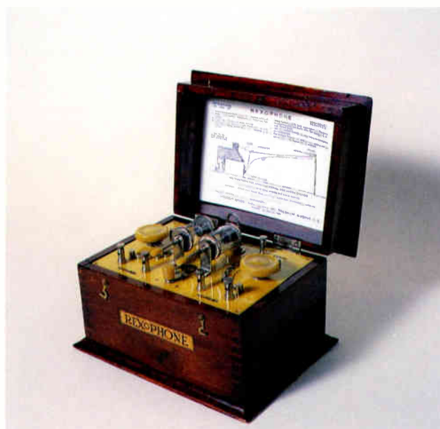
Rexophone crystal set with unusual top panel in the plastic Xylonite which imitated onyx. Two separate crystal-and-cat's whisker detectors were set before listening in, so that if one failed, the other could be selected. Solid mahogany, nickel and gold fittings. British. 1923. 15.2cm x 22.8cm x 12.7cm (6" x 9" x 5").
