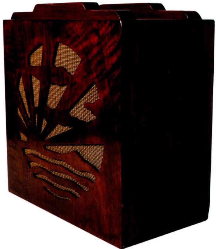
British Pye Q four-valve portable battery receiver with internal frame aerial. The solid walnut and plywood case bears the 'rising sun' motif, first used in 1927. 44.4cm × 40.6cm × 24.1cm (17½" × 16" × 9½").
