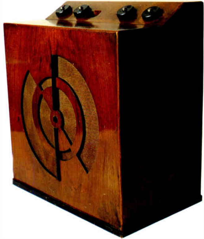
Murphy B4 four-valve portable battery receiver in a mahogany cabinet with a geometric loudspeaker-fret design. British. 1952. 45.1cm × 58.1cm × 22.8cm (17" × 15" × 9").
