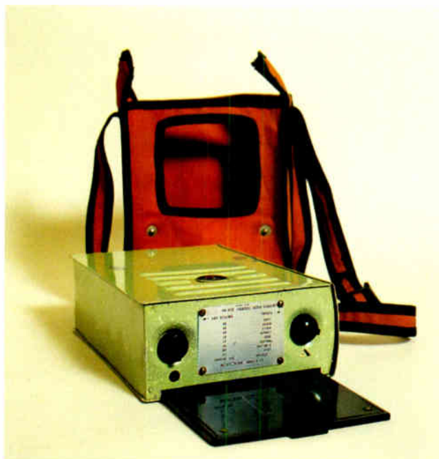
The British Hermes Radio Tourist battery valve portable of 1947 was made of sprayed metal in the shape of a book, 21.5cm x 15.2cm x 7.6cm (8½" x 6" x 3"), and supplied with a canvas satchel.
