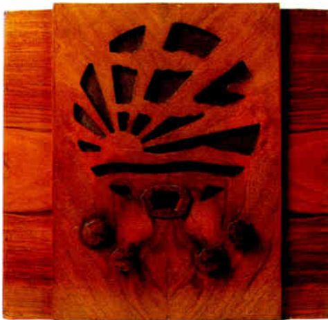
A 1932 walnut-cased three-valve mains receiver by the British Pye firm. 59.5cm x 40.6cm x 19cm (15½" x 16" x 7½").
