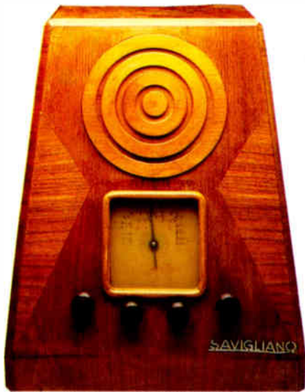
The 1958 Italian Savigliano type 93 mains five-valve receiver in wooden cabinet with contrasting veneers, that was considered very modern in its day.
