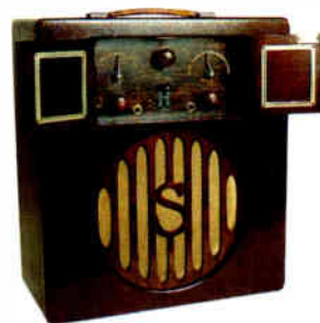
British-made Selecta four-valve portable of 1929 – typical of the heavy, bulky portables intended for car picnics then in fashion.
