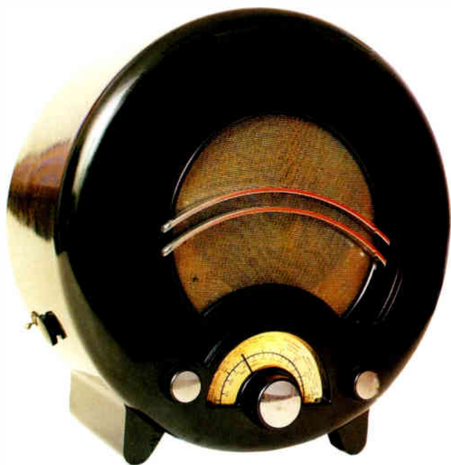
The 1955 Ekco AD36 black-and-chrome mains three-valve radio – a variation in the circular model range. 56.8cm (14½") diameter.
