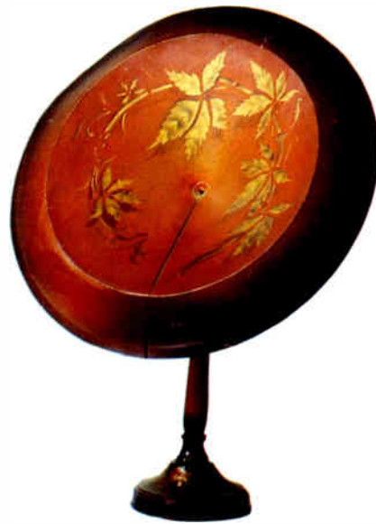
(Above) Moving-iron loudspeaker by Sterling on turned wooden stand with painted cone. British. 1926. 35.5cm (14") diameter × 50.8cm (20") high.
