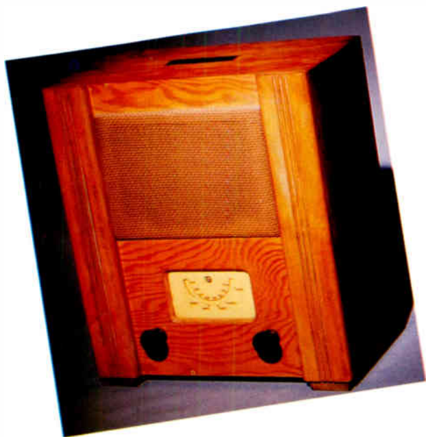
Britain's Wartime Utility Set of 1944 was produced to a cheap, standard design under government direction. Mains. 54.2cm x 50.4cm x 16.5cm (15½" x 12" x 6½").
