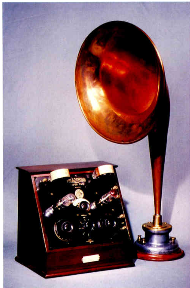
Fellophone Super Two battery receiver in mahogany case with ebonite front and brass fittings. Shown with a TMC loudspeaker. British. 1923. 30.4cm × 30.4cm × 22.8cm (12" × 12" × 9").
