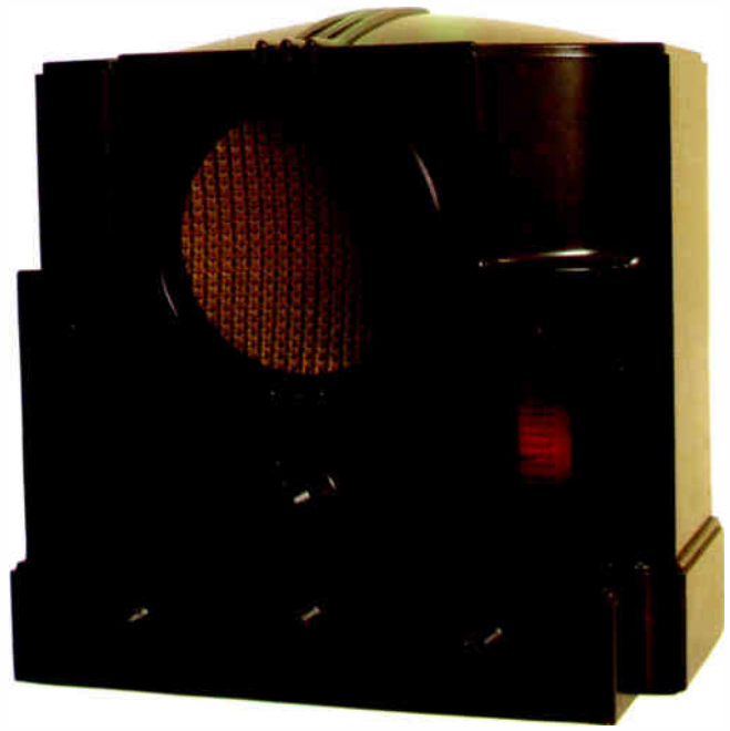
The art deco style 1955 Bruan bakelite Defiant two-valve mains radio, made for the Co-operative Wholesale Society, was thus named because it defied the radio industry's price-fixing system by offering a dividend to customers. 51.7cm × 55cm × 20.5cm (12½" × 15" × 8").
