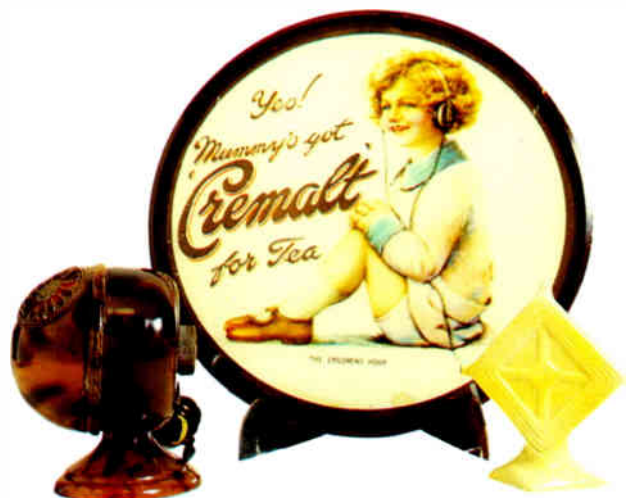
The Magnora miniature loudspeaker (left) in celluloid plastic, with earphone-type drive unit, claimed to be the smallest in the world in 1924. British. 8.8cm (3½") high and 6.3cm (2½") diameter. Pictured here with a contemporary advertising plaque in glass and a china ornament frame-aerial.
