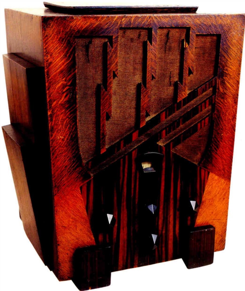
British Amplion three-valve mains receiver in an art deco style cabinet made up from oak and rosewood veneered plywood and large sawn-out sections of solid mahogany. British. 1952. 49.5cm × 45.1cm × 8.8cm (19½" × 17" × 3½").
