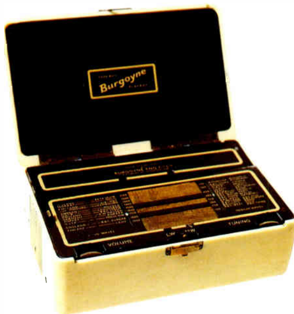
Typical of the personal portables introduced as a result of the development of low-consumption miniature valves, was this 1947 American battery radio called the Burgoyne Playboy, measuring only 6.3cm × 17.7cm × 11.4cm (2½" × 7" × 4½"). Presented in attractive plastic cases, such radios were aimed at an increasingly affluent youth market which was becoming increasingly mobile and demanded music on the move.
