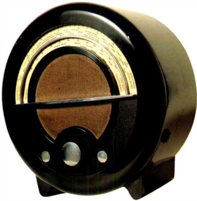
The British 1955 four-valve mains AD76 radio was a variation on the famous AD65 round Ekeo radio and came in brown or green bakelite or the slightly more expensive black-and-chrome version illustrated. 40.6cm (16") diameter × 20.5cm (8") deep.
