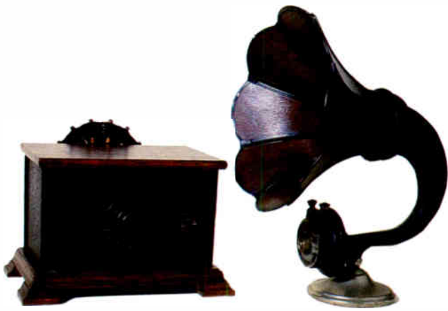
Pye two-valve Model 222 in solid oak case with black crystalline metal front. Coils plugged into the back increased waveband coverage. British. 1926. 17.7cm × 27.9cm × 17.7cm (7" × 11" × 7"). Shown with a wood-borned Amplion Junior Dragon loudspeaker, 58.1cm (15") high.
