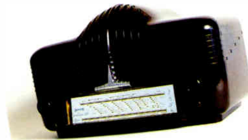
The 1947 Sonora Excellence 301, designed in the USA for the French market, looks like a big American car. Mains. 26.6cm x 45.7cm x 22.8cm (10½" x 18" x 9").
