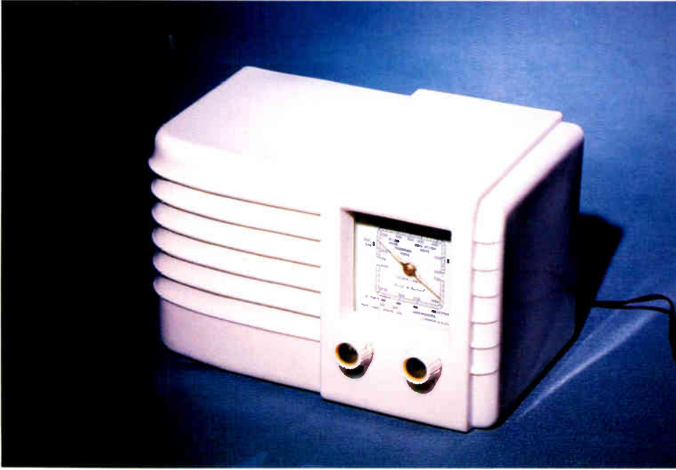
British McMichael four-valve mains radio c. 1950 in a sprayed bakelite cabinet.
