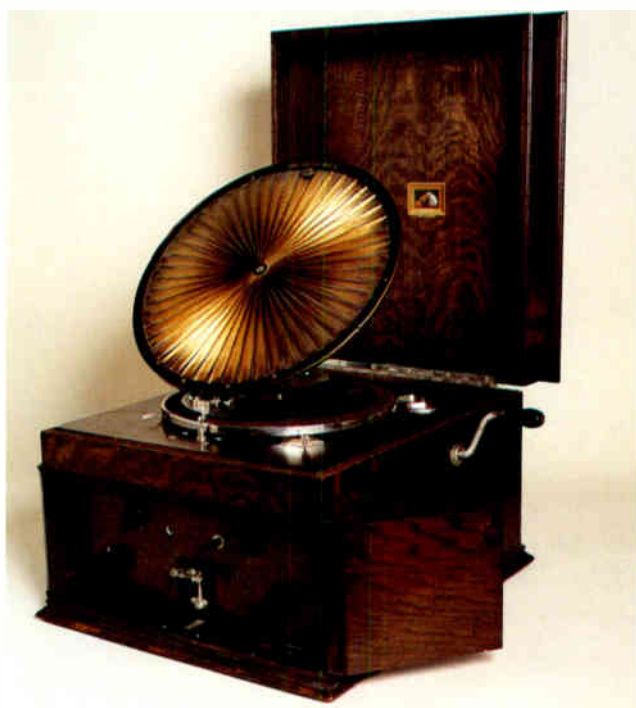
The world's first radiogram: an acoustic windup HMV gramophone with a crystal set built into the front. When wireless reception was desired the playing stylus which actuated the Lumière pleated Speaker was placed on a magnetic transducer connected to the crystal set. Oak. British. 1924. 58cm x 45.7cm x 45.7cm (15" x 18" x 18").
