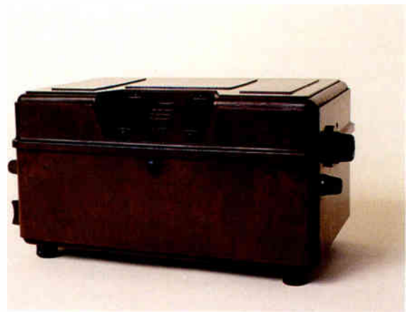
The 1950 British Philips three-valve mains type 2531 in its plain bakelite cabinet was unusual among its ornate wooden contemporaries. It needed an external loudspeaker. 17.7cm × 55.5cm × 20.5cm (7" × 14" × 8").
