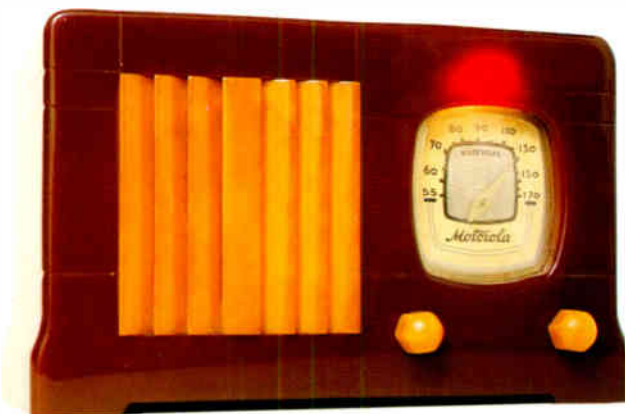
American Motorola midget radio of 1959 with hand-cast cabinet in polished translucent Catalin plastic, produced in several colours. 15.2cm x 24.1cm x 11.4cm (6" x 9 1/2" x 4 1/2").
