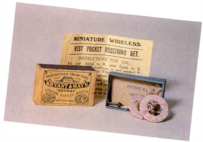
The Radiax/Samuel's Miniature Wireless Marvel of 1925 needed bulky earphones and a long outdoor aerial to pick up even a clove station. British. 5.8 cm x 5.7cm x 5.8cm (1½" x 2¼" x 1½").
