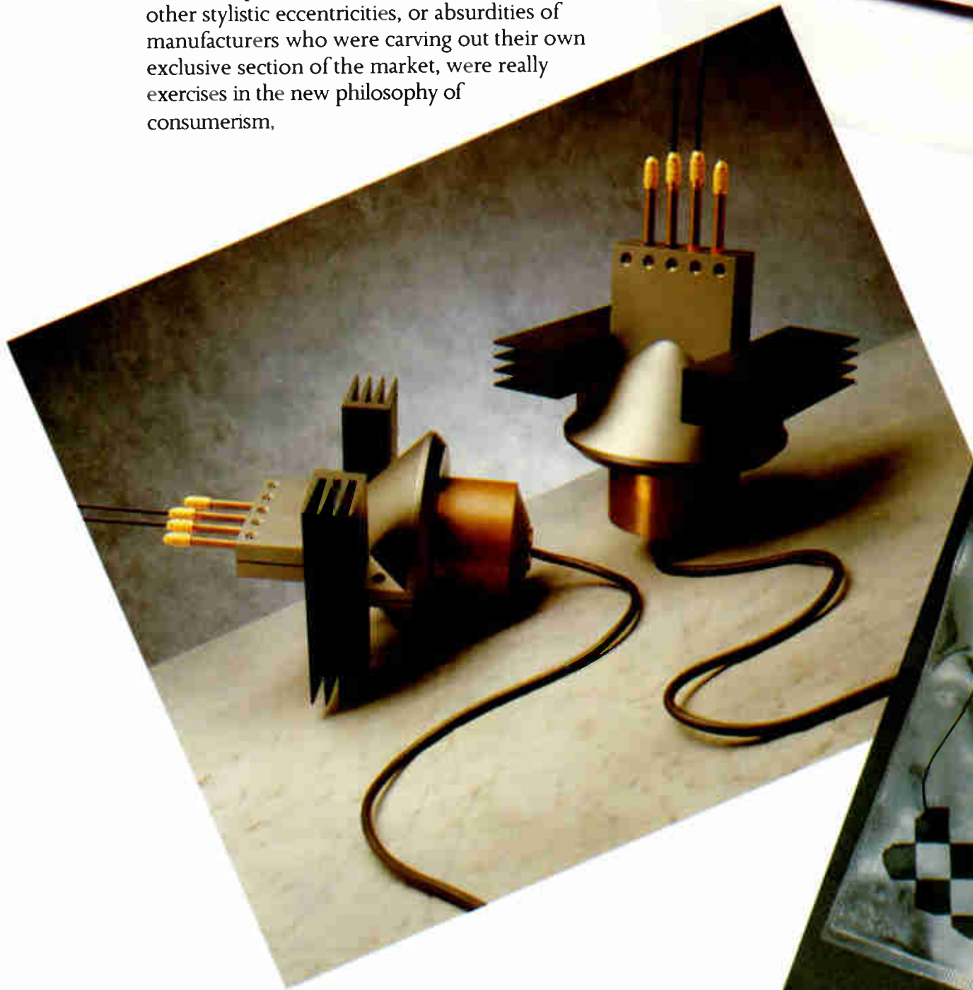
These Space-Age style hi-fi power amplifiers in aluminium and copper by Pirate Design Associates, manufactured by Be³W Loudspeakers UK, make a stylistic virtue of technological necessity: the finned structures are needed for cooling. 54.9cm x 24.6cm (15 3/4" x 9 7/8").
