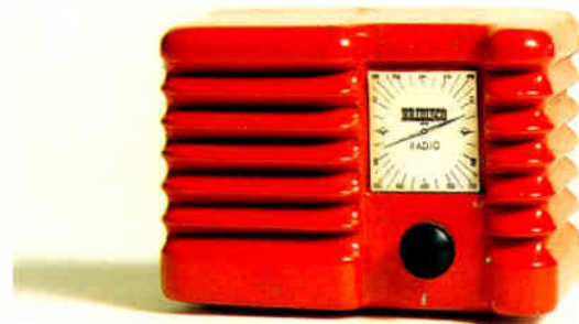
The 1957 British Marconi P60B (also HMV 1410G) used a combination of two of the old-fashioned valves and two of the new transistors. 15.2cm x 19cm x 7.6cm (6" x 7½" x 3").
