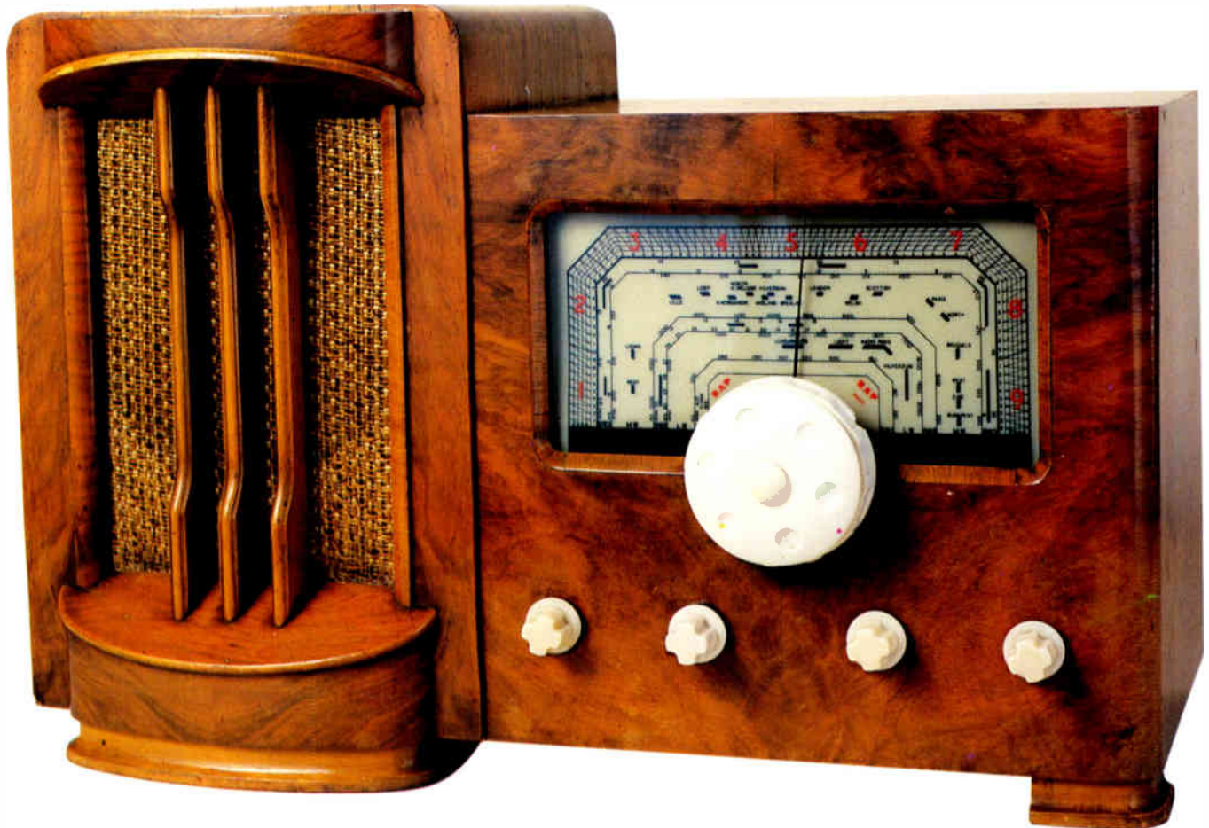
This 1946 British RAP radio had a plain wooden box with a large dial, coupled with a curiously outdated Odeon-style loudspeaker, a chrome-plated chassis and a glass back so the customer could see the works. 55cm x 45.7cm x 22.8cm (15" x 18" x 9").
